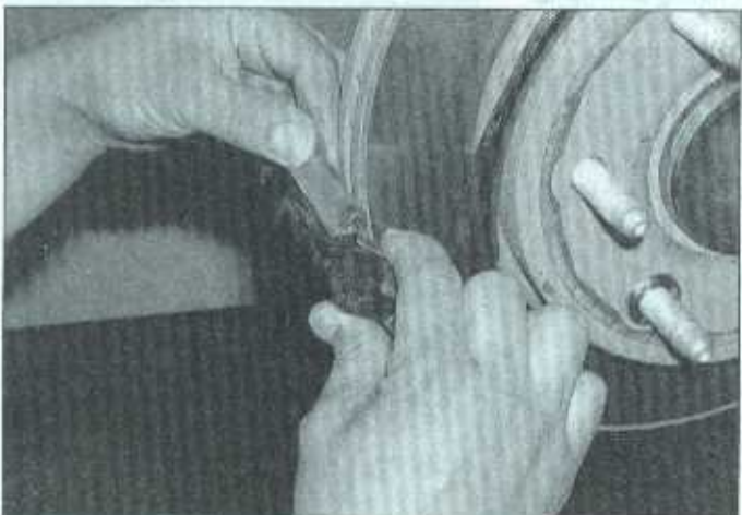
3.5i Install the upper and lower pad retainers on the caliper mounting bracket
