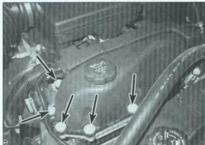
4.7 Front valve cover bolt locations (there are six total in front) - make sure all perimeter bolts are removed before attempting to remove the cover
