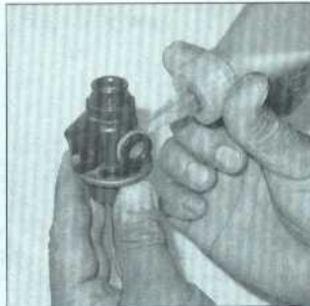
13.8 Lubricate the O-ring with clean engine oil
