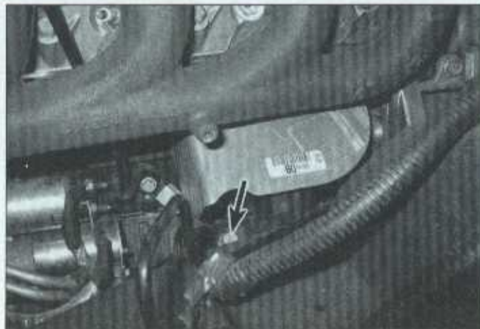
18.9 One of the three engine mount-to-frame bolts, seen from above
