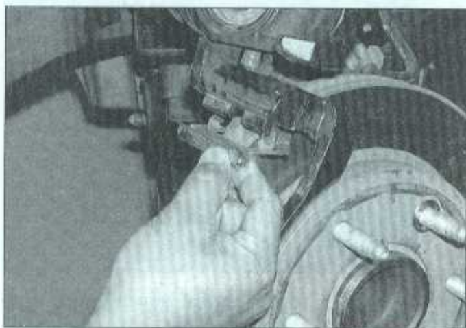
3.5g Remove the upper and lower pad retainers from the caliper mounting bracket; if they are cracked or distorted, replace them
