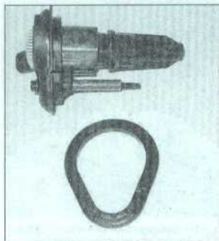
7.10 Install new seal(s) on the ignition coil(s) if they are damaged or hardened
