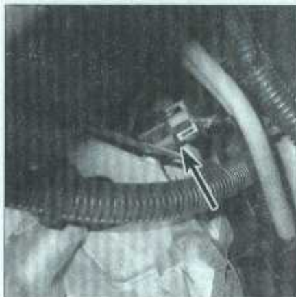
9.4 The Crankshaft Position (CKP) sensor is located at the left rear of the engine block on inline engines
