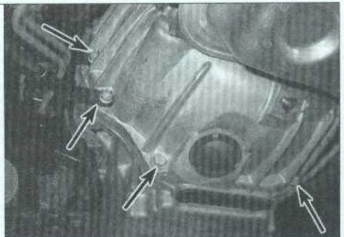
8.18 Remove the bellhousing bolts (lower and left side shown)
