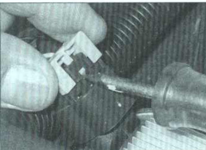
26.6 Use a pointed tool to depress the tab while pulling up the locking part of the ignition coil connector, then disconnect the electrical connector
