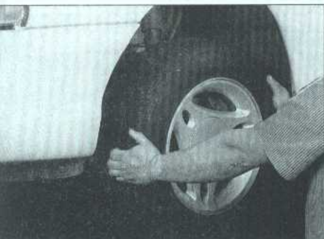
27.11 With the steering wheel in the locked position and the vehicle raised, grasp the front tire as shown and try to move it back-and-forth - if any play is noted, check the steering gear mounts and tie-rod ends for looseness
