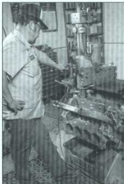
1.1 An engine block being bored. An engine rebuilder will use special machinery to recondition the cylinder bores.
