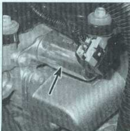
16.2 The camshaft position actuator solenoid is located at the right front corner of the cylinder head on inline engines
