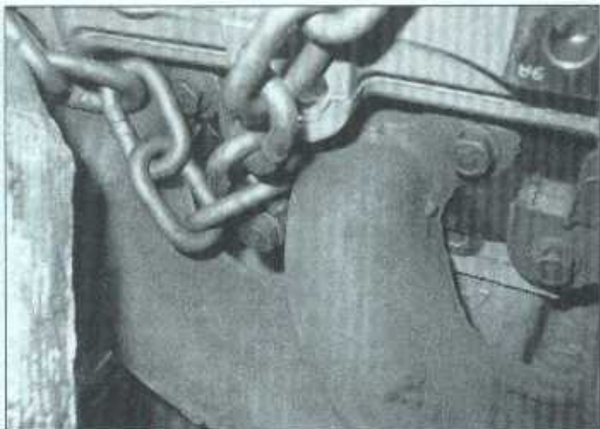
7.25b ... and to the cylinder head at the right rear of the engine (use a bolt that is longer than the original exhaust manifold bolt and a washer, if necessary). As an alternative, you can wrap the chain around one of the manifold runners and bolt it together
