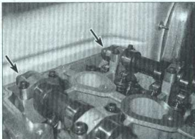
7.14 When the engine is at Top Dead Center for cylinder number one (on the compression stroke), the flats at the rear ends of the camshafts will be facing up, parallel with the top of the cylinder head (the camshaft holding tool engages these flats)
