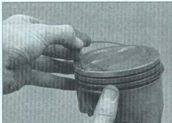
9.19b DO NOT use a piston ring installation tool when installing the oil control ring side-rails
