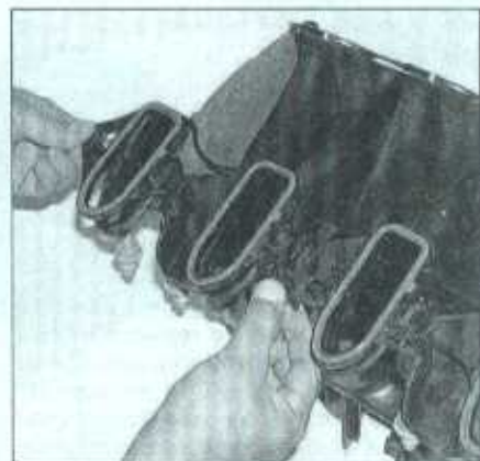
7.12 Align the tabs on the intake gaskets with the tabs on the manifold and snap the gasket into place
