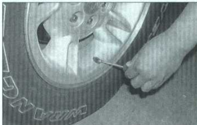
5.4a If a tire loses air on a steady basis, check the valve stem core first to make sure it's snug (special inexpensive wrenches are commonly available at auto parts stores)
