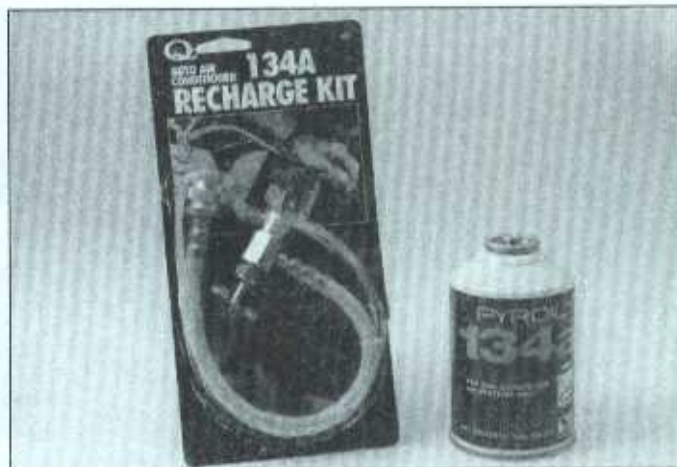
13.18 A basic charging kit for 134a systems is available at most auto parts stores - it must say 134a (not R-12) and so must the can of refrigerant
