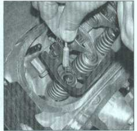
6.8 Once the spring is depressed, the keepers can be removed with a small magnet or needle-nose pliers (a magnet is preferred to prevent dropping the keepers)
