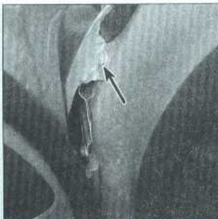
13.3c With the door open, remove this bolt at the top-rear of the fender
