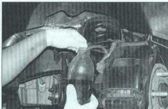
10.8 When bleeding the brakes, a hose is connected to the bleed screw at the caliper and then submerged in brake fluid - air will be seen as bubbles in the tube and container (all air must be expelled before moving to the next wheel)
