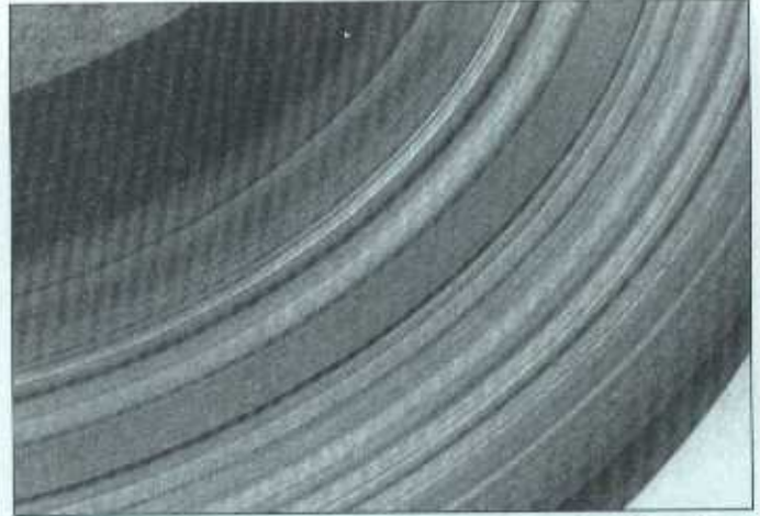
5.3 The brake pads on this vehicle were obviously neglected, as they wore down completely and cut deep grooves into the disc - wear this severe means the disc must be replaced
