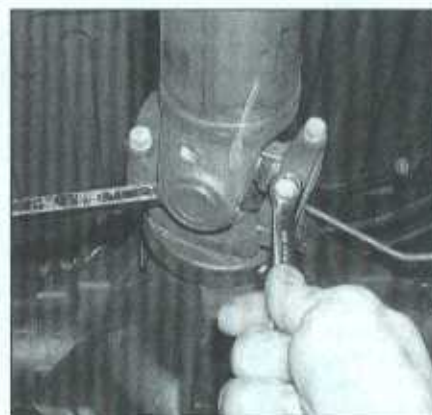
10.3 Insert a screwdriver or prybar through the driveshaft yoke to prevent the shaft from turning when you loosen the bolts
