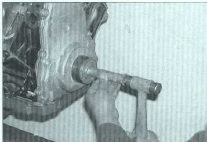
11.4 Drive the new seal into place with a large socket and hammer
