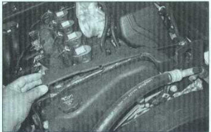
4.5 Carefully pry open the cover over the engine harness and set the harness aside
