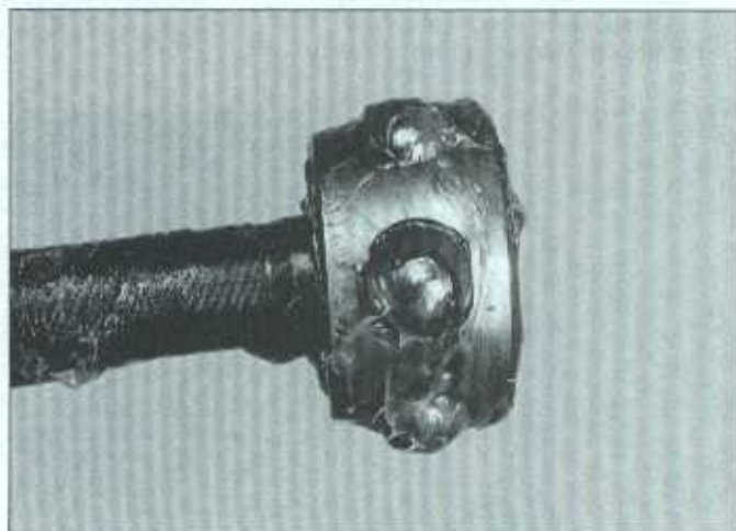
20.3l Install the inner race and cage assembly with the bulge facing the end of the axle shaft
