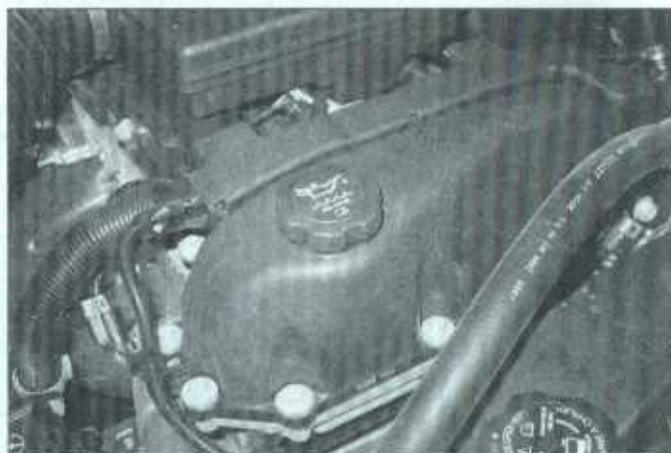
4.6 Oil is added to the engine after unscrewing the oil filler cap - always make sure the area around the opening is clean before removing the cap to prevent dirt from contaminating the engine
