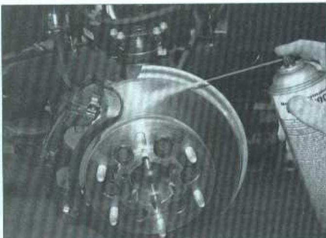
3.5a Before disassembling the brake, wash it thoroughly with brake system cleaner and allow it to dry - position a drain pan under the brake to catch the residue - DO NOT use compressed air to blow off brake dust!
