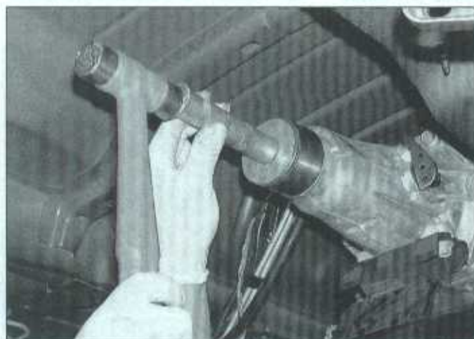
6.5 Drive the new seal into place with a seal driver or a large socket and hammer
