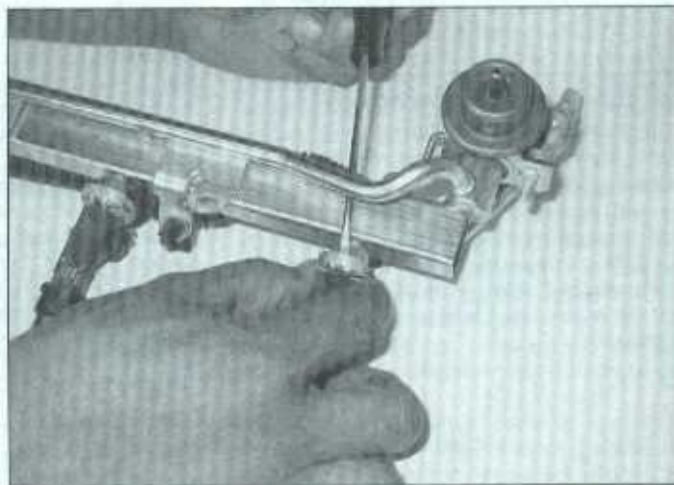
14.12 The retaining clip must be removed prior to removing the injector
