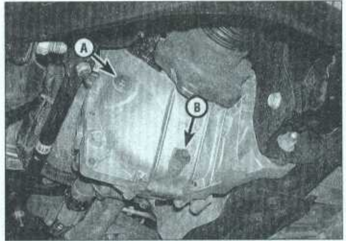
16.2b Remove the front (4WD) axle filler plug (A) to check the differential lubricant level - B is the drain plug (typical)
