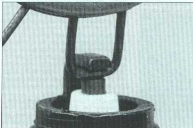
26.5a The manufacturer recommends using a wire-type gauge to check the spark plug gap - if the wire doesn't slide between the electrodes with a slight drag, adjustment is required
