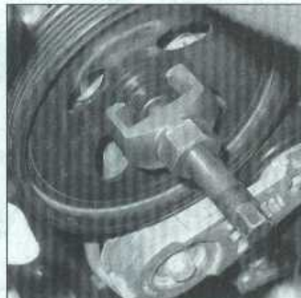
21.4 Remove the pulley from the power steering pump with a pulley removal tool
