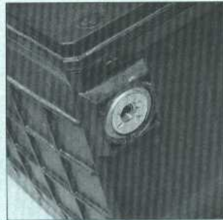
11.7c Regardless of the type of tool used on the battery and cables, a clean, shiny surface should be the result
