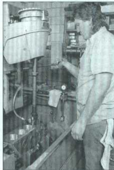
1.2 If the cylinders are bored, the machine shop will normally hone the engine on a machine like this
