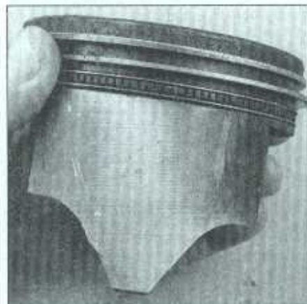
1.6 Uneven piston wear like this indicates a bent connecting rod
