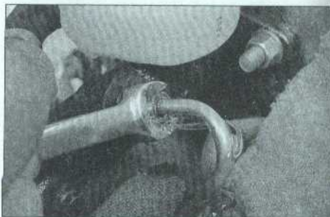
8.16 Have an assistant depress the brake pedal and hold it down, then loosen the fitting nut, allowing air and fluid to escape; repeat this procedure on both fittings until the fluid is clear of air bubbles
