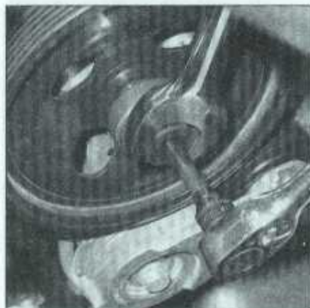
21.7 Press the pulley onto the shaft using a pulley installation tool - don't attempt to drive it on with a hammer or push it on with a traditional press!
