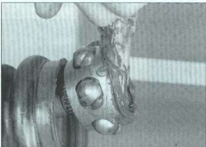
20.3m Pack CV joint grease into the bearing until it's completely full, then assemble the outer race onto the inner race and install the retaining ring. Caution: Don't use any other kind of grease
