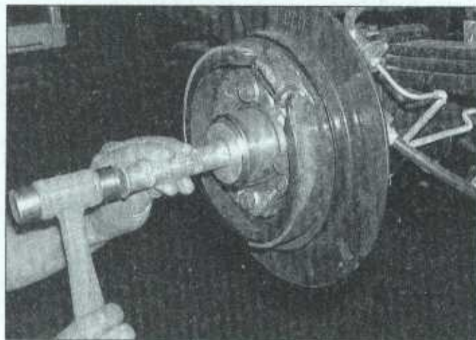
15.4 Use a bearing driver or a large socket to tap the bearing evenly into the axle housing
