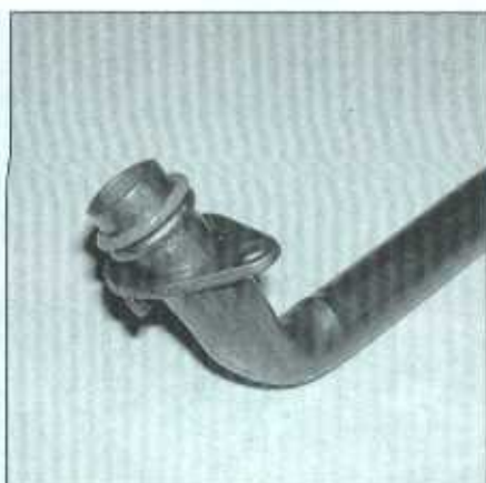
15.8 Always install a new O-ring on the oil pump pick up tube
