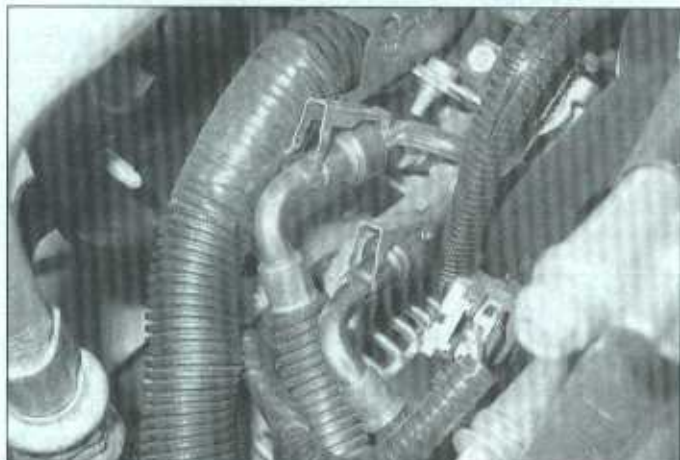
4.11c To disconnect a metal collar type fitting, remove the safety tether from the fitting . . .
