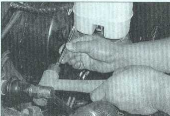
8.19 Driving out the roll pins that retain the master cylinder fluid reservoir
