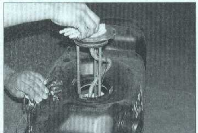
7.6 Carefully remove the fuel pump module from the tank and drain the fuel from the reservoir
