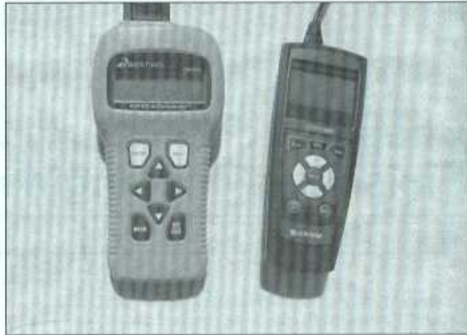
2.2 Scanners like these from Actron and AutoXray are powerful diagnostic aids - they can tell you just about anything that you want to know about your engine management system
