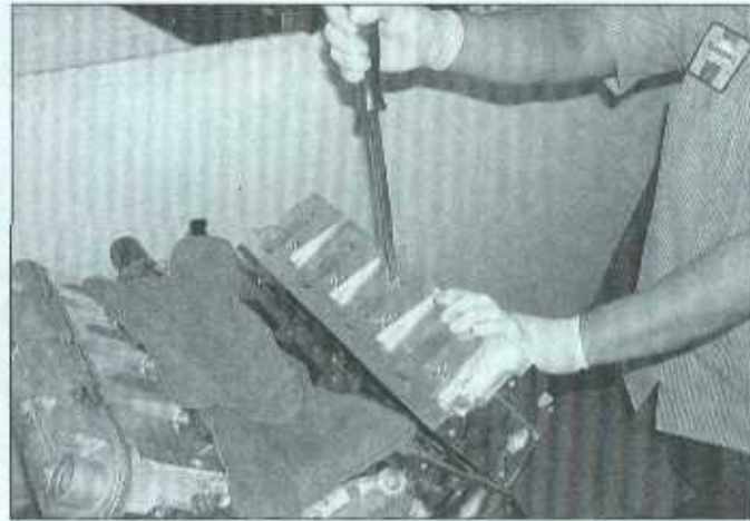
9.12 Using a prybar inserted into an intake port to break the head loose - do not use excessive force or damage to the head may result
