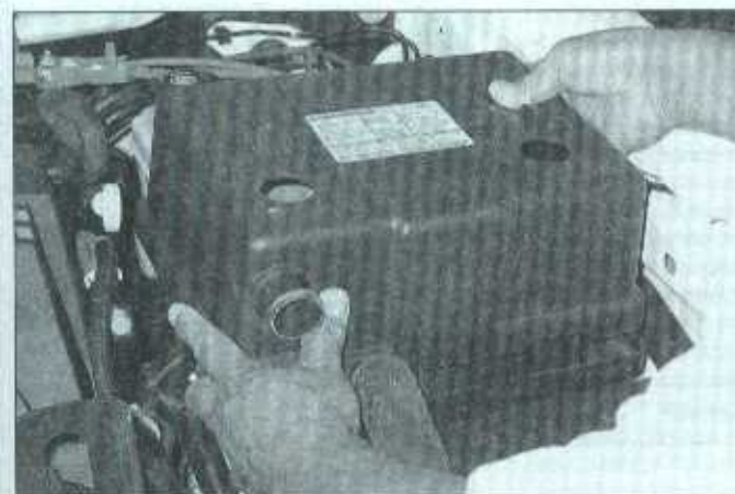
3.7 Depress the clips on each side of the battery cover, then lift the cover straight up
