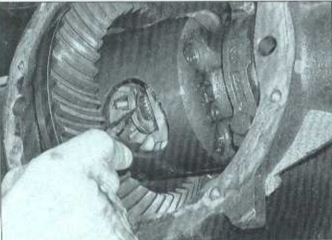
13.5a Push the axle flange in, then remove the C-lock from the inner end of the axleshaft
