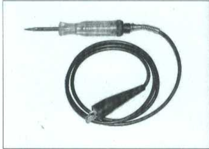
2.5b A test light is a very handy tool for checking voltage
