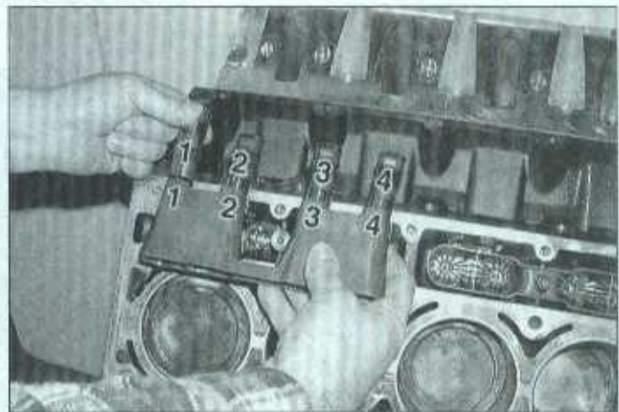
13.13b Once the lifters and retainers are removed from the block they can be marked (for location and installation purposes) and inspected
