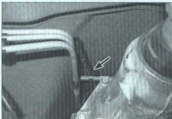
8.13 Disconnect the vent hose from the transmission
