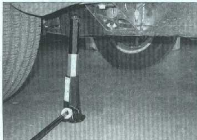
Front jacking location - make sure the jack head securely engages the pocket in the frame
