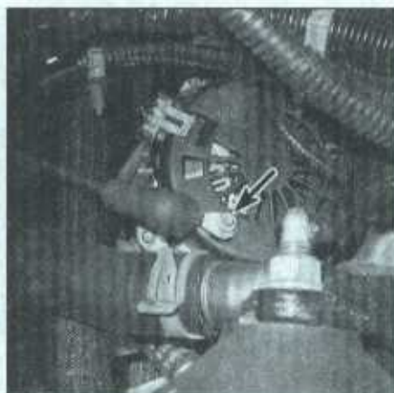
4.4b Disconnect the lead from the alternator
