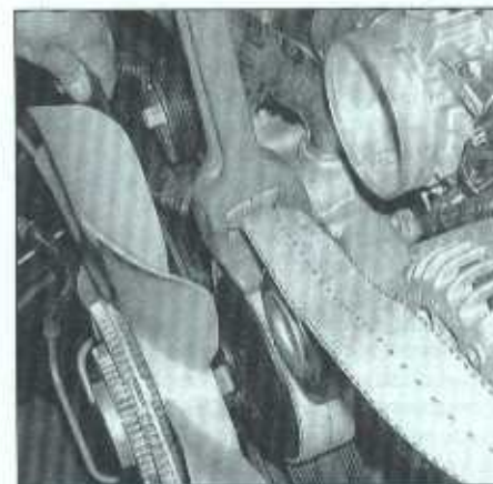
5.5 A strap wrench can be used to immobilize the water pump pulley while loosening the fan clutch hub
