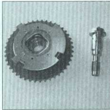
12.11 Camshaft position actuator system components - the "bolt" is the solenoid valve (it must be replaced with a new one whenever it's removed); don't try to disassemble the actuator mechanism
