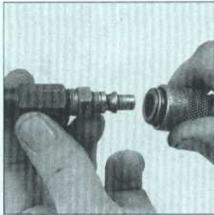
6.5 Thread the air hose adapter into the spark plug hole - adapters are commonly available from auto parts stores
