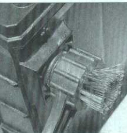
11.7a A tool like this one (available at auto parts stores) is used to clean the side-terminal type battery-cable contact area
