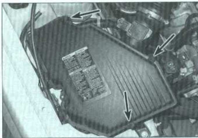
24.3a Loosen the screws and lift the air filter housing cover off
