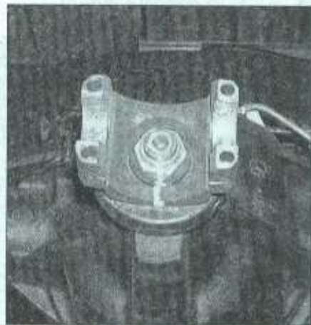
16.4 Before removing the nut, mark the position of the flange to the shaft and count the number of exposed threads
