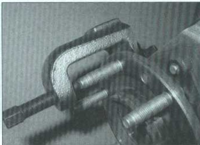
10.3 Use a small press tool such as this to push the stud out of the flange
