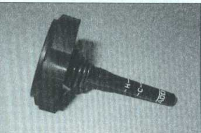
6.6 The power steering fluid dipstick has marks on it so the fluid can be checked hot or cold
