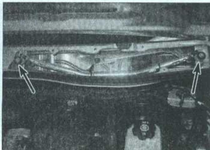
18.9 Remove the wiper linkage mounting bolts, then twist or rock the assembly out from the cowl
