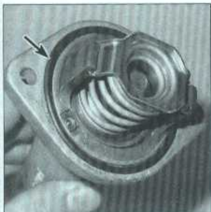
3.11 After the housing is cleaned, or a new thermostat/housing is used, a new O-ring should always be used
