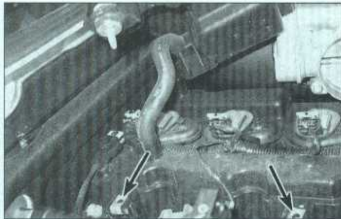
3.2 Pry up the resonator box until its pins come loose from the clips
