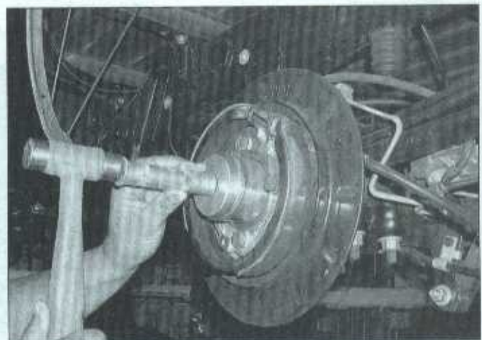
14.3 Using a seal driver to install the axleshaft oil seal - drive the seal in until it's flush with the bore
