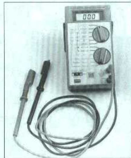
2.3 Digital multimeters can be used for testing all types of circuits; because of their high impedance, they are much more accurate than analog meters for measuring low-voltage computer circuits
