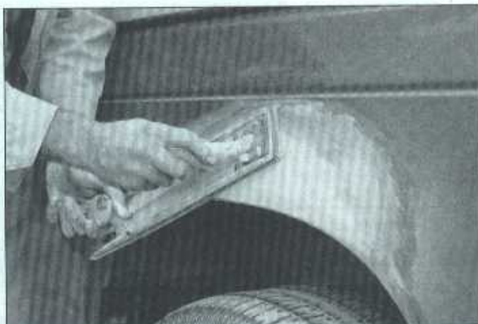
8 Use coarse-grit sandpaper and a sanding board or block to work the filler down until it's smooth and even. Work down to finer grits of sandpaper - always using a board or block - ending up with 360 or 400 grit
