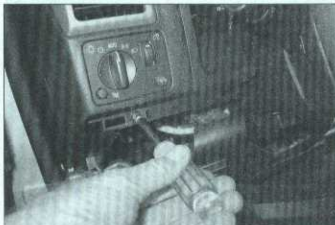
10.3 Remove the headlight switch mounting screw
