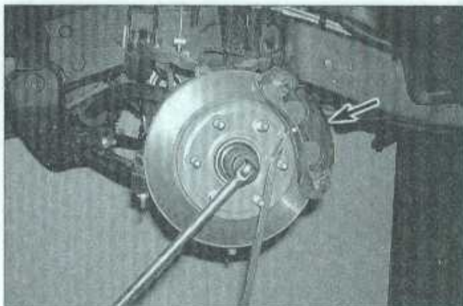
19.4 A large prybar can be used to immobilize the hub while loosening the nut, or a screwdriver can be inserted through the window in the brake caliper (arrow) and into the disc cooling vanes
