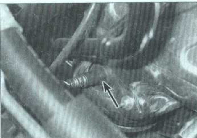
11.9a Location of the engine monitoring (pre-catalyst) oxygen sensor, at the bottom of the exhaust manifold
