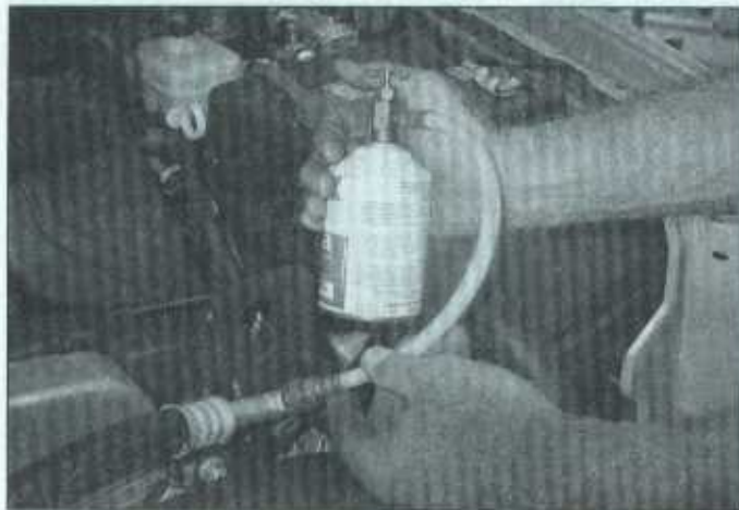
13.21 Attach the refrigerant kit to the low-side charging port - the cap may be marked with an "L"
