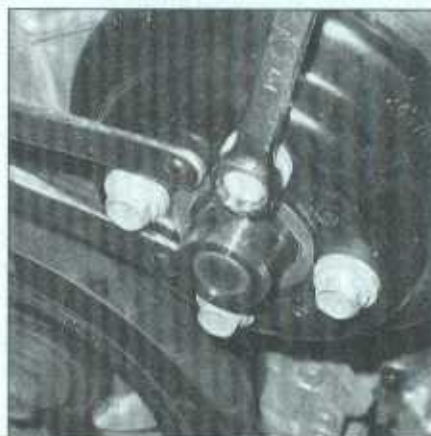
7.10 To remove the water pump pulley, prevent it from turning with a pin spanner (or a strap wrench wrapped around the pulley) and unscrew the bolts - inline engines only
