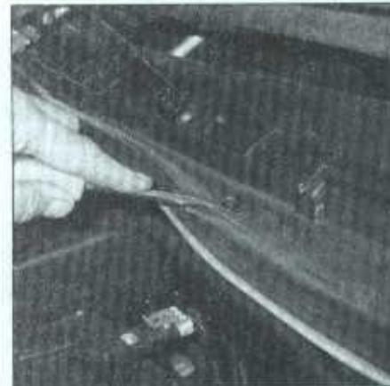
14.3 Remove the cowl cover pushpins
