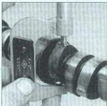
8.8 Measuring cam lobe height with a micrometer - make sure you move the micrometer to get the highest reading
