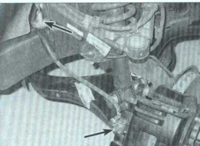
19.11 Check along the brake hoses and at each fitting for deterioration, cracks and leakage
