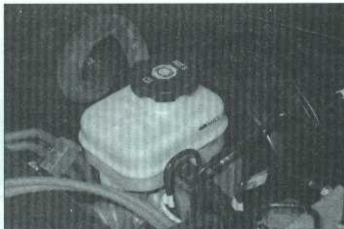
4.19 Never let the brake fluid level drop below the MIN mark
