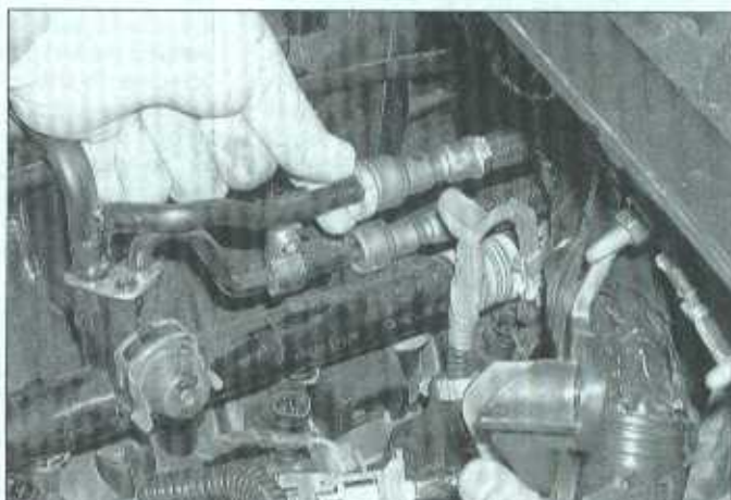
4.11d . . . place the tool over the fuel line, insert it squarely into the fitting and pull the lines apart (the tool is not required to connect the lines)
