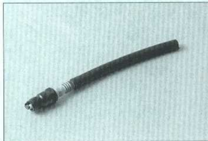
26.10 A length of snug-fitting rubber hose will save time and prevent damaged threads when installing the spark plugs
