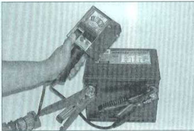
3.3 Connect a battery load tester to the battery and check the battery condition under load following the tool manufacturer's instructions
