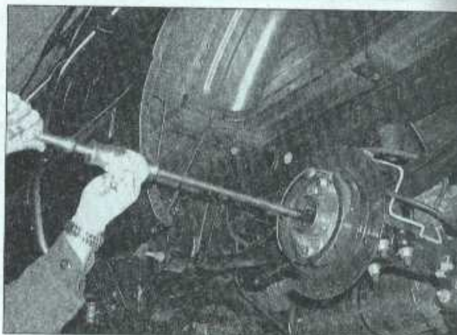
15.3 Removing the axleshaft bearing with a slide hammer
