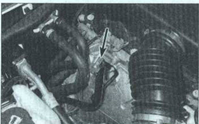
7.3 The automatic transmission dipstick is located at the right rear of the engine compartment - flip up the handle before pulling out the dipstick
