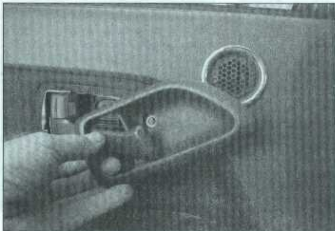
15.3 Remove the screw and slide the door handle bezel off
