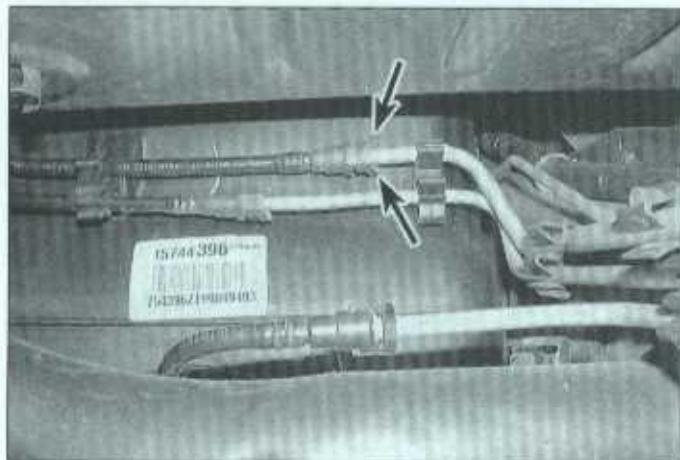
4.11a To disconnect a plastic collar two-tab type fitting, squeeze the two tabs together and pull the lines apart
