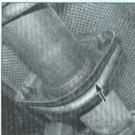
20.2b Inspect all flanged joints for signs of exhaust gas leakage
