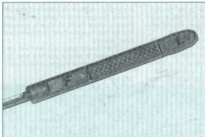
4.4 The oil level must be maintained between the marks at all times - it takes one quart of oil to raise the level from the L mark to the F mark
