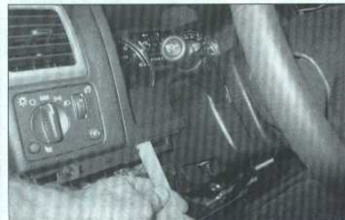
23.10 Pry up the instrument cluster bezel with a trim tool
