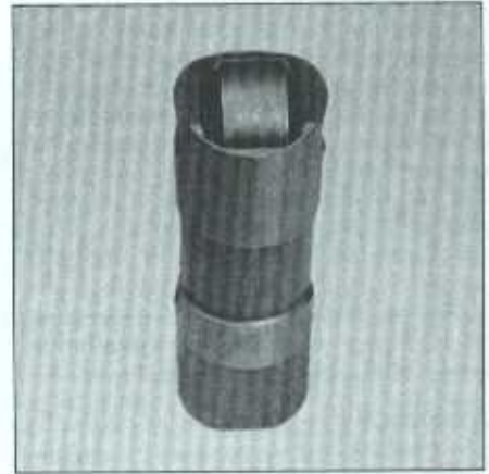
13.24 The roller on hydraulic roller lifters must turn freely - check for wear and excessive play as well
