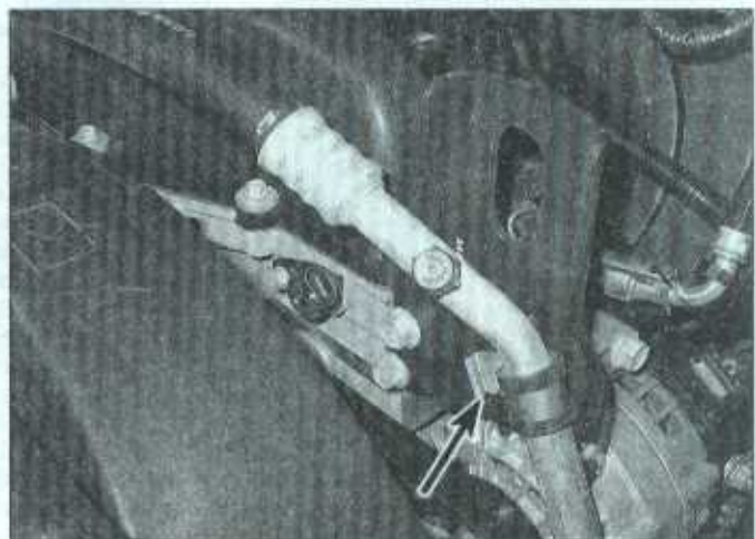
10.4 Unbolt and set aside the refrigerant hose, then remove the engine lifting bracket - inline engine
