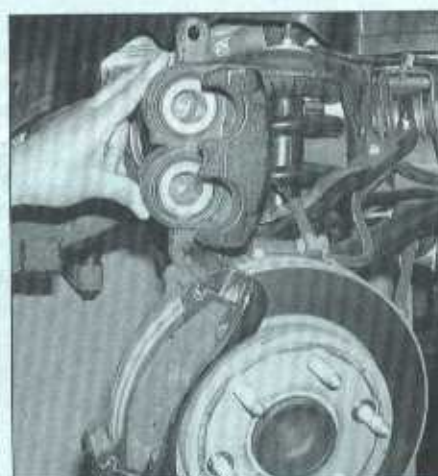
3.5d Remove the lower mounting bolt and pivot the caliper up, supporting it in this position
