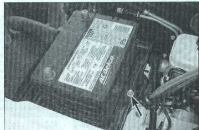
3.8 Remove the nut and retainer, then lift the battery out
