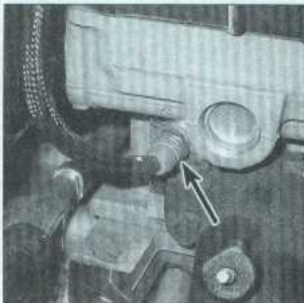
8.4 ... the sensor itself is threaded into the cylinder head at the right-rear on inline engines
