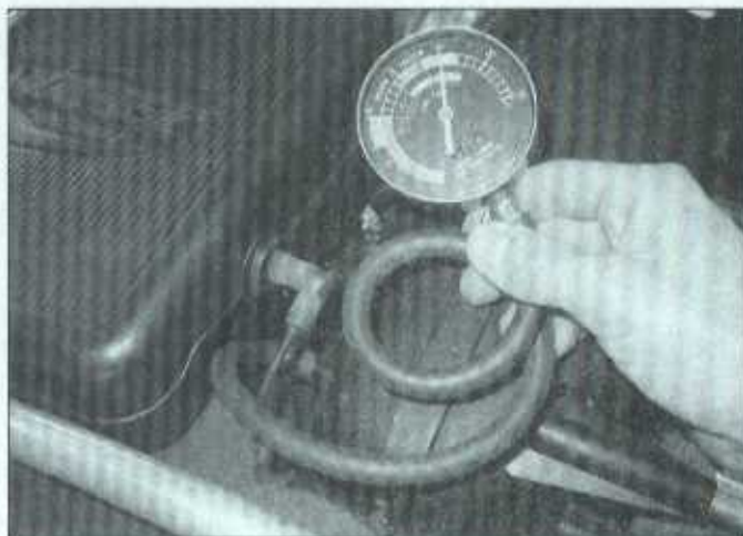
3.17 An inexpensive vacuum gauge can tell you a lot about an engine's condition
