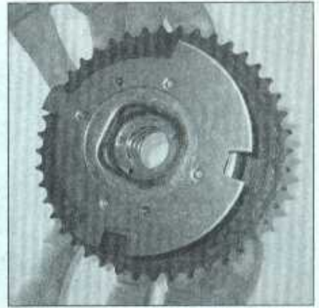
12.12 Place your fingers as shown when pulling the actuator from the end of the camshaft - don't pull on the reluctor ring as it could pop apart and be destroyed
