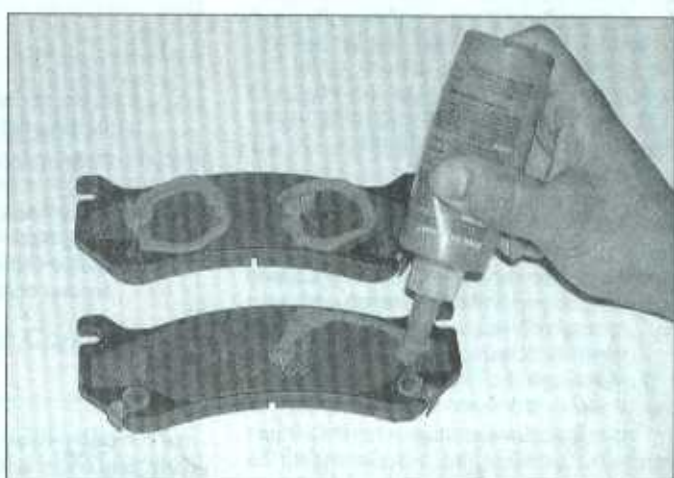
3.5h Apply anti-squeal compound to the back of both pads (let the compound set up a few minutes before installing them)
