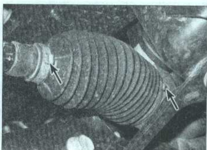
19.3 Cut the steering gear boot clamps off with a pair of side cutters
