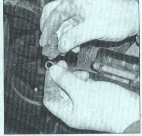
4.2 There is a sealing washer on either side of the brake hose inlet fitting; be sure to replace these with new ones when reconnecting the hose
