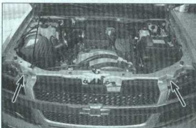
9.2a Release the grille clips (two indicated here) with a screwdriver
