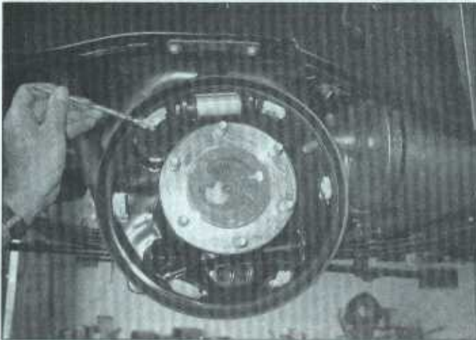
6.4i Clean the backing plate with brake cleaner and lightly lube the shoe contact points with brake grease
