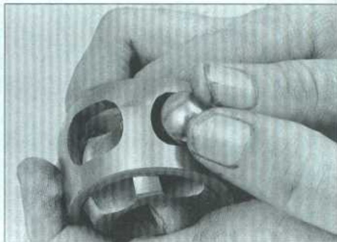
20.3j Press the balls into the cage through the windows
