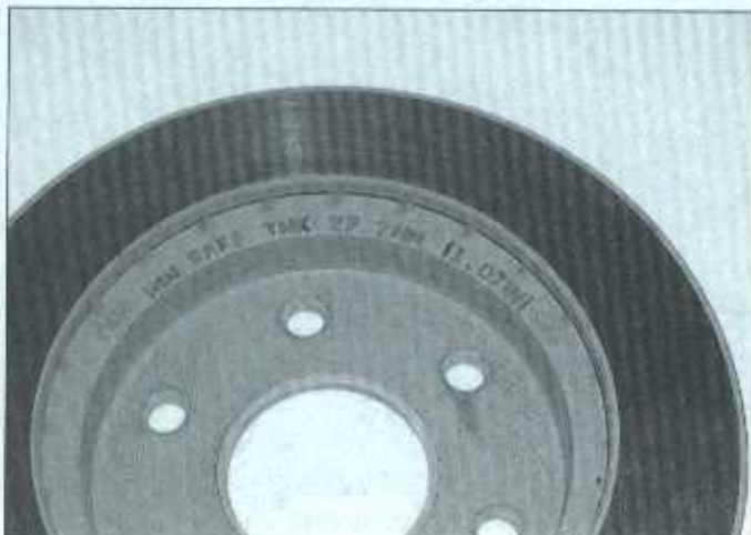
5.5a The minimum thickness is cast into the disc (typical)
