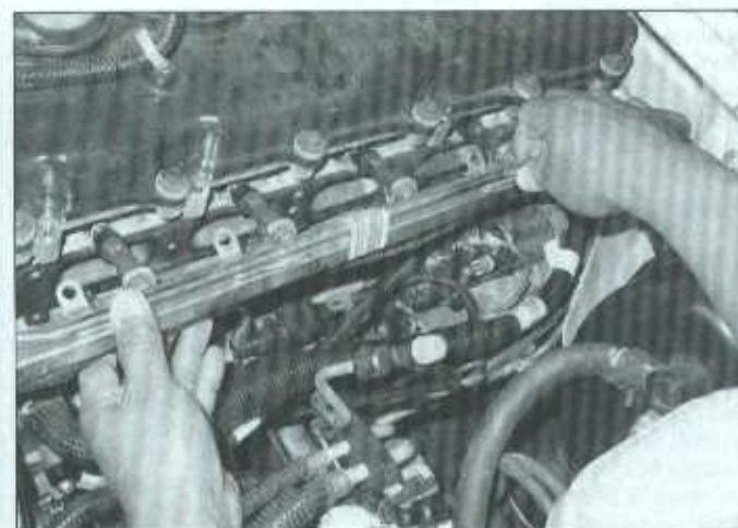
14.10 The fuel rail and injectors are removed as a unit, then the individual injectors can be serviced
