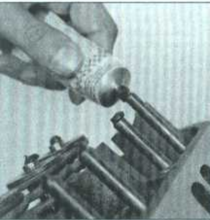
5.9 Lubricate the pushrod ends and the valve stems with engine assembly lube before installing the rocker arms
