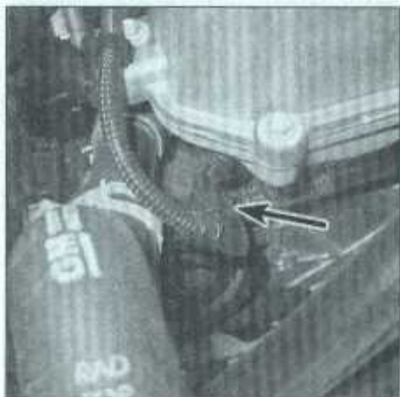
10.3a The exhaust Camshaft Position Sensor (CMP) is located at the right front corner of the cylinder head on inline engines
