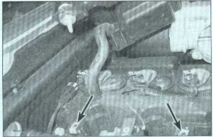
9.5 Pull up the air intake resonator box until its two pins release from the clips on the engine (inline engine)
