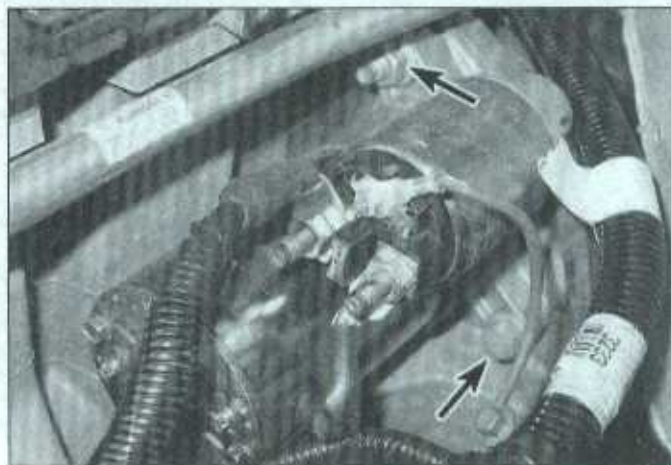
13.4 Remove the starter mounting nut and bolt - inline engine
