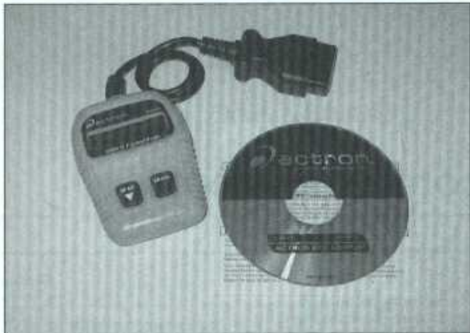
2.1 Simple code readers are an economical way to extract trouble codes when the CHECK ENGINE light comes on
