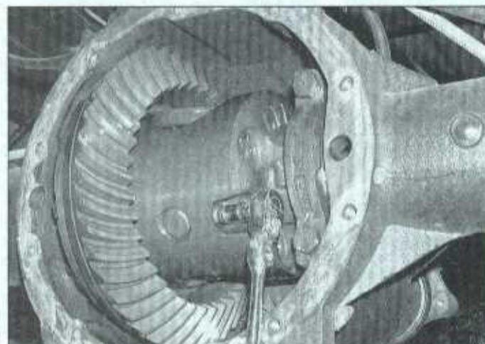
13.3 Remove the pinion shaft lock bolt
