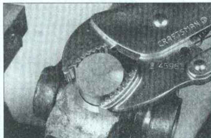
11.5 Locking pliers can be used to remove the bearing caps from the yoke
