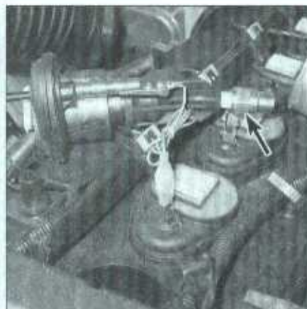
7.4 To use a calibrated ignition tester, remove an ignition coil, connect the tester to the spark plug boot and clip the tester to a convenient ground, then crank the engine over
