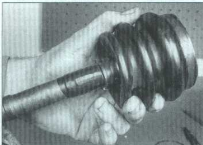
20.3k Wrap the axle shaft splines with tape to avoid damaging the boot, then slide the small clamp and boot onto the axle shaft
