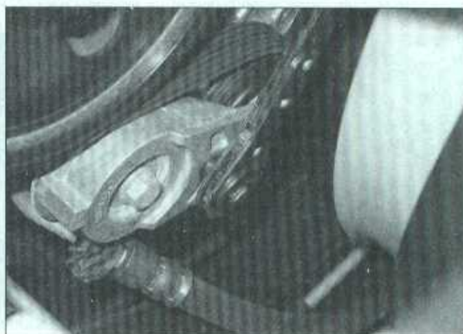
12.5 Use a drivebelt tool to turn the tensioner clockwise for belt removal (there may not be room for a standard ratchet or breaker bar)
