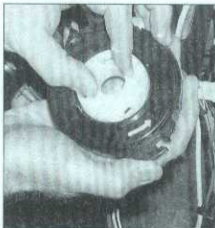
15.12 To center the clockspring on models with a spring lock tab, hold it with its underside facing up, depress the spring lock and rotate the hub in the direction of the arrow until it stops, then turn it in the opposite direction 2-1/2 turns
