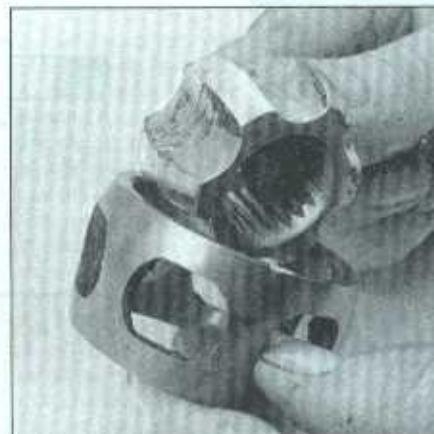
20.3g Tilt the inner race 90-degrees and rotate it out of the cage
