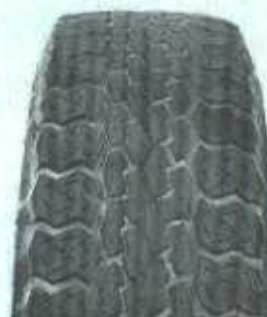
FEATHERING DUE TO MISALIGNMENT
