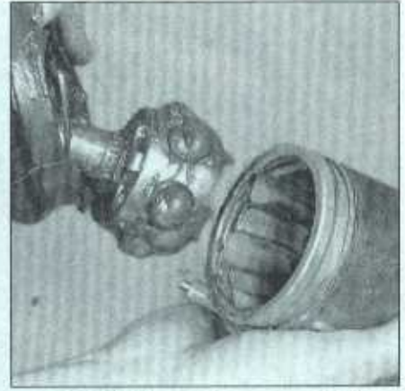
20.3c With the retainer removed, the outer race can be pulled off the bearing assembly
