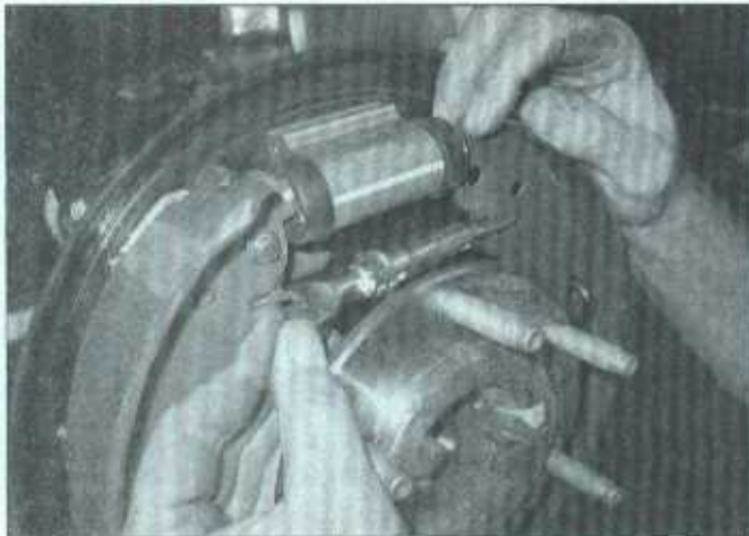
6.4m Clean and lube the threads of the adjuster and reinstall it between the shoes
