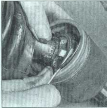
20.3b Pry the wire retainer ring from the CV joint housing with a small screwdriver
