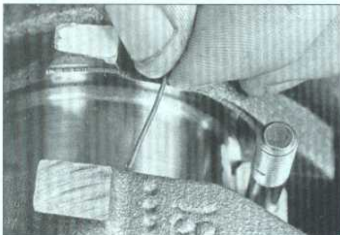
9.37 Place Plastigage on each connecting rod bearing journal parallel to the crankshaft centerline
