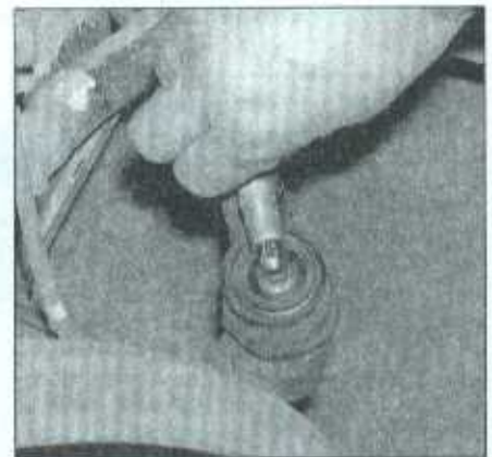
17.2 After cleaning the grease fitting, push the gun nozzle firmly into place and pump the grease into the component (usually about two pumps will be sufficient)
