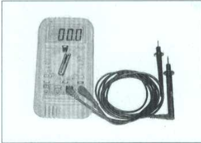
2.5a The most useful tool for electrical troubleshooting is a digital multimeter that can check volts, amps, and test continuity
