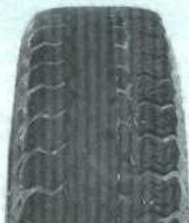
INCORRECT TOE-IN OR EXTREME CAMBER
