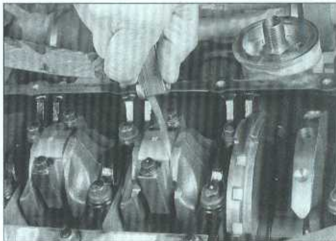
9.3 Checking the connecting rod endplay (side clearance) (typical)
