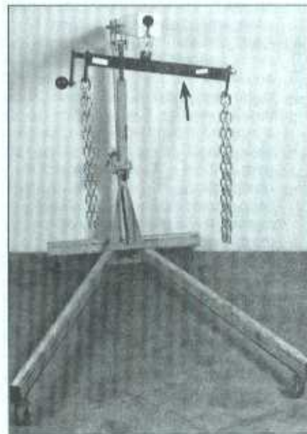
6.3 Get an engine hoist that's strong enough to easily lift your engine in and out of the engine compartment; an adapter, like the one shown here, can be used to change the angle of the engine as it's being removed or installed
