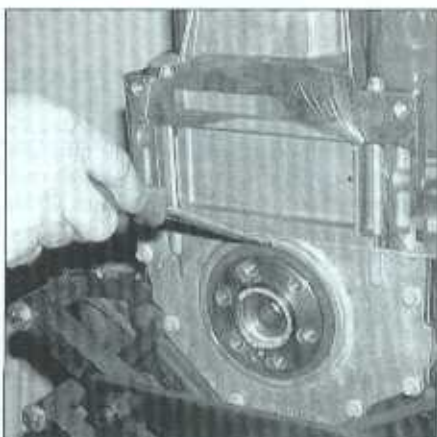
17.3 Carefully pry the old seal out with a screwdriver at the notches provided in the rear cover
