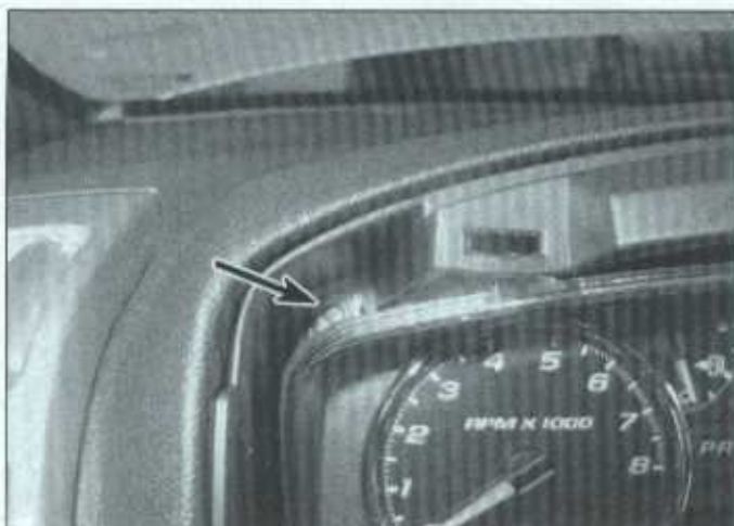
11.4a Instrument cluster upper mounting screws (left screw shown)
