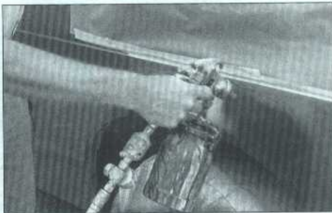
10 Apply several layers of primer to the area. Don't spray the primer on too heavy, so it sags or runs, and make sure each coat is dry before you spray on the next one. A professional-type spray gun is being used here, but aerosol spray primer is available inexpensively from auto parts stores
