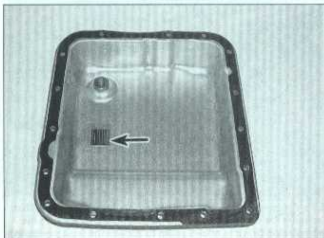
28.12 Clean the transmission pan, position the magnet back in place, and install the new pan gasket
