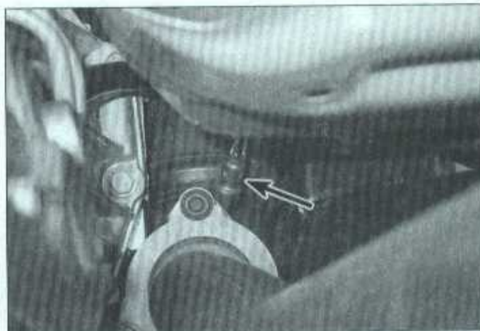
11.9b Location of the catalyst monitoring (post-catalyst) oxygen sensor, seen from below the vehicle
