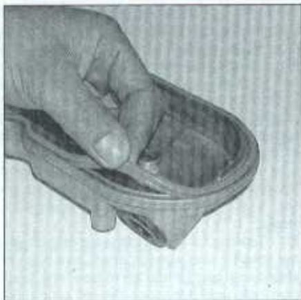
4.11 Position the new gasket in the valve cover lip
