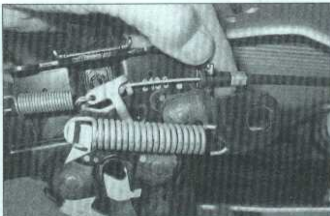
11.1 To disconnect the cable from the hood latch mechanism, detach the cable casing from the bracket, then unhook the cable end from the latch lever
