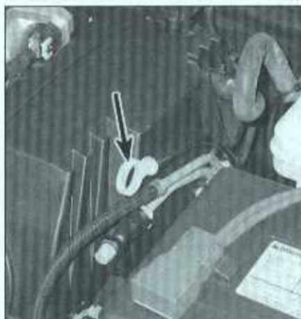
4.2 The engine oil dipstick is located along the right side of the engine
