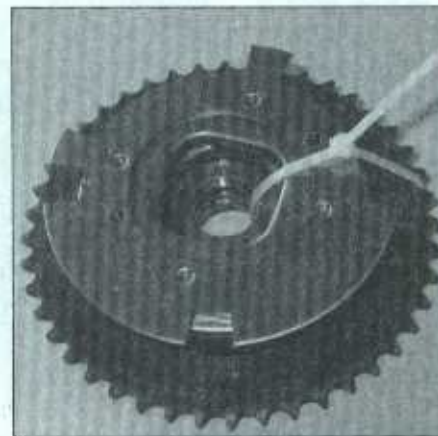
12.14 Secure the actuator with a wire tie or something similar to ensure that it doesn't come apart
