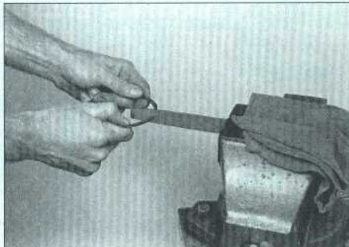
9.15 If the ring end gap is too small, clamp a file in a vise as shown and file the piston ring ends - be sure to remove all raised material
