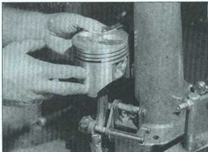
1.4 A machinist checks for a bent connecting rod using specialized equipment
