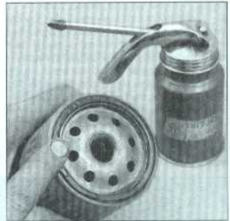
8.18 Lubricate the oil filter gasket with clean engine oil before installing the filter on the engine
