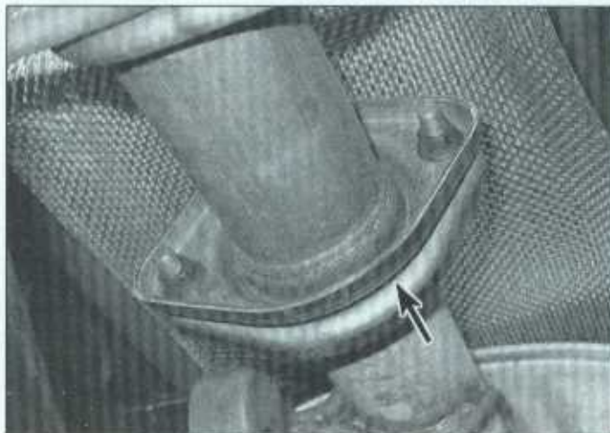
15.2a Inspect the exhaust system connections for leakage
