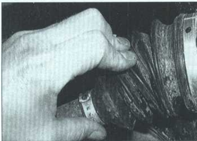
27.15 Inspect the inner and outer driveaxle boots on 4WD models for loose clamps, cracks or signs of leaking lubricant (inner boot shown)
