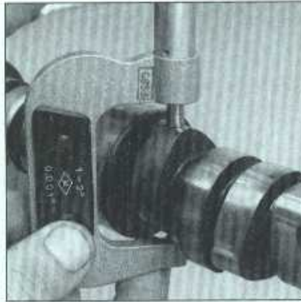
13.18a If the camshaft is removed from the engine, lobe lift can be obtained by measuring camshaft lobe height . . .
