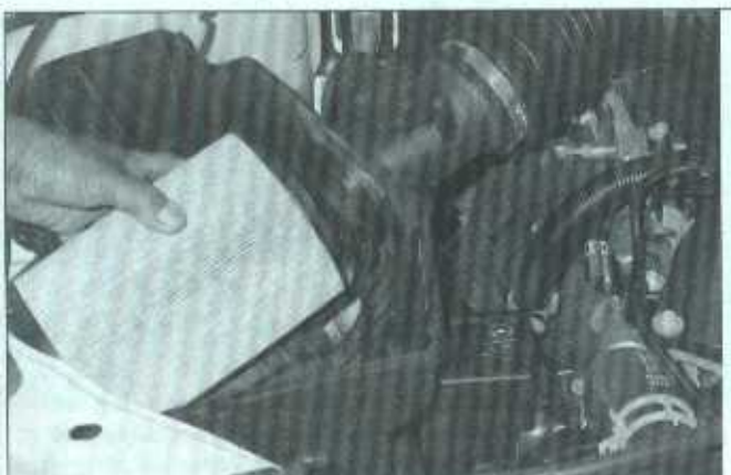
24.3b With the cover removed, pull the filter element from its retainers in the lower housing
