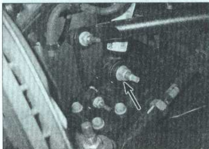
2.5 Remove the lower shock bolt at the lower control arm
