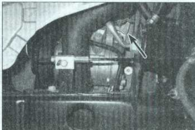
3.7 The thermostat housing is located on the left side of the engine, above the air conditioning compressor (one of the two bolts is visible here)
