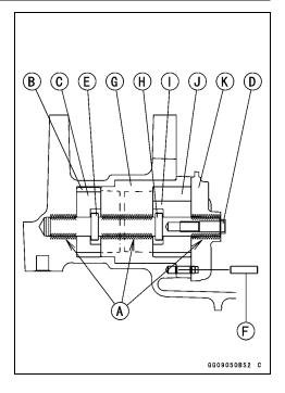
Apply a non-permanent locking agent to the oil pump cover bolts and tighten them.
