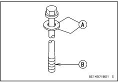
Apply molybdenum disulfide oil solution to flange [A] and the threads [B] of the M8 bolts which is tightening order is [7 ~ 10] only (see the next figure).
