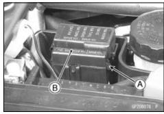
• Pull out the ECU fuse [A] from the fuse box.
