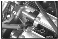
OEach piston has two inlet and two exhaust valves. Measure these two inlet or exhaust valves at the same crankshaft position.
