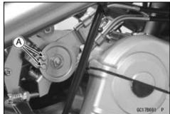
After removing the throttle body assy, stuff pieces of lint -free, clean cloth into the throttle body holders.
