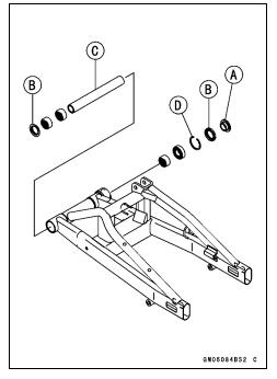
• Remove the ball bearing and needle bearings.
