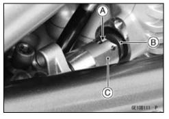
Tighten the tensioner mounting bolts [A].
