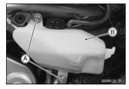
Put [A] the projection [B] on the reserve tank into the hole
