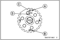
OMeasure the valve clearance of the valves for which the cam [A] are turned away from each other.
