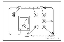
OWhen checking a harness [A] for short circuit, open one end [B] and check the continuity between the other end [C] and ground [D]. If there is continuity, the harness has a short circuit to ground, and it must be repaired or replaced.
