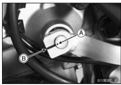
Be sure the shift pedal position is as shown. Shift Pedal Damper [A]
