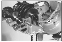
• Be sure that the dowel pins [A] are in position.
