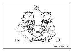
• Using the thickness gauge [A], measure the valve clearance between cam and valve lifter.
