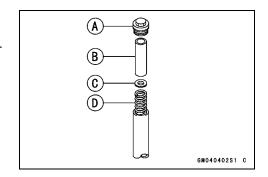
Remove the Allen bolt [A] from the bottom of the fork.
