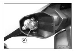
• Insert the new bulb [A] by aligning its upper and lower pins [B] with the upper and lower grooves [C] in the socket, and turn the bulb clockwise.
