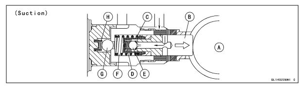
When the pump discharges the brake fluid, the inlet valve [E] is closed by the spring [D], and the piston [B] is moved left by the cam [A], producing pressure in the cylinder [F]. The pressure pushes the spring [H], opens the outlet valve [G], and the brake fluid returns to the master cylinder.
