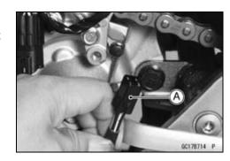
Set the hand tester [A] to the × 1 Ω range and connect it to the terminals in the oxygen sensor lead connector [B].
