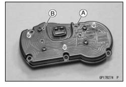
Separate the meter assembly [A] and upper meter cover [B].
