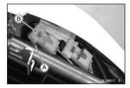
Pull out the relay fuse [A] from the fuse box with needle nose pliers.
