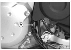
• Remove the oxygen sensor [A].
