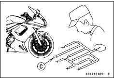
Even when the DFI system is operating normally, the FI indicator light (LED) [A] may light up under strong electrical interference. No repair needed. Turn the ignition switch OFF to stop the indicator light.
