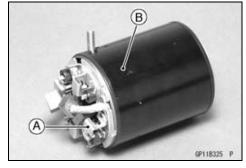
• Remove the brush plate [A] from the plate cover [B].
