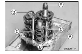
Remove: Shift Drum Cam Bolt [A] Shift Drum [B] and Pin Shift Drum [C]
