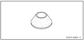
Valve Seat Cutter Holder Bar: 57001-1128
