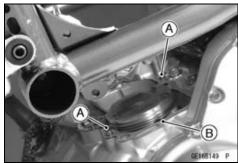
The piston ring openings must be positioned as shown in the figure. The openings of the oil ring steel rails must be about 30 ~ 40° of angle from the opening of the top ring.
