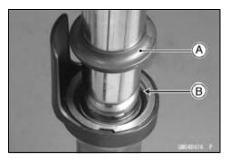
• Separate the inner tube [A] from the outer tube [B].
