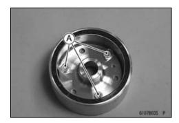
Remove: Starter Motor Clutch [A]
