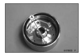
Remove: Starter Motor Clutch [A]
