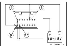
If each lights (LED) does not go on, replace the meter assembly.
