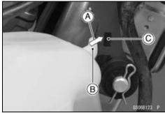
• Place a container under the water pump drain bolt [A], then remove the drain bolt.
