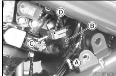
Push and pull [A] the fuel hose joint [B] back and forth more than two times and make sure it is locked and doesn't come off.
