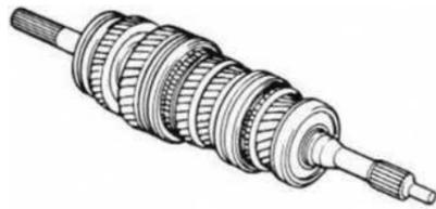
Main shaft and input shaft assembly
