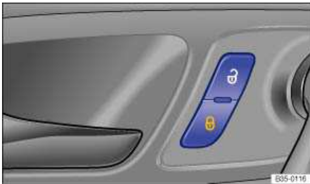
Fig. 21 In the vehicle doors: Power locking button.
