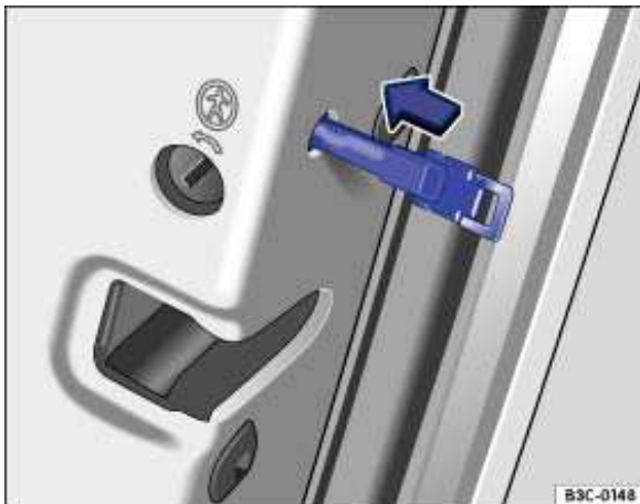
Fig. 163 Locking the vehicle using the emergency key.
