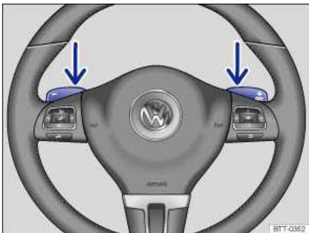
Fig. 120 Steering wheel with optional Tiptronic shift paddles.
