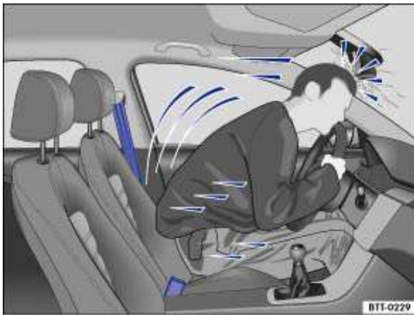
Fig. 49 The unbelted driver is thrown forward.
