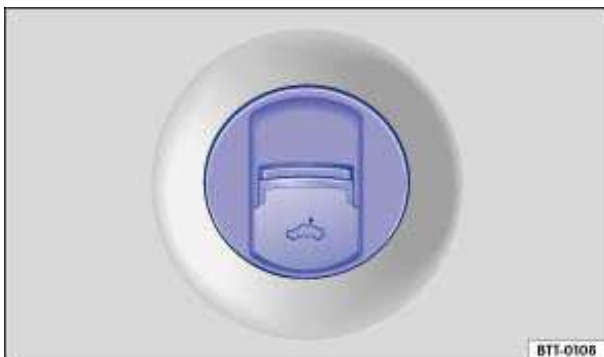
Fig. 28 In the headliner: switch for the Panoramic tilting sunroof.
