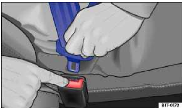
Fig. 53 Releasing the buckle tongue from the belt buckle.
