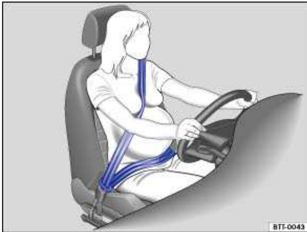
Fig. 55 Proper safety belt positioning for expectant mothers.
