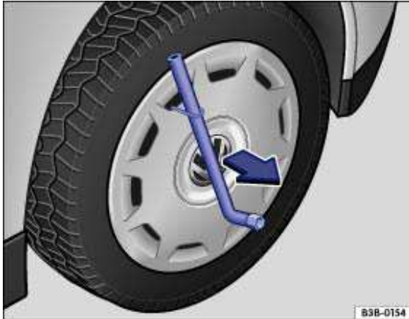
Fig. 173 Pulling the wheel cover off.
