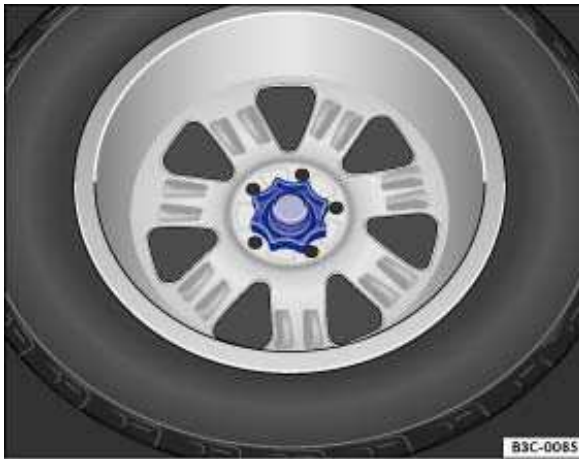
Fig. 155 In the luggage compartment: Handwheel holding spare wheel in place.
