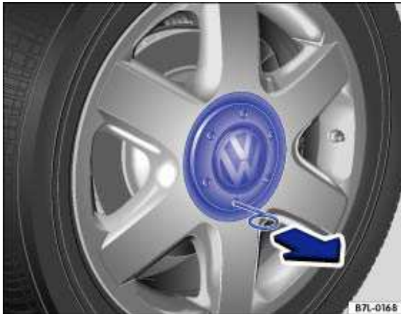
Fig. 171 Pulling the hubcap off.
