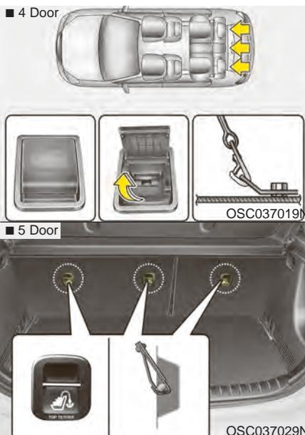
Child restraint hook holders are located on the package tray (4 Door) or the floor behind the rear seat (5 Door).
