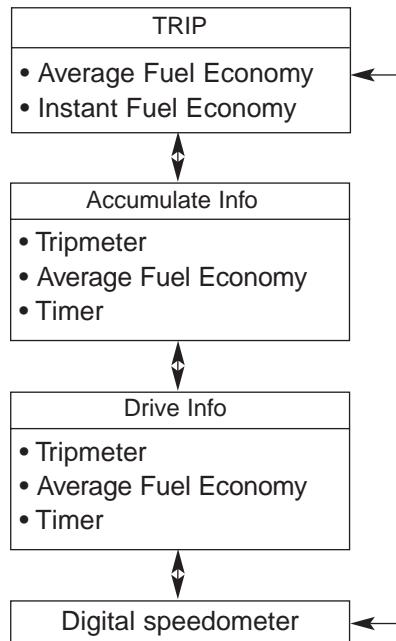
To change the trip mode, scroll the MOVE scroll switch ( $\wedge/\vee$ ) in the trip computer mode.
