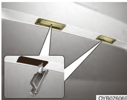
3. Remove the bulb from bulb-socket by pulling it out.
