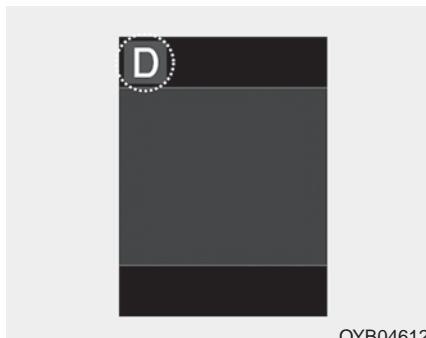
This indicator displays which automatic transaxle shift lever is selected.
