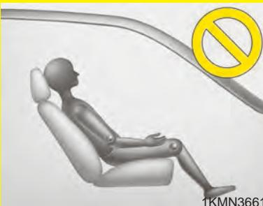
The driver must advise the passenger to keep the seatback in an upright position whenever the vehicle is in motion. If a seat is reclined during an accident, the restraint system's ability to restrain will be greatly reduced.
