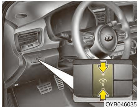
The instrument panel illumination intensity can be adjusted by pressing the control switch with the headlight switch in any position when the ignition switch is in the ON position.
