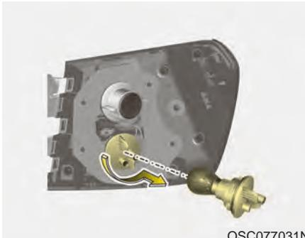
3. Remove the socket from the assembly by turning the socket counterclockwise until the tabs on the socket align with the slots on the assembly.
