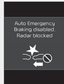
When the sensor is covered or dirty with foreign substances, such as snow or rain, the AEB operation may temporarily stop. In this case, a warning message will appear to notify the driver.
