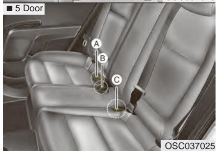
The seat belt should be locked into the buckle on each seat cushion to be properly fastened.
