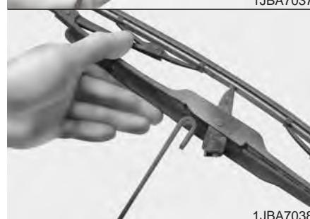
2. Compress the clip (1) and slide the blade assembly downward (2).
