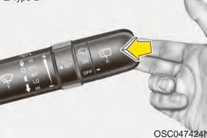
In the OFF position, pull the lever gently toward you to spray washer fluid on the windshield and to run the wipers 1-3 cycles.
