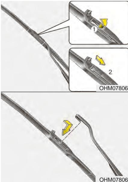
2. Lift up the wiper blade clip. Then pull down the blade assembly and remove it.
