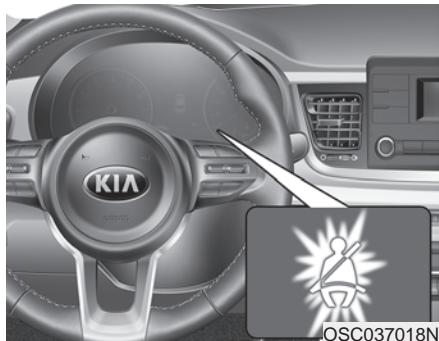
As a reminder to the driver, the driver's seat belt warning lights will illuminate and warning chime will sound for approximately 6 seconds each time you turn the ignition switch ON regardless of belt fastening.
