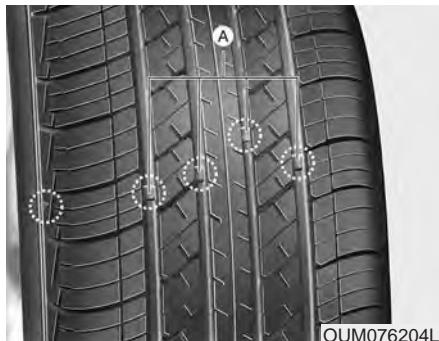
If the tire is worn evenly, a tread wear Indicator (A) will appear as a solid band across the tread. This shows there is less than 1/16 inch (1.6 mm) of tread left on the tire. Replace the tire when this happens.
