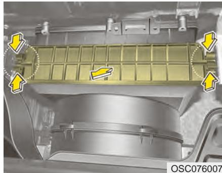
3. Remove the climate control air filter cover while pressing the lock on the both sides of the cover.
