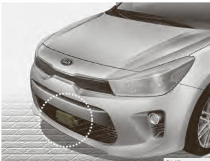
The sensor is to maintain a certain distance from the vehicle in front. However, the smudged sensor with foreign substances, such as snow and rain, adversely affects the sensing performance. It may even temporarily cancel the AEB. Always keep the sensor clean.
