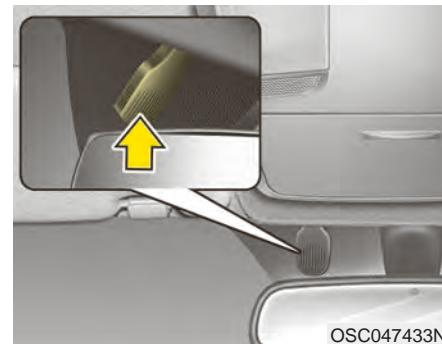
Auto defogging reduces the possibility of fogging up the inside of the windshield by automatically sensing the moisture of inside the windshield and air flow toward the windshield can increase.
