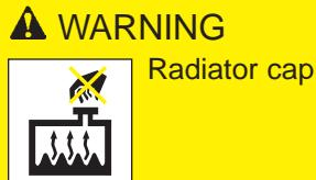
Do not remove the radiator cap when the engine and radiator are hot. Scalding hot coolant and steam may blow out under pressure which may result in serious injury.
