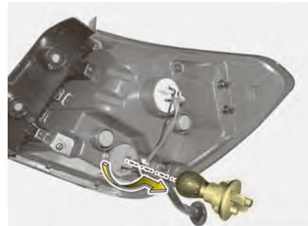
5. Remove the socket from the assembly by turning the socket counterclockwise until the tabs on the socket align with the slots on the assembly.
