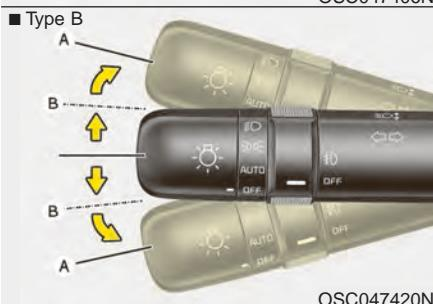
The ignition switch must be on for the turn signals to function. To turn on the turn signals, move the lever up or down (A). The green arrow indicators on the instrument panel indicate which turn signal is operating.
