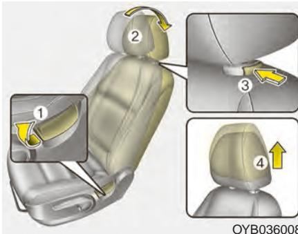
3. Press the headrest release button (3) while pulling the headrest up (4).
