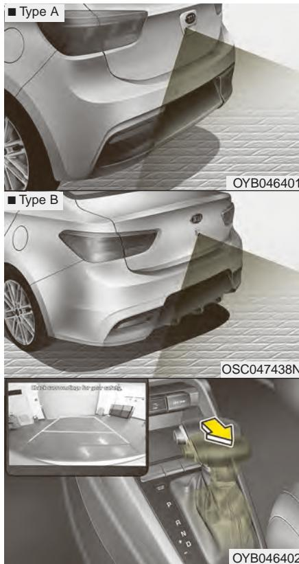
The rear view camera will activate with the ignition switch on and the shift lever in the R (Reverse) position.
