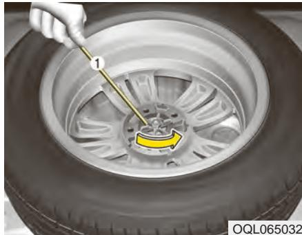
If it is hard to loosen the tire hold-down wing bolt by hand, you can loosen it easily using the jack handle.
