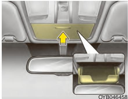
To open the sunglass holder, press the cover and the holder will slowly open. Place your sunglasses with the lenses facing out. To close the sunglass holder, push it up. Do not open the sunglass holder while the vehicle is moving. The rear view mirror of the vehicle can be blocked by an open sunglass holder.
