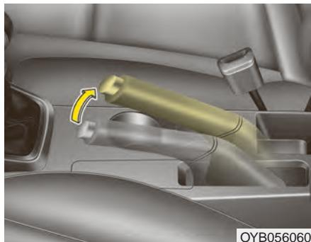
To engage the parking brake, first apply the foot brake and then without pressing the release button in, pull the parking brake lever up as far as possible. In addition it is recommended that when parking the vehicle on a gradient, the shift lever should be positioned in the appropriate low gear for manual transaxle vehicles or in the P (Park) position for automatic transaxle vehicles.
