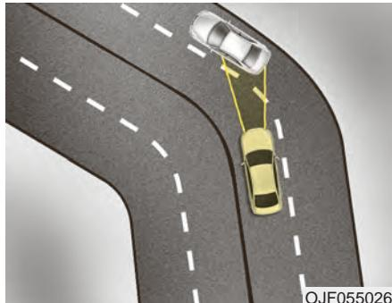
While driving on a curve, the AEB may recognize the vehicle in front in the next lane. Exercise caution, and, if necessary, depress the brake pedal. Or, depress the accelerator pedal to maintain the driving speed. Always, take a look around the vehicle for your safety.
