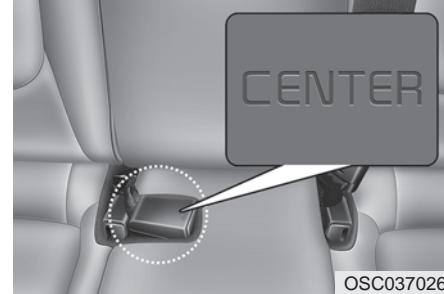
When using the rear center seat belt, the buckle with the "CENTER" mark must be used.
