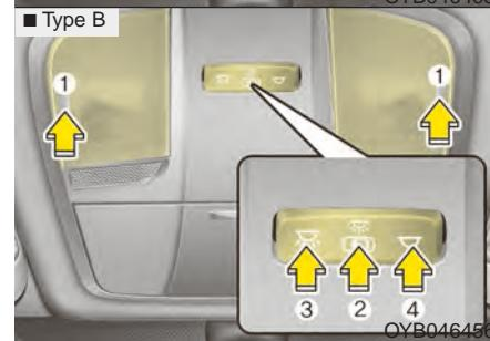
Push the lens (1) to turn the map lamp on or off. This light produces a spot beam for convenient use as a map lamp at night or as a personal lamp for the driver and front passenger.
