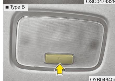
To turn the room lamp ON or OFF, push the switch.
