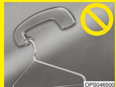
Do not hang other objects such as hangers or hard objects except clothes. Also, do not put heavy, sharp or breakable objects in the clothe pockets. In an accident or when the curtain air bag is inflated, it may cause vehicle damage or personal injury.
