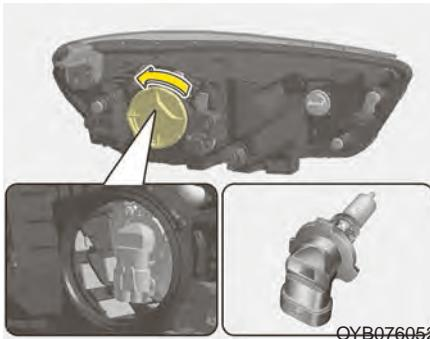
5. Install a new bulb-socket assembly in the headlamp assembly by aligning the tabs on the bulb-socket with the slots in the headlamp assembly. Push the bulb-socket into the headlamp assembly and turn the bulb-socket clockwise.
