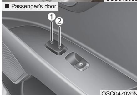
Operate by pressing the central door lock switch.
