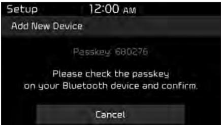
4-2. For devices that require passkey confirmation, the following screen is shown on the audio system. A 6-digit passkey input screen is shown in the *Bluetooth®* Wireless Technology device.
