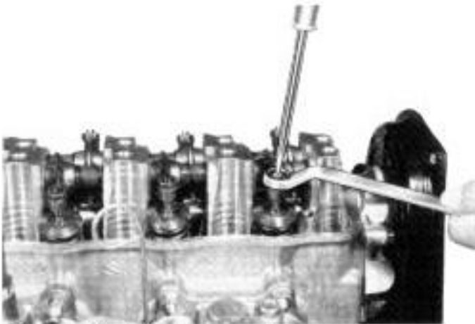
Fig. 3-152 Adjusting valve clearance
