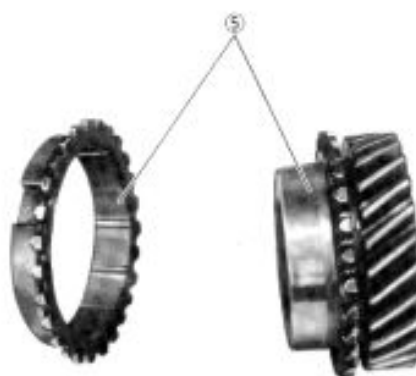
Fig. 13-21 ⑤ Checking contacting surface
