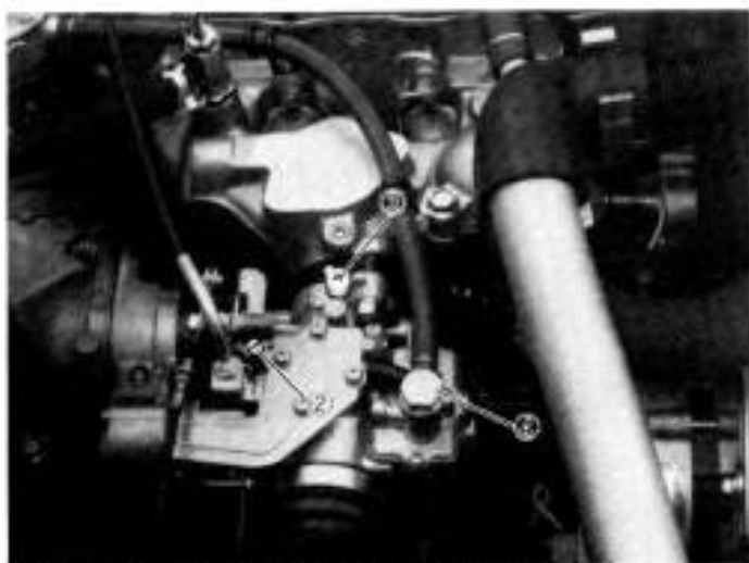
Fig. 4-13 (4) Tightening torque: 1.8 kg-m (13.0 lb-ft)
