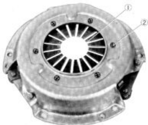
Fig. 11-7 ① Spring wear; ② Rivet
