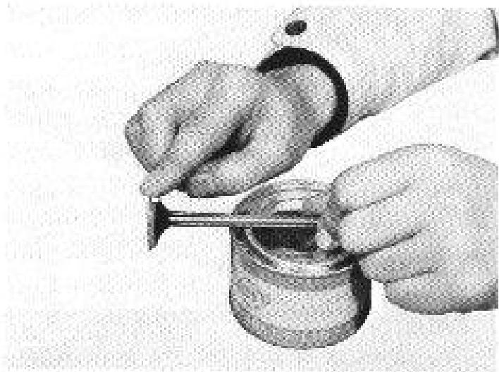
Fig. 3-69 Applying lapping compound to valve face
