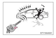
When "OLD is pushed for longer than about one second, an alarm will sound for about 60 seconds and the vehicle lights will flash to deter any person from trying to break into or damage your vehicle.
