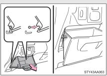
2. Pull up the box and disengage the claws. Remove the stoppers from the cutouts and remove the box.
