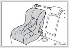
Seat belts equipped with a child restraint locking mechanism (ALR/ELR belts except driver's seat belt) (→P. 41)
