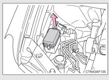
Type B: Push the tab in and lift the lid off. (if equipped)
