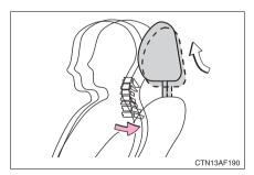
When the occupant's back presses against the seatback during a rear-end collision, the head restraint moves slightly forward to help reduce the risk of whiplash on the seat occupant.
