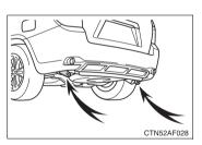
If your vehicle becomes stuck and cannot move, the emergency hooks are used for another vehicle to pull your vehicle out in an emergency.
