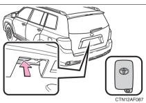
Press the button to unlock the door.
