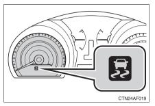
If the vehicle is in danger of slipping, rolling backwards when starting on an incline, or the front wheels (2WD models) or four wheels (4WD models) spin, the indicator flashes to indicate that the Enhanced VSC/TRAC systems have been engaged.
