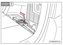
Unhook the tightening strap and remove the pad.
