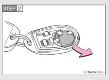
Remove the discharged transmitter battery.
