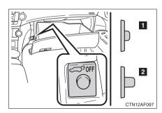
Turn the main switch in the glove box OFF to disable the power back door system.
