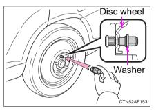
Turn the nut washers until they come into contact with the disc wheel.
