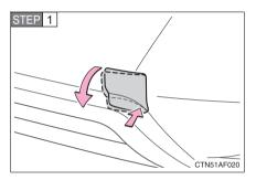
Remove the eyelet cover while pushing it.
