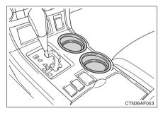
Removing the adapters changes the size.  $(\rightarrow P. 364)$
