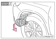
Remove the fender liner.
