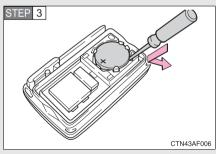
Remove the depleted battery.
