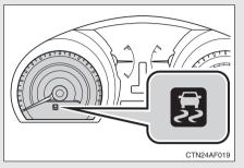
If the vehicle is in danger of rolling slipping, backwards when starting on an incline, or the front wheels (2WD models) or four wheels (4WD models) spin, the indicator flashes to indicate that the hill-start assist control system have been engaged.
