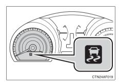
The slip indicator will flash to indicate that the downhill assist control system is operating, and the stop lights and high mounted stoplight will turn on.
