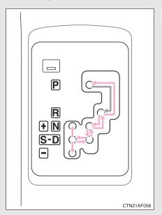
While the "ENGINE START STOP" switch or the engine switch is in ON, depress the brake pedal and move the shift lever.
