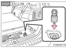
Attach the adapter socket (for removing a spare tire) on the spare tire clamp bolt.
