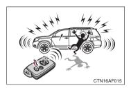
When (() is pushed for longer than about one second, an alarm will sound for about 60 seconds and the vehicle lights will flash to deter any person from trying to break into or damage your vehicle.
