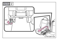
Pull the lock release lever to remove the second center seat.
