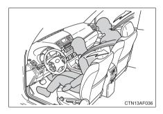
The pretensioner helps the seat belt to quickly restrain the occupant by retracting the seat belt when the vehicle is subjected to certain types of severe frontal collision or a vehicle rollover
