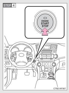
Press the "ENGINE START STOP" switch.
