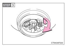
Release the bulb retaining spring.
