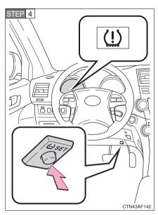
Press and hold the tire pressure warning reset switch for at least 3 seconds
