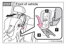
Outside seat: Open the anchor bracket cover. Latch the hook onto the anchor bracket and tighten the top strap.
