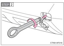
Insert the towing eyelet into the hole and tighten partially by hand.
