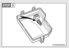
Remove the fuse with the pullout tool.
