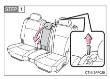
Fold down the second center seatback while pulling the seatback lock release strap.
