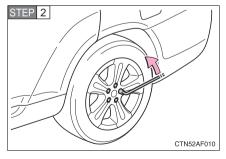
Slightly loosen the wheel nuts (one turn).
