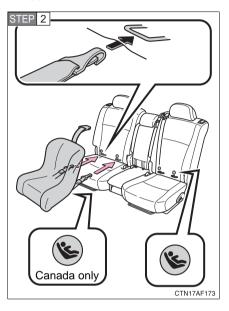
Latch the buckles onto the anchorages.
