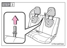
Pull the strap to fold down the head restraints.
