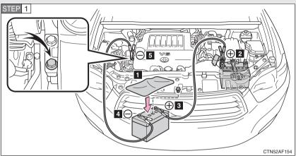
Connecting the jumper cables
