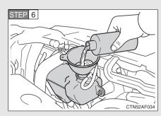
Add engine coolant if necessary.
