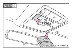
Press and hold down one of the buttons on the HomeLink<sup>®</sup> and the button on the transmitter. When the indicator light on the HomeLink<sup>®</sup> changes from a slow to a rapid flash after 20 seconds, you can release both buttons.
