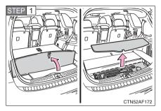
Open the center deck board and remove the cover.
