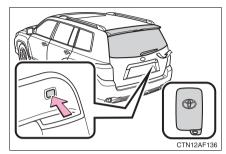
Press and hold the button to unlock the glass hatch. The glass hatch will pop up.
