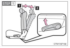
Fold the seatback while pulling the lever. Return the seatback and secure it at the 1st lock position (most upright position). Adjust the seatback to the 3rd lock position.  $(\rightarrow P. 78)$
