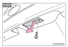
Remove the screw and remove the unit.
