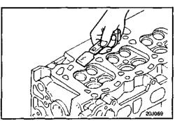
28000, 09222-28100), remove the retainer lock. Next remove the spring retainer, valve spring, spring seat and valve. **NOTE**
