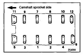
5. Tighten the bearing caps to the specified torque in two or three steps as shown.
