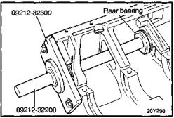
5. Using special tool, install the right counter balance shaft rear bearing to the cylinder block.
