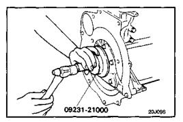
10. Install the oil separator into the oil seal so that the oil hole in the separator is directed downward (arrow in illustration).
