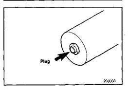
4. Using a vise soft jaws push in the auto tensioner rod. If the rod can be easily retracted, replace the auto tensioner. You should feel a fair amount of resistance when pushing the rod in.
