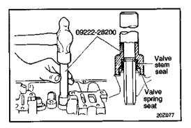
Install springs and spring retainers. Valve springs should be installed with the enamel coated side toward the valve spring retainer.
