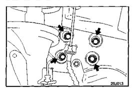
1. While checking the connections of the harnesses, pipes, hoses, etc., and making sure that none of them are being caught, damaged, etc., install the engine and transaxle assembly.
