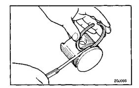
2. To measure the piston ring end gap, insert a piston ring into the cylinder bore. Position the ring at right angles to the cylinder wall by gently pressing it down with a piston. Measure the gap with a feeler gauge. If the gap exceeds the service limit, replace the piston ring.
