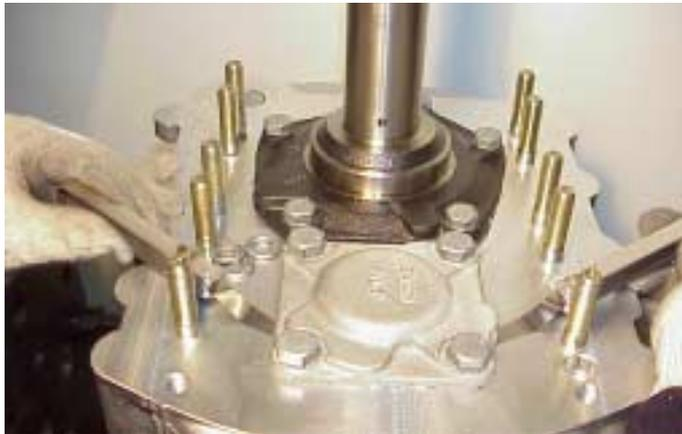
24. Back off the four capscrews to zero torque then retighten just sufficiently to nip the bearing cover plate. Using feeler gauges, measure the clearance between the cover plate and the case at several points. From the range of graded spacers select the thickness which give the required preload to the layshaft bearings of 0,075 to 0,125 mm with new bearings or 0,00 to 0,05 with used bearings.
