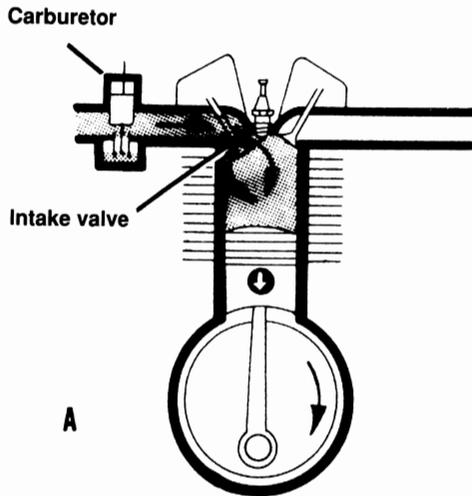
As the piston travels downward, the exhaust valve is closed and the intake valve opens, allowing the new air-fuel mixture from the carburetor to be drawn into the cylinder. When the piston reaches the bottom of its travel (BDC), the intake valve closes and remains closed for the next 1 1/2 revolutions of the crankshaft.
