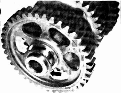
12. Refer to Figure 66 for correct placement of all gears. Make sure the circlip is correctly seated in the shaft groove.
