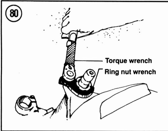
11. Install the upper steering stem and the steering stem nut.
