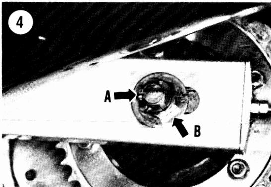
7. Remove the cotter pin (A, **Figure 4**). Loosen then remove the rear axle nut (B, **Figure 4**) and the special washer.
