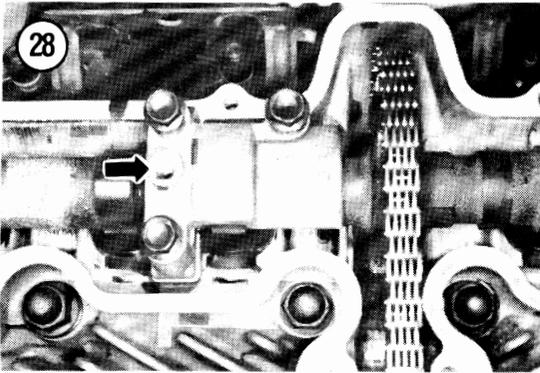
16. Secure the camshaft chain with wire or place a screwdriver or scribe (A, **Figure 32**) through the chain loop to prevent the chain from falling into the crankcase.
