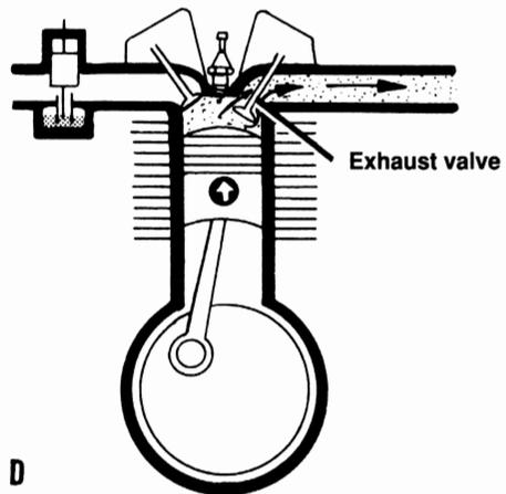
When the piston almost reaches BDC, the exhaust valve opens and remains open until the piston is near TDC. The upward travel of the piston forces the exhaust gases out of the cylinder. After the piston has reached TDC, the exhaust valve closes and the cycle starts all over again.
