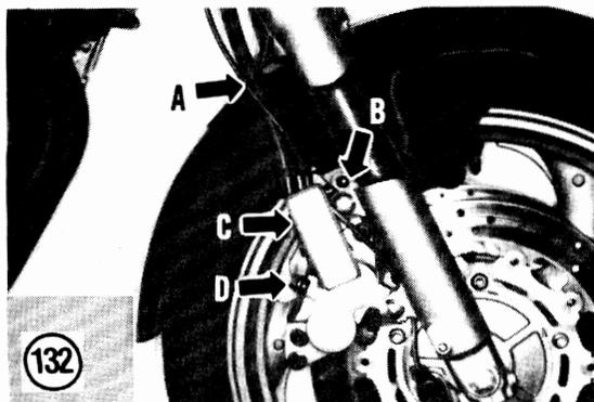
*Yamaha flexible brake hoses are designed to have the same minimal flexing characteristics as the steel lines. When replacing the flexible brake hoses be sure to install authorized Yamaha replacement hoses specifically designed for use with the ABS system. Using a flexible brake hose of an alternate design will drastically change the characteristics of the brake system.*
