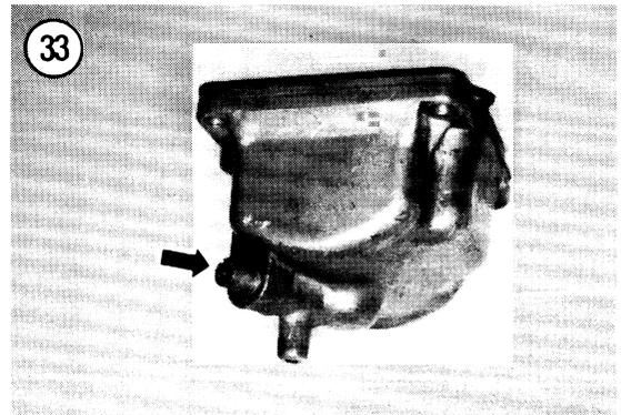
bly will cause the carburetor to flood and overflow fuel.
