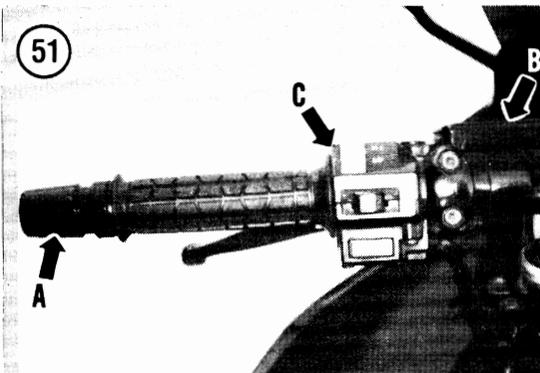
5. Remove the screws and separate the right-hand switch assembly (C, **Figure 50**). Disconnect the front brake light switch. Disconnect the throttle cables from the twist grip. Remove the switch assembly from the handlebar.
