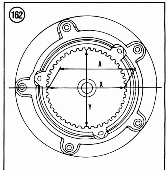
13. At 6 equally spaced intervals, use a Vernier caliper and measure the distance from the hub surface to the top of the sensor rotor Dimension "A" in **Figure 163**.
