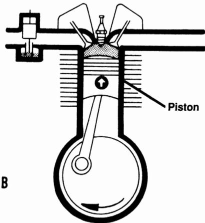
While the crankshaft continues to rotate, the piston moves upward, compressing the air-fuel mixture.
