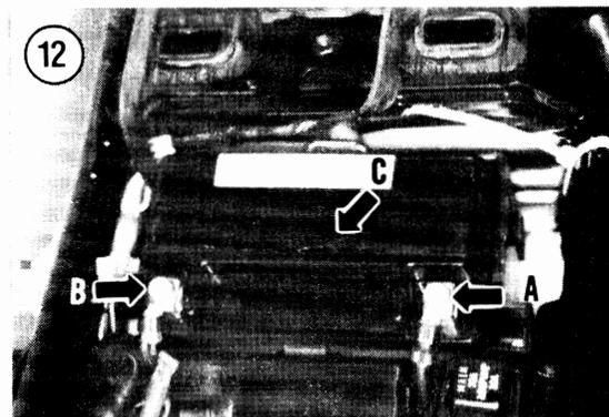
The electrolyte level cannot be corrected on a sealed battery as the battery top is not removable.
