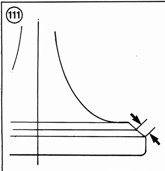
11. Check that the finish has a smooth and velvety surface, it should *not* be shiny or highly polished. The final seating will take place when the engine is first run.
