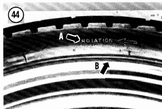
6. Check the bead on both sides of the tire for an even fit around the rim.
