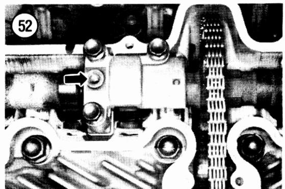
Tighten the bolts to the torque specification listed in **Table 2**.
