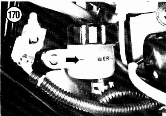
12. If necessary, add fluid to correct the level in the master cylinder reservoir. It must be above the "LOWER" level line. Refer to **Figure 169** for the front master cylinder or **Figure 170** for the rear master cylinder.
