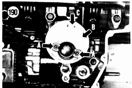
16. Inspect the strainer screen (A, **Figure 193**) for aluminum build-up or damage. If necessary, replace the strainer screen.
