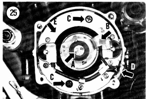
7. Disconnect the electrical connector from the ignitor unit or main harness and remove the pickup coil assembly from the frame.
