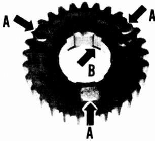
8. Inspect the countershaft drive sprocket splines (**Figure 74**) for wear or discoloration.
