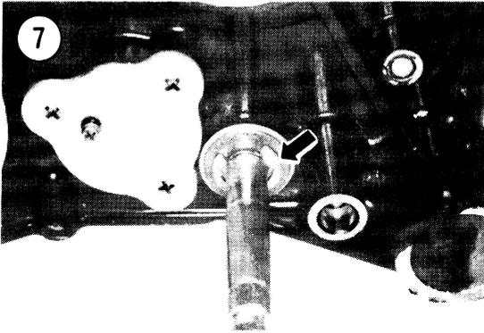
a loose return spring pin; a bent or weak return spring; or worn stopper lever spring or roller.
