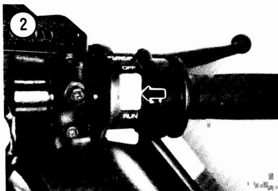
before getting out your tools. Go down the following list step by step. Do each one; you may be embarrassed to find the engine stop switch off, but that is better than wearing down the battery.
