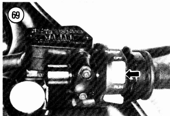
the starter button. Turn the main switch OFF after performing each test.
