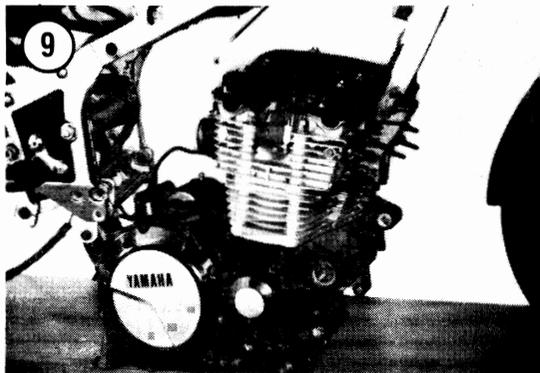
13B. On 1991-on models, remove the following engine mounting components in this order:
