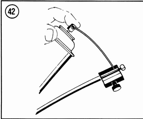
5. Insert the nozzle of the lubricant can into the lubricator, press the button on the can and hold it down until the lubricant begins to flow out of the other end of the cable. Repeat for the other throttle cable.
