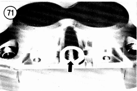
and brake fluid temperatures. Replace the piston and dust seals if the following conditions exist:
