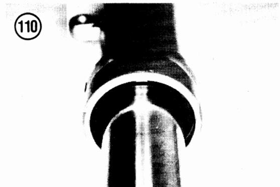
12. Slide the dust seal (B, **Figure 111**) down the fork tube and seat it in the lower fork tube.
