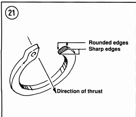
thrust situation (transmission shafts, fork tubes, etc.), the sharp edge must face away from the part producing the thrust. When installing circlips, observe the following:
