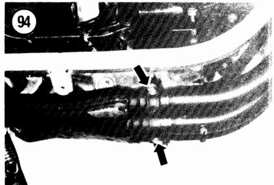
10. Carefully move the front portion of the exhaust system forward to clear the threaded studs on the cylinder head exhaust ports and remove the front portion of the exhaust system.
