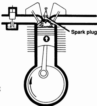
As the piston almost reaches the top of its travel, the spark plug fires, igniting the compressed air-fuel mixture. The piston continues to top dead center (TDC) and is pushed downward by the expanding gases.
