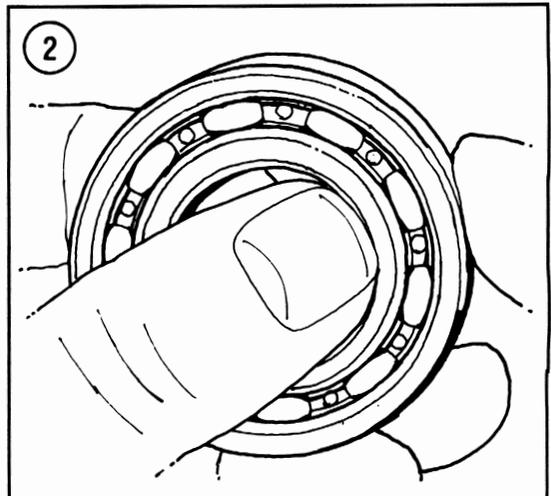
damage. To prevent bearing damage when using compressed air, hold the inner bearing race by hand (**Figure 2**).
