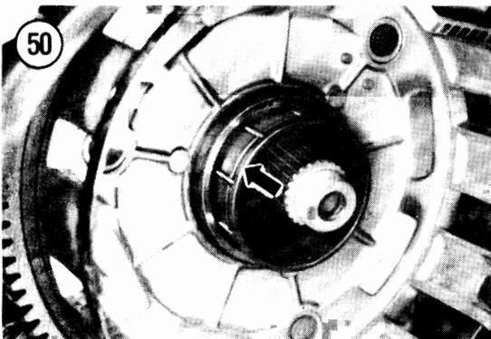
the drive gear is meshed properly with the oil pump drive gear. This is necessary for proper oil pump operation.
