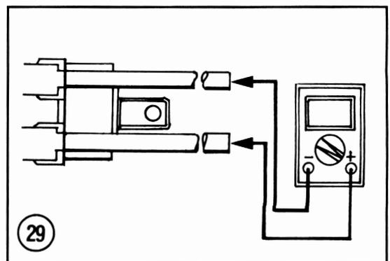
9. Measure the secondary resistance using an ohmmeter set at  $R \times 1,000$ . Measure between the coil's secondary spark plug leads (**Figure 29**). The correct secondary resistance is listed in **Table 1**.
