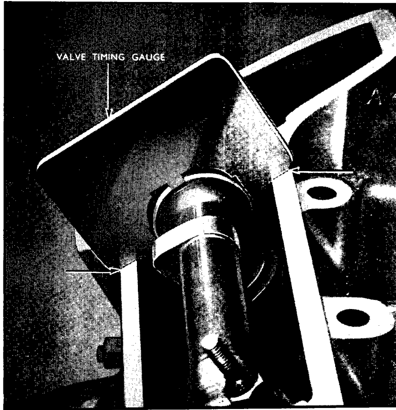
PLATE B.20. VALVE TIMING GAUGE IN POSITION (Ensure that gauge is seated at points indicated by arrows).
