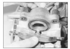
4.24 Removing the inboard pad from the caliper piston - models with ventilated discs
