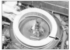
27.4 Removing the air cleaner element note clip for crankcase ventilation hose (arrowed)
