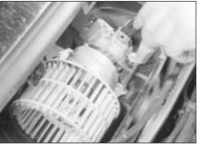
18.6 Unscrewing a heater blower motor clamp screw
