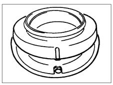
4.24 Mark on suspension strut damper ring aligned with hole in spring seat
