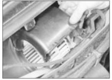
18.4 Unclip the cover from the heater blower motor
