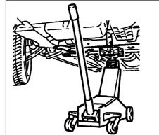
When raising the front of the vehicle, locate the jack underneath the centre of the subframe. Note the use of the block of wood placed on the jack head
