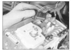
18.5 Disconnecting an instrument panel wiring plug. Note speedometer cable retaining clip (arrowed)
