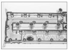
4.13 Camshaft cover removed to show one-piece rubber gasket
