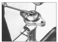
16.5 Holding the primary piston depressed while extracting the circlip from the cylinder body - GMF type master cylinder
