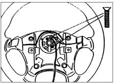
58.3 Airbag contact unit retaining screws
