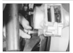
9.5A Withdrawing a rear caliper mounting bolt . . .
