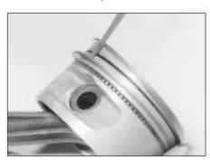
33.5A Using a feeler blade to aid removal of a piston ring - 2.0 litre SOHC engine
