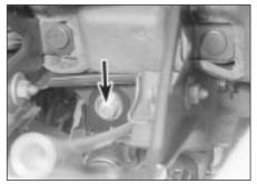
33.13 Steering column to dashboard mounting bracket bolt (arrowed)
