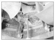
34.18 Removing a front foglamp cover securing screw
