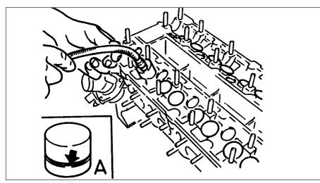
10.5 Remove the hydraulic valve lifters using a rubber plunger. Inset (A) shows valve lifter upright, with oil groove (arrowed) at bottom
