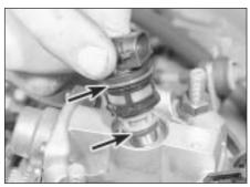
29.6 Renew injector sealing rings (arrowed)
