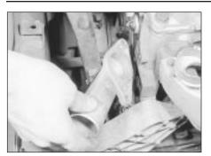
9.6 Remove the thermostat housing . . .
