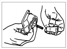
4.21 Belt tensioner pulley and spacer sleeve. Note that smaller diameter of spacer sleeve fits against pulley
