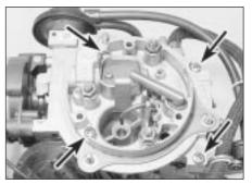
15.8 Carburettor top cover securing screws (arrowed)
