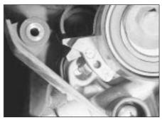
12.12 Timing belt tension is correct when the tensioner indicator pointer aligns with the centre of the baseplate notch
