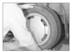
5.4 Check for wear in the hub bearings by grasping the wheel and trying to rock it
