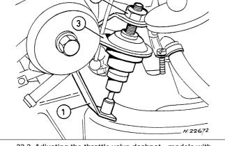
22.2 Adjusting the throttle valve dashpot - models with automatic transmission 2 Locknut
