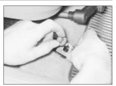
40.3 Removing a front seat rail securing bolt, washer and backplate
