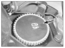
23.6A Prise out the plastic cover (arrowed) . . .
