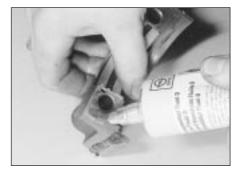
34.25B . . . and the lower surfaces with sealing compound -2.0 litre SOHC engine
