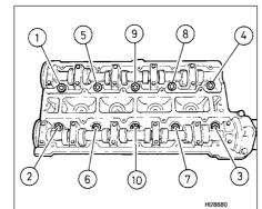
8.27A Cylinder head bolt loosening sequence - (20 XEJ and C 20 XE engines)
