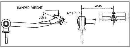
8.10B Correct position of front anti-roll bar damper weight (All dimensions in mm)
