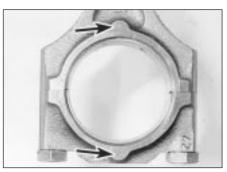
32.14C Lugs (arrowed) on connecting rod and big-end cap must point towards flywheel end of engine - 1.6 litre engine
