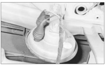
22.5 Horn viewed from behind with radiator removed - single horned model
