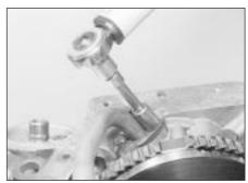
29.15B ... and tighten the securing bolts to the specified torque - 2.0 litre engine
