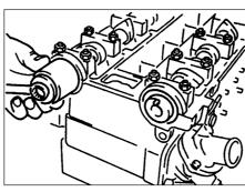
6.5 Using the camshaft sprocket bolt, washer, and a tube to fit a new camshaft front oil seal
