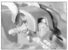
37.10C ... and upper shrouds (steering wheel removed)
