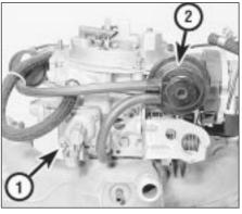
12.1A Side view of carburettor, showing accelerator pump (1) and main choke pulldown diaphragm unit (2)
