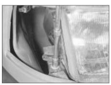
25.5A Unscrewing the lower headlamp securing screw
