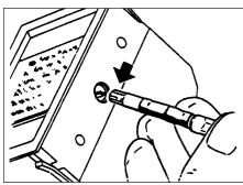
20.6 Removing the trip computer display module illumination bulb
