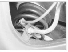
26.5 Brake fluid line/ABS sensor wire bracket and locking clip on semi-trailing arm - DOHC model
