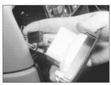
16.3 Disconnecting the wiring plugs from the clock
