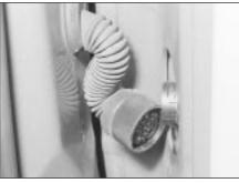
16.3 Disconnect the wiring connector from the front edge of the door
