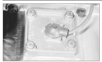
21.18 Engine oil level sensor - DOHC model
