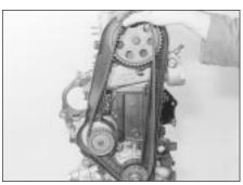
11.23 Refitting the timing belt -2.0 litre engine
