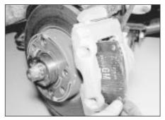
4.8 Withdrawing the outboard disc pad models with solid discs
