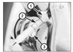
**43.2 Tie-rod end viewed from underneath** 1 Tie-rod end clamp bolt 2 Threaded adjuster pin
