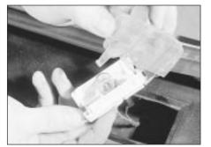
34.27 Unclip the lens from the rear number plate lamp . . .
