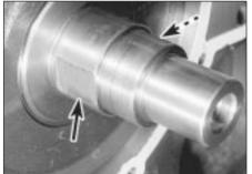
30.9B . . . and with two flats (arrowed) on 1.8 and 2.0 litre engines
