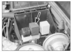
23.9 ABS surge arrester relay (arrowed)
