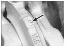
34.8 Main bearing cap identification mark (arrowed) - 1.6 litre engine
