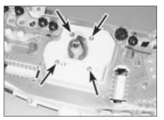
19.14 Speedometer securing screws (arrowed)
