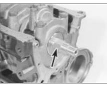
30.9A Oil pump inner gear must engage with hexagon flats on crankshaft (arrowed) on 1.4 and 1.6 litre engines . . .
