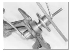
2.12 Drawing the hub into the bearing using improvised tools
