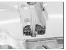
4.12 Unscrewing a camshaft cover securing bolt
