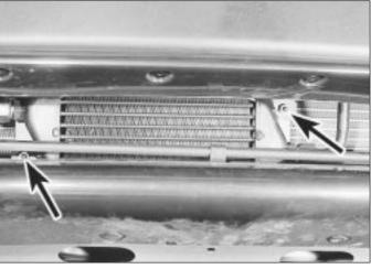
15.1 Oil cooler viewed through front spoiler. Securing nuts arrowed
