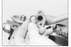
29.15A Fit a new O-ring to the oil pick-up pipe . . .
