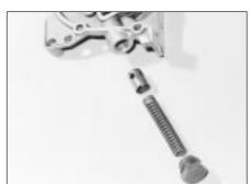
31.7 Oil pressure relief valve components - 2.0 litre SOHC engine
