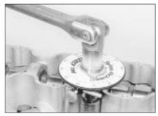
20.37C ... then through the specified angle - 2.0 litre engine
