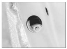
19.10B ... to expose the servo securing bolts
