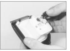
24.16 Removing the clock illumination lamp bulbholder
