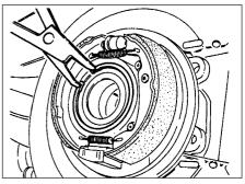
23.11 Extracting the rear hub bearing retaining circlip - DOHC models
