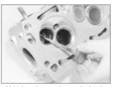
22.11 Inserting an exhaust valve into its guide
