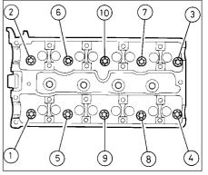
8.27B Cylinder head bolt loosening sequence - (X 20 XEV engines)
