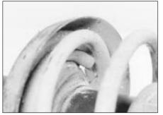
4.22 Lower end of spring rests against lug (arrowed) on lower spring seat
