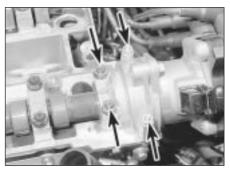
7.4 Exhaust camshaft rear bearing cap securing nuts (arrowed)
