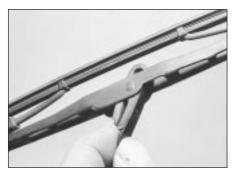
35.3 Removing a wiper blade
