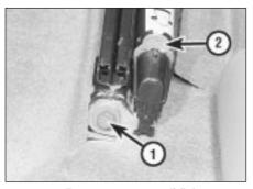
**43.5 Front outer seat rail fixings** *1 Securing bolt*
