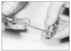
24.9B Locate the cap flange in the plunger groove
