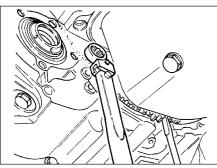
7.35 Commercially-available torque wrench adapter being used to tighten torque converter bolts
