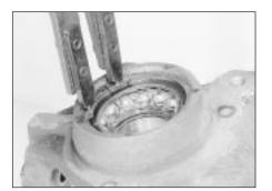
2.6 Extracting the outer bearing retaining circlip
