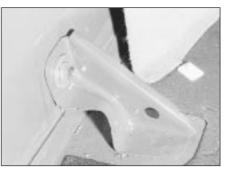
28.8B ... to expose the bumper securing nuts
