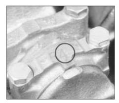
32.3 Big-end cap centre punch identification marks (circled). Note that lug on bearing cap faces flywheel end of engine - 2.0 litre SOHC engine
