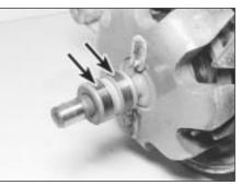
11.4 Alternator slip rings (arrowed) -Delco-Remy alternator
