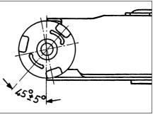
19.11 Trailing arm bush positioning -SOHC models
