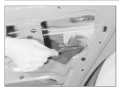
21.12 Unclip the plastic shield from the lock
