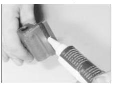
34.25A Fill the side grooves of the rear main bearing cap with RTV jointing compound . . .
