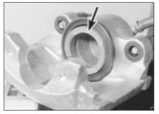
4.25 Caliper piston cutaway recess (arrowed) correctly positioned - models with ventilated discs
