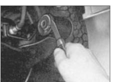
19.8 Cutting inner flange from trailing arm bush - SOHC models
