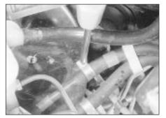
7.14B Fuel hose-to-pipe connections at right-hand side of engine compartment -2.0 litre SOHC model
