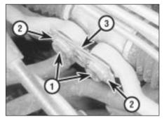
44.05 Tie-rod to steering gear fixings 1 Fixing bolts 3 Spacer plate
