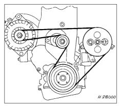
8.23 Correct routing of the ribbed V-belt
