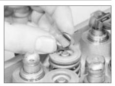
20.25B ... and their thrust pads from the cylinder head - 1.6 litre engine
