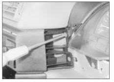
37.16 Unscrewing the left-hand instrument panel upper trim panel securing screw
