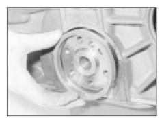
28.4 Fitting a new crankshaft rear oil seal -2.0 litre engine
