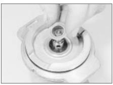
20.13 Removing the thrustwashers
