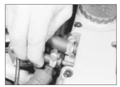
4.10 Disconnecting a breather hose from the rear of the camshaft cover
