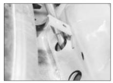
19.11A Unscrew the securing bolts ....
