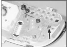
19.5 Instrument panel voltage stabiliser (arrowed)
