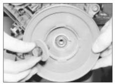
11.24A Refitting the crankshaft pulley -1.6 litre engine
