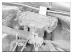
24.1 MSTS-i manifold pressure sensor -1.6 litre model
