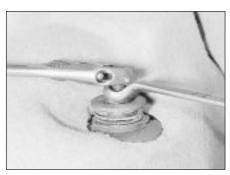
14.4 Unscrewing a rear shock absorber top mounting nut - Hatchback model
