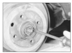
10.5 Loosen rear hub nut until spacer washer can be moved with a screwdriver model with rear disc brakes
