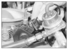
23.8 Disconnecting the throttle position sensor wiring plug - DOHC model
