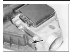
25.2 Airflow meter securing bolt (arrowed) - SOHC model
