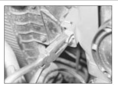
6.6 Compressing a radiator securing clip -2.0 litre SOHC model
