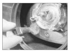
34.6 Pull the sidelamp bulbholder from the headlamp . . .
