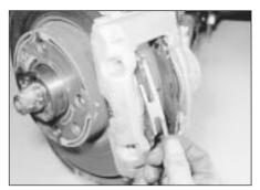
4.7 Removing an anti-rattle spring models with solid discs
