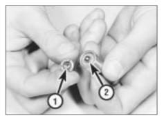
24.9A Spring (1) located in plunger cap, and ball (2) located on seat in plunger
