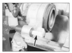
8.20A Extract the nylon compression sleeve (arrowed) . . .
