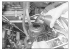
17.2 Topping-up the power steering fluid level
