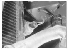
15.1 Cooling fan switch location -2.0 litre SOHC model viewed from below
