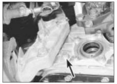
33.2B Transmission oil level plug (arrowed) - F16 type transmission (viewed from below, with driveshaft removed)
