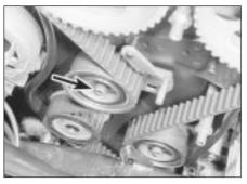
4.8 Timing belt tensioner pulley securing bolt (arrowed)
