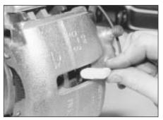
4.21 Withdrawing the pad wear sensor from the inboard pad - DOHC model
