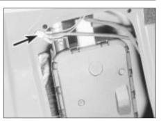
47.3 Radio aerial earth lead securing screw (arrowed) - electric aerial
