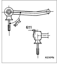
9.7 Correct position of end link on front anti-roll bar (Dimensions in mm)
