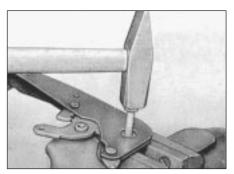
28.11 Driving out the handbrake lever ratchet segment securing sleeve
