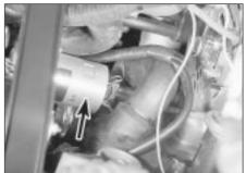
22.9 Idle speed adjuster (arrowed) viewed from underneath vehicle -DOHC model
