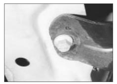
3.10A Front subframe front securing bolt
