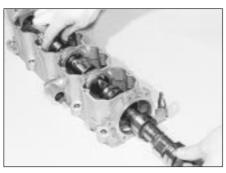
18.6 Withdrawing the camshaft from the housing - 2.0 litre engine
