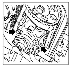
40.6 Power steering pump mounting bolts (arrowed) -1.6 litre models, up to 1992
