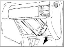
59.6 Removing the passenger side airbag
