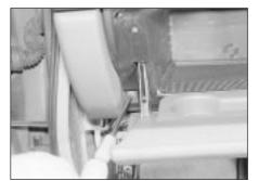
37.35B ... and lower glovebox securing screws ...
