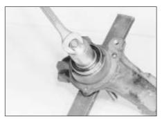
2.9 Fitting a new front wheel bearing using a socket, nut, bolt, washers, and length of bar
