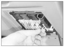
3.5 Removing a fuse - 2.0 litre model shown
