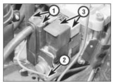
20.4 ABS hydraulic modulator (cover removed)
