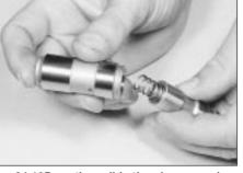
24.10B ... then slide the plunger and spring assembly into the cylinder
