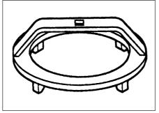
17.4 Vauxhall special tool KM-673 for removing fuel level sender units
