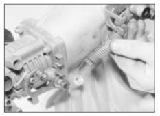
31.8 Unhook the throttle return spring from the bracket on the inlet manifold (inlet manifold removed for clarity)
