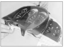
19.8 Removing the instrument panel shroud
