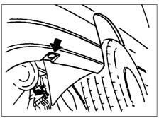
20.12 Trip computer outside air temperature sensor location (arrowed)
