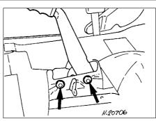
28.9 Handbrake lever securing bolts (arrowed)
