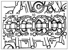
20.23 Cylinder head bolt loosening sequence - SOHC engines
