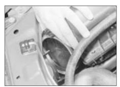
34.2 Removing the cover from the rear of the headlamp
