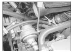
6.3 Disconnecting a fuel hose from the fuel pump - 1.6 litre model
