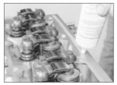
20.35 Apply sealing compound to the cylinder head top mating face
