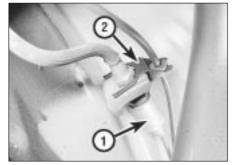
24.10 Brake pressure-proportioning valve on rear underbody - DOHC model 1 Valve 2 Retaining clip
