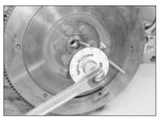
25.13C ... and then through the specified angle - 1.6 litre engine
