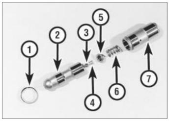
24.1 Hydraulic valve lifter components - SOHC engines
