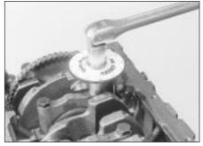
34.27B ... then through the specified angle - 2.0 litre SOHC engine
