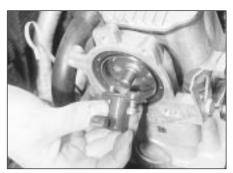
17.10B ...and withdraw the rotor arm -2.0 litre model
