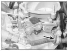
31.23 Remove the fuel hose bracket (arrowed) from the throttle body -DOHC models
