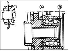
2.8 Cross sectional view of front wheel bearing/hub assembly A Outer bearing retaining circlip B Inner bearing retaining circlip
