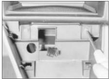
38.12 Extract the two centre console-tofacia securing screws
