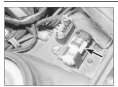
22.3 Octane coding plug (arrowed) -2.0 litre model
