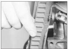
11.42 Checking timing belt tension by twisting belt through 90° between thumb and forefinger
