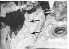
8.14B Rear engine/transmission mountingto-transmission bolts (arrowed)
