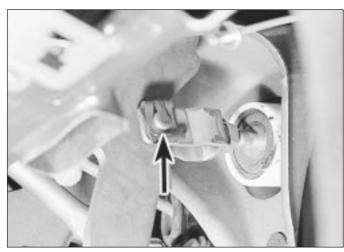
29.4 Brake servo fork-to-pedal pivot pin spring clip (arrowed)
