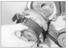
11.5A Withdraw the coolant pump . . .
