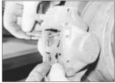
5.5 Removing a rear disc pad retaining pin anti-rattle spring
