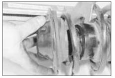
4.14 Lift off the upper spring seat and damper ring
