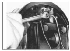
12.6 Unscrewing rear wheel cylinder brake fluid pipe union
