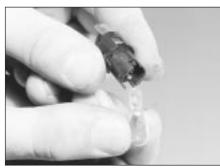
34.07 ... then pull the bulb from the bulbholder
