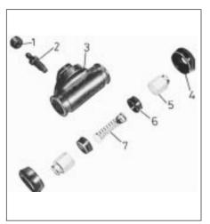
12.13A Exploded view of a rear brake wheel cylinder
