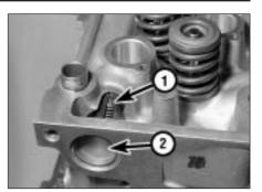
23.10 Oil pressure regulating valve (1) and plug (2) - 2.0 litre engine
