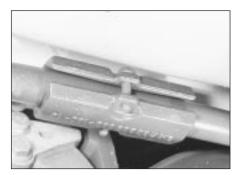
8.10A Front anti-roll bar damper weight
