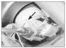
18.7 Heater blower motor resistor retaining clip (arrowed)
