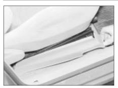
40.1 Withdrawing the outer seat rail trim
