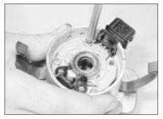
20.16A Remove the securing screws . . .
