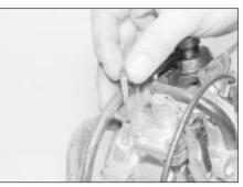
21.6 Refitting the carburettor fuel filter
