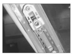
41.15 Upper rear quarter trim panel removed, to expose upper seat belt mounting height adjuster
