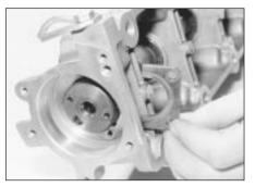
18.5 Removing the camshaft thrustplate - 2.0 litre engine
