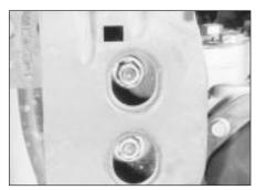
8.14A Rear engine/transmission mounting-to-front subframe nuts
