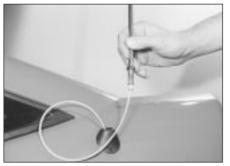
48.7 Push the mast assembly down, until it engages in the clutch mechanism
