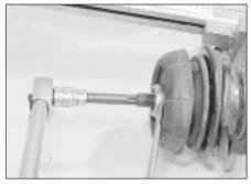
4.27 Tightening the piston rod nut
