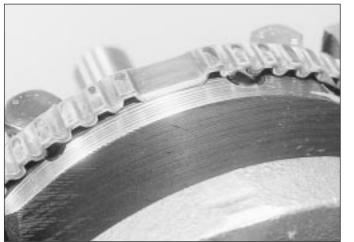
35.9 Check the condition of the TDC sensor wheel teeth at the front of the crankshaft - 2.0 litre SOHC engine
