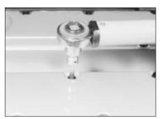
4.24 Tightening a camshaft cover securing bolt
