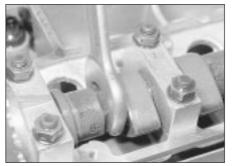
4.14 Spanner positioned to counterhold exhaust camshaft
