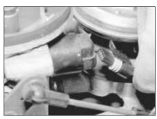
33.3 Disconnecting the idle air control stepper motor wiring plug
