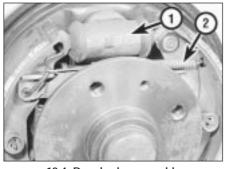
**12.4 Rear brake assembly** 1 Wheel cylinder
