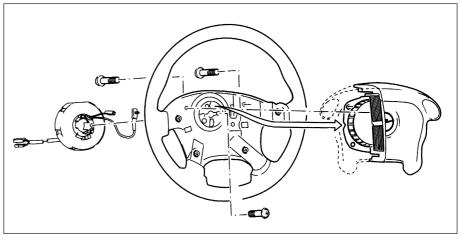
56.3 Airbag, steering wheel and contact unit details
