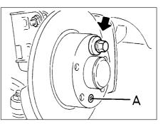
10.2 Refit a wheel bolt and spacer (arrowed) opposite the disc securing screw (A) before checking brake disc run-out
