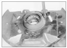
2.5 Removing a brake disc shield securing screw
