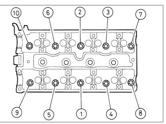
8.36B Cylinder head bolt tightening sequence -X 20 XEV engines
