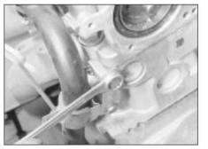
20.19B Unbolting the crankcase breather tube bracket from the cylinder head -2.0 litre model
