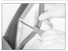
25.12 Unscrewing the window rear guide securing screw
