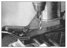
28.13 Drilling out the handbrake lever pawl pivot pin
