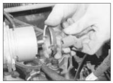
17.5 Removing the rotor arm and plastic shield - 1.6 litre model (Bosch distributor)
