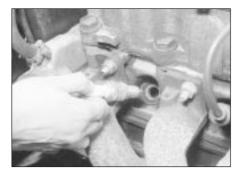
30.3 Removing a spark plug
