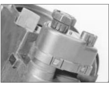
26.2A Headlamp aim adjustment motor (headlamp removed)
