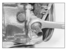
14.4 Unscrewing the oil pressure warning lamp switch -SOHC model (engine removed)
