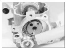
18.13 Tightening a camshaft thrustplate securing bolt - 2.0 litre engine
