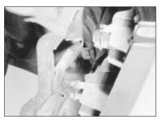
28.5 Front bumper retaining clips released from body
