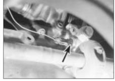
14.2 Oil pressure warning lamp switch (arrowed) viewed from underneath vehicle - SOHC model
