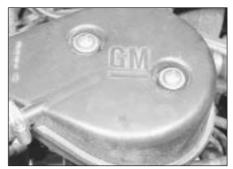
5.4B Do not overtighten the air box screws
