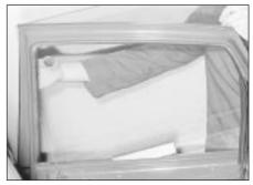
25.15 Withdrawing the window glass from the door
