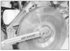
25.13B Tighten the flywheel securing bolts to the specified toque . . .
