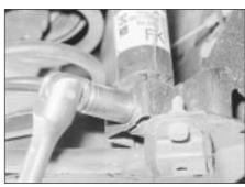
14.7 Unscrewing a rear shock absorber lower mounting bolt - SOHC models
