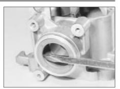
18.10 Prising out the camshaft front oil seal - 2.0 litre engine
