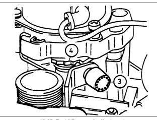
19.27 Fast idle speed adjustment
