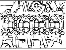
20.37A Cylinder head bolt tightening sequence - SOHC engines
