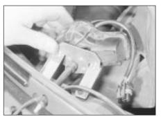
40.5B ... and withdraw the motor
