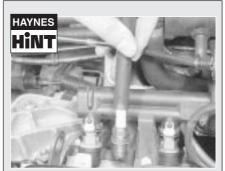
It is very often difficult to insert spark plugs into their holes without crossthreading them. To avoid this, fit a short length of 8 mm (internal diameter), rubber hose over the end of the spark plug. The flexible hose acts as a universal joint to help align the plug correctly. Should the plug begin to cross-thread, the hose will slip on the spark plug, preventing damage to the thread in the cylinder head.
