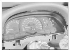
37.17 Withdrawing the instrument panel upper trim panel
