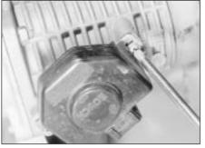
23.3 Removing a throttle position sensor securing screw - SOHC early model
