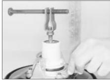
19.15 Measuring the servo operating fork dimension using a bolt inserted through the pivot pin hole
