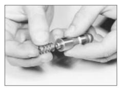
24.10A Locate the spring over the plunger cap . . .
