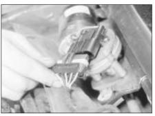
38.4 Disconnecting the windscreen wiper motor wiring plug
