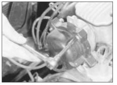
17.8 Unscrewing a distributor cap securing screw - 2.0 litre model
