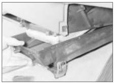
17.4 Removing the plastic cover from the heater matrix
