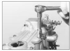
11.22D ... fit the cover and tighten the bolts. Note position of HT lead brackets
