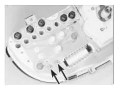
19.12 Tachometer securing nuts (arrowed)
