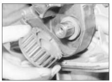
11.20C ... the crankshaft sprocket ...
