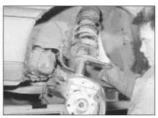
4.8 Withdrawing a suspension strut
