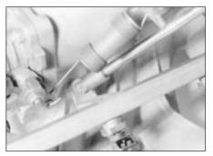
28.6B ... and inner fuel rail securing bolts ...
