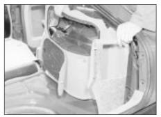
36.19B Withdrawing the lower rear quarter trim panel - Hatchback model
