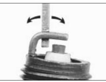
Adjusting spark plug gap
