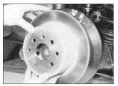
10.18 Withdrawing the rear brake disc - DOHC model
