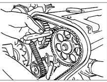
4.44 Working anti-clockwise from the TDC mark on the exhaust camshaft sprocket, mark the seventh tooth on the sprocket
