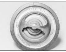
10.2 View of thermostat showing opening temperature markings - 1.6 litre model
