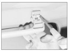
39.2 Removing a grab handle securing screw
