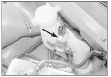
43.1 Headlamp washer fluid non-return valve (arrowed)
