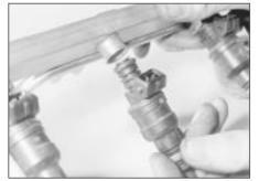
28.7B ... then pull the injector from the fuel rail - SOHC model
