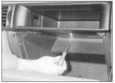
37.33A ... then release the lower retaining clips ...
