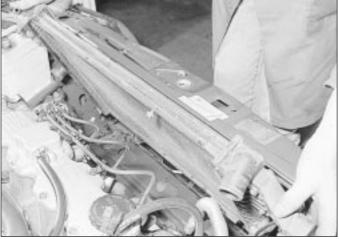
6.7B Withdrawing the radiator - 2.0 litre SOHC model
