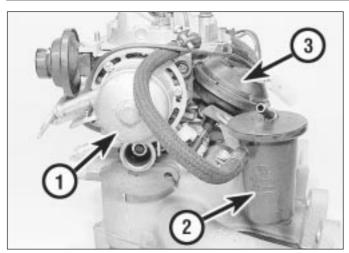
12.1B Side view of carburettor, showing automatic choke housing (1), vapour separator (2) and secondary throttle valve vacuum diaphragm (3)
