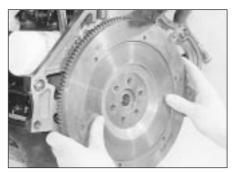
25.5 Removing the flywheel -1.6 litre engine
