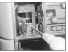
16.4A Remove the two heater control panel securing screws from the clock/trip computer aperture . . .
