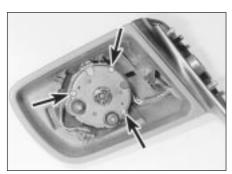
27.10 Mirror motor securing screws (arrowed)
