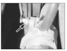
14.1B Temperature gauge sender location (arrowed) - 2.0 litre SOHC model
