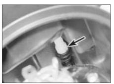
26.2B Headlamp aim adjuster balljoint (arrowed)
