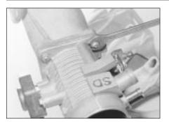
31.10A Unscrew the securing nuts . . .
