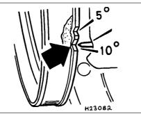
11.7C Crankshaft pulley 10° BTDC notch aligned with pointer on rear timing belt cover - 1.4 litre engine
