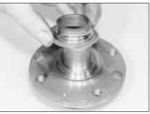
2.4 Removing the half inner bearing race from the hub
