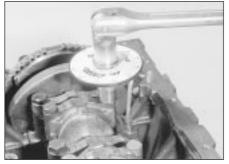
32.18B ... then through the specified angle - 2.0 litre SOHC engine
