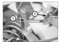
29.7 Rear anti-roll bar fixings -DOHC model 1 End link 2 Clamp bracket
