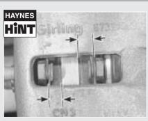
For a quick check, the thickness of the friction material on each brake pad can be measured through the aperture in the caliper body.
