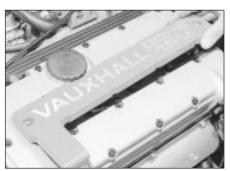
4.11 Removing the spark plug cover
