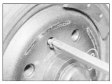
6.6A Extracting a brake drum securing screw
