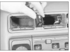
7.11 Withdrawing the hazard warning flasher switch from the facia
