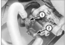
40.11 Power steering pump connections -2.0 litre models
