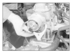
18.7B . . . remove the clamp plate . . .
