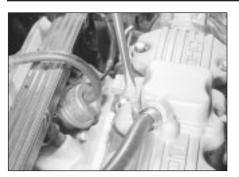
20.7 Disconnecting a camshaft cover breather hose -2.0 litre engine
