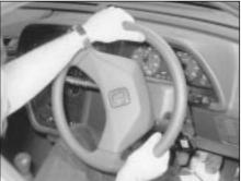
movement of the steering wheel, indicating wear in the column support bearings or couplings.
