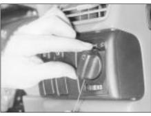
7.2 Using a thin rod to depress the lightning switch knob retaining clip
