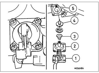
18.11 Carburettor accelerator pump components
