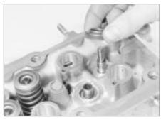
22.12 Fit the valve seat (exhaust valve shown)
