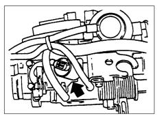
25.1 Carburettor idle cut-off solenoid (arrowed) - 1.8 litre models
