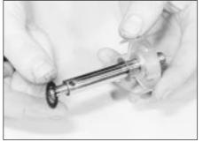
20.14 Recovering the thrustwashers from the shaft - 1.6 litre (Bosch distributor)
