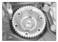
23.6B ... for access to the rear hub nut -DOHC models
