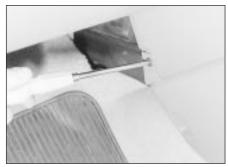
38.13 Unscrewing a side centre consoleto-facia securing screw
