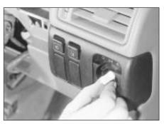
7.3A Press the switch securing clips towards the switch spindle . . .
