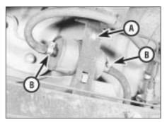
10.6 Fuel filter - 'in tank', fuel pump type
