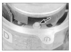
20.16C Sensor plate screw (arrowed) -1.6 litre (Lucas distributor)
