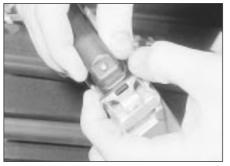
22.4B ... and release the wiring plug retaining clip - ABS-2E system
