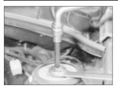
4.7 Unscrewing the suspension strut top mounting nut
