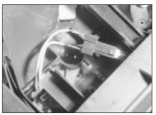
24.20 Heater control panel illumination lamp bulbholder withdrawn
