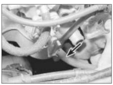
26.5 . . . and the camshaft cover breather hose (arrowed) from the inlet manifold -1.6 litre model
