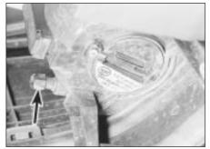
31.7 Foglamp aim adjustment screw (arrowed)
