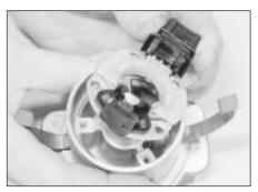
20.16B ...and withdraw the sensor plate -1.6 litre (Bosch distributor)
