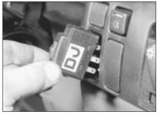
27.4 The headlamp aim adjustment switch - 1992-on models
