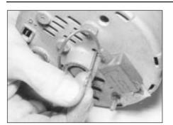
11.15 Withdrawing the twist drill used to retain the brushes -Delco-Remy alternator
