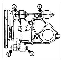
40.15A Mounting and adjuster bolts (arrowed) must be loosened to adjust drivebelt tension - 1.8 and 2.0 litre models, up to 1992
