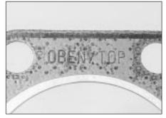
20.31A Cylinder head gasket "Oben/TOP" markings
