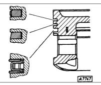
33.5C Sectional view showing correct orientation of piston rings - all engines
