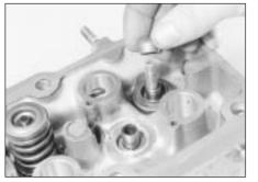
22.14A ... then fit the valve stem oil seal ...
