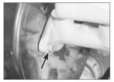
15.7 Master cylinder securing nut (arrowed)
