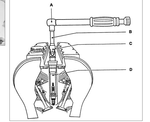
37.3 Removing spark plugs using special adapter (DOHC models)
