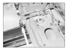
42.2 Power steering fluid cooler pipe unions in engine compartment -2.0 litre SOHC model
