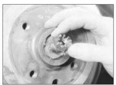
13.17B ... and the hub nut - model with rear disc brakes
