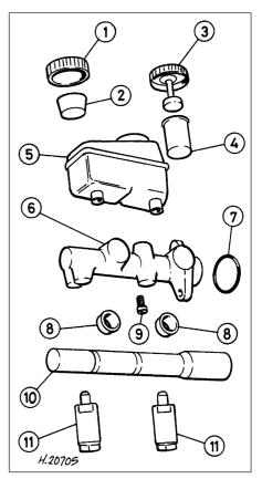
**42** Where applicable, screw the pressureproportioning valves into the base of the cylinder.
