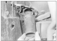
4.12 Removing the resonance box connector tube
