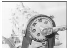
11.22B ... and tighten the securing bolt to the specified torque - 2.0 litre engine
