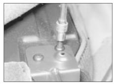
40.21 Extracting a hinge-to-seat back securing screw
