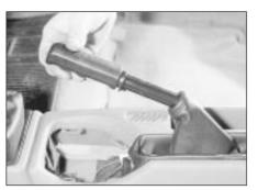
38.3 Pull the grip from the handbrake lever
