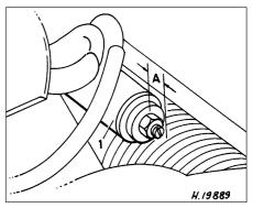
**35.4 Steering damper securing nut setting** 1 Damper tube A = 12.5 top 13.5 mm
