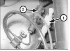
21.3 Front wheel sensor wiring under wheelarch - DOHC model 1 ABS sensor connector
