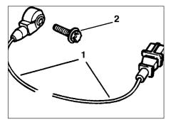
37.8 Knock sensor and wiring (Simtec system)
