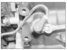
24.17 Unscrewing the crankshaft speed/position sensor securing bolt - 1.8 litre model
