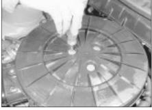
27.3 Air cleaner-to-carburettor mounting cap nuts
