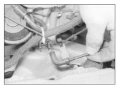
7.12 Disconnect the pressure sensor vacuum pipe from the carburettor -1.6 litre model
