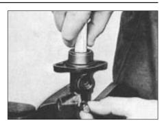
16.25 Depressing the secondary piston while extracting the stop screw - ATE type master cylinder
