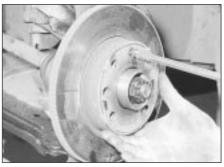
10.12 Removing a disc securing screw -SOHC model
