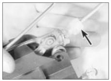
21.7 Exterior handle operating rod adjuster wheel (arrowed) at lock end of rod
