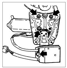
44.10 Front door electric window motor securing nuts and pulse pick-up securing screw (arrowed)
