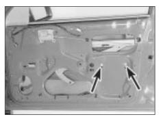
25.5 Window lower guide rail securing screws (arrowed)
