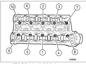
8.36A Cylinder head bolt tightening sequence -20 XEJ and C 20 XE engines
