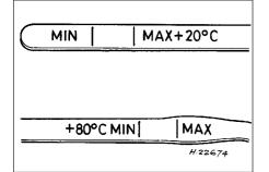
7.4 When checking the fluid level, ensure side of dipstick used corresponds with fluid temperature significant amounts of fluid are being lost (carefully note the amounts being added, and how often), check the transmission for leaks and either repair the fault or take the vehicle to a Vauxhall dealer for attention.
