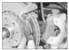
4.23B Withdrawing the caliper, inboard and outboard pad - models with ventilated discs
