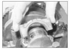
32.17 Fitting a big-end bearing cap -2.0 litre SOHC engine
