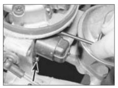
33.4A Unscrew retaining screws (second screw arrowed) . . .
