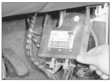
35.3 Withdrawing the fuel injection/ignition system ECU
