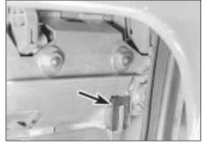
46.10 Central door locking operating microswitch (arrowed) in driver's door
