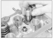
22.14B ... and push onto the spring seat using a socket
