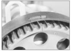
11.7A Camshaft sprocket TDC mark aligned with notch in rear timing belt cover . . .
