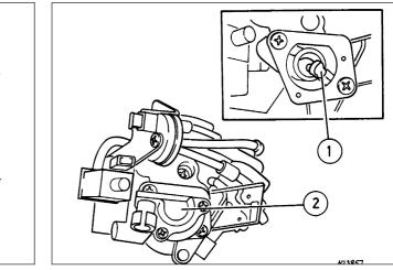
23.4 Throttle position sensor - models with automatic transmission 1 Adapter 2 Sensor
