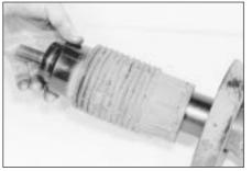
4.15 Slide off the bellows and the rubber buffer
