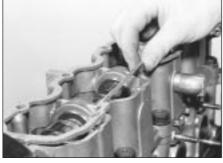
11.22C Fit the camshaft cover gasket . . .
