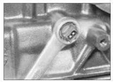
24.11 Unscrewing the MSTS-i oil temperature sensor - 1.6 litre model (engine removed)
