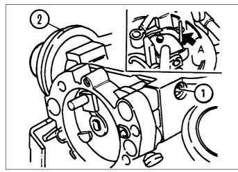
20.12A Choke vacuum pull-down adjustment 1 Adjustment screw 2 Diaphragm unit A Twist drill
