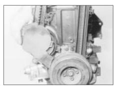
11.5B ...and the smaller cover from the coolant pump - 2.0 litre engine
