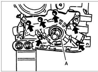
14.3 Oil pump securing bolts (arrowed) and crankshaft spacer ring (A)
