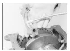
34.24 Lubricate the main bearing shells before fitting the caps -2.0 litre SOHC engine
