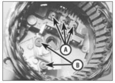
11.5 Delco-Remy alternatorA Stator lead securing nutsB Brush holder/voltage regulator securing screws
