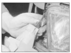
29.3 Disconnecting the front indicator lamp unit wiring plug
