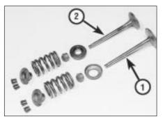
22.7 Inlet (1) and exhaust (2) valve components
