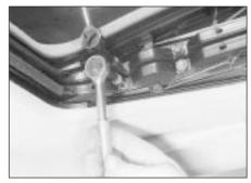
34.5 Loosening a glass panel securing screw
