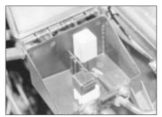
3.11 Relays in engine compartment box - 2.0 litre SRi model shown
