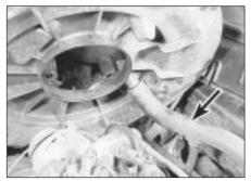
3.4 Disconnecting the crankcase ventilation hose (arrowed)
