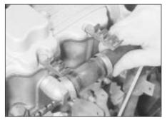
20.19A Disconnecting the crankcase breather tube stub hose -2.0 litre engine
