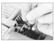
19.4 Disconnecting the throttle cable end from the throttle valve lever - SOHC model
