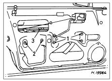
26.9 Front door window regulator and guide components
