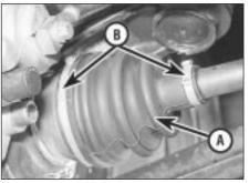
6.1 Check the condition of the driveshaft gaiters (A) and clips (B)
