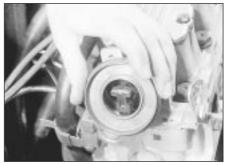
17.9 Removing the plastic shield from the rotor arm housing - 2.0 litre model
