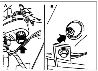
27.3B Headlamp alignment adjustment screws - models with electric aim adjustment
