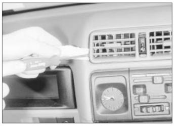
19.2A Using a screwdriver with protected blade . . .
