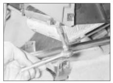
17.5 Unscrewing a heater matrix securing strap screw
