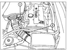
27.5A Hot film mass airflow meter attachments - Motronic M2.8
