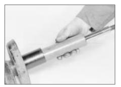
4.17B ... and withdraw the shock absorber cartridge
