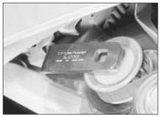
12.8 Using a special spanner to adjust the timing belt by moving the coolant pump
