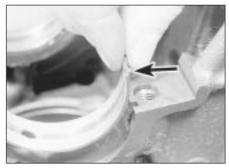
34.17 Main bearing shell tag (arrowed) engages with groove in cylinder block -2.0 litre SOHC engine
