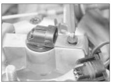
29.5 Unscrewing the injector retainer Torx screw
