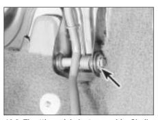
10.3 Throttle pedal pivot assembly. Circlip arrowed
