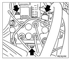
20.7 ABS hydraulic modulator securing screws (arrowed)
