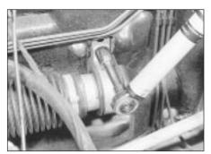
37.13 Tightening a steering gear mounting bolt
