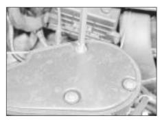
11.1 Removing an air box securing screw
