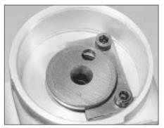
18.4 Camshaft thrustplate and securing bolts -1.6 litre engine
