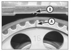
12.9B ... and stamped line (A) on camshaft sprocket with timing belt rear cover notch (B)
