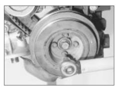
11.24B Tightening a crankshaft pulley securing bolt - 2.0 litre engine
