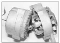
11.3 Separating the drive end housing from the slip ring end housing - Delco-Remy alternator
