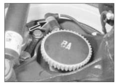
21.14 ABS rear wheel sensor (arrowed) - DOHC model
