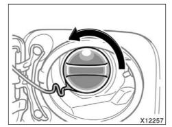
2. To remove the fuel tank cap, turn the cap counterclockwise. Pause slightly before removing it.
