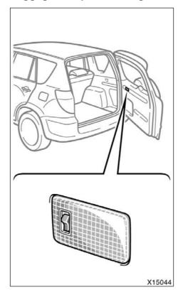
To turn on the luggage compartment light, push the luggage compartment light switch upwards. The light turn on when the back door is opened. The light goes off when the back door is closed.
