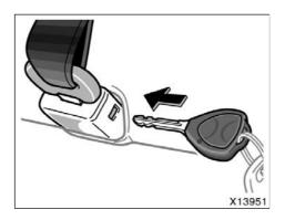
To release the hook end tab, insert the key into the hole on the buckle and allow the belt to retract.
