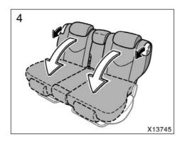
Pull down the seatback angle adjusting lever and fold down the seatback.
