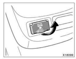
This power outlet is designed for use as a power supply for the audio device connected to the A/V input adapter.
