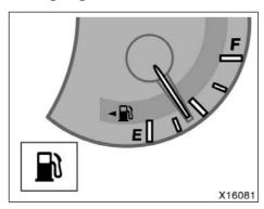
The gauge indicates the approximate quantity of fuel remaining in the tank when the ignition switch is on.
