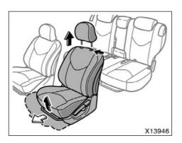
2. Remove the front head restraint. Hold the center of the lever and pull it up. Then slide the front seat further forward than the front-most lock position.
