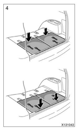
Push the seat on the front side against the floor and push the seat on rear side against the floor. Make sure it is locked securely.
