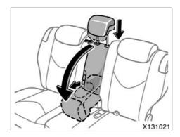
To use the armrest, lower the center head restraint. Pull the strap and pull the armrest down.
