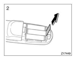
2. Remove the insulating sheet.
