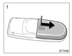
Remove the cover of the controller as shown.
