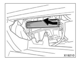
3. Remove the filter cover as shown in the illustration.
