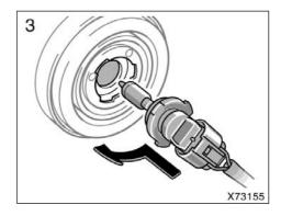
3. Pulg in a new bulb into the connector and install it into the mounting hole.
