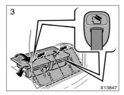
3. Pull and hold the seat lock release strap and lift up the seat rearward. Then push the seat down.
