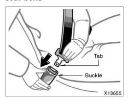
Adjust the seat as needed and sit up straight and well back in the seat. To fasten your belt, pull it out of the retractor and insert the tab into the buckle.
