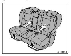
Hold the center of the lever and pull it up. Then slide the rear/second seats fully backward and pull it forward slightly until it locks.
