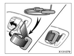
Insert the tabs of the center seat belt into the cover. Make sure the tabs are securely locked in the cover.
