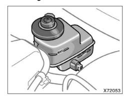
To check the fluid level, simply look at the see-through reservoir. The level should be between the "MAX" and "MIN" lines on the reservoir.
