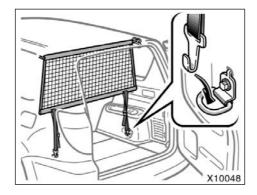
You can use the tie-down hooks to hook the claw of the separation net strap.
