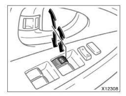
The windows can be operated with the switch on each door. The passengers' windows can also be controlled by the switches on the driver's door.
