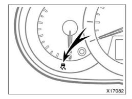
When the hill-start assist control system is operating, the slip indicator light flashes and the stoplights and high mounted stoplight are lit.
