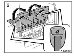
2. Pull the seatback lock release strap and raise the seatback.
