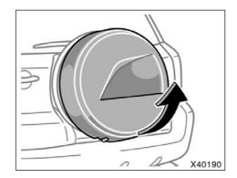
2. Close the back door. Remove the spare tire cover.
