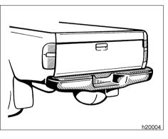
The rear step bumper is for rear end protection and easier step-up loading.
