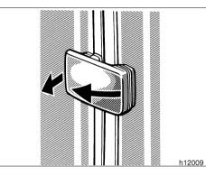
To unlock the rear window, pull the left end of the latch handle toward you and disengage the right end from the catch.
