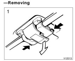
1. Pull the handle down while pushing in one of the lock buttons.
