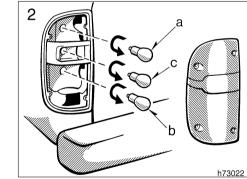
a: Rear turn signal light c: Back-up light b: Stop and tail light
