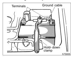
Check the battery for corroded or loose terminal connections, cracks, or loose hold-down clamp.
