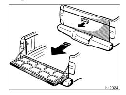
To open the tailgate, pull the handle up. The support cables will hold the tailgate horizontal.
