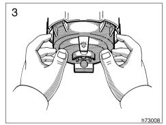
3. Install the rubber cover with the "TOP" mark upward and snuggle on the boss. Then insert the connector.
