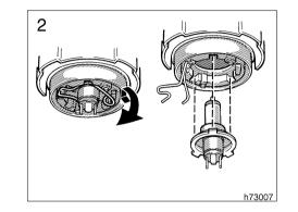
2. Release the bulb retaining spring and remove the bulb. Install a new bulb and the bulb retaining spring.
