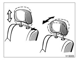
For your safety, adjust the head restraint before driving.
