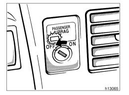
Only when you put a rear-facing child restraint system on the front seat unavoidably, turn the passenger airbag switch to the "OFF" position.
