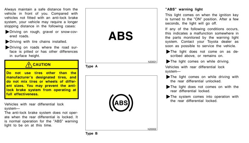
Even if the anti-lock brake system should fail, the brake system will still operate conventionally. However, when the "ABS" warning light is on (and the brake system warning light is off), the anti-lock brake system is not assisting brake performance so that the wheels can lock-up during sudden braking or braking on slippery road surfaces. Have your vehicle checked by your Toyota dealer as soon as possible.
