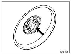
On steel wheel ornaments for free-wheeling hubs, place the wheel ornament replacer over the opening and tap on the replacer to snap the ornament into place. Be careful not to slip off the replacer.
