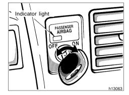
This system is designed to disable the passenger airbag in order to allow usage, if necessary, of a rear-facing child restraint system in the front seat. Disable the passenger airbag only when you put a rear facing child restraint system on the front seat unavoidably. Switch the system as follows:
