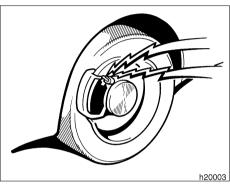
The brake pad wear limit indicators on your disc brakes give a warning noise when the brake pads are worn to where replacement is required.
