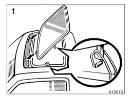
1. Insert the flat hinges of the moon roof panel into the cutouts on the body. Then slowly lower it while holding the roof with your hands.
