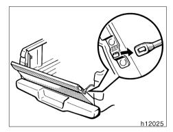
To lower the tailgate fully, release the support brackets from the lugs as shown.
