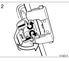
2. Press in the retaining spring arms and insert them into the holes. Then push the handle up with the palm of your hand and lock the roof.
