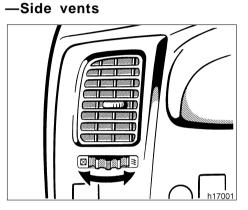
If air flow control is not satisfactory, check the side vents. The side vents may be opened or closed as shown.
