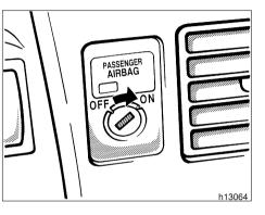
The passenger airbag system is equipped with a cutoff switch and indicator light. Turning the passenger airbag switch to the "ON" position makes the passenger airbag system operational. Turning the passenger airbag switch to the "OFF" position disables the passenger airbag system. The indicator light on the passenger airbag switch will come on when the passenger airbag system has been disabled.
