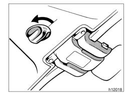
To remove: Support the sun shade panel with your hand while you unlock the sun shade by turning the knob counterclockwise.
