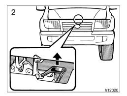
2. In front of the vehicle, pull up on the auxiliary catch lever and lift the hood.
