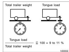
The trailer cargo load should be distributed so that the tongue load is 9 to 11 % of the total trailer weight, not exceeding 158 kg (350 lb.).
