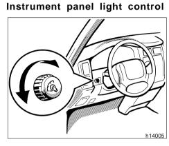
To adjust the brightness of the instrument panel lights, turn the knob.
