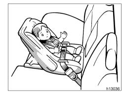
(A) INFANT SEAT INSTALLATION An infant seat is used in rear-facing position only. With the child restraint system installed, check that your driving position is satisfactory and that the child restraint system does not interfere with your driving.
