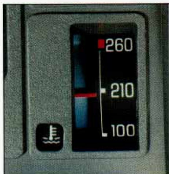
Engine Coolant Temperature Gage Standard Cluster
