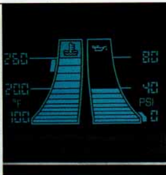
Engine Coolant Temperature Gage Digital Cluster
