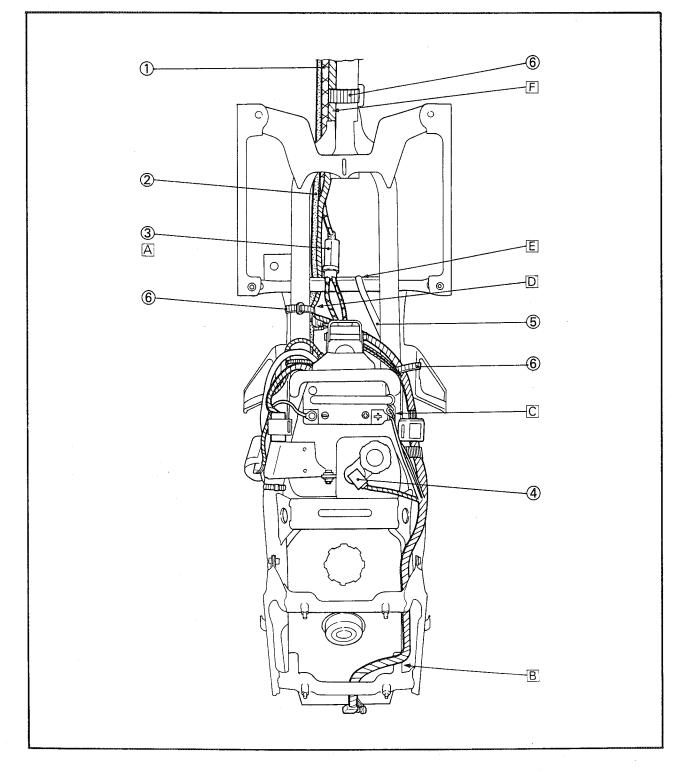
APPX **CABLE ROUTING** A Pass meter cable and brake cable through the 1 Inner fender 2 C.D.I. unit
