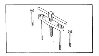
3. Primary Sheave Holder P/N. YS-01880This tool is used when holding the clutch hub.
