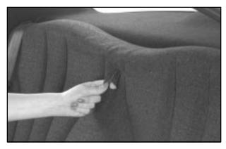
To open the fold-down rear seat, pull forward on the seat tab.
