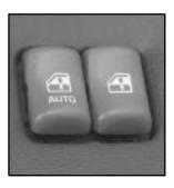
With power windows, switches on the center console control each of the windows only when the ignition is on. In addition, on four-door models, each rear passenger door has a control switch for its own window.
