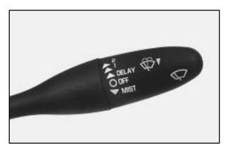
You control the windshield wipers by moving the stalk with the windshield wiper symbol on it up or down.
