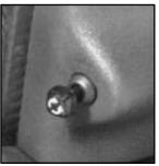
The mirror control is located on the driver's door. Turn the control clockwise or counterclockwise to choose the mirror you want to adjust.
