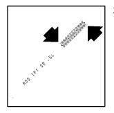
3. Check both sides of the dipstick, and read the lower level. The fluid level must be in the cross-hatched area.
