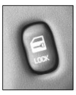
You can lock or unlock all doors of your vehicle from the driver's or front passenger's door lock switch.
