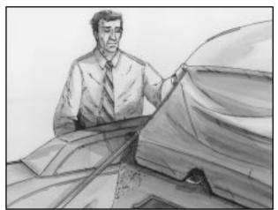
4. Go to the rear of the vehicle. Pull the snap knobs rearward to disengage the rear center cover. Carefully tuck the center boot behind the rear seatback. Make sure that the center cover is not covering the rear seatback latch. Tuck the end of the center boot rearward to keep it away from the rear seatback hinge.
