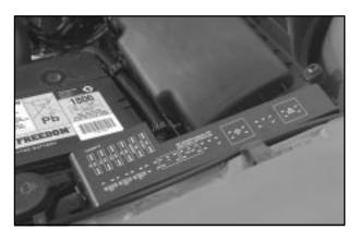
The engine compartment fuse block is located on the driver's side of the engine compartment. Lift the cover to check the fuses.
