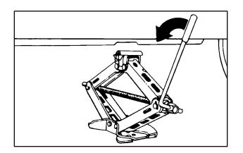
9. Lower the vehicle by turning the wheel jack handle counterclockwise. Lower the jack completely.
