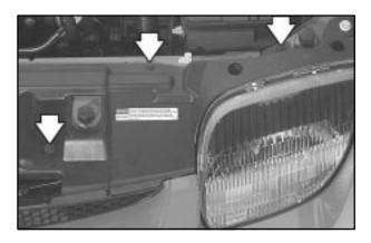
1. Remove the six plastic fasteners holding the shield. Use the end of a flat-head screwdriver to pull up the center of the fastener. Be careful not to break the fasteners that hold the shield in place.
