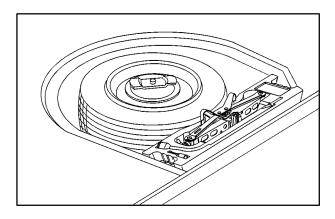
Lift and remove the tire cover. See "Compact Spare Tire" later in this section for more information about the compact spare.
