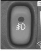
Use your fog lamps for better vision in foggy or misty conditions. The switch for your fog lamps is next to the instrument panel intensity control.
