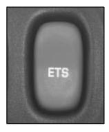
To turn the system on or off, press the ETS button on the located on the left side of the instrument panel near the instrument panel brightness control.
