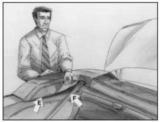
4. Attach the two snaps on the inside flap of the side cover, to the side of the quarter trim panel. Attach the front snap (E) first and then the rear snap (F). The rear snap is adjustable for ease of installation. Repeat this step for the opposite side boot cover.
