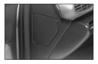
The fuse panel is located at the driver's side end of the instrument panel. To open, push the tab on the access door to the left and pull the door forward. There is a white fuse removal tool located in the fuse block area. Make sure to insert the tabs first when reinstalling the cover.
