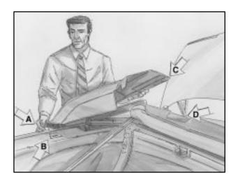
3. Install the boot side cover by inserting the tab (A) on the underside of the cover into the slot (B) at the top of the quarter trim panel. Place the rear flap of the boot side cover in the trunk lid opening, aligning the eyelet (C) over the boot snap ball stud (D). Repeat this step for the opposite side boot cover.
