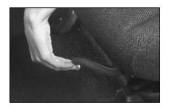
Lift the lever under the driver's seat to unlock it. Slide the seat to where you want it. Then release the lever and try to move the seat with your body, to make sure the seat is locked into place.
