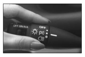
The band on the turn signal/multifunction lever controls your vehicle's lamps.
