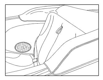
5. Raise the rear seatback to the up position. Push the seat back to make sure it is latched.
