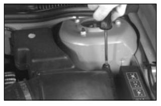
To check or replace the filter, remove the screws that hold the cover on and lift the cover. Be sure to reinstall the air cleaner filter and reinstall the cover tightly.
