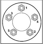
10. Tighten the wheel nuts firmly in a crisscross sequence, as shown.
