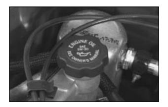
This is where you add oil if you have a 2.4L L4 Engine. Be sure to fill it enough to put the level somewhere in the proper operating range. Push the dipstick all the way
