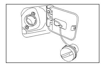
While refueling, hand the cap inside the fuel door by placing the fuel cap strap in the strap hanger.
