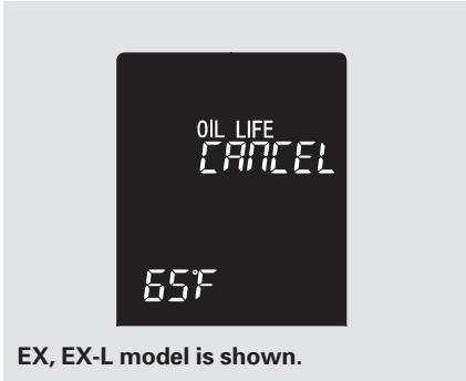
3. Press the select/reset knob for about 10 seconds. The information display shows the reset mode initial display as shown.
