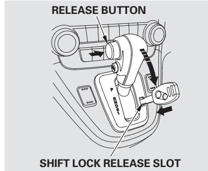
6. Remove the key from the shift lock release slot, then reinstall the cover. Make sure the notch on the cover is on the right side. Insert the key back into the ignition switch, press the brake pedal, and restart the engine.
