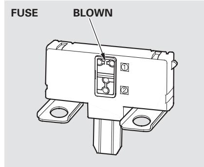
3. Check each of the large fuses in the under-hood fuse box by looking through the side window at the wire inside. Removing these fuses requires a Phillips-head screwdriver.
