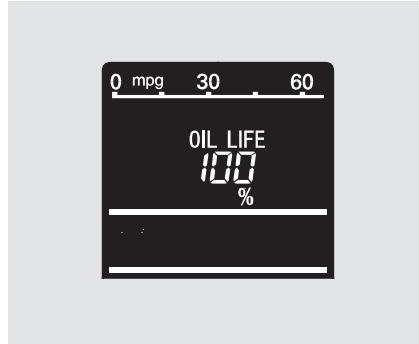
5. The engine oil life and the maintenance item code(s) will begin to blink. Press the select/reset knob for another 5 seconds.
