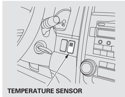
The climate control system has two sensors: a sunlight sensor on top of the dashboard, and a temperature and humidity sensor next to the steering column. Do not cover the sensors or spill any liquid on them.
