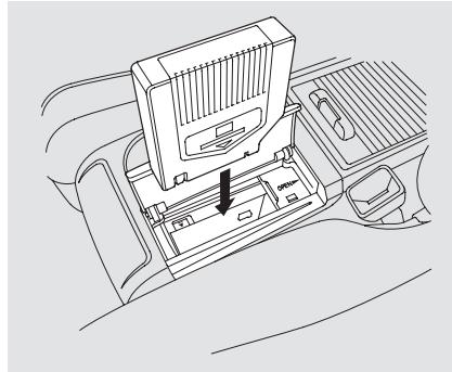
6. Store all six trays in the magazine, and reinstall the magazine in the CD changer as shown.
