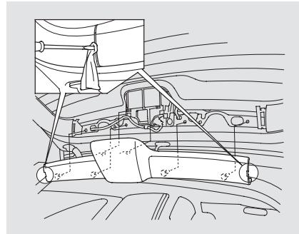
2. Place a cloth on the side edge of the cover to prevent scratches. Remove the cover by carefully prying on the edge with a small flat-tip screwdriver and pulling the cover off.
