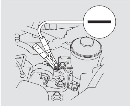
4. Connect the second jumper cable to the negative (−) terminal on the booster battery. Connect the other end to the stud bolt on the engine side as shown. Do not connect this jumper cable to any other part of the engine.
