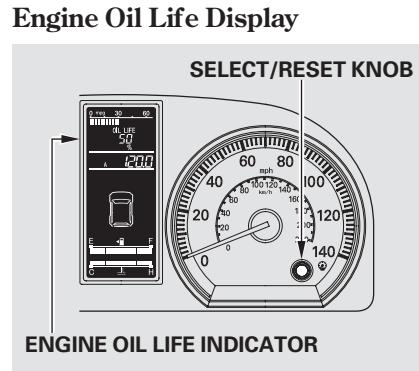
To see the current engine oil life, turn the ignition switch to the ON (II) position, then press and release the select/reset knob repeatedly until the engine oil life indicator appears (see page 68).
