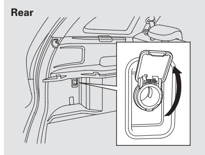
Make sure to put the socket cover back in place to prevent any small foreign objects from getting into the socket.
