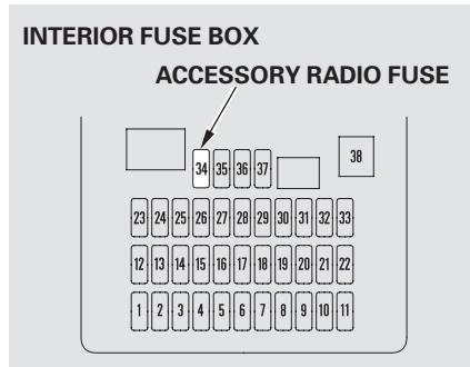
Only remove the fuse after you have performed the transmission shifting procedure, and the key is in the ACCESSORY (I) position. Store the fuse in an obvious location (center tray, coin pockets, etc) as a reminder to re-install the fuse before driving
