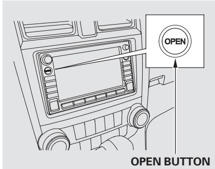
The in-dash disc player is behind the navigation screen. To use the disc player, press the OPEN button beside the screen. The screen folds back, and the disc slot appears.
