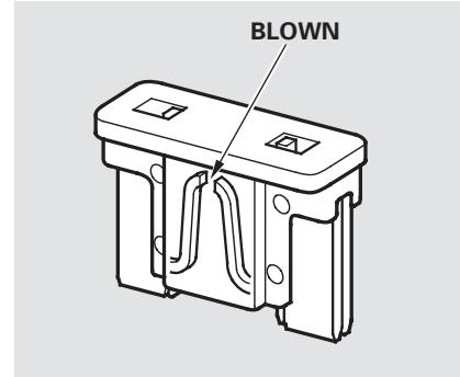
4. Check the smaller fuses in the under-hood fuse box and all the fuses in the interior fuse box by pulling out each one with the fuse puller provided on the back of the under-hood fuse box cover.
