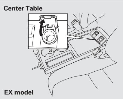
To use an accessory power socket, the ignition switch must be in the ACCESSORY (I) or ON (II) position.
