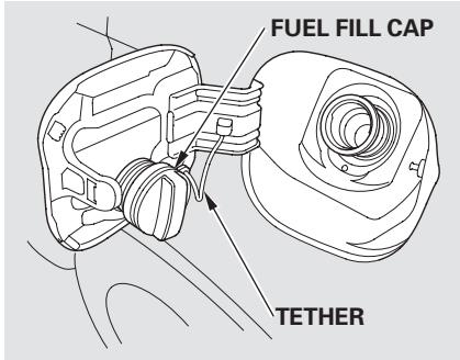
3. Remove the fuel fill cap slowly. You may hear a hissing sound as pressure inside the tank equalizes. The fuel fill cap is attached to the fuel filler with a tether. Place the cap in the holder on the fuel fill door.
