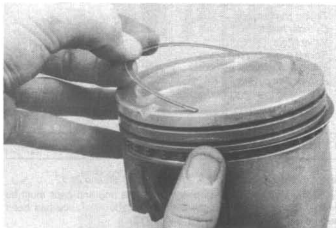
21.9b DO NOT use a piston ring installation tool when installing the oil ring side rails
