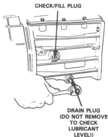
5.1 The manual transmission lubricant check/fill plug is located on the right side of the transmission case (which is the passenger's side of the vehicle) – a 3/8-inch drive ratchet or breaker bar will fit into the square hole to unscrew the plug
