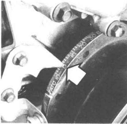
3.6a Turn the crankshaft until the zero on the vibration damper scale is directly opposite the pointer
