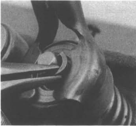
8.3 Use a valve spring compressor to compress the spring, then remove the keepers from the valve stem
