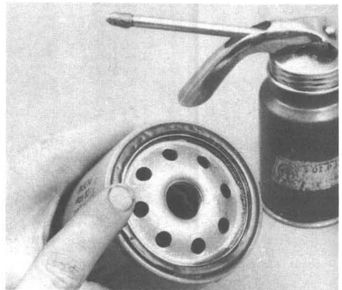
10.16 Lubricate the oil filter gasket with clean engine oil before installing the filter on the engine
