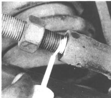
19.2b Use white paint to mark the position of the tie-rod end on the tie-rod
