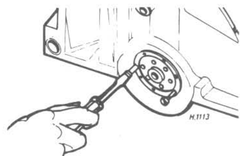
15.20 Thread two sheet metal screws into the crankshaft rear oil seal to pry it out
