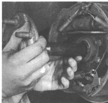
18.19 Pull the axle out of the housing, supporting it with one hand to prevent damage to the seal
