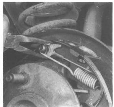
6.4v Bend the ends of the return springs around the anchor pin
