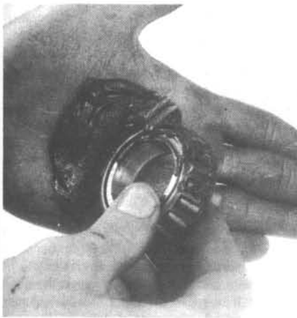
28.15 Pack each wheel bearing by working the grease into the rollers from the back side
