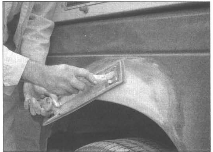
8 Use coarse-grit sandpaper and a sanding board or block to work the filler down until it's smooth and even. Work down to finer grits of sandpaper - always using a board or block - ending up with 360 or 400 grit
