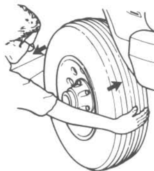
24.11 To check the steering gear mounts and tie-rod connections for play, grasp each front tire like this and try to move it back-and-forth – if play is noted, check the steering gear mounts and make sure that they're tight; if either tie-rod is worn or bent, replace it
