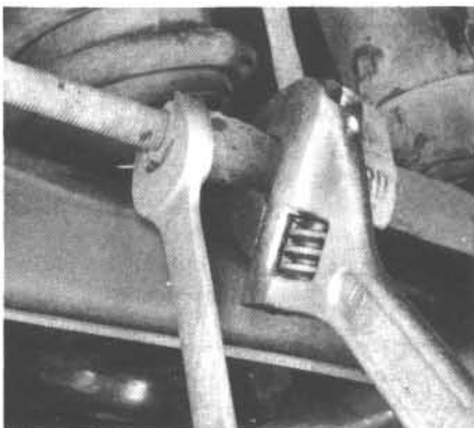
19.2a Hold the tie-rod end with a wrench and loosen the jam nut
