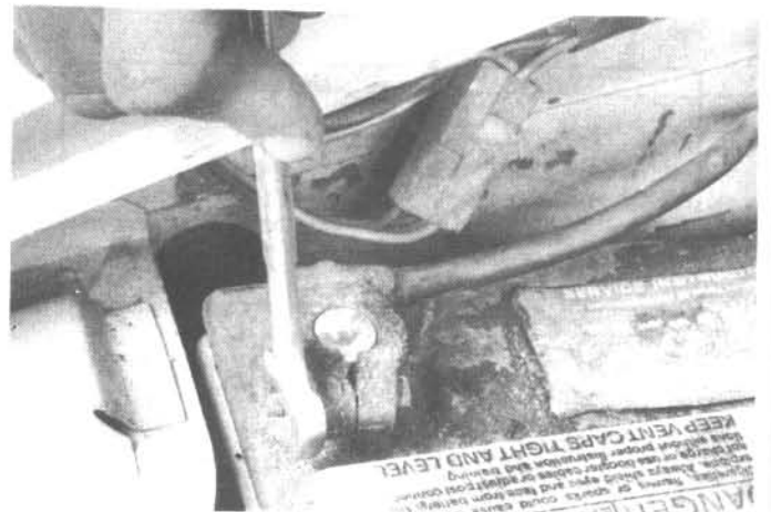
15.8b Removing the cable from a battery post with a wrench – sometimes a special battery pliers is required for this procedure if corrosion has caused deterioration of the nut hex (always remove the ground cable first and hook it up last!)
