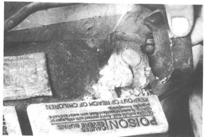
15.8a Battery terminal corrosion usually appears as light, fluffy powder
