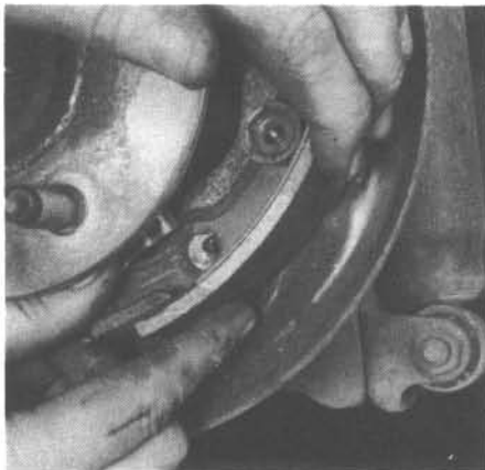
6.4q Hook the other end of the spring into the adjuster lever and push the lever toward the secondary shoe, hooking it into the hole provided
