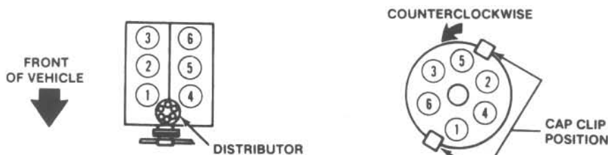
Cylinder locations and firing order – 3.8L V6 engine
