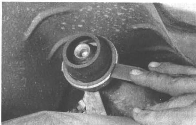
6.3 A chisel is used here to carefully tap around the flange of the oil seal and separate it from the transmission extension housing
