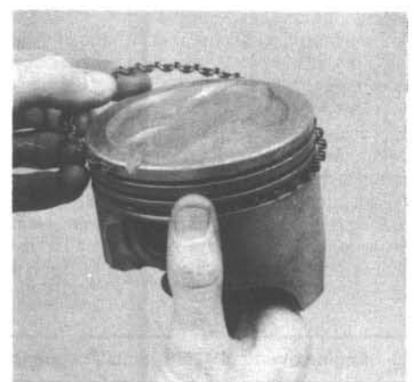
21.9a Installing the spacer/expander in the oil control ring groove
