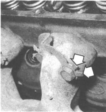
8.12c Some models are equipped with manifold bolt locking tabs – bend these down before removing the bolts – use new locking assemblies on installation, bending the tabs up to lock the bolts in place
