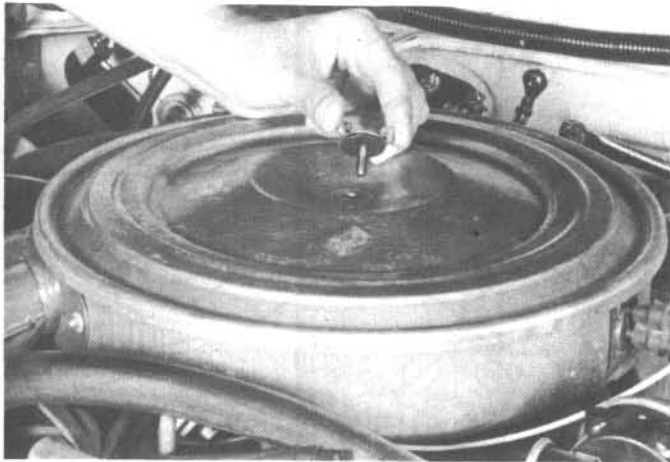
16.2 On carbureted and CFI models, remove the air cleaner wing nut ...
