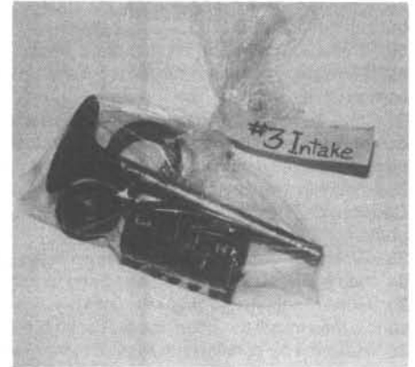
8.5 A small plastic bag, with an appropriate label, can be used to store the valve train components so they can be kept together and reinstalled in the original location
