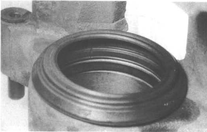
3.18 Install the dust boot in the upper groove in the caliper bore, making sure it's completely seated
