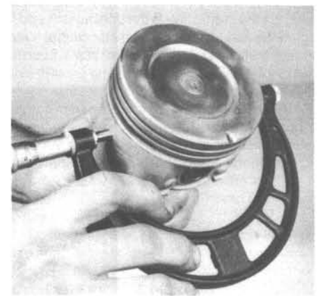
17.11 Measure the piston diameter at a 90-degree angle to the piston pin and in line with it
