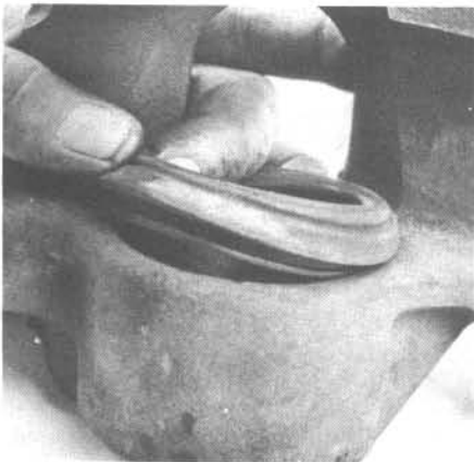
3.6 Remove the dust boot from the caliper bore groove
