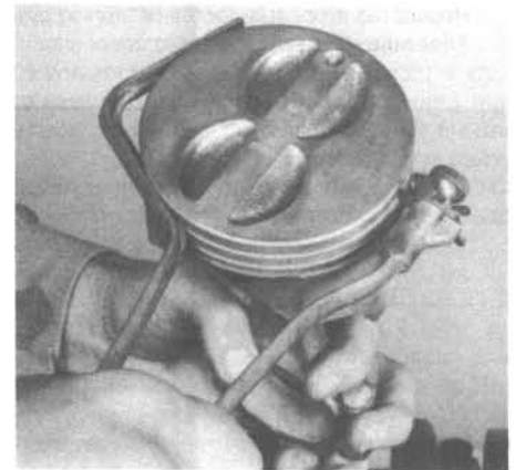
17.4a The piston ring grooves can be cleaned with a special tool, as shown here, . . .
