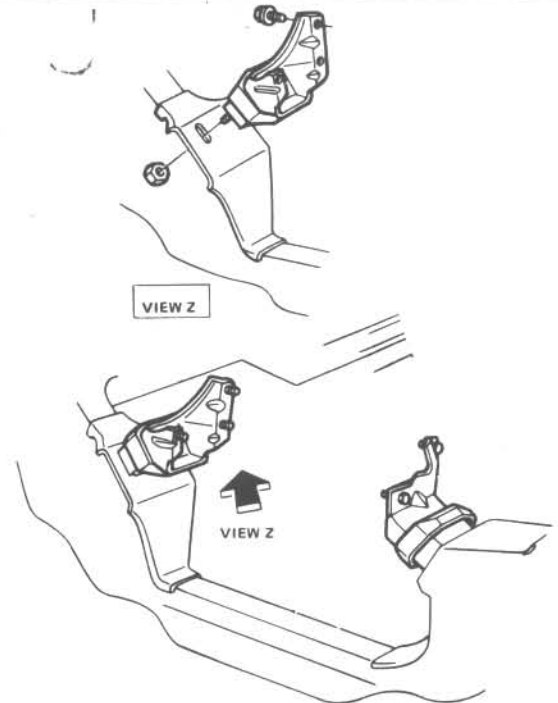
17.8 Engine mount details – typical
