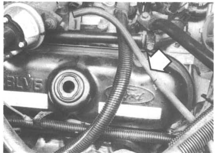
4.11 Remove the oil filler cap and, after disconnecting the exhaust heat control valve vacuum hose (arrow), push it aside
