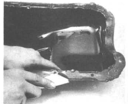
14.20 Scrape away all traces of gasket material and sealant, then clean the gasket surfaces with lacquer thinner or acetone
