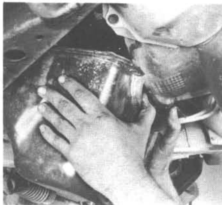
14.19 Slip the oil pan out, turning it slightly to clear the oil pick-up (V6 engine)
