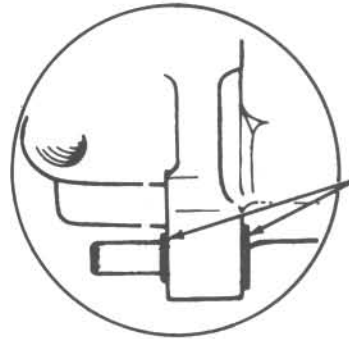
3.14 Push the new insulators through the holes in the caliper ears, making sure they are installed all the way; on models with plastic sleeves inside the insulators, install the sleeves
