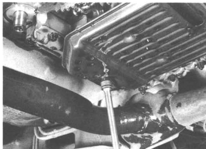
12.12 The automatic transmission filter is held in place with small bolt(s)
