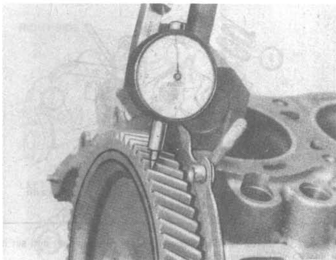
11.5 Timing gear backlash is checked with a dial indicator positioned against one of the camshaft gear teeth
