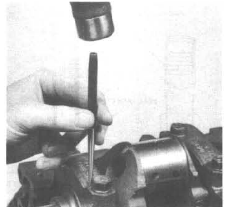
13.4a Use a center punch or number stamping dies to mark the main bearing caps to ensure installation in their original locations on the block (make the punch marks near one of the bolt heads)
