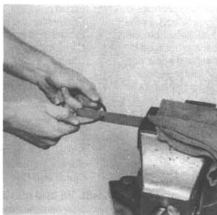
21.5 If the end gap is too small, clamp a file in a vise and file the ring ends (from the outside in only) to enlarge the gap slightly
