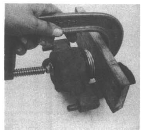
3.20 Use a C-clamp and a block of wood to bottom the piston in the caliper bore – make sure it goes in perfectly straight, or the sides of the piston may be damaged, rendering it useless
