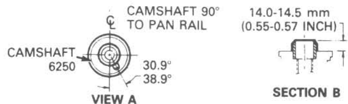
12.31 Be sure to turn the camshaft until the pin is in the five o'clock position as shown here before installing the head
