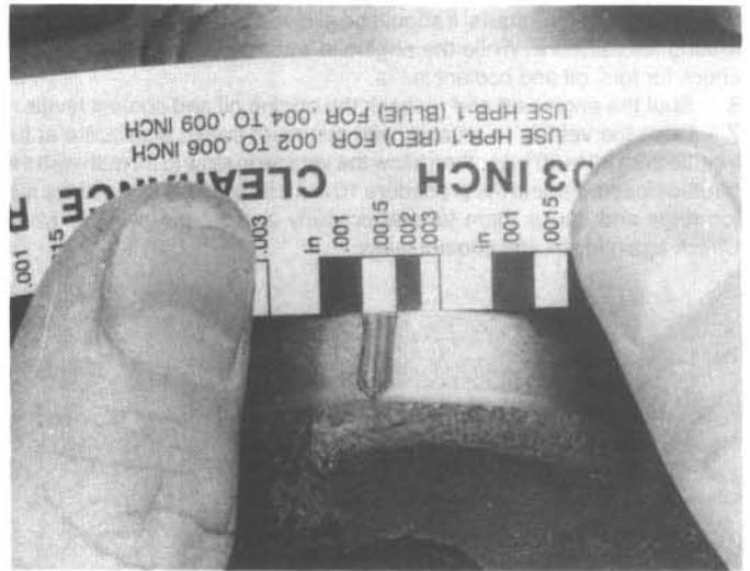
24.17 Measuring the width of the crushed Plastigage to determine the rod bearing oil clearance (be sure to use the correct scale – standard and metric ones are included)
