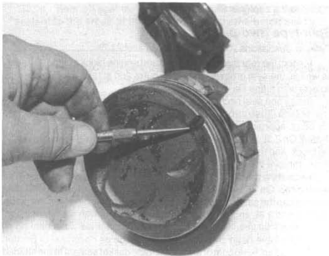
24.9 The notch or arrow in the top of each piston must face the FRONT of the engine as the pistons are installed
