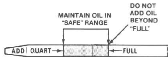
3.4 The engine oil level should be in the SAFE range – if it's below the ADD line, add enough oil to bring the level into the SAFE range (DO NOT add more oil if the level is at the FULL line)
