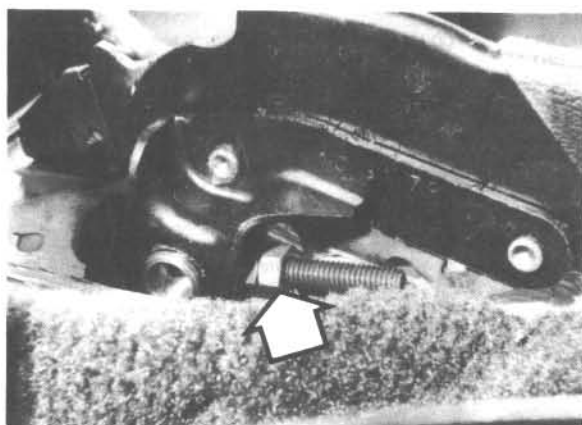
12.4 Parking brake equalizer locknut and adjusting nut – models with rear drum brakes (arrow)
