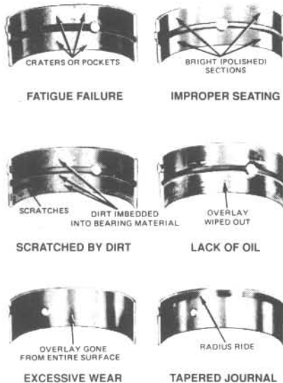
19.1 Typical bearing failures
