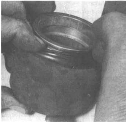
3.21 Install the lip of the dust boot in the groove in the caliper piston
