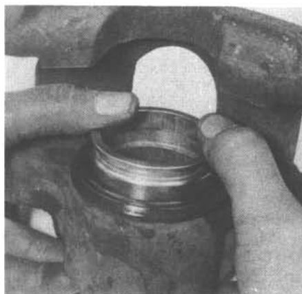
3.19b . . . and push it straight into the caliper as far as possible by hand
