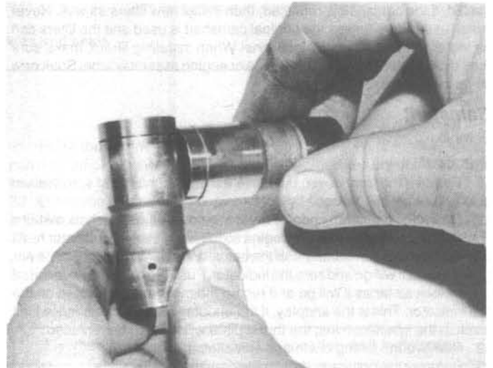
9.8b The foot of each lifter should be slightly convex – the side of another lifter can be used as a straightedge to check it; if it appears flat, it's worn and must not be reused
