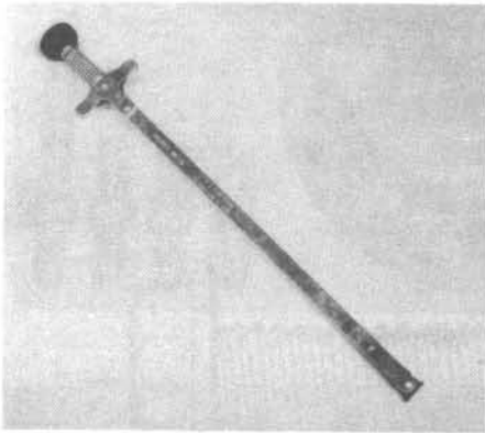
Hydraulic lifter removal tool
