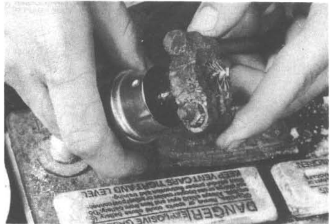
15.8d When cleaning the cable clamps, all corrosion must be removed (the inside of the clamp is tapered to match the taper on the post, so don't remove too much material)
