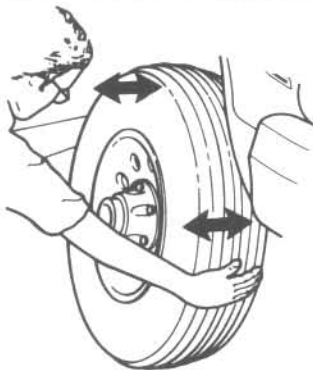
28.3 To check the wheel bearings, try to move the tire in-and-out – if any play is noted, or if the bearings feel rough or sound noisy when the tire is rotated, maintenance is required
