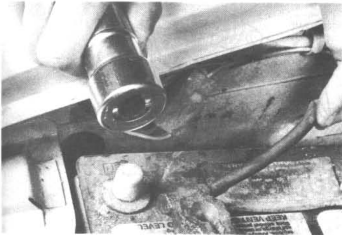
15.8c Regardless of the type of tool used on the battery posts, a clean, shiny surface should be the result
