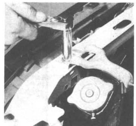
4.8 Removing the upper radiator mounting bolts (inline six-cylinder model shown)
