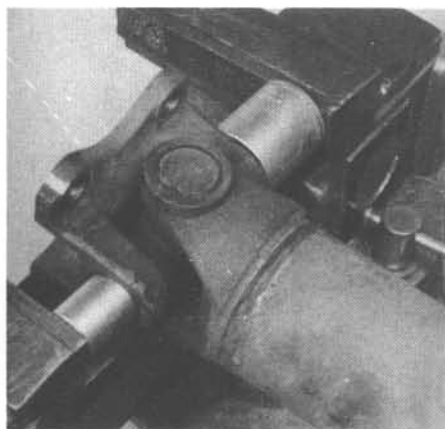
16.4 To press the universal joint out of the driveshaft yoke, set it up in a vise with the small socket pushing the joint and bearing cap into the large socket
