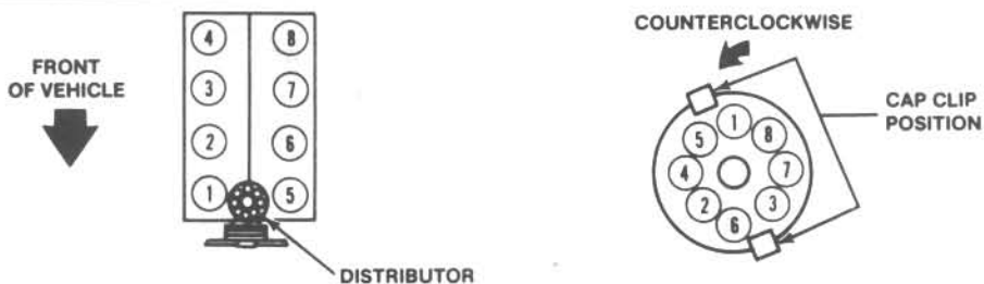
Cylinder locations and firing order - V8 engines except HO
