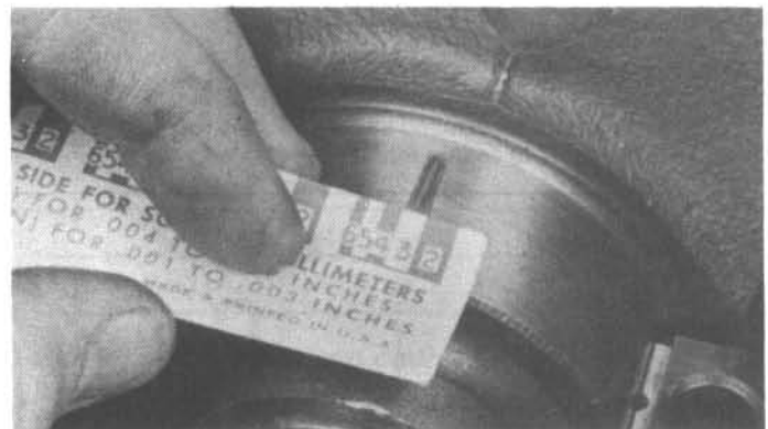
22.15 Compare the width of the crushed Plastigage to the scale on the envelope to determine the main bearing oil clearance (always take the measurement at the widest point of the Plastigage); be sure to use the correct scale – standard and metric ones are included
