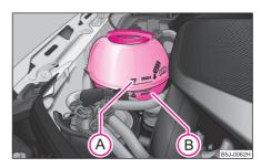
Fig. 159 Engine compartment: Coolant expansion bottle
