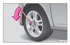
Fig. 172 Changing a wheel: Slackening wheel bolts
