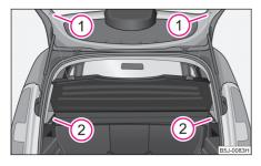
Fig. 63 Removing the luggage compartment cover
