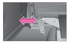
Fig. 201 Bottom support of the safety partition
