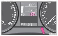
Fig. 3 Display: Counter for distance driven
