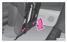
Fig. 54 Unlocking the folded forward seat
