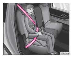
Fig. 141 Child seat in Group 3 installed on the rear seat facing the direction of travel
