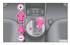
Fig. 108 Selector lever: Manual shifting of gears
