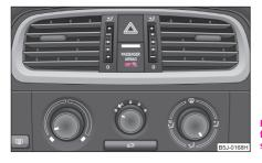
Fig. 134 Indicator light for a switched off front seat passenger airbag
