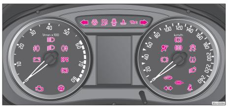
Fig. 15 Instrument cluster with warning lights
