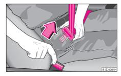
Fig. 124 Releasing lock tongue from belt lock
