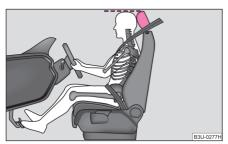
Fig. 117 The correct head restraint adjustment for the driver
