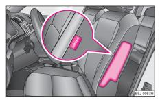
Fig. 129 Driver seat: Installation position of airbag
