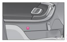
Fig. 27 Interior monitor pushbutton
