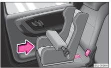
Fig. 143 The ISOFIX child seat is pushed into the mounting funnels
