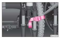
Fig. 68 Fastening the front wheel
