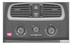
Fig. 39 Switch for rear window heater
