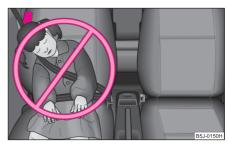
Fig. 136 Seated position of an unprotected child at risk from side airbag
