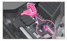
Fig. 181 The battery: Opening of the positive terminal cover.
