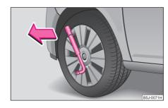
Fig. 169 Removing the full wheel trim
