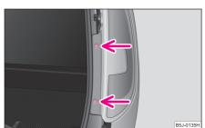
Fig. 191 Remove the rear light unit
