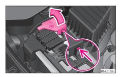
Fig. 161 The battery: Open up the cover
