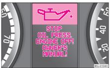
Fig. 13 Information display: Oil pressure is low
