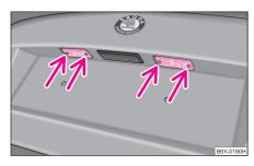
Fig. 190 Remove the licence plate light
