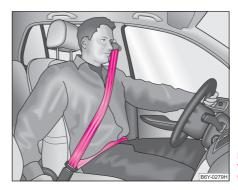
Fig. 121 Routing of webbing over the shoulders and the lap belt
