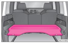
Fig. 64 Luggage compartment cover in the lower position
