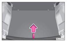
Fig. 198 Loop for raising the loading floor
