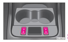
Fig. 48 Rocker switch: Front seat heating
