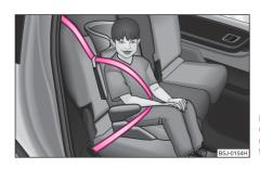
Fig. 140 Child seat in Group 2 installed on the rear seat facing the direction of travel
