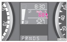
Fig. 5 Instrument cluster: Multi-functional indicator
