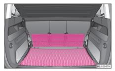
Fig. 61 Fixing net: double horizontal pocket, floor fixing net
