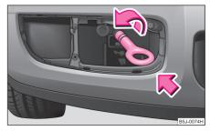
Fig. 177 Front bumper: Installing the towing eye
