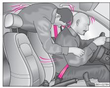
Fig. 120 The rear seat occupant is thrown forward if not wearing a belt
