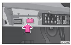
Fig. 32 Fuse box: Switch for daylight driving lights
