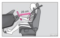
Fig. 116 The correct distance of the driver from the steering wheel
