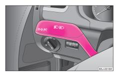
Fig. 36 Turn signal and main beam lever
