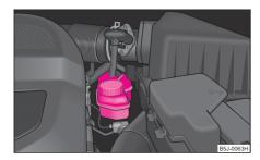
Fig. 160 Engine compartment: Brake fluid reservoir
