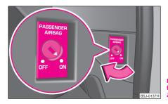
Fig. 133 Switch for the front seat passenger airbag(s)
