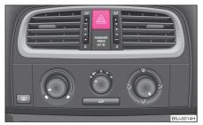
Fig. 35 Dash panel: Switch for hazard warning lights
