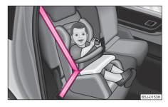
Fig. 139 Child seat with padded table in Group 1 installed on rear seat bench facing the direction of travel
