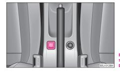
Fig. 147 Button for setting the tyre inflation pressure control value
