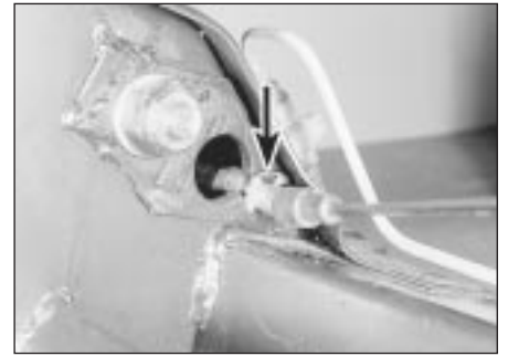
30.21a Pull out the clip (arrowed) . . .
