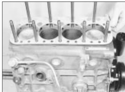
4.7 Removing the cylinder head gasket (1275 cc engine)
