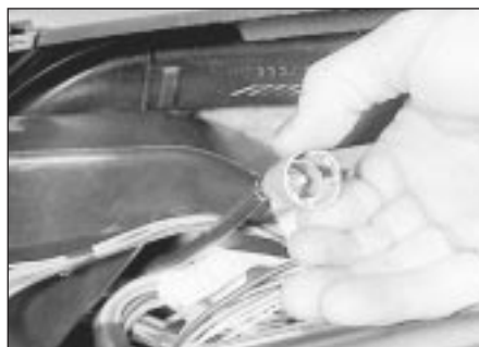
14.17 Squeeze the speedometer cable connector to release it
