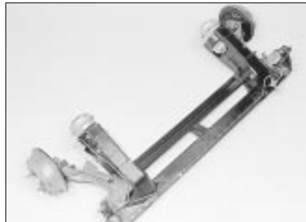
30.22 Rear subframe removed from the car
