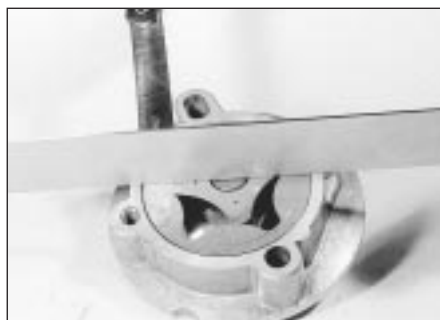
8.9b . . . outer rotor endfloat . . .
