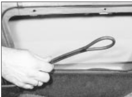
8.11a Fuel tank vent tube
