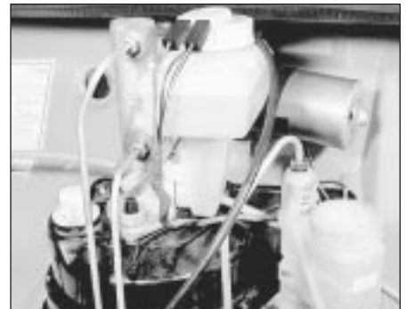
12.5 Brake master cylinder location (left) showing fluid level warning switch wires - clutch master cylinder on right
