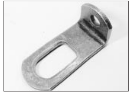
3.27 Suitable engine lifting bracket
