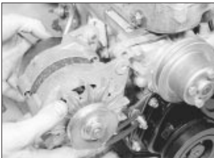
12.5 Removing the alternator
