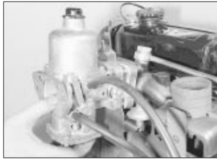
13.12b Removing the carburettor
