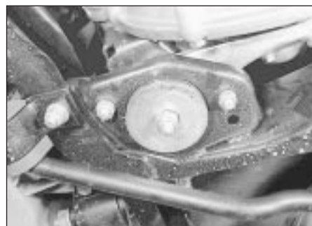
3.28e Right-hand front engine mounting (from below)
