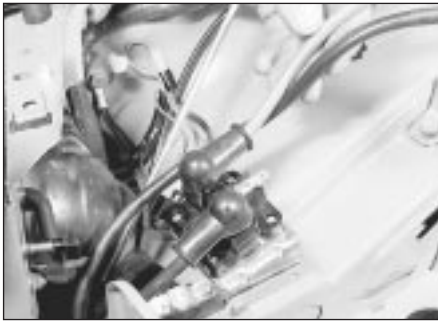
3.3 Removing the solenoid
