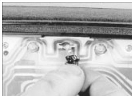
14.5a Removing a bulb holder from the instrument panel - early model
