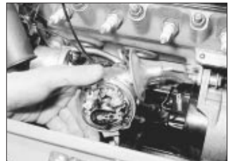
6.9B Installing the distributor (engine in car)
