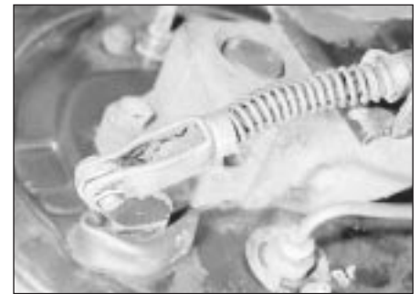
30.12 Handbrake cable end fitting and clevis pin
