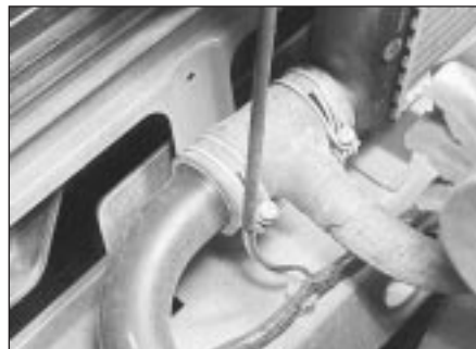
1.4 Bottom hose with take-off for oil cooler
