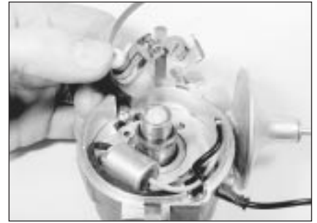
34.3 Removing the contact breaker set (Lucas)
