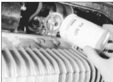
3.7b Removing the oil filter cartridge
