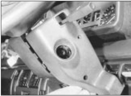
5.4 Removing the right-hand steering column cowl
