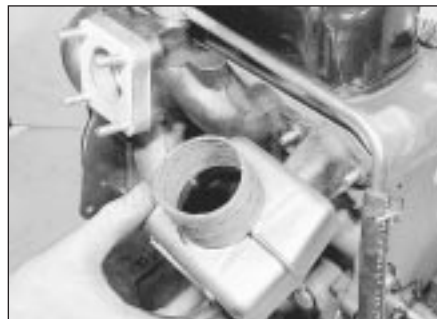
19.4b. . . and withdraw the heat stove
