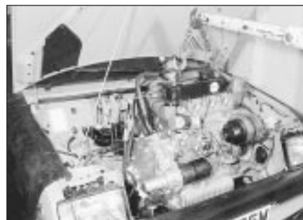
3.30a Removing the engine/gearbox
