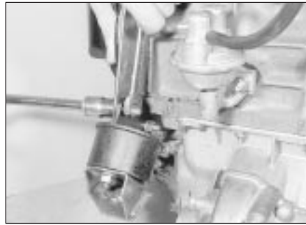
5.1a Left-hand rear engine mounting
