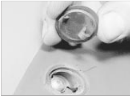
34.1 Rear spoiler screw cover plug
