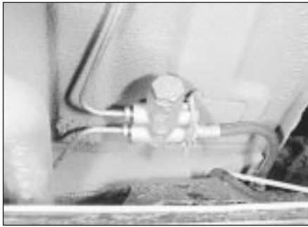
1.2a Pressure compensating valve (early models)
