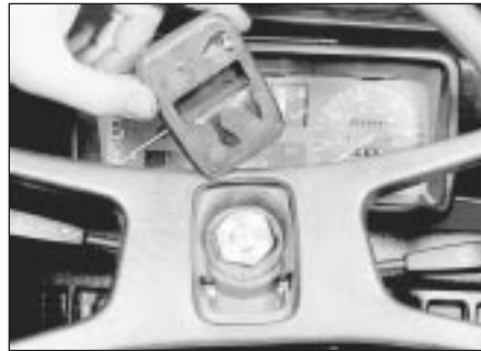
14.2 Removing the steering wheel central cover
