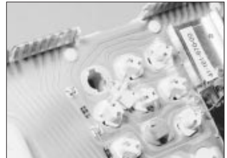
14.20b Removing a warning light bulb
