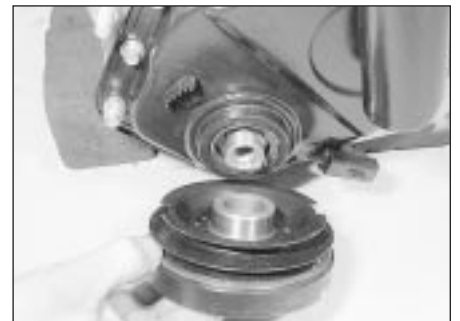
6.6 Removing the crankshaft pulley and damper (1275 cc engine)
