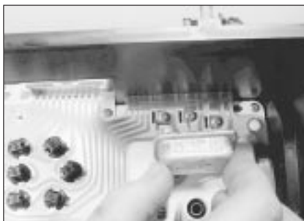
15.3 Extracting the voltage stabilizer
