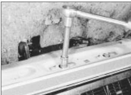
11.6a Removing the front heater mounting bolts
