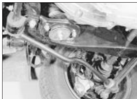
5.5 Anti-roll bar and front bearing bracket
