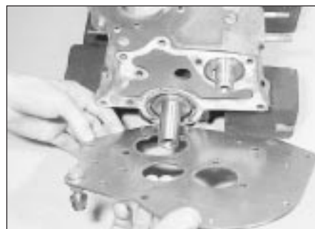
10.3 Removing the engine front plate
