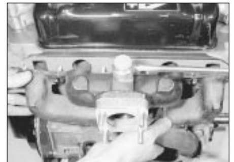
19.5 Removing the manifold (1.3 HLS)
