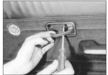
15.1c Removing the interior door handle surround screw . . .
