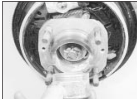
12.4 Removing the rear hub grease cap
