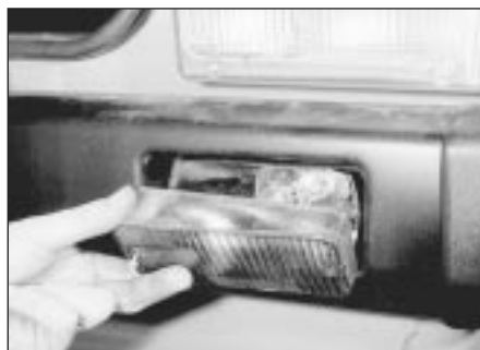
12.13 Removing the rear foglamp lens
