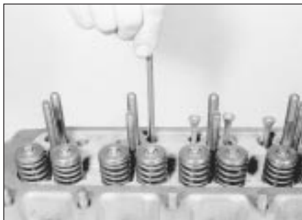
4.5 Removing a pushrod
