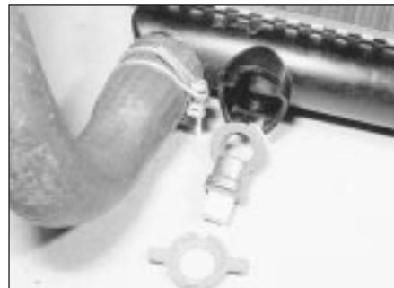
9.3 Thermostatic switch components
