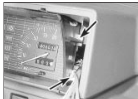
14.18 Instrument panel side screws (arrowed)
