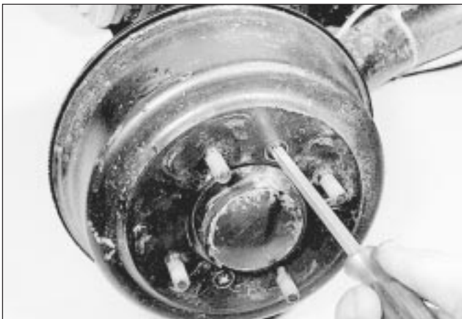
5.2 Removing the brake drum
