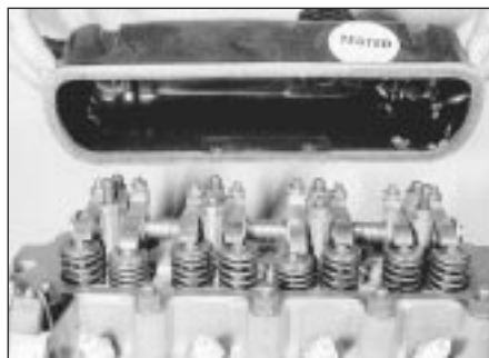
4.1b Removing the rocker cover
