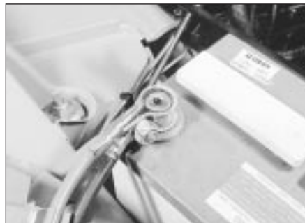
3.3 Battery positive terminal and lead
