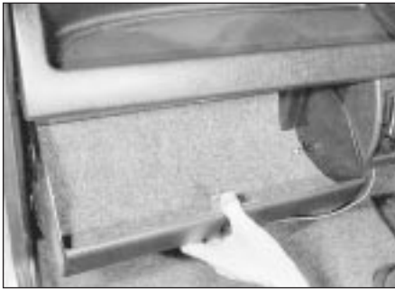
29.2 Removing the glovebox
