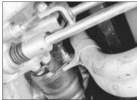
27.5b Exhaust system front mounting clamp (1.3 HLS)
