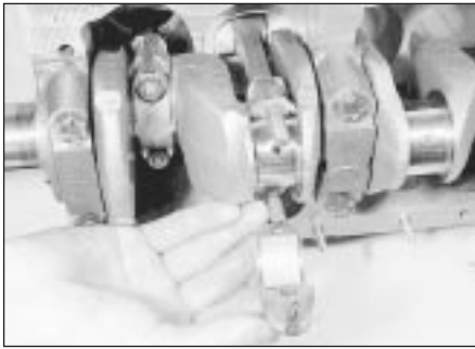
9.6 Removing a big-end bearing cap
