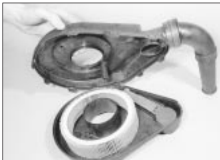
5.1 Removing the air cleaner lid
