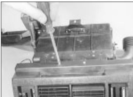
11.8b Removing the heater cover panel
