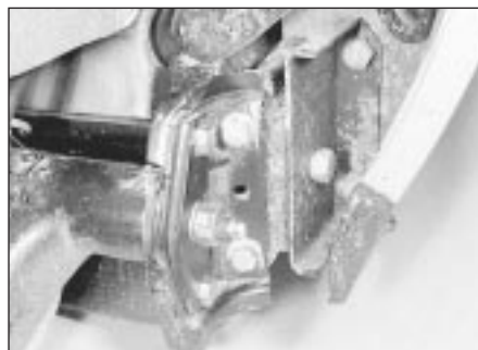
11.5b Rear suspension arm outer mounting
