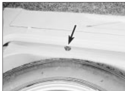
10.4c ... and reaction strap inner mounting nut (arrowed)
