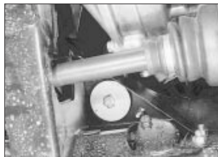
3.29b Right-hand rear engine mounting (from below)
