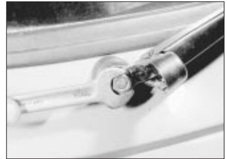
21.3 Unscrewing the wiper arm spindle nut
