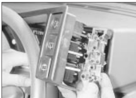
7.2e ... then disconnect the multi-plugs (later models)
