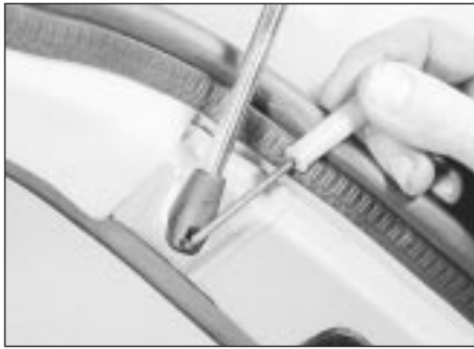
9.2a Releasing the tailgate strut locking peg
