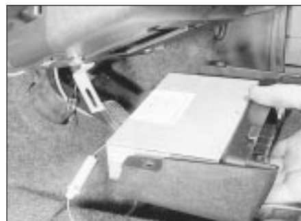
29.4 Removing the radio
