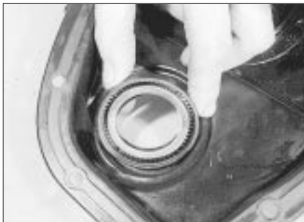
6.17 Fitting the timing cover oil seal
