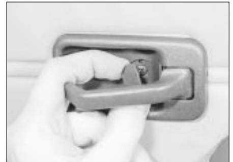
15.1e Removing the plastic cap from the interior door handle surround - later models
