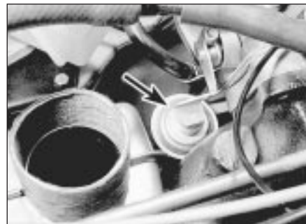
16.2 Throttle damper location
