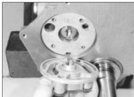
8.4a Removing the oil pump . . .
