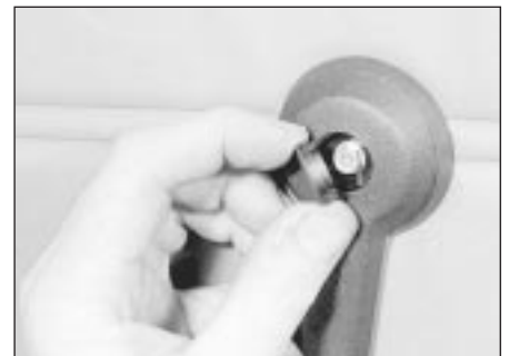
15.2b Removing the plastic cap from the window regulator handle - later models
