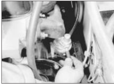
5.6b Disconnecting the outlet pipe from the fuel pump
