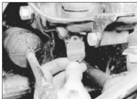
5.1 Removing a front suspension rebound buffer
