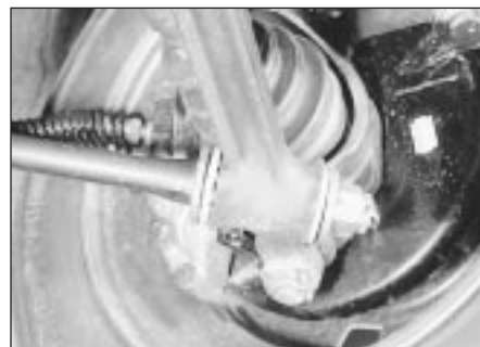
5.4 Anti-roll bar-to-lower suspension arm joint
