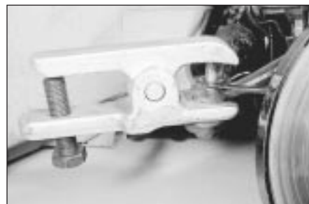
17.3b Using a separator tool to release the tie-rod end balljoint
