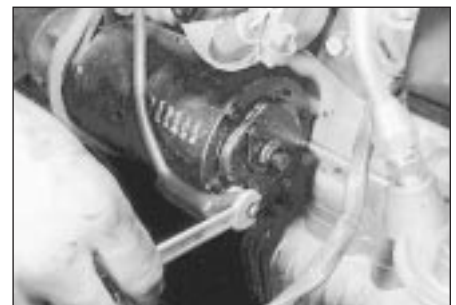
14.10 Disconnecting the starter supply lead
