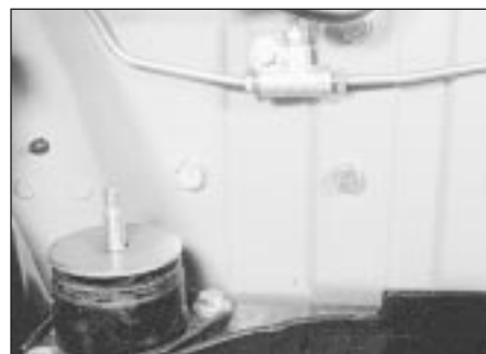
3.29a Right-hand rear engine mounting (from above) - engine removed
