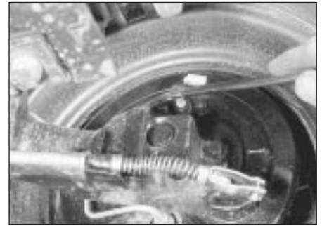
3.3 Adjusting the rear brakes
