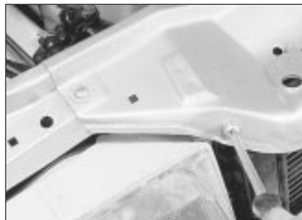
5.3b Removing the front cross panel mounting screws
