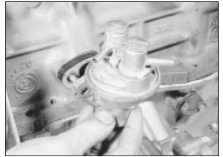
5.7 Removing the fuel pump (except MG Turbo)
