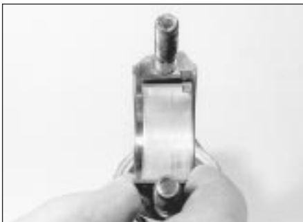
9.19a Installing a big-end bearing shell
