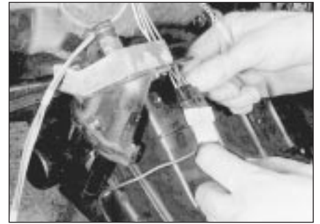
11.5 Disconnecting the heater wiring multi-plug
