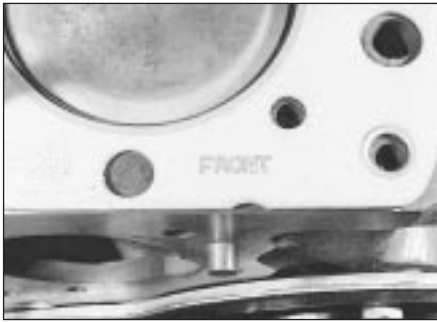
4.9 Cylinder head gasket "FRONT" marking
