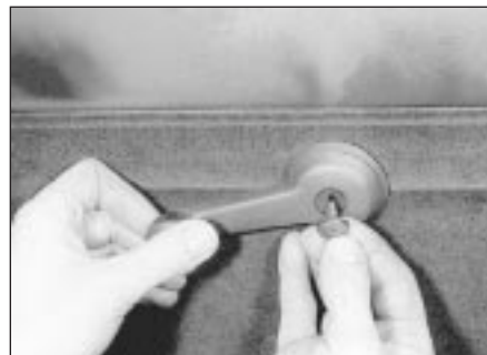
15.2a Removing the window regulator handle - early models
