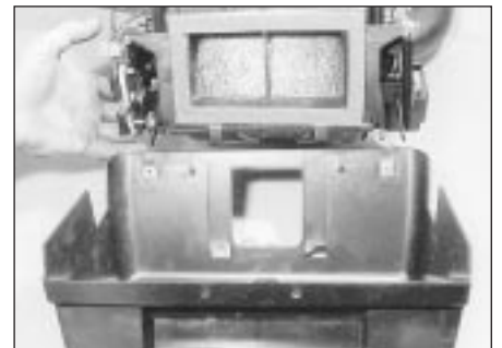
11.12 Removing the heater case
