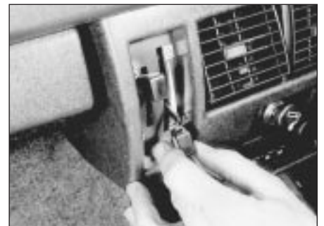
11.8a Removing the heater control knobs
