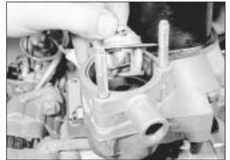
6.4 Removing the thermostat
