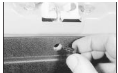
22.4 Removing a tailgate trim panel fastener
