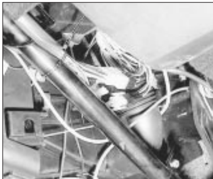
15.3 Steering column and wiring multi-plug
