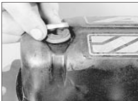
4.1a Rocker cover washer and seal
