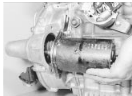
14.12 Removing the starter motor
