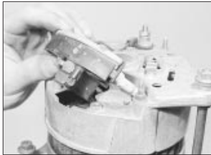
13.3B Withdraw the regulator and brushbox . . .
