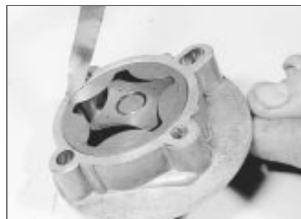
8.9c . . . outer rotor clearance . . .
