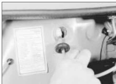
18.3 Removing the speedometer cable from the head
