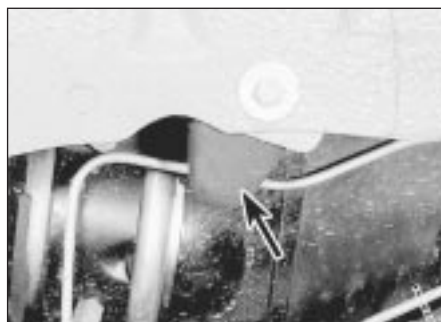
10.4a Rear suspension bump rubber (arrowed) ...
