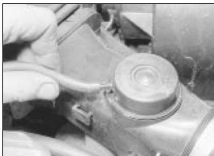
2.1 Air cleaner vacuum hose connection
