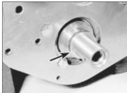
6.20 Crankshaft gear shim location
