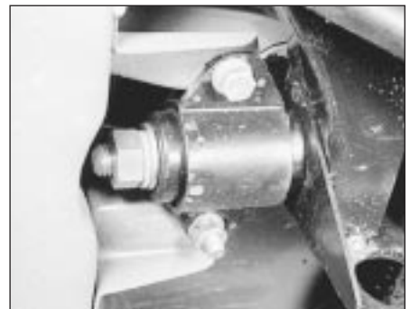
30.7 A front subframe front mounting
