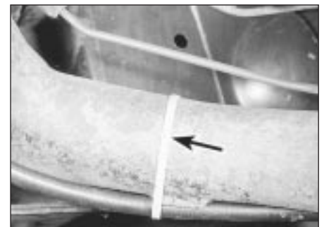
30.13 Plastic strap (arrowed) holding handbrake cable to rear radius arm
