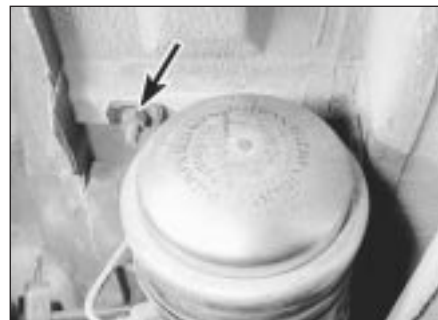
30.17a Hydragas unit outer strap bolt (arrowed)
