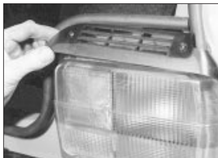
12.8 Removing the rear lamp cluster air vent
