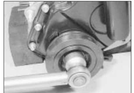
6.29 Tightening the crankshaft pulley bolt
