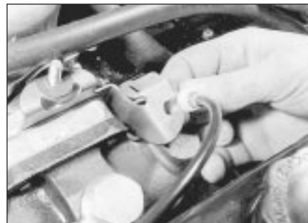
11.3 Removing the accelerator outer cable
