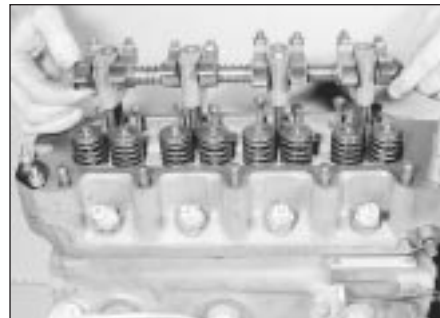
4.4 Removing the rocker shaft assembly
