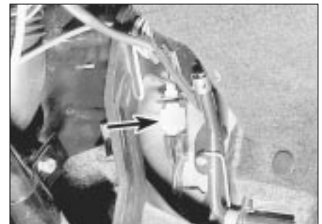
21.3 Stoplight switch location (arrowed)
