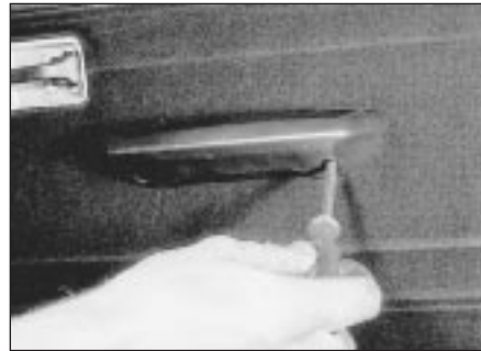
15.1b Removing the armrest
