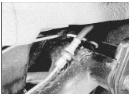
11.4 Brake pipe and hose connection on rear suspension radius arm
