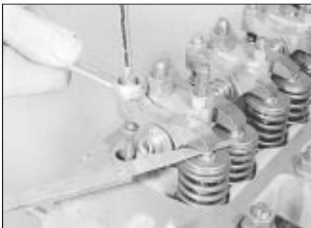
5.4 Checking the valve clearances
