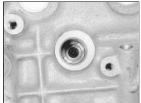
7.21c Installed position of the distributor driveshaft
