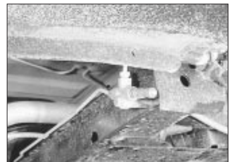
10.8 Rear Hydragas interconnecting pipe and three-way connector
