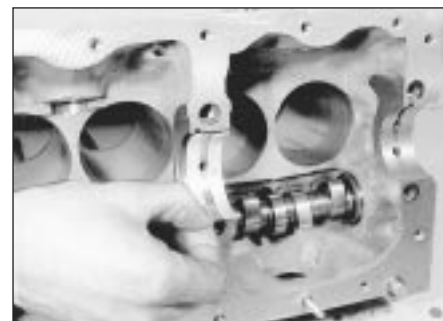
10.8 Removing a main bearing shell
