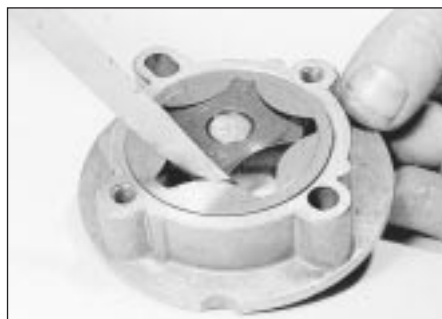
8.9d . . . rotor lobe clearance (central) . . .
