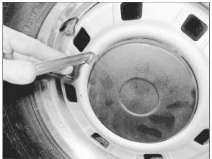
Levering off the hub cover
