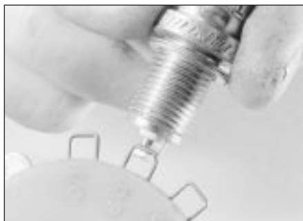
6.9b Measuring the spark plug gap with a wire gauge . . .
