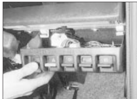
7.2b Lowering the switch panel - early models
