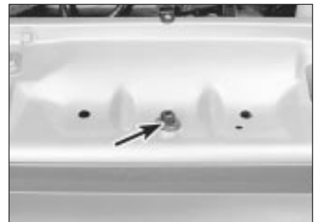
5.3c Radiator upper left-hand mounting (arrowed)
