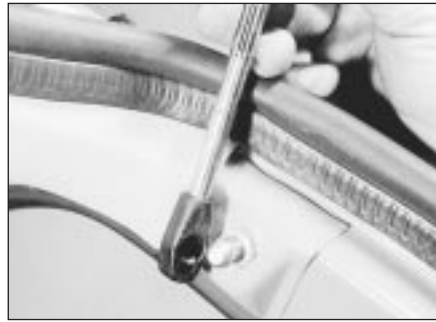
9.2b Removing the tailgate strut
