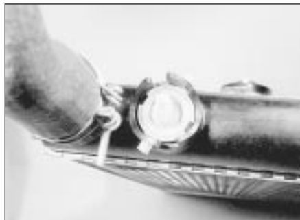
9.2 Cooling fan thermostatic switch location
