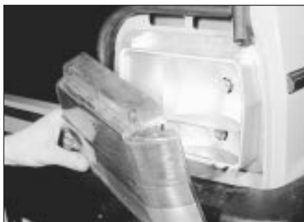
12.9b . . . and rear lamp lens
