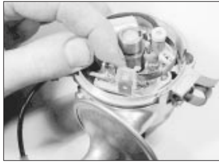
34.2 Disconnecting the contact spring from the insulator (Lucas)
