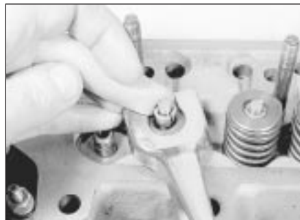
6.1 Removing the valve split collets
