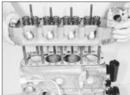
4.6 Removing the cylinder head (1275 cc engine)
