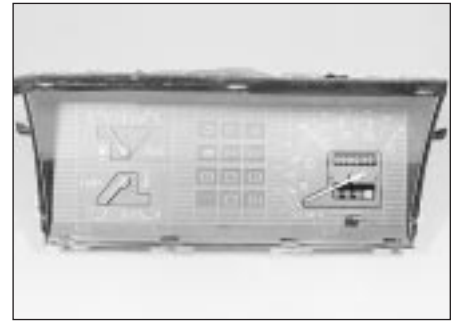
14.19c Front view of the 1985-on instrument panel
