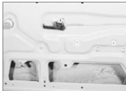
17.5a Inner door handle and rod
