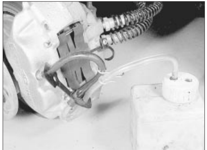
17.12d Typical brakes bleeding kit connected to front brake caliper - note that two tubes are required for lower circuit
