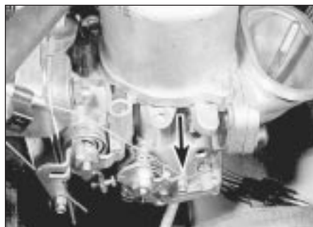
10.2 Choke cable - inner cable and clamp pin
