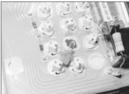
14.20c Removing the "no-charge" warning light bulb
