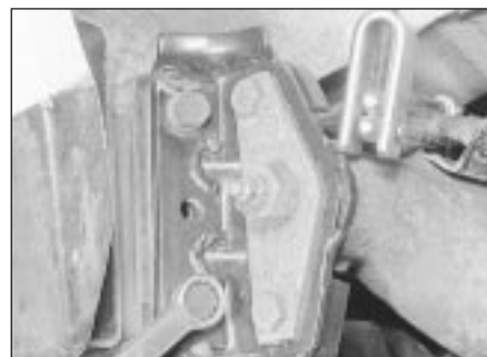
30.18 Unbolting the subframe from the front mountings
