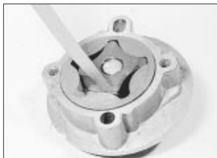
8.9e . . . and rotor lobe clearance (off centre)
