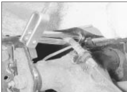
30.14 Clamp fitted to rear brake hose
