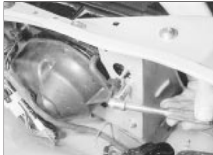
11.9 Removing the headlamp retaining nuts (1.3 HLS)
