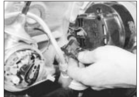
12.2 Removing the multi-plug from the alternator
