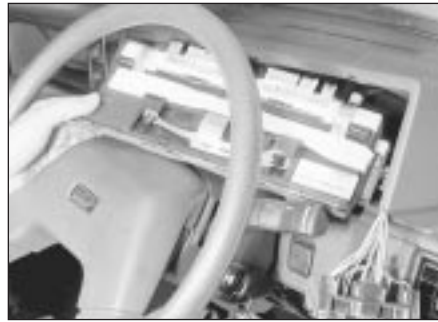
14.19b Removing the instrument panel
