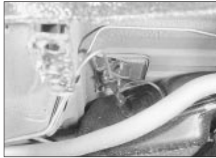
8.6 Fuel tank gauge sender unit location
