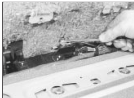
11.6b Removing the rear heater mounting bolt
