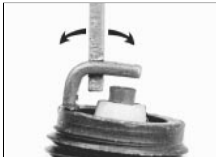
Adjusting spark plug gap
