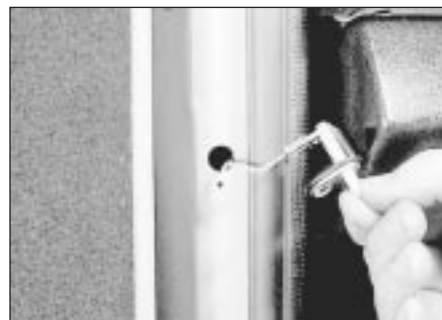
9.2 Removing the courtesy light switch
