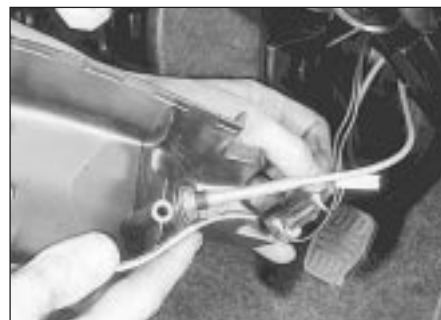
10.7 Choke warning switch and cable connection to steering column cowl
