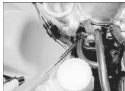
15.8 Adjusting the mixture
