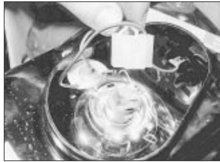
11.5 Removing the headlamp bulb socket (1.3 HLS)
