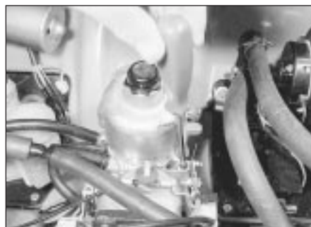
15.7 Adjusting the idling speed
