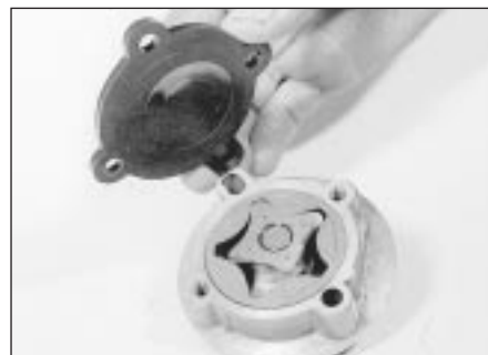
8.5 Removing the oil pump cover
