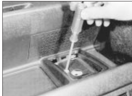
29.6b Removing the centre fascia retaining screw
