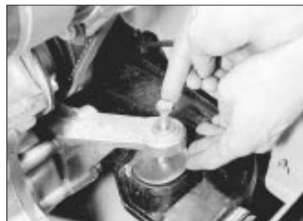
3.28c Left-hand engine mounting (from above)
