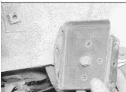
30.24b . . . and remove the rear subframe mounting
