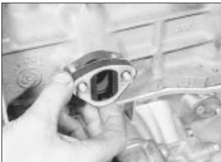
5.8 Fuel pump insulator block and gaskets
