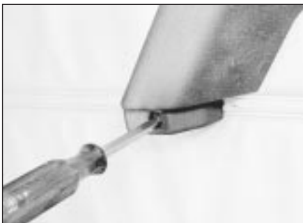
15.1f Removing the front door pull lower screw on 5-door models
