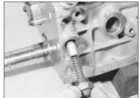
11.7 Removing the oil pressure relief valve
