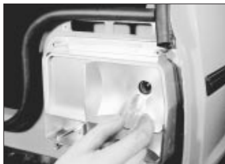
12.10 Removing a stop light bulb
