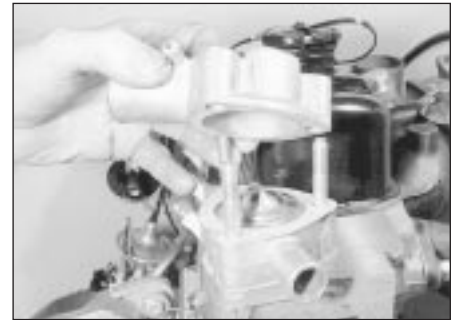
6.3 Removing the outlet elbow
