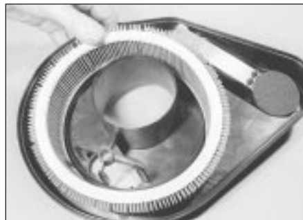
5.3 Lifting out the air cleaner element
