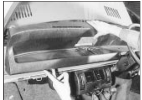
29.7 Removing the fascia
