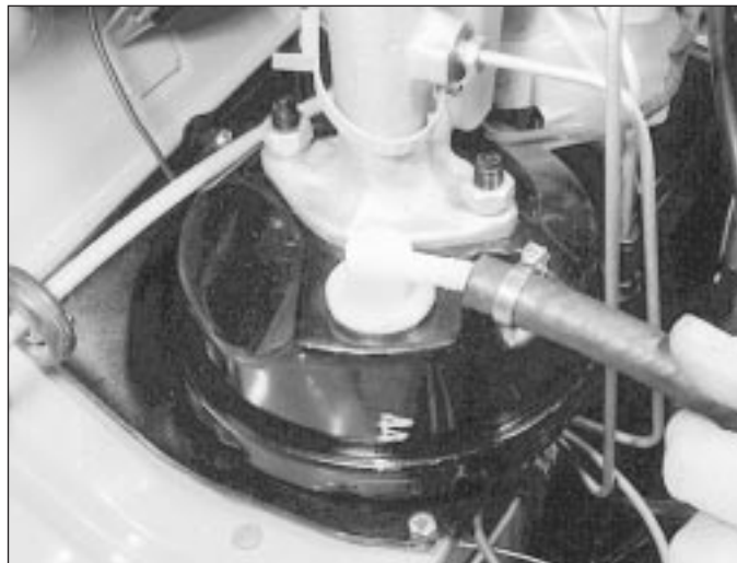
23.2 Removing the vacuum hose from the servo
