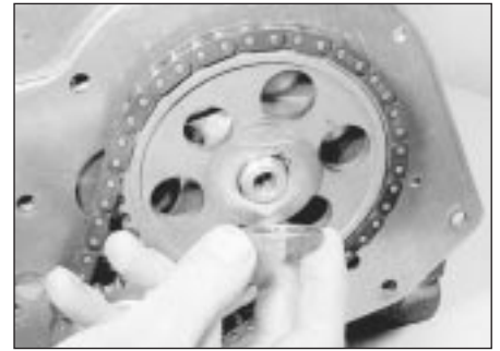
6.10 Removing the camshaft gear retaining nut
