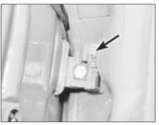
7.3 One of the hinge cotter pins (arrowed)
