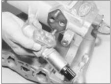
34.3 Removing the idle speed control valve
