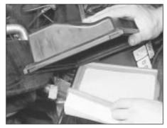
38.19 Removing the air cleaner element (fuel-injection DOHC)
