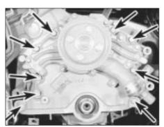
36.27 Timing cover retaining bolts (arrowed)
