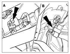
21.3 Speedometer sender unit securing bolt (arrowed)
