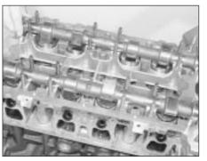
18.14b Lifting out the exhaust camshaft
