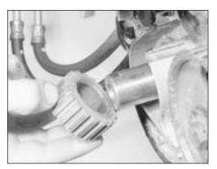
13.9 Removing the crankshaft sprocket
