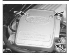
9.5a Three screws (arrowed) secure the throttle linkage cover
