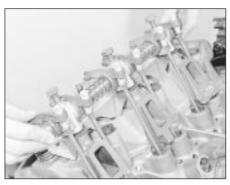
38.7b Fitting an assembled rocker shaft
