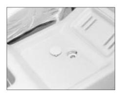
42.3 The central console securing screw (low series)
