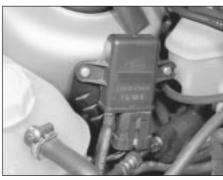
28.1 Manifold Absolute Pressure (MAP) sensor location - models equipped with a catalytic converter
