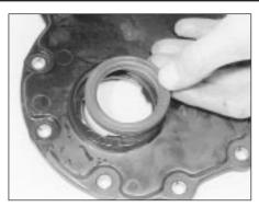
15.31 Fitting a new lower timing chain cover oil seal
