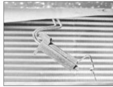
27.9 Removing the air temperature sensor
