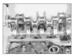
22.8a Removing the crankshaft
