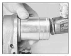
43.1 Fitting the camshaft front bearing oil seal
