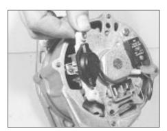
7.2 Removing the voltage regulator/brush carrier
