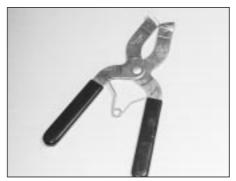
Piston ring removal/installation tool
