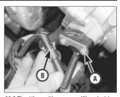
32.9 Throttle position sensor (A) and wiring plug (B)
