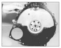
15.4 Removing the engine adaptor plate (backplate)
