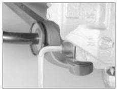
7.4 Undoing a caliper slide bolt
