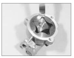
26.2a Checking the outer rotor-to-housing clearance
