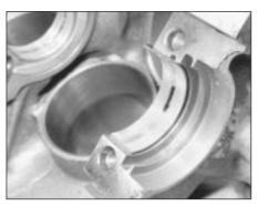
31.1 Rear main bearing shell in the crankcase
