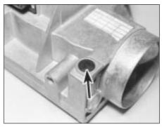
31.7 Tamperproof plug (arrowed) covering mixture adjusting screw
