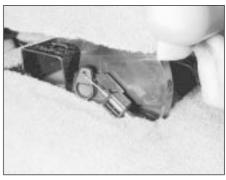
18.14 Rear heater control cable at nozzle
