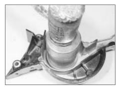
17.4 Using a socket and a hammer to seat the new seal
