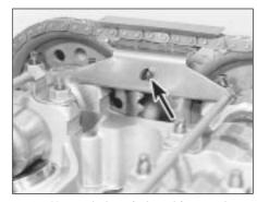
18.7 Upper timing chain guide securing lugs (arrowed)
