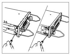
30.11 Releasing a DIN extraction tool
