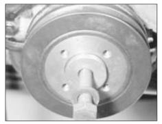
45.5b Crankshaft pulley bolt and washer
