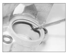
10.5 Removing the piston seal
