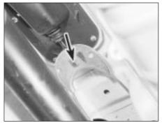
23.3 Circlip (arrowed) on equaliser yoke Note protruding screws in transmission tunnel
