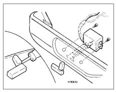
15.57 Removing the front seat adjusting switch
