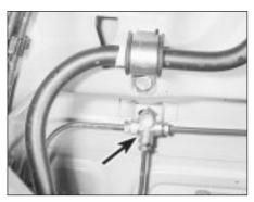
21.7 Brake pipe union T-piece (arrowed)
