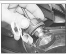
3.20 Removing the bulb and holder from the direction indicator light unit
