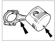
29.2 Relationship of piston crown arrow and connecting rod oil splash hole (arrowed)
