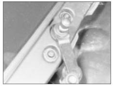
**23.2c... and two screws on the left.** *Eighth screw is midway between the spindles*
