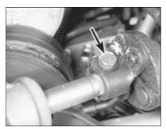
5.29 Intermediate shaft lower clamp bolt (arrowed)
