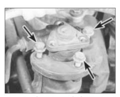
11.11 . . . for access to the front pump securing bolts (arrowed)
