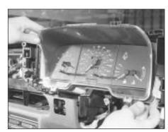
7.4b Removing the instrument cluster
