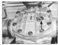
27.3 Final drive oil filler/level plug (arrowed)
