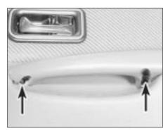
22.4a The two armrest screws (arrowed) - low level trim
