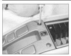
42.7 Removing a switch panel screw (high series)
