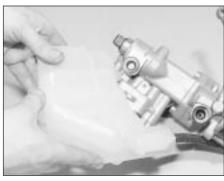
16.6 Removing the hydraulic fluid reservoir
