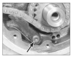
15.9 Oil pump chain tensioner securing screw (arrowed)
