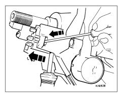
12.10 Removing the horn brush unit
