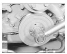
10.27a Unscrewing the vibration damper centre bolt
