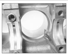
29.4b Checking a ring gap at the bottom of the cylinder
