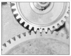
10.13 Camshaft and crankshaft gear marks in alignment (engine inverted)
