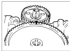
36.4 Crankshaft and camshaft gears correctly aligned
