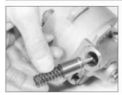
27.5b . . . and withdraw the spring and plunger
