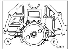
24.4 Tool used to fit the oil seal A Rear oil seal housing
