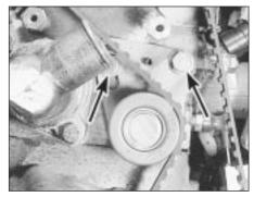
13.4 Timing belt tensioner bolts (arrowed)
