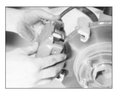
7.5 Lifting a front caliper off the disc
