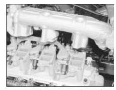
38.22 Lowering the plenum chamber into position
