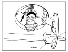
27.5 Fuel filler switch screw (arrowed)
