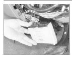
36.6 Removing the anti-theft alarm control module
