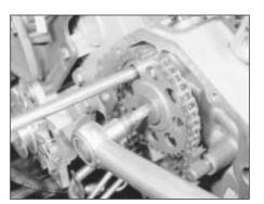
10.39 Slackening camshaft sprocket retaining bolt
