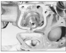
14.4 Removing the auxiliary shaft front cover
