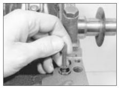
19.4 Removing the oil pump driveshaft
