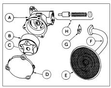
26.2d Exploded view of the oil pump
