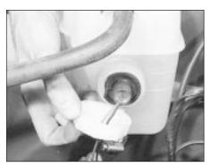
27.16 Removing the coolant level switch
