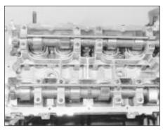
18.30b Camshaft oil spray bars correctly fitted
