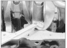
19.2 Unbolting the oil pump pick-up strainer from the block
