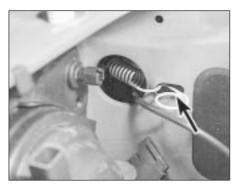
3.19 Unhook the spring (arrowed) to release the front indicator light unit
