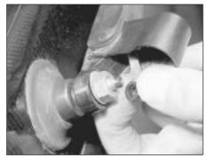
22.7 Disconnecting the rear wiper arm washer hose
