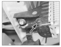
46.4a Radiator drain plug (arrowed) -**OHC** engine
