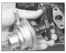
4.6a Removing the mechanical fuel pump
