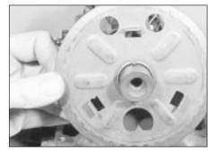
11.3 Removing the camshaft sprocket backplate
