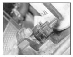
24.1 Crankshaft speed/position sensor (viewed from underneath)
