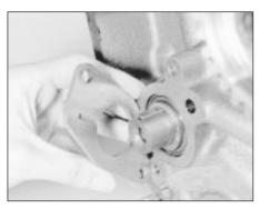
32.3b Fitting the camshaft thrust plate
