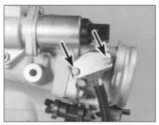
32.3 Throttle position sensor retaining bolts (arrowed)
