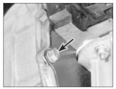
5.33 Engine adaptor plate bolt (arrowed)
