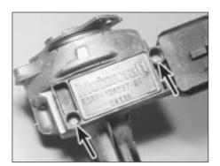
15.4 Two screws (arrowed) which secure the ignition module
