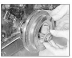
36.9 Fitting the crankshaft pulley
