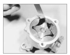
26.2b Checking the inner-to-outer rotor clearance
