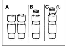
18.34 Timing chain tensioner plunger assembly
