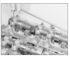
18.13 Lifting off a camshaft oil spray bar
