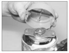
39.9 Removing a rotor arm
