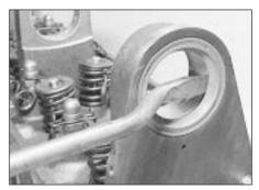
11.9 Prise out the camshaft bearing oil seal
