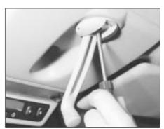
10.4 Removing the sliding roof operating handle
