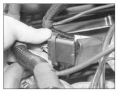
8.19a Disconnecting the distributor wiring plug
