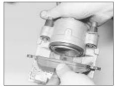
7.8a Clipping the inboard front pad into the piston
