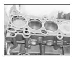
18.22 Fitting a new cylinder head gasket
