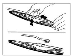
22.5 Removing a wiper blade
