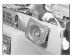
33.3 Removing the joystick fader
