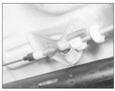
**22.3 Handbrake cable adjuster**Locknut previously backed off adjuster nut
