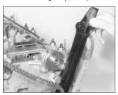
15.11c Withdrawing the lower timing chain guide
