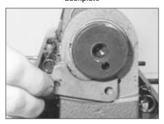
11.7 Removing the camshaft thrust plate
