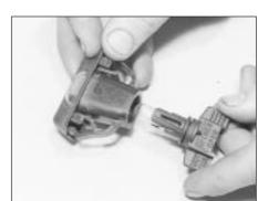
3.30 Separate the unit to gain access to the number plate light bulb
