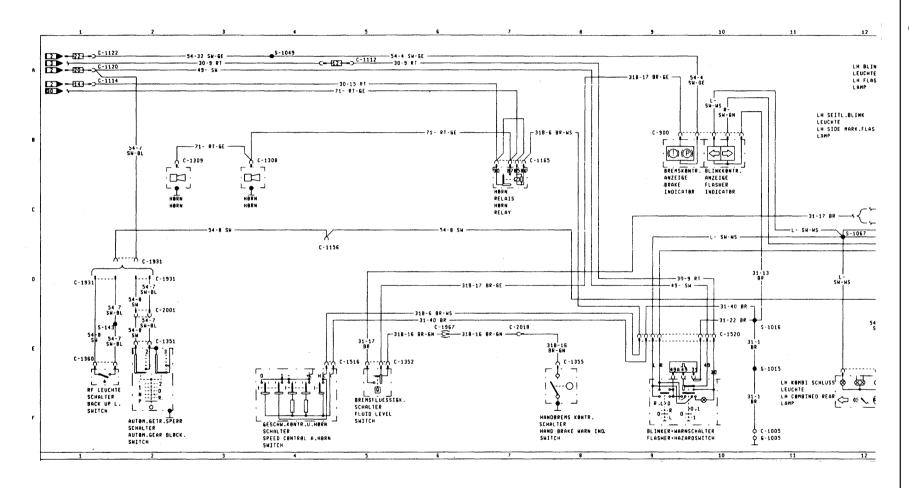
Diagram 9. Signalling and warning systems
