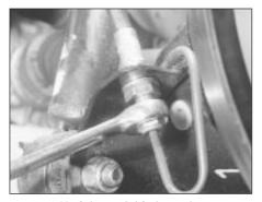
21.3 Undoing a rigid pipe union nut Flexible hose locknut is just above
