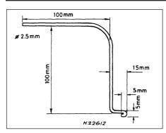
18.45 Fabricated tool used to unlatch tensioner plunger piston
