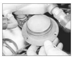
21.5 Removing the manifold heater
