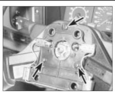
12.3 Three screws (arrowed) secure the horn switch plate
