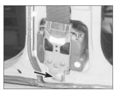
47.5 Seat belt retractor mechanism - securing the bolt arrowed
