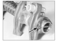
20.1 Rocker shaft roll pin (arrowed)
