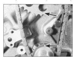
10.37 Timing sprocket alignment marks (arrowed)
