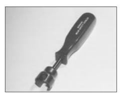
Brake shoe steady spring cup removal tool
