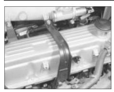
40.34 Inlet manifold-to-cylinder head bracing strut
