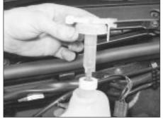
3.14 Removing the brake fluid reservoir cap
