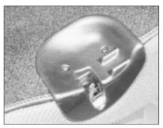
49.6 Backrest catch cover, showing securing screws
