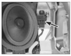
7.3 Fuel cut-off inertia switch location Estate models
