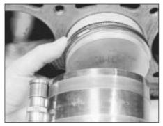
37.4a Fitting a piston ring compressor
