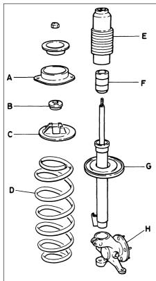
22.5 Front suspension strut components
