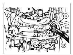
12.12 Pierburg 2V carburettor fitted to later 1.8 litre engines
