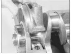
22.7 Removing the rear main bearing cap
