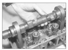
11.8 Removing the camshaft
