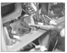
41.19 Undo the heater control panel retaining screws and free the panel from the facia
