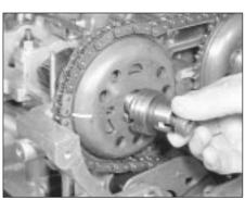
18.5 Removing the inlet camshaft sprocket bolt and the distributor rotor shaft
