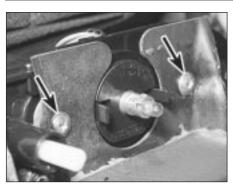
17.14 Heater control panel retaining screws (arrowed)
