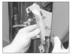
41.35b . . . then undo the screws and remove the bracket from behind the facia
