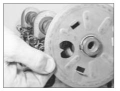
43.7 Fitting the camshaft sprocket backplate
