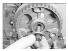
11.2 Removing the camshaft sprocket bolt and sprocket
