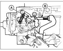
26.11 Fast idle speed adjustment - Weber 2V TLD carburettor
