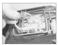
3.10 Removing the auxiliary driving light bulb
