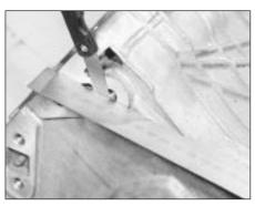
25.15 Measuring the clearance between the cylinder block and sump end faces
