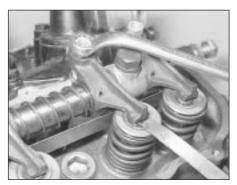
23.20 Adjusting a valve clearance - V6 engine
