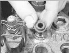
12.4 Removing a valve stem oil seal
