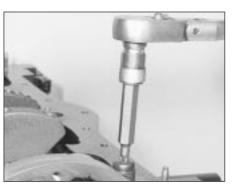
30.4 Unscrewing a sump mounting plate securing bolt
