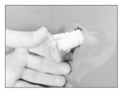
3.24a Removing a direction indicator side repeater
