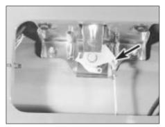
17.5 Operating rod (arrowed) connected to tailgate lock lever
