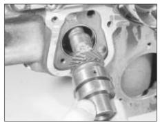
14.5b Removing the auxiliary shaft
