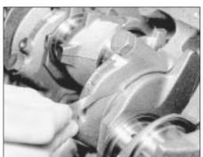
31.13 Checking crankshaft endfloat
