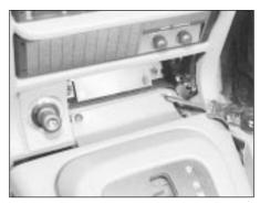
42.12 Removing a centre console front securing screw (high series)
