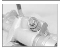
18.5 Hydraulic unit pump mounting bolt
