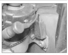
16.6 Suppresser secured by one of the coil retaining screws
