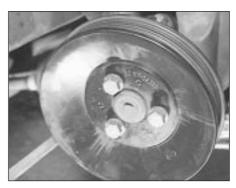
11.10 Unbolt the power steering pump pulley . . .
