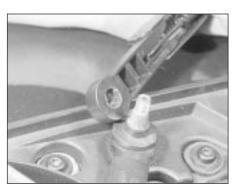
22.3b Pull the arm off the spindle
