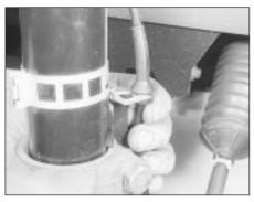
26.4 Unclipping the sensor wire from the strut
