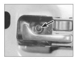
15.4 Door interior handle securing screw (arrowed)
