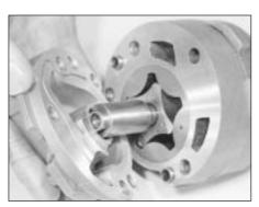
27.3 Removing the oil pump cover
