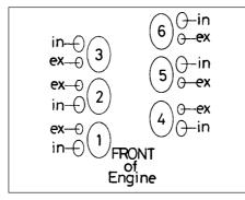
23.19 Inlet and exhaust valve location - 2.8 litre V6 engine
