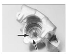
12.8 Remove the circlip (ends arrowed) to release the pushrod and key plate
