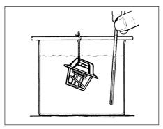
8.1 Checking the thermostat opening temperature
