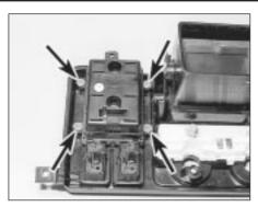
26.9 Fuel computer retaining screws (arrowed)
