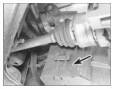
44.6 Carbon canister location (arrowed) - models from July 1990
