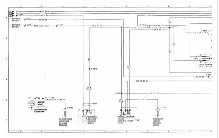
Diagram 4A. Engine management (2.0 litre carburettor)
