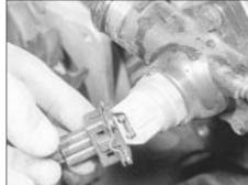
7.13 Disconnect the cooling fan switch wiring plug . . .
