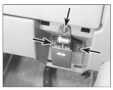
41.27a Remove the three bonnet release lever retaining screws (arrowed)
