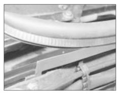
29.2 Pulling off the rubber sealing strip
