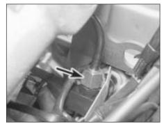
36.7 Fuel feed union (arrowed) on fuel rail
