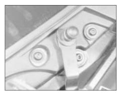
23.2b . . . three screws around the righthand spindle . . .
