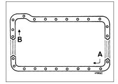
37.5 Sump bolt tightening sequence For A and B see text
