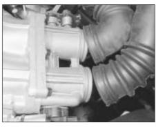
8.13 Disconnecting the air hoses from the throttle valve housing
