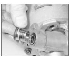
27.5a Unscrew the pressure relief valve plug and washer . . .
