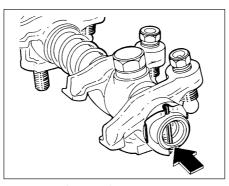
20.4 Notch (arrowed) shows position of oil holes
