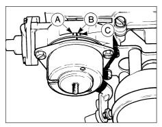
18.11 Bi-metal housing alignment marks -Weber 2V carburettor
