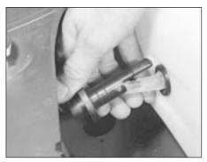
27.19 Removing the washer fluid level switch
