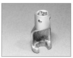
23.11 Cutaway socket spanner
