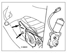
19.7 Front seat recline motor bolts (arrowed)
