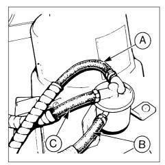
10.1a Fuel vapour separator without pressure regulator
