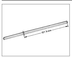
34.2 Oil pump driveshaft washer location
