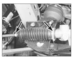
4.2 Steering rack bellows retaining clips (arrowed)
