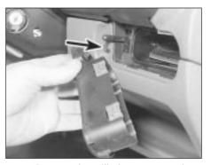
41.5 Remove the grille for access to the screw (arrowed)
