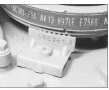
13.20 Crankshaft pulley notch set to the 12° BTDC position
