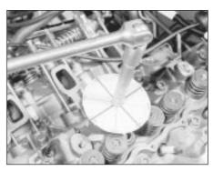
38.16 Tightening a cylinder head bolt using an angular tightening disc
