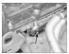
17.6 Hose bracket bolted to cylinder head (arrowed)
