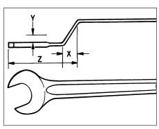
9.3a Dimensions of spanner for undoing fan clutch nut. Spanner thickness must not exceed 5 mm (0.2 in)
