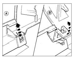
27.5 Removing the radiator grille centre section
