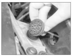
36.9 Removing the alarm system warning buzzer
