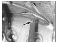
8.3 Throttle pedal showing "keyhole" cable fitting (arrowed)
