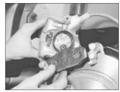
8.5 Removing a rear brake pad
