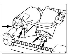
19.2 Seat adjusting motor bolts (arrowed)
