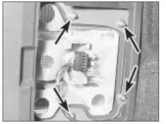
4.12 Four rear light unit securing nuts (arrowed) - there are two more out of sight
