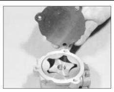
26.1 Removing the oil pump cover
