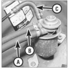
10.1b Fuel vapour separator and pressure regulator
