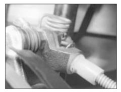
23.4 Handbrake cable outer attached to caliper bracket
