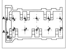
18.17 Cylinder head bolt tightening sequence
