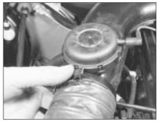
38.4 Disconnecting the air cleaner cold air inlet trunking (carburettor model)
