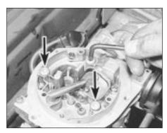
12.8 Undoing a carburettor securing screw.
