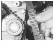
45.12 Twisting the timing belt to assess its tension
