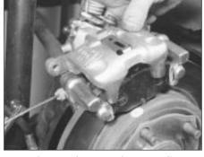
11.5b . . . and remove the rear caliper
