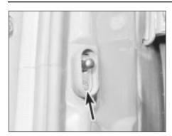
15.24 Door pillar switch securing screws (arrowed)
