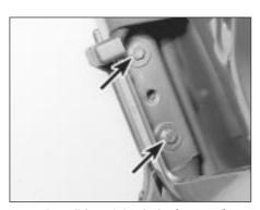
9.3 Boot lid retaining bolts (arrowed) -Saloon models
