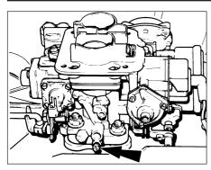
16.12 Idle mixture adjustment screw (arrowed) - Weber 2V carburettor
