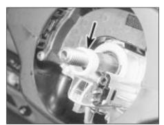
5.6 Spacer ring (arrowed) fits below steering wheel
