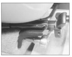
44.1 Removing a front seat retaining bolt
