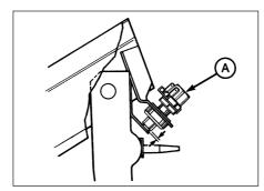
15.44 Fitting the stop-light switch (A) Plunger protrusion (between arrows) must be at least 2 mm (0.08 in)
