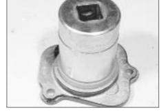
41.3b Fitting a new oil seal in the auxiliary shaft cover
