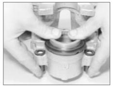
10.9 Pressing the piston into the bore
