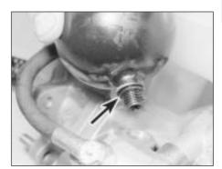
17.4 Removing the accumulator Note O-ring (arrowed)
