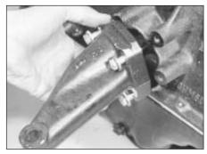
9.1b Removing an engine bearer arm
