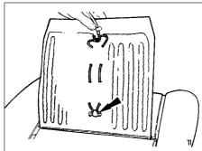
13.3 Seat heating element Thermostat (arrowed) must face the foam
