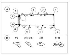
44.11 Rocker cover bolts (A) and reinforcing plates (B)
