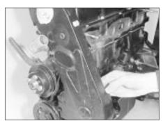
10.2 Removing the timing cover
