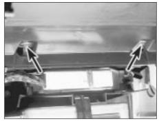
41.34c Facia mounting nuts (arrowed) situated in glovebox aperture
