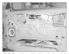
22.8b Front door with rubber sheet peeled back
