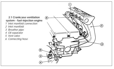
manifold. Piston blow-by gases are drawn through the oil separator and the vent valve to the inlet manifold. The blow-by gases are then drawn into the engine together with the fuel/air mixture. Refer to Chapter 1 for maintenance of the system.
