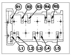
18.30a Camshaft bearing cap tightening sequence
