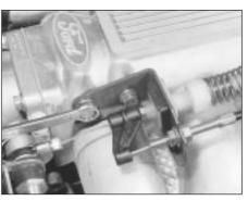
40.36 Unbolting the throttle cable bracket
