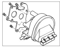
19.4 Carburettor stepper motor and mounting bracket
