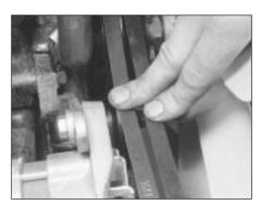
21.3 Checking drivebelt tension
