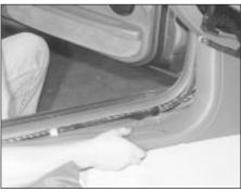
41.30 Removing the passenger side lower kick panel
