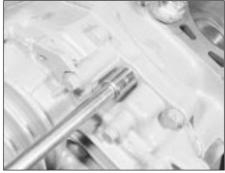
10.36 Removing a timing cover retaining bolt
