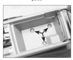
42.20a Centre console rear retaining screws (arrowed)
