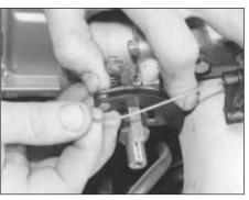
9.6 Removing a throttle cable inner - barrel and slot type
