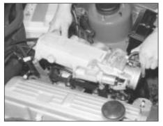
40.40a Removing the inlet manifold
