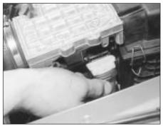
8.14a Front airflow sensor wiring plug
