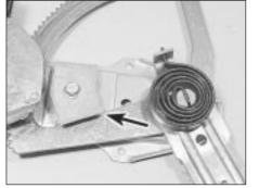
18.2a Make sure that the lever is against the stop (arrowed) . . .
