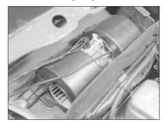
29.5 Blower motor showing wiring connections
