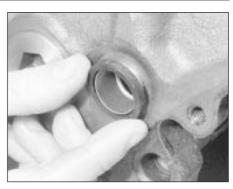
32.4 Timing cover dowel and seal
