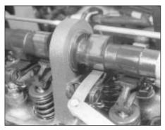
23.7 Measuring a valve clearance - SOHC engine
