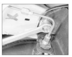
10.35 Unscrewing crossmember side bracket mounting bolts
