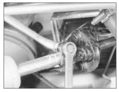
10.32 Steering shaft coupling pinch bolt
