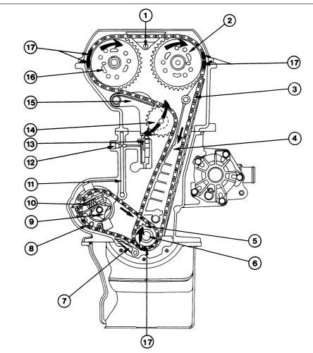
15.2 Timing chain, oil pump drive chain and associated components
