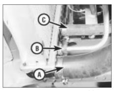
5.2b Radiator bottom hose (A) Also shown are automatic transmission fluid cooler lower union (B) and hose to expansion
