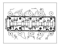
44.7 Cylinder head bolt tightening sequence
