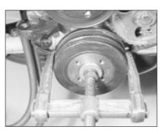
13.7 Using a puller to remove the crankshaft pulley
