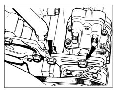
22.4 Air conditioning compressor adjuster strap bolts (arrowed)
