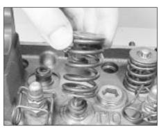
12.2b Removing a valve spring and cap
