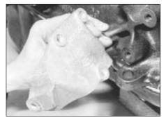
9.1c Removing the alternator bracket
