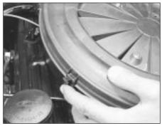
38.2 Releasing an air cleaner cover clip (carburettor model)
