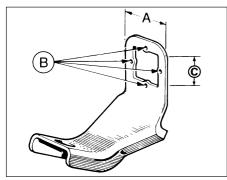
9.7 Tool for releasing accelerator cable
