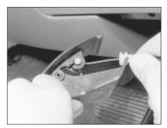
41.27b Withdraw the bonnet release lever and disconnect it from the operating cable
