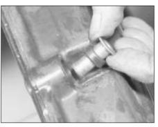
18.54 Fitting a camshaft cover reinforcing sleeve and sealing ring
