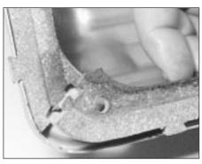
44.10 Dovetail section of rocker cover gasket
