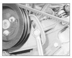
36.39b Power steering pump drivebelt tensioner bolt
