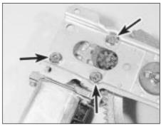
18.2b . . . then remove the three bolts (arrowed) which secure the motor
