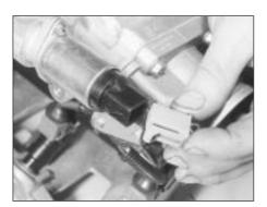
34.2 Disconnecting the idle speed control valve
