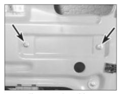
24.5a The two regulator slide screws (arrowed)
