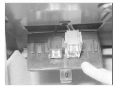
16.3 Auxiliary fuse box in the glovebox
