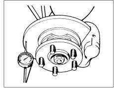
4.3 Measuring brake disc run-out
