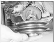
45.5a Refitting the crankshaft pulley
