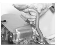
29.2 Removing the oil pick-up pipe
