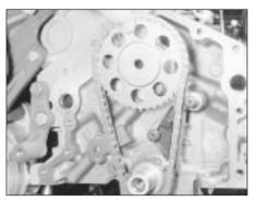
36.18 Fitting timing chain and sprockets
