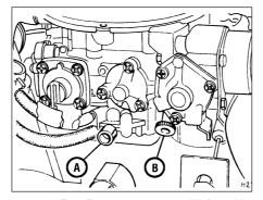
16.13 Idle adjustment screws- Weber 2V TLD carburettor
