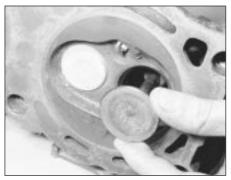
23.2c Removing an inlet valve
