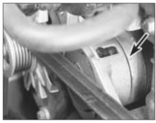
21.14b Water pump/alternator drivebelt tensioner wear indicator location (arrowed)
