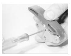
36.20 Releasing timing chain tensioner pawl
