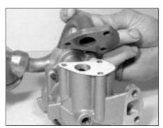
27.16a Removing the pick-up from the oil pump
