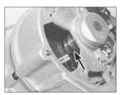
7.4 Clean the slip rings (arrowed)
