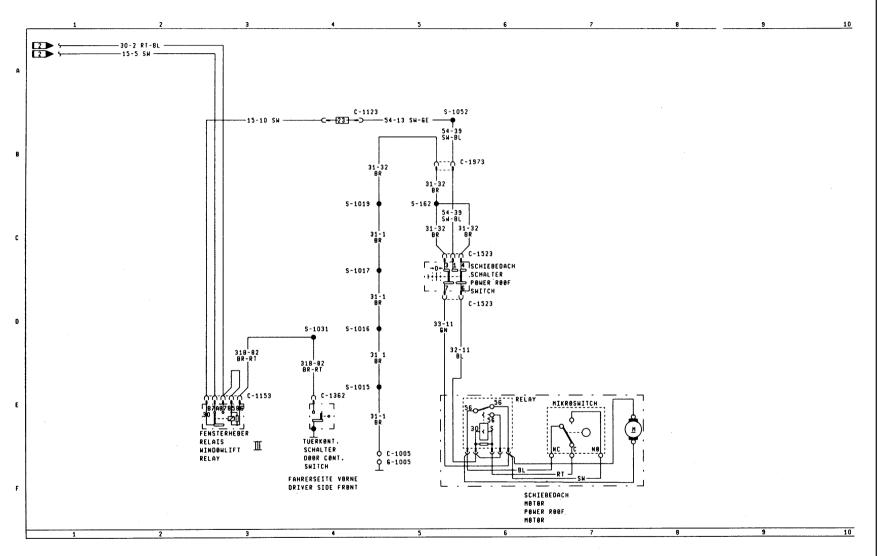
Diagram 16. Power-operated sliding roof
