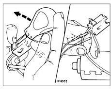
19.3 Removing the spade connectors from the multi-plug
