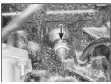
9.1a Engine oil pressure switch (arrowed)
