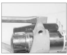
22.2 Spreading the stub axle carrier clamp
