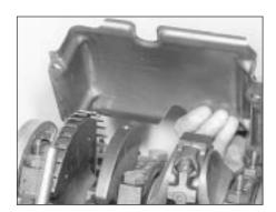
29.3 Withdrawing the oil baffle
