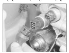
15.3d Disconnecting the pressure switch multi-plug
