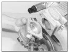
40.42b Removing the throttle body housing
