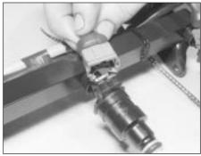
36.11 Disconnecting a fuel injector multiplug
