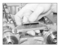
18.30c Fitting the timing chain guide plate
