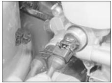
15.3c Disconnecting the main valve plug
