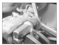
8.3 Undoing a rear caliper front slide bolt
