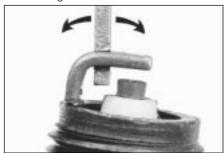
Adjusting spark plug gap
