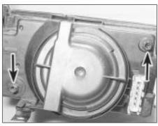
5.5 Headlight beam adjustment screws (arrowed)
