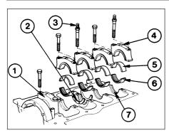
30.11 Crankshaft main bearings and associated components
