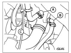
11.19 Water pump housing hose connections
