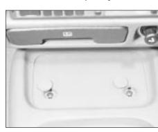
42.1 The two front screws which secure the low series console
