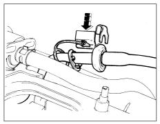
36.55b Fitting fuel rail connector clip
