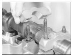
18.14a Lifting off a camshaft bearing cap
