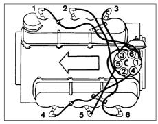
23.22 Cylinder numbering and HT lead connections - V6 engine
