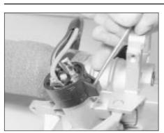
**14.3 Ignition/starter switch removal**Depress the retaining tabs to lift off the switch
