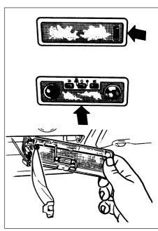
6.2 Courtesy light bulb renewal Prise at points arrowed
