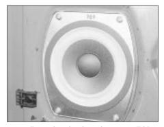
31.4 Front door loudspeaker - note TOP marking
