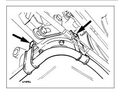
10.9 Heater connecting pipe clip bolts (arrowed)
