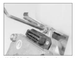
16.4 Undoing the reservoir securing screw
