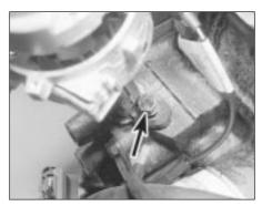
13.6 Distributor clamp bolt (arrowed)
