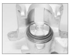
12.21 Dust boot fitted to caliper and piston
