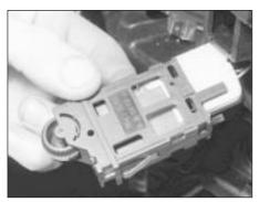
15.10 Removing the instrument illumination dimmer switch
