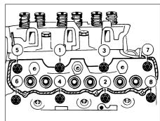
38.5 Cylinder head bolt tightening sequence
