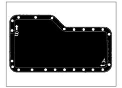
39.4 Sump bolt tightening sequence For A and B see text
