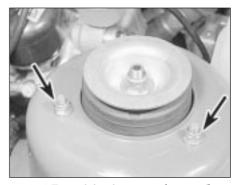
21.8 Two of the three nuts (arrowed) securing the suspension strut to the turret
