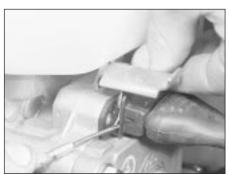
15.3a Disconnect the valve block multiplug. Lift the clip and pull off the plug
