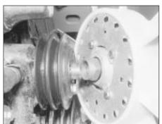
9.3c Removing the fan and clutch
