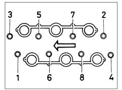
40.79 Inlet manifold bolt tightening sequence
