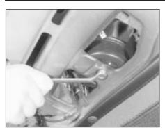
31.8 Removing a rear speaker retaining bolt
