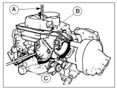
18.7 Adjusting the vacuum pull-down - Weber 2V carburettor
