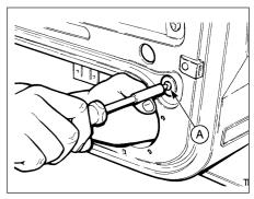
23.4 One of the front door window channel screws (A)
