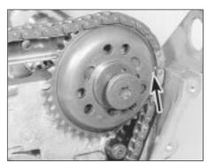
18.38 Spacer and sprocket securing bolt fitted to end of camshaft, with camshaft in TDC position (timing marks arrowed)
