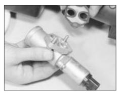
34.12 Withdrawing the idle speed control valve
