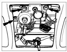
20.2 Sliding roof motor retaining bolts (arrowed)
