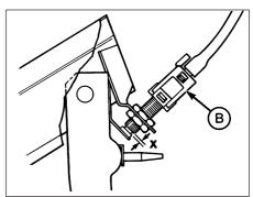
28.8 Vacuum dump valve/switch (B) X = 1.5 mm (0.06 in) minimum
