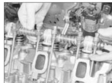
8.29 Removing rocker shaft and pedestal
