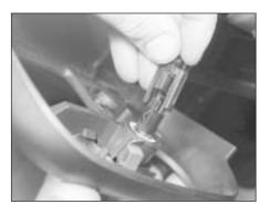
6.22 Removing the switch symbol illumination light
