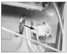
14.2 Unhook the operating rod (arrowed) from the lock barrel lever
