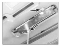
32.6 Radio aerial pre-amplifier retaining screws (arrowed)
