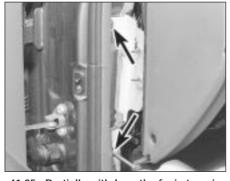
41.35a Partially withdraw the facia to gain access to left-hand support bracket retaining screws (arrowed) . . .
