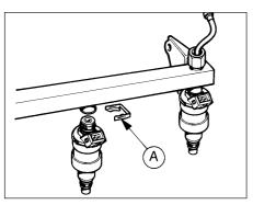
36.12 Removing a fuel injector from the rail A Retaining clip
