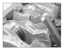
22.6 Checking crankshaft endfloat
