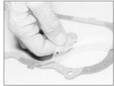
38.21 Peeling off rocker cover gasket protective shield
