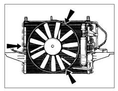
22.10 Condenser fan securing bolts (arrowed)
