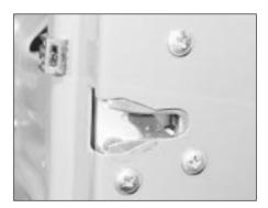
15.6 Door latch securing screws
