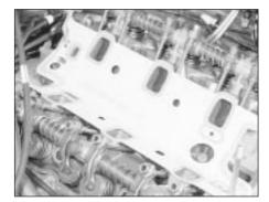
38.18a Inlet manifold gasket correctly located
