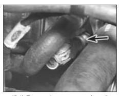
15.1b Temperature gauge sender unit location (arrowed)
