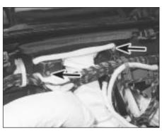
19.19 Release the facia wiring loom from the bulkhead to gain access to the demister nozzle retaining nut and screw (arrowed)
