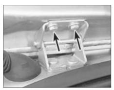
8.14 Tailgate hinge retaining bolts (arrowed) - Estate models
