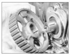
13.11 Removing the auxiliary shaft sprocket
