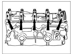
27.3b Main bearing cap marks (arrowed) denote oversize parent bore
