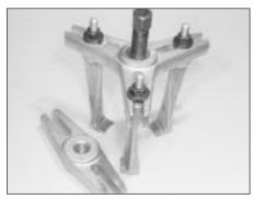
Three-legged hub and bearing puller
