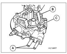
21.4 Float and needle valve locations in carburettor top cover - Weber 2V TLD carburettor
