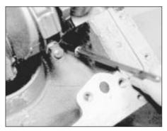
34.4 Fitting the oil pump driveshaft
