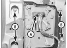
4.17 Rear light cluster wiring connector (A) and retaining nuts (B)
