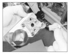
41.22 Withdraw the light switch surround and disconnect the wiring connector
