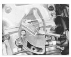
9.5b Throttle linkage with cover removed
