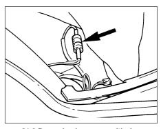
26.9 Rear wheel sensor multi-plug (arrowed)
