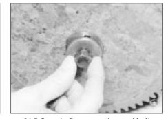
36.5 Camshaft gear washer and bolt
