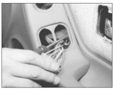
22.4b Access to the screw is through the window switch aperture
