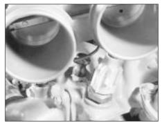
8.18a Coolant temperature sensor location
