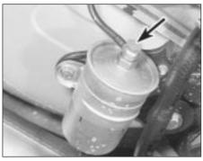
41.4 Fuel filter outlet union (arrowed) - OHC engine
