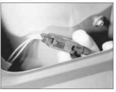
9.2 On Saloon models remove the trim panel to gain access to the lock and warning switch wiring connectors
