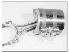
33.6a Piston with ring compressor fitted
