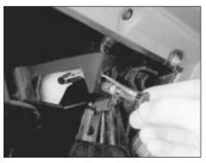
41.29c Withdraw the glovebox illumination light and disconnect the wiring connector
