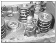
42.3 Cam follower ball-pins and spring clips fitted
