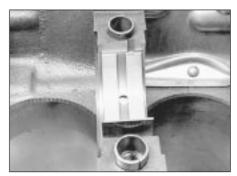
22.9 Removing the centre main bearing shell
