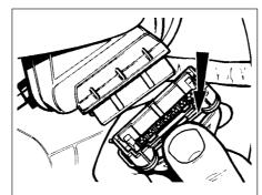
16.3 Depress locking clip (arrowed) when disconnecting stepper motor multi-plug
