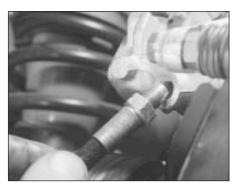
21.5 Disconnecting the hose from the caliper
