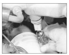
20.4 Coolant temperature sensor multi-plug
