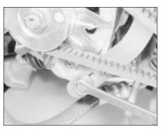
36.39a Alternator drivebelt tensioner strap bolt
