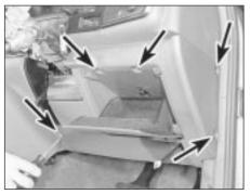
41.28 Undo the five right-hand lower facia panel retaining screws (arrowed)
