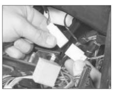
41.32 Disconnect the alarm warning LED wiring connector
