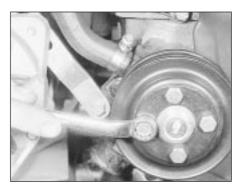
11.4 Undoing a water pump pulley bolt
