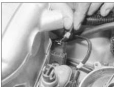
36.47 Disconnecting a fuel injector wiring connector
