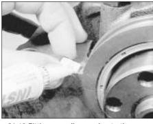
36.19 Fitting a sealing wedge to the rear main bearing cap
