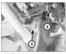
14.4 Pushrod spring clip (A) and brake pedal shaft clip (B)
