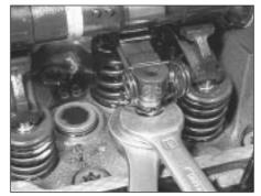
23.9 Adjusting a valve clearance - SOHC engine
