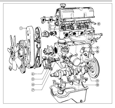
The cylinder head is of crossflow design with the inlet manifold mounted on the left-hand side and the exhaust manifold mounted on the right-hand side.
