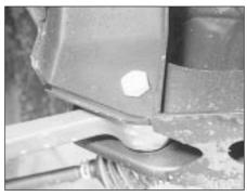
15.3 Front suspension lower arm pivot bolt
