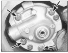
26.3 Oil pump securing bolts (arrowed)
