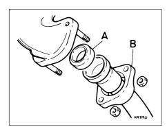
42.11 Exhaust pipe flanged joint
