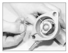
7.5a Remove the retaining clip . . .
