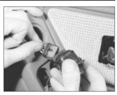
15.15 Removing a mirror control switch
