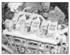
38.18b Fitting inlet manifold complete with fuel rail and injectors
