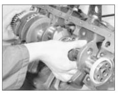
31.6 Placing the crankshaft in position
