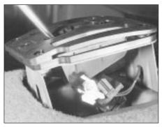
6.37 Automatic transmission selector with bulbholder displaced
