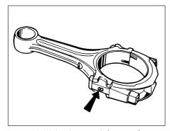
29.1 Weight class mark (arrowed) on connecting rod
