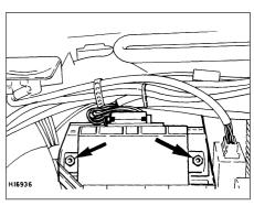
27.22 Auxiliary warning system control assembly - retaining nuts arrowed
