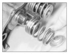
23.2b Removing the spring retainer and spring
