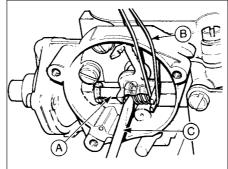
18.5 Choke vacuum pull-down check -Weber 2V carburettor
