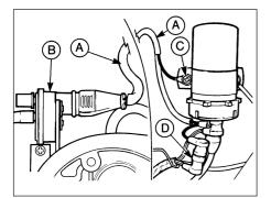
12.13 Wiring connections to Pierburg 2V carburettor fitted to later 1.8 litre engines
