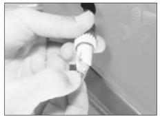
3.24b Fitting a new side repeater bulb
