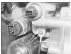
15.4 Earth strap (arrowed) bolted to hydraulic unit
