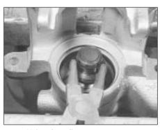
12.6 Using the adjuster nut to compress the caliper spring
