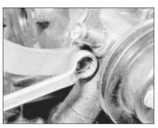
11.7a This water pump bolt also secures the alternator strap
