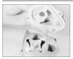
27.16b Removing the oil pump cover
