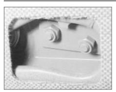
8.6 Tailgate hinge nuts are accessible through headlining
