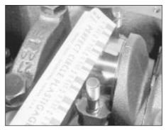
27.5 Checking the width of the Plastigage filament against the scale on the packet
