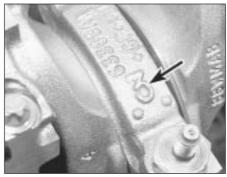
30.5 Main bearing cap identification mark (arrowed)
