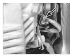
27.4 Vehicle speed sensor wiring plug (arrowed)
