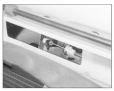
11.5 Bonnet release cable connected to catch
