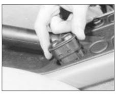
15.31 Removing a window operating switch
