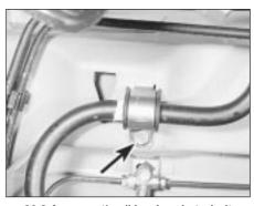
30.3 A rear anti-roll bar bracket - bolt arrowed
