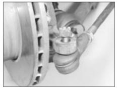
13.3 Track rod end balljoint nut unscrewed
