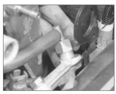
36.31 Disconnecting the fuel feed hose from the fuel rail
