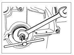
18.2 Using an oil seal removal tool to extract the crankshaft rear oil seal
