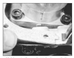
39.2 Locate the gasket tabs beneath the sealing strips
