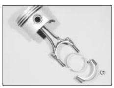
21.4 Piston, connecting rod, cap and bearing shells
