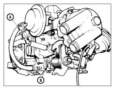
15.3 Idle adjustment screws - Pierburg 2V carburettor
