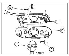
17.15 Exploded view of the heater control panel
