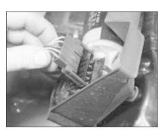
23.3 Disconnecting the wiper motor multiplug
