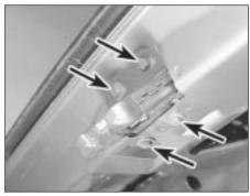
18.4 Boot lid lock retaining bolts (arrowed) - Saloon models
