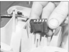
4.13 Disconnecting the multi-plug from the rear light unit
