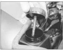
35.2 Removing the power steering fluid dipstick
