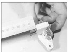
7.3 Measuring brush protrusion
