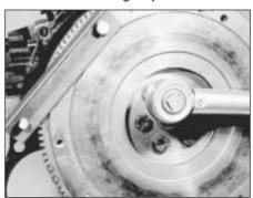
40.4b Tightening a flywheel bolt
