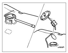
6.3 Removing the fuel gauge sender unit
