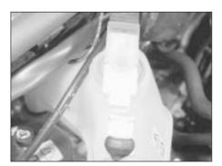
15.3b Disconnecting a fluid level sensor plug
