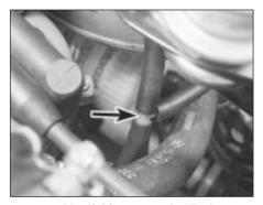
40.29 Manifold vacuum pipe T-piece (arrowed)
