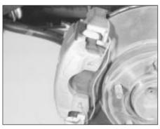
7.2 Spring clip fitted to outboard face of front caliper
