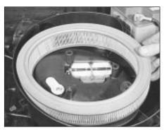
38.3 Removing the air cleaner element (carburettor model)
