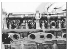
11.4 Removing the camshaft oil supply
