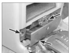
41.24 Ashtray retaining screw locations (arrowed)
