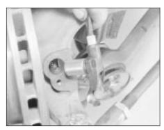
26.3 Removing a front sensor
