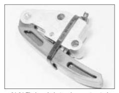
36.21 Timing chain tensioner retracted using a cable-tie
