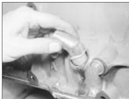
13.4 Withdraw the crankcase breather tube elbow
