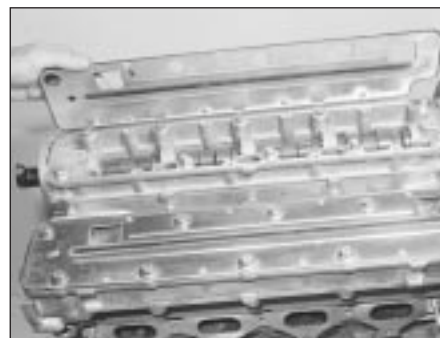
4.5 Remove the baffle plates over the camshafts
