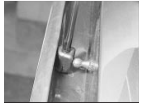
15.3 Release the strut lower end from its stud
