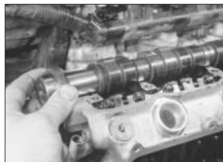
15.12 Carefully lift out the camshafts
