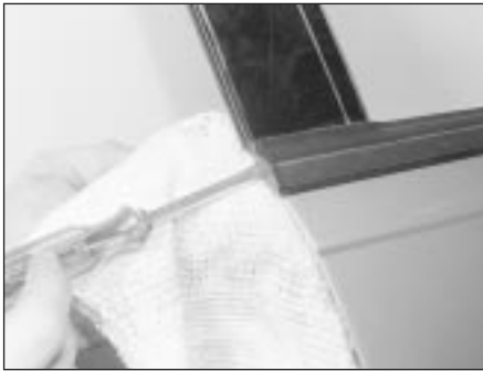
27.2a Prise up the door panel waist seal . . .
