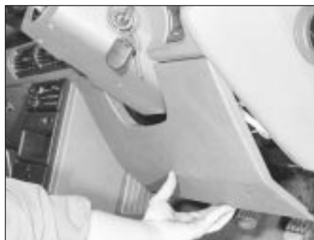
21.3a Remove the upper trim panel . . .
