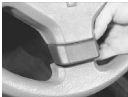
18.3a Prise off the steering wheel pad . . .
