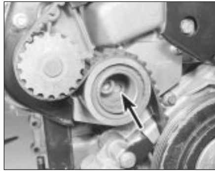
7.23 Tensioner hexagonal adjusting hole (arrowed)
