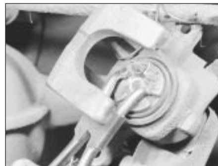
7.11 Using angled circlip pliers to screw the piston back into the caliper. Note the position of the cut-outs
