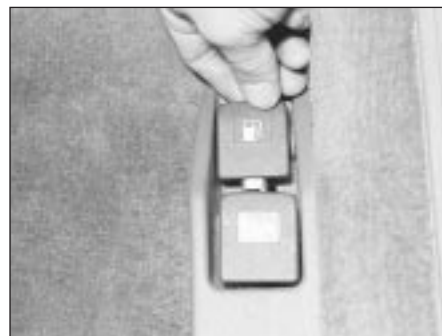
11.1 Withdraw the boot lid/tailgate and fuel filler flap release lever knobs
