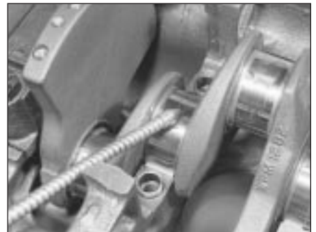
21.14 Thoroughly lubricate the crankshaft journals
