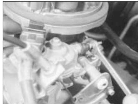
11.15a Slacken the base idle speed adjusting screw locknut . . .
