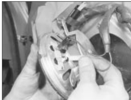
21.11 Withdraw the speaker and disconnect the wiring
