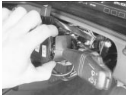
4.5a Depress the top and bottom switch retainers . . .
