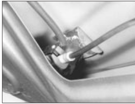
17.9 Private lock component attachments on later models
