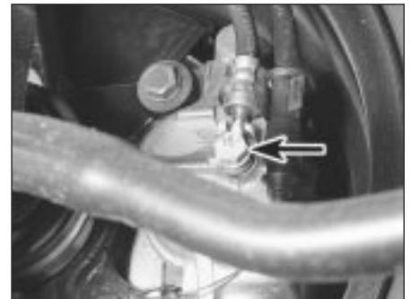
15.10 Front brake hose-to-caliper banjo union bolt (arrowed)
