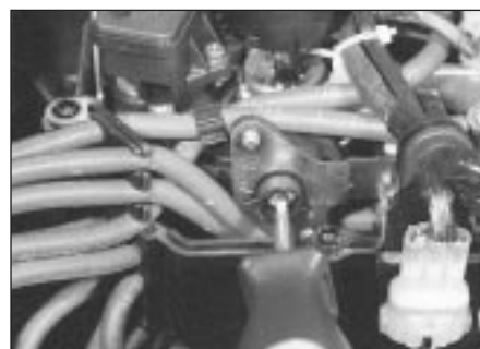
10.27 Turn the ignition timing adjuster to advance or retard the timing
