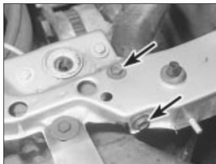
5.6 Centre platform retaining bolts - right-hand side (arrowed)
