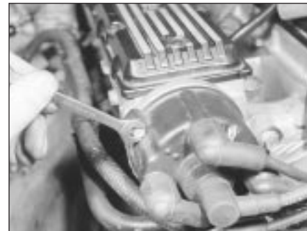
5.1 Undo the two retaining screws and lift off the distributor cap
