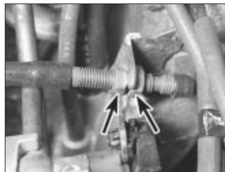
3.2 Slacken the outer cable locknuts, then withdraw the outer cable from the support bracket
