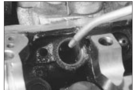
15.31a Fill the tappet bores with oil before fitting the tappets
