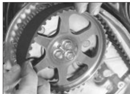
12.5 Ease the belt off the camshaft sprockets
