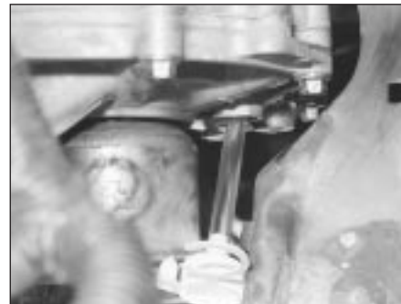
20.2 Topping up the manual transmission oil
