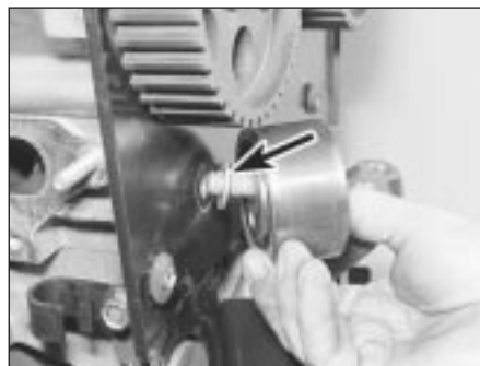
10.2 Remove the timing belt idler pulley and recover the spacer (arrowed)
