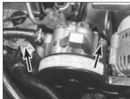
26.27a Undo the three nuts/bolts (arrowed) securing the pulley covers to the top of the engine ...
