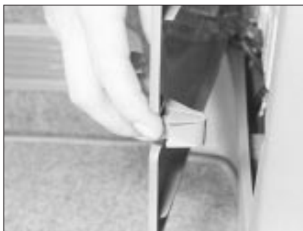
5.25 Press the retainer on the access panel and remove the panel
