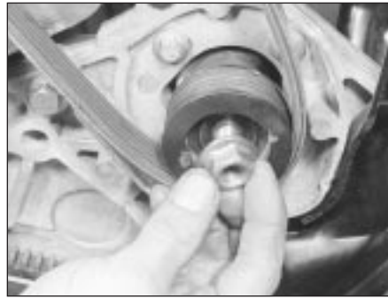
26.8 Unscrew the pump pulley retaining nut
