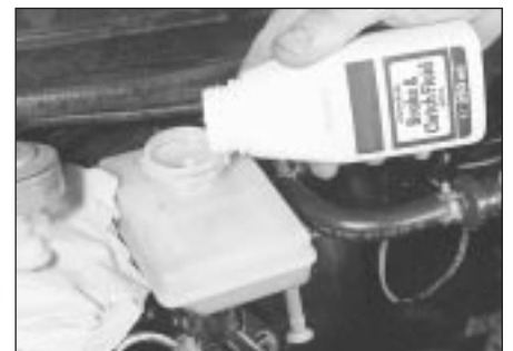
3.22 Topping up the brake master cylinder reservoir
