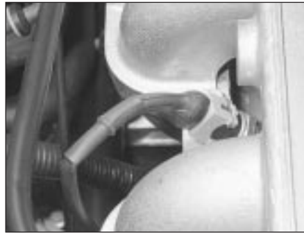
12.30 Fuel temperature switch wiring multiplug
