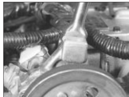
16.33b ... then engage the end of a socket bar in the lug on top of the pump to adjust the belt
