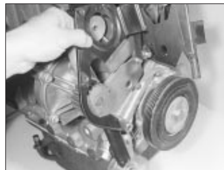
9.3 Removing the lower backplate from the engine (early metal version shown, later plastic version similar)
