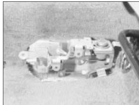
11.3b . . . for access to the release control assembly
