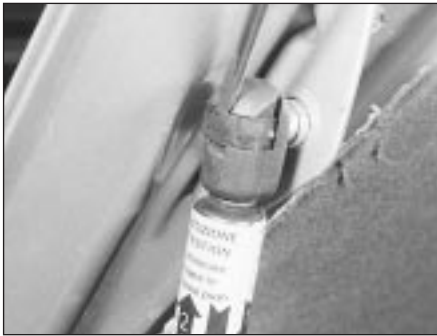
6.7 Prise out the support strut retaining clips
