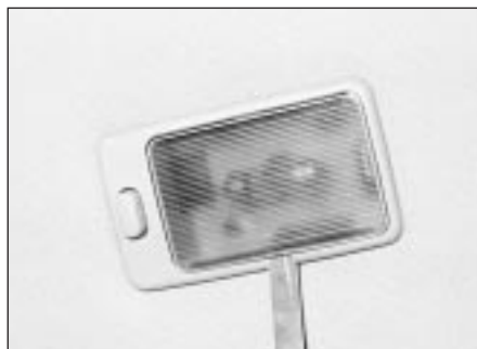
6.1 Prise off the courtesy light lens
