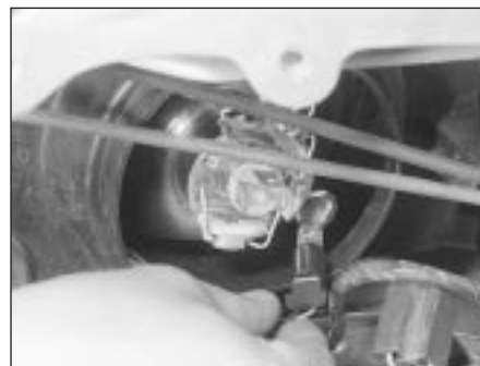
5.6 Withdraw the sidelight bulbholder from the headlight unit
