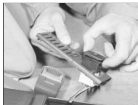
4.21 Centre console switch removal
