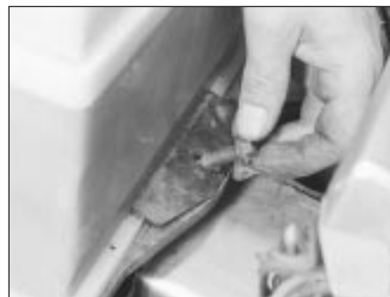
2.4 Removing the battery clamp retaining bolt
