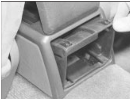
47.6 Remove the rear ashtray and insert . . .
