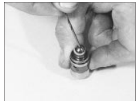
15.24a Using a small drill bit that will just fit through the hole in the end of the tappet . . .
