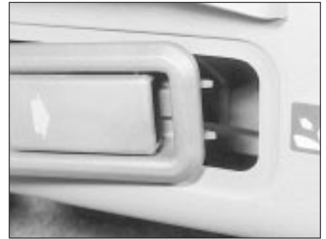
44.2b . . . and disengage the locating lugs
