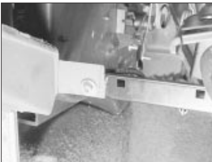
48.13 Undo the cross-brace screws
