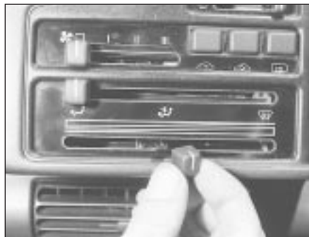
48.4 Pull off the heater knobs
