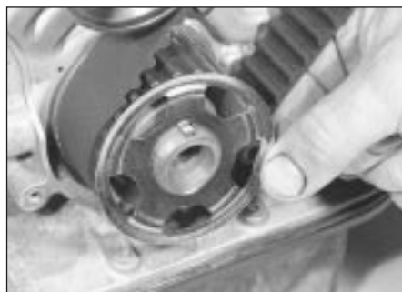
12.3 Remove the belt guide from the crankshaft sprocket
