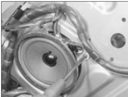
21.10 Undo the main door speaker retaining screws
