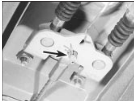
19.4 Extract the cable retaining spring clip and clevis pin (arrowed)
