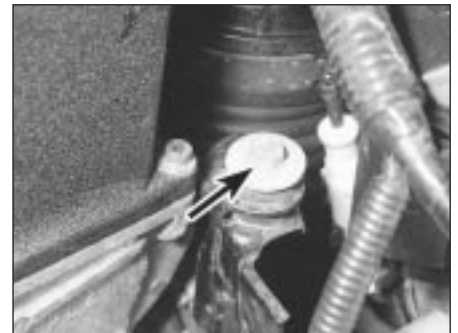
2.10a Undo the rear bolt arrowed . . .
