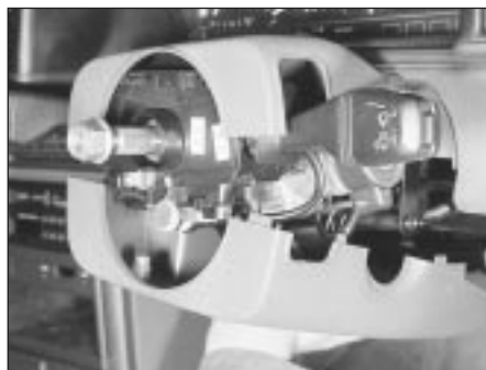
4.3c . . . then lift off the steering column shrouds
