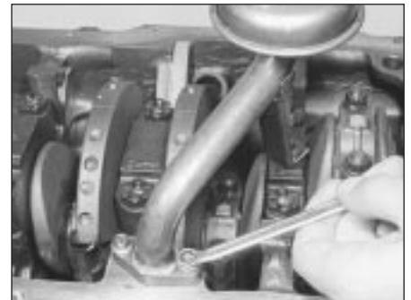
13.10 Undo the two pick-up pipe-to-crankcase bolts
