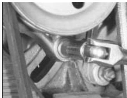
16.33a Slacken the V6 engine power steering pump adjusting nut ...
