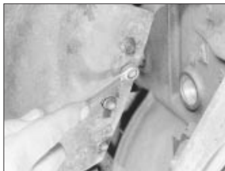
6.8a Undo the bolts securing the two halves of the manifold stove . . .
