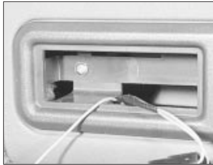
44.2a Undo the release lever surround retaining screw . . .
