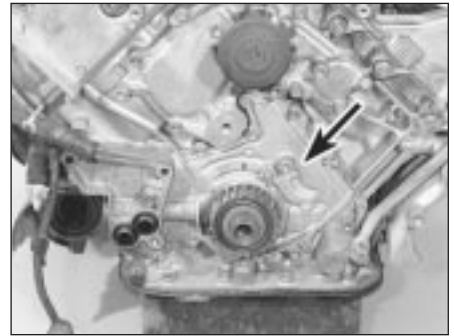
19.11 Oil pump housing location on the front of the engine
