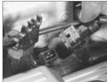
12.54 Disconnect the injector wiring multiplugs
