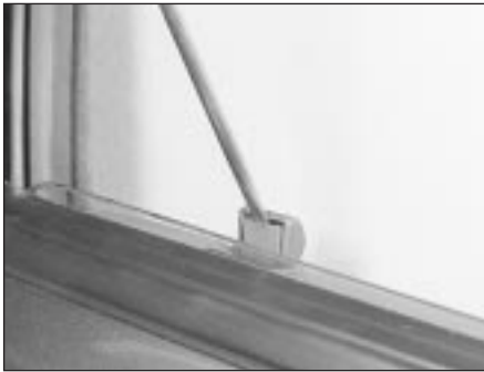
21.1a Prise apart the interior lock button . . .
