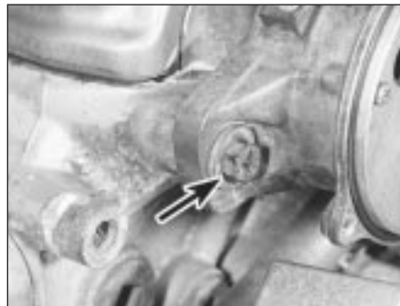
6.15a Undo the distributor retaining bolt . . .
