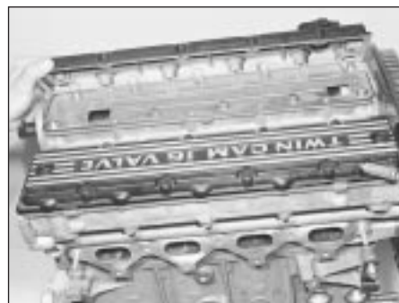
4.4b . . . and remove the covers
