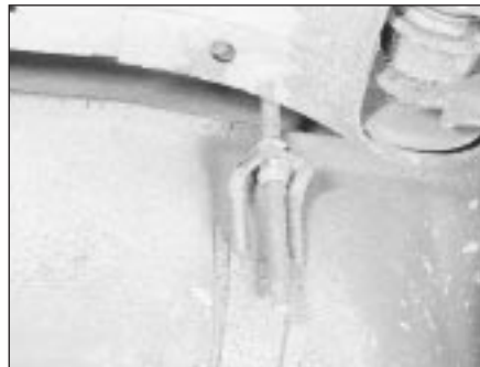
8.12 Fuel tank retaining strap and locknut
