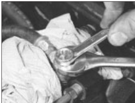
5.4 Releasing the fuel system pressure at the bleed screw on the banjo union
