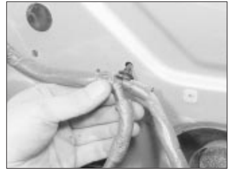
27.6a Release the wiring loom retaining clips . . .
