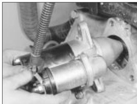
21.4 Removing the starter motor on 4-cylinder engines
