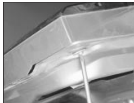
7.14 Remove the rear lens reflector and number plate assembly
