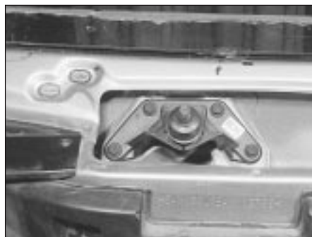
16.15a Wiper linkage centre spindle assembly . . .
