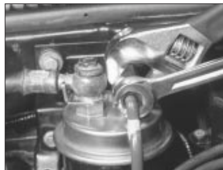
34.4 On V6 engines, unscrew the inlet union nut and withdraw the pipe from the filter head
