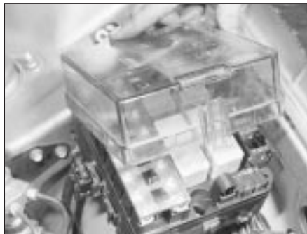
3.8 Removing the engine compartment fuse and relay box cover
