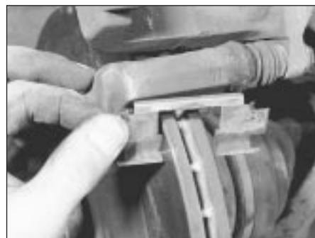
3.4b Remove the upper anti-rattle shim ...
