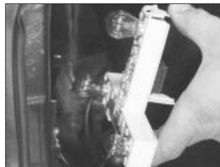
5.26b On the alternative bulb panel, press the top and bottom retainers together and remove the panel
