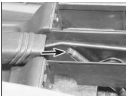
17.7 Handbrake adjuster location (arrowed)
