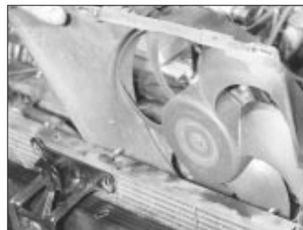
5.10b Removing the cooling fan assembly
