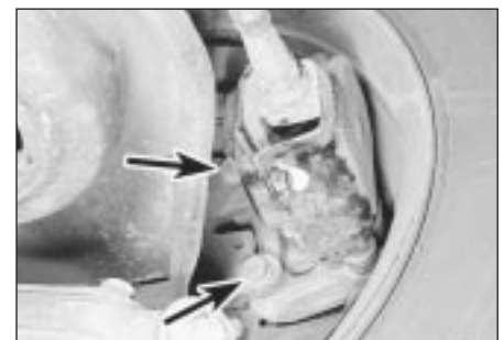
10.2 Carrier bracket-to-rear hub carrier retaining bolts (arrowed)
