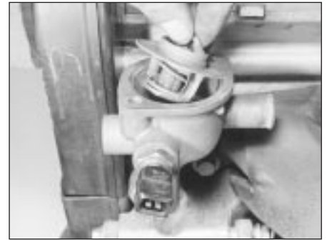
4.4 Withdraw the thermostat from the housing
