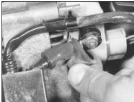
17.12 Pull back the rubber cap and unscrew the main terminal nut
