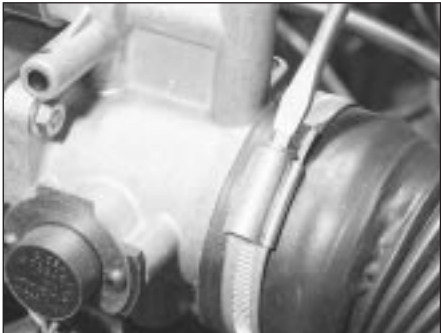
2.1 Disconnect the air trunking at the throttle housing
