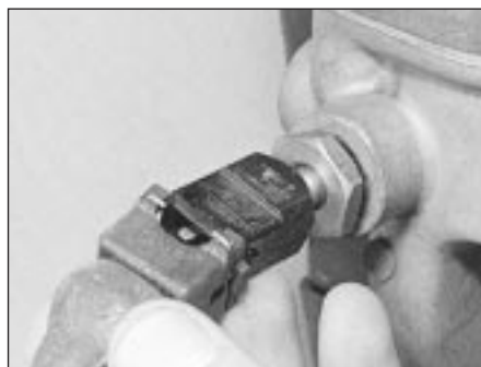
6.7a Disconnecting the coolant temperature sensor multiplug on the 4-cylinder engine
