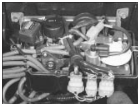
9.5 Wiring multiplug connections on the front of the control box
