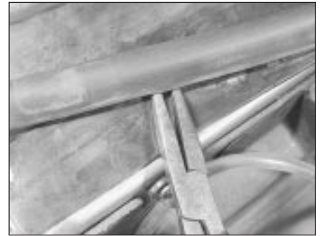
16.5a Release the rubber sealing strip retaining clips . . .
