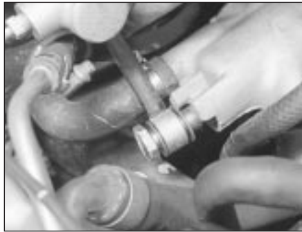
5.7 Undo the brake servo banjo hose union at the manifold
