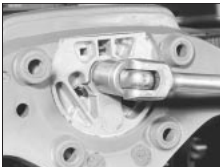
18.6 Undo the steering wheel retaining nut
