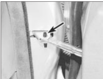
22.4 Tap out the door check strap retaining roll pin (arrowed)
