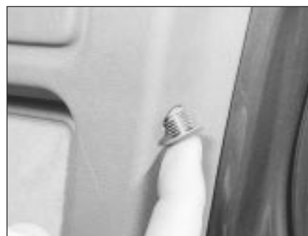
21.7a Pull out the blanking plug . . .
