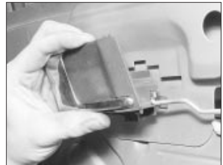
26.4 Withdraw the handle from the door
