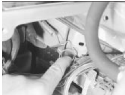
5.13 Unhook the direction indicator lens retaining spring
