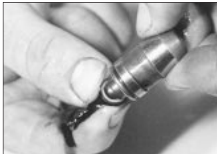
15.29 Depress the internal tappet valve to drain the oil prior to installation
