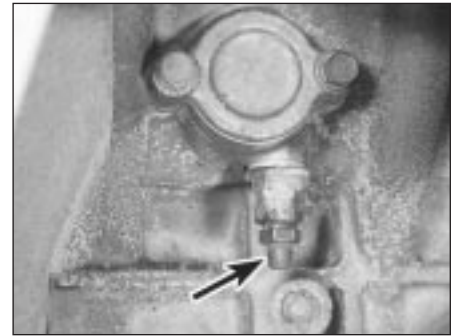
38.5 V6 engine cylinder block drain plug (arrowed)
