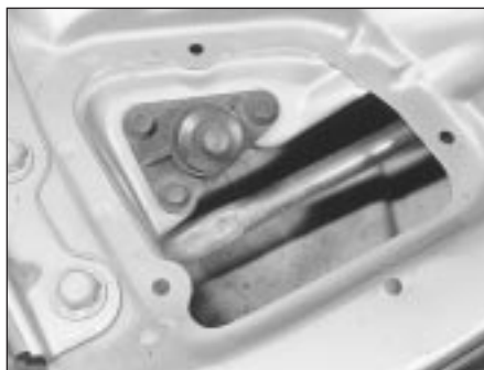
16.15b . . . and right-hand spindle assembly
