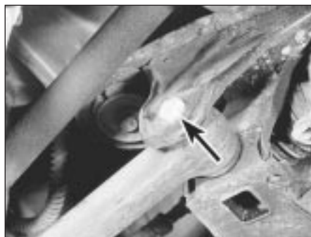
8.6 Lower suspension arm inner mounting bolt (arrowed)
