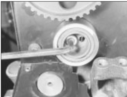
11.3 Undo the timing belt idler pulley bolt
