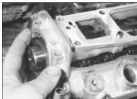
15.11 Lift the camshaft carrier off the cylinder head
