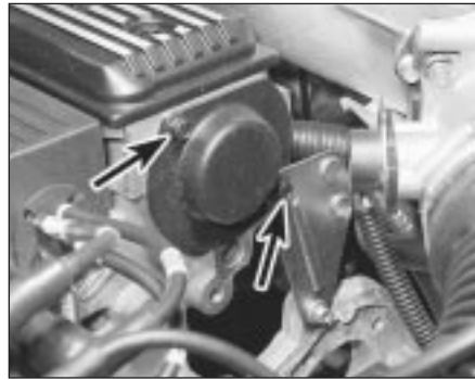
10.17 Undo the two bolts (arrowed) and remove the blanking plate
