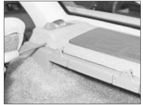
21.4 Remove the trim panel over the rear speaker on Fastback models
