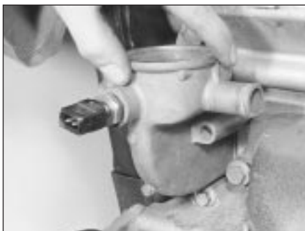
4.7 Removing the thermostat housing
