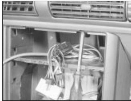
48.11a Undo the lower facia upper screws . . .
