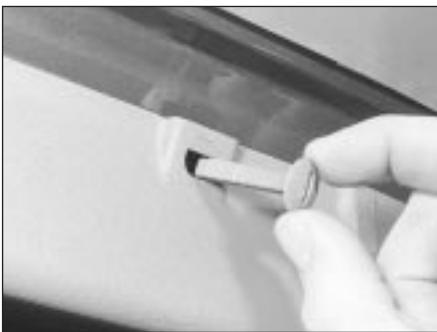
16.1 Release the screw studs and remove the tailgate inner trim panel
