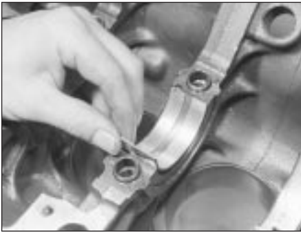
21.4 Fitting the main bearing shell upper halves
