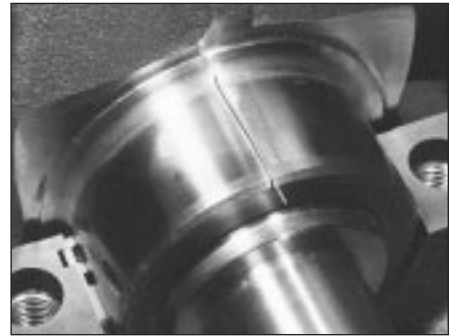
21.7 Plastigage in place on a crankshaft main bearing journal
