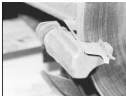
7.6c . . . and lower anti-rattle shim
