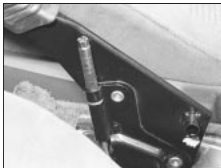
18.3 Unscrew the handbrake adjuster on the side of the lever
