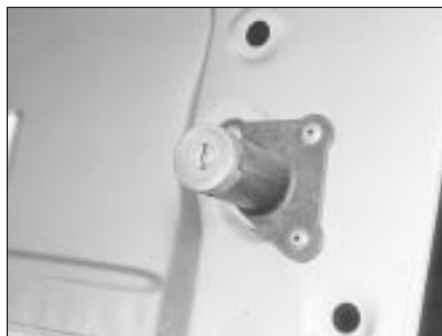
10.4 Boot lid private lock retaining rivets
