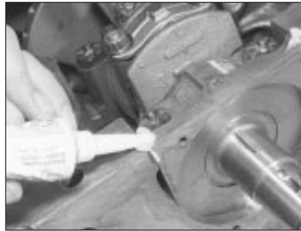
13.15 Apply sealant to the main bearing cap joints
