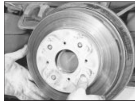
11.6b . . . and remove the brake disc
