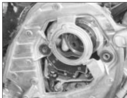
14.3 Remove the timing belt backplate from the front cylinder head
