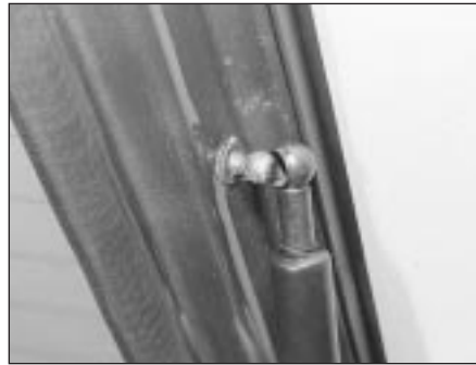
15.2b . . . and release the strut from the stud
