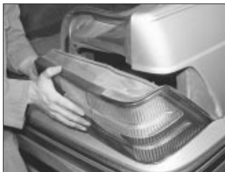
7.8b Removing the rear light cluster assembly
