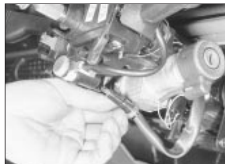
6.27 Withdraw the bulbholder from the fibre optic diffuser unit
