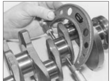
17.4 Measuring the main bearing journal diameters
