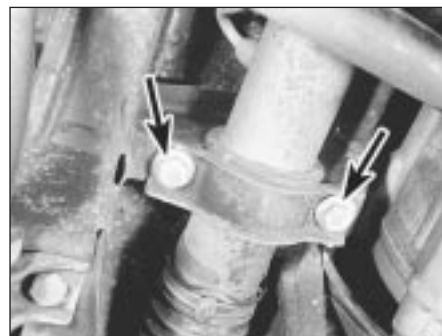
24.12b . . . and left-hand mounting bracket bolts (arrowed)
