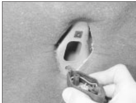
6.2 Remove the under-bonnet illumination light
