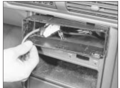
48.8b . . . and remove the mounting plate
