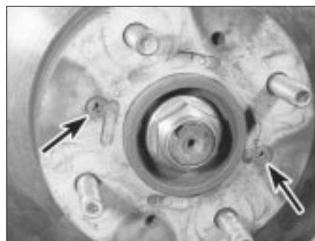
6.9a Undo the two retaining screws (arrowed) . . .
