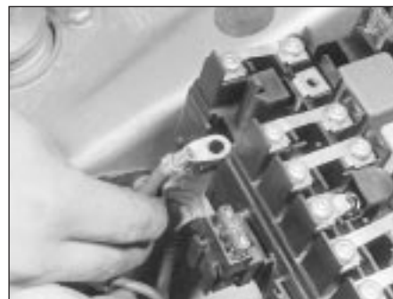
4.21c . . . and remove the cable from the fuse and relay box
