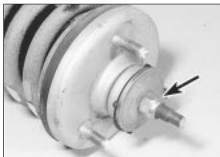
6.3 Remove the retaining nut (arrowed) from the shock absorber spindle
