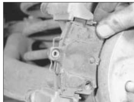
7.6a Lift out the two brake pads . . .
