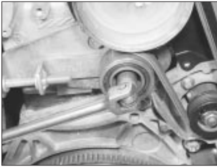
26.7 Slacken the tensioner wheel retaining nut
