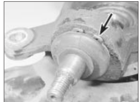
4.2 Balljoint retaining circlip (arrowed)
