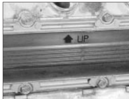
6.6 Ensure that the arrow, and the word UP are at the top when refitting the side covers
