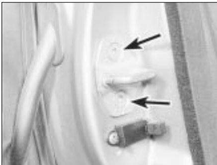
22.8 Door striker plate retaining screws (arrowed)
