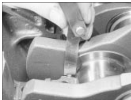
13.3 Checking crankshaft endfloat using feeler gauges
