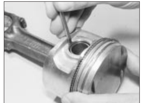
16.13 Using a small screwdriver to extract the gudgeon pin circlip
