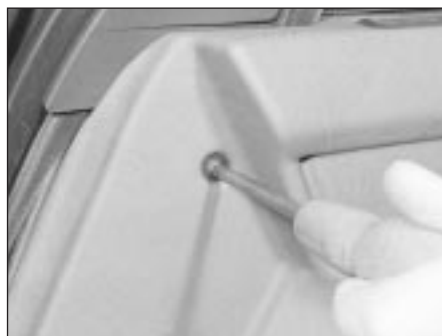
21.8 Undo the screw at the front corner
