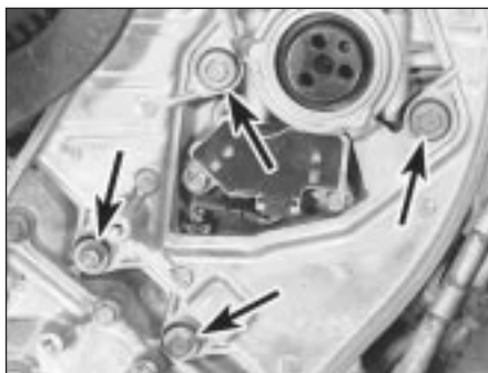
14.2 Front cylinder head backplate retaining bolts (arrowed)
