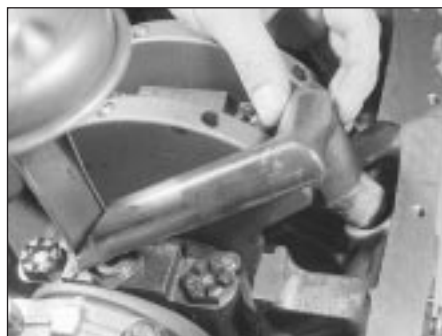
13.5 Remove the crankcase breather tube extension tube
