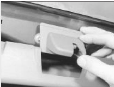
16.3 Remove the plastic cover from the lock
