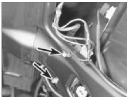
22.13 Aerial amplifier unit retaining bolts (arrowed) on Fastback models
