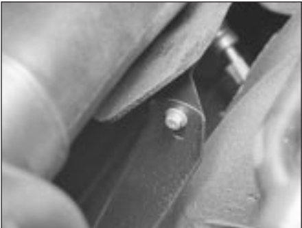
2.3 Forward air trunking to support bracket bolt
