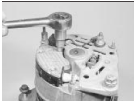
18.2 Undo the regulator and brushbox retaining screws
