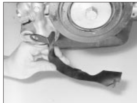
7.13 Removing the timing belt bottom cover
