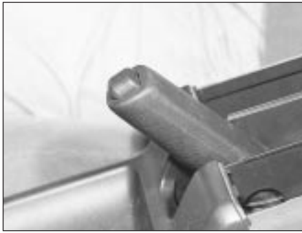
47.11a Apply the handbrake fully . . .
