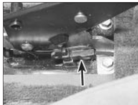
18.5 Disconnect the warning light switch wiring plug (arrowed)
