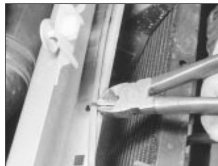
5.8 Cut off the cable ties securing the bonnet release cable
