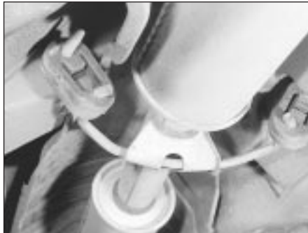
23.2 Typical exhaust system rubber mountings and brackets
