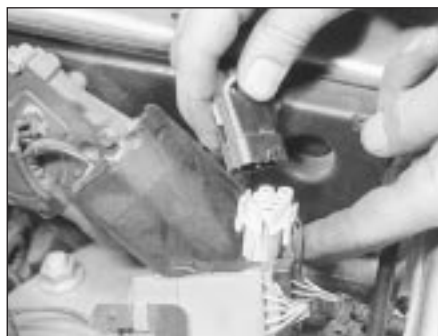
16.8 Disconnect the motor wiring multiplug
