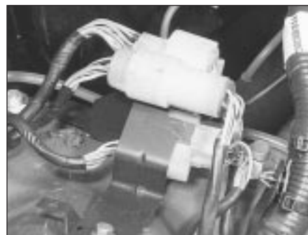
4.18c Disconnect the appropriate multiplugs at the rear of the engine compartment
