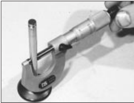
9.12 Measuring the valve stem diameter
