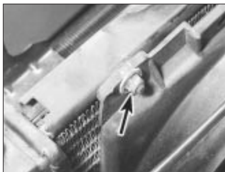
5.10a Cooling fan upper retaining nut (arrowed)
