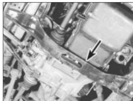
4.35 Undo the bolts and remove the longitudinal support member (arrowed)
