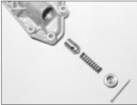
15.2 Oil pressure relief valve components
