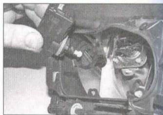
7.5b ... pull the motor away from the headlight unit to release the balljoint from the reflector ...
