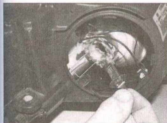
5.9b ... then lift the bulb out of the light unit
