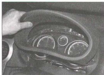
9.2 Pull the instrument panel shroud away from the fascia to release the five retaining clips
