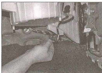
9.33 Disconnect the wiring connector from the underside of the blower motor resistor undo the three bolts and remove the servo motor from the side of the air distribution housing (see illustration).
