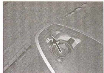
26.8 Undo the retaining screw (arrowed) at the front of the information display cover panel
