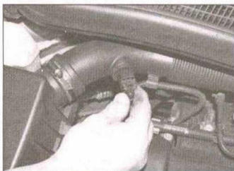
2 Check that the airflow meter or air temperature sensor wiring is connected securely.
