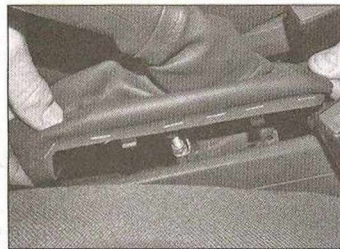
13.3 Unclip the handbrake lever gaiter from the centre console and fold it up the handbrake lever
