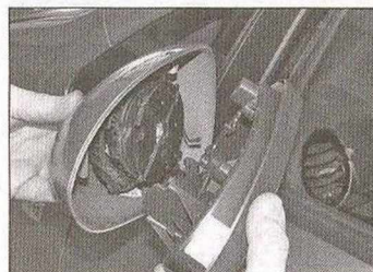
17.5c ... and remove the rear part of the mirror housing from the mirror body
