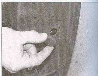
13.2 Open the door and carefully prise out the blanking cap from the rear edge of the door
