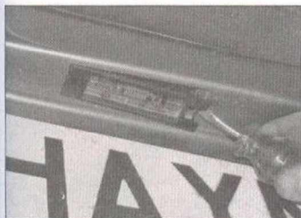
5.35 Carefully prise the number plate light unit out from its location
