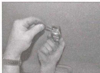
6.7 Carefully prise the rear courtesy light unit out of position, and withdraw the unit
