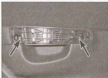
12.12b ... and undo the two screws now exposed (arrowed)
