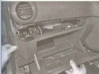
26.3 Withdraw the glovebox from the facia and disconnect the glovebox light wiring connector (where applicable)
