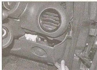
26.16 Withdraw the lower trim panel downwards to disengage the upper lugs
