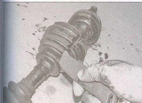
3.3 Cut the gaiter open using a suitable knife and remove it from the driveshaft
