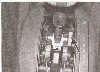
6.12 Push the yellow release lever (arrowed) on the lock solenoid downward to release the selector lever lock
