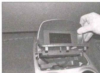
10.6a With the four screws removed, lift the information display unit up to release the three clips ...
