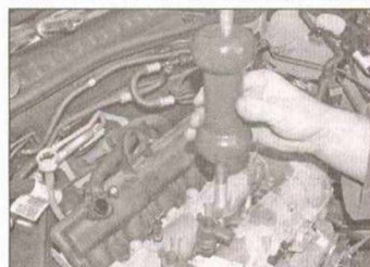
13.10a If necessary, use a slide hammer to free the injectors ...
