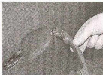
13.5 Disengage the exterior handle front pivot from the frame and remove the handle from the door
