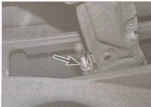
23.6 . . . for access to the handbrake cable adjuster nut (arrowed)
