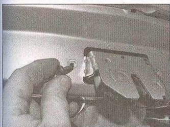
16.4 Undo the two lock assembly retaining screws
