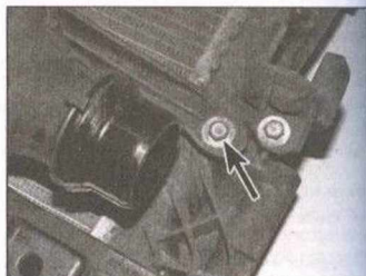
16.3 Intercooler retaining bolt (arrowed)
