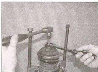
4.11 Counterhold the strut piston rod with an Allen key or suitable bit, and unscrew the piston rod nut
