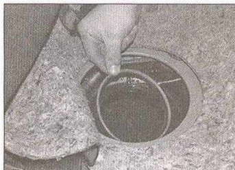
6.10 Collect the O-ring seal from the top of the fuel tank
