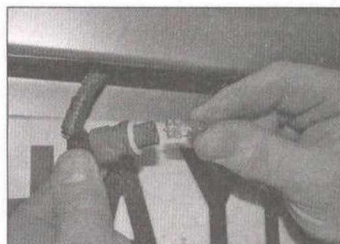
5.36b . . . and remove the push-fit bulb
