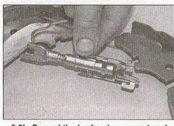
5.3k Spread the brake shoes apart and disengage the adjuster mechanism from the brake shoes
