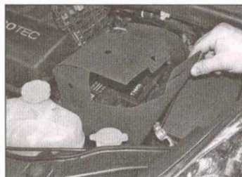
4.6 Where fitted, lift the battery jacket up and off the battery
