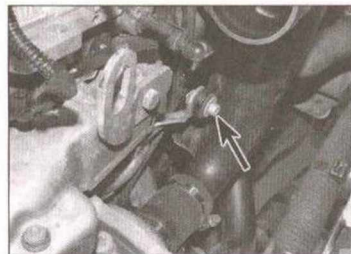
3.24 Undo the bolt (arrowed) securing the charge air pipe to the support bracket
