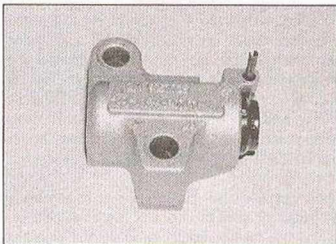
7.6 Timing chain tensioner plunger fully retracted and locked with the roll-pin
