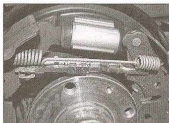
5.3d Pull the upper end of the trailing shoe outward and disengage it from the wheel cylinder piston
