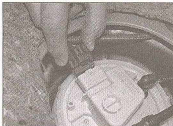
6.6 Disconnect the wiring connector from the tank module cover
