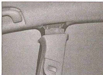
24.8 Prise the centre of the trim panel away from the B-pillar, then disengage the locating lugs at the top
