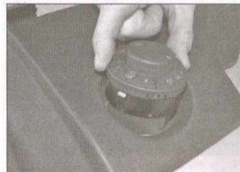
4.4b . . . then remove the switch from the trim panel
