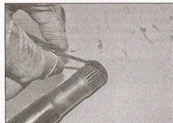
3.7 Removing the circlip from the groove in the driveshaft splines
