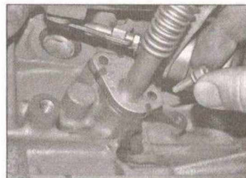
19.11 Undo the two bolts securing the turbocharger oil return pipe to the cylinder block
