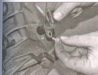
10.13 Undo the retaining bolt and remove the crankshaft speed/position sensor from the cylinder block
