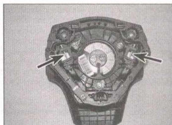
23.2b ... to depress the airbag internal spring retainers (arrowed – shown with airbag removed)
