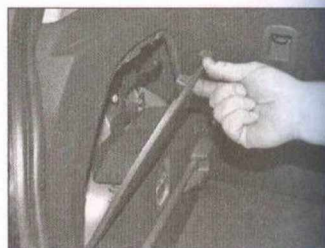
5.28 Open the access cover in the luggage compartment trim panel
