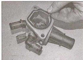
4.14 Remove the sealing ring from the thermostat housing – diesel engines
