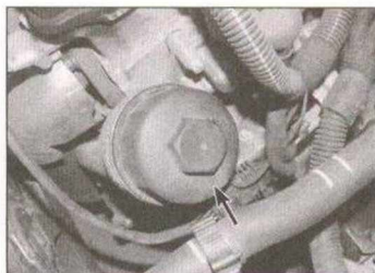
3.6 Oil filter on 1.4 litre engines (arrowed)
