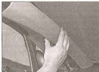
24.2 Pull the trim panel away from the A-pillar to release the two retaining clips
