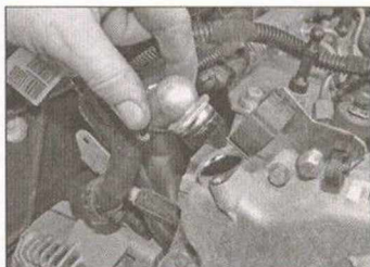
15.12 Undo the retaining bolt and detach the crankcase ventilation hose attachment
