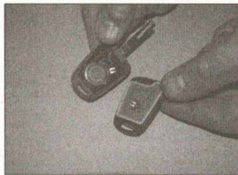
23.1 Prise the battery cover from the ignition key fob
