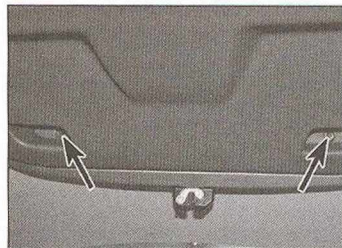
16.3 Undo the two screws (arrowed) securing the tailgate inner trim panel to the tailgate
