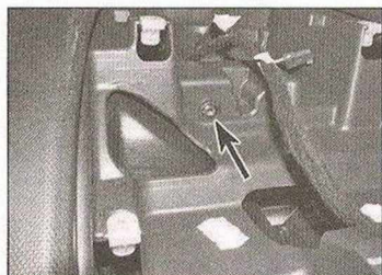
26.37c ... and the bolt (arrowed) in the fascia centre switch/vent panel aperture
