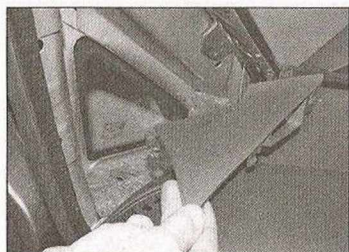
26.35 Unclip and remove the fascia upper end panels on both sides
