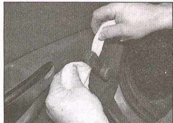
12.2a With a manual window regulator, locate a cloth rag between the handle and the trim panel and pull it to one side to release the spring clip ...
