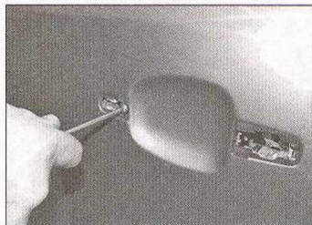
13.21a Undo the exterior handle frame front retaining screw and extract the rear guide clip ...
