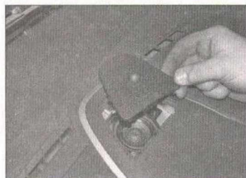
10.2 Carefully prise free the centre speaker panel from the upper centre of the facia
