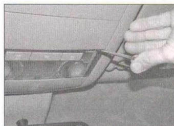
6.4 Carefully prise the light unit lens from the overhead console
