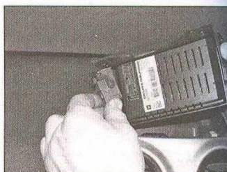
26.11b . . . then disconnect the wiring connector and remove the unit
