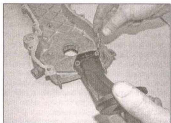
13.2a Remove the oil pick-up pipe from the oil pump cover ...
