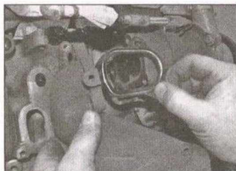
6.21 Separate the catalytic converter from the turbocharger and recover the gasket
