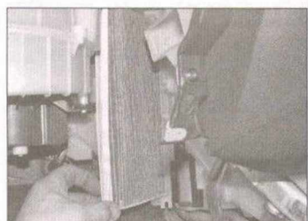
19.4 Withdraw the pollen filter from the housing
