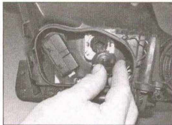
5.3 Push the dipped beam bulb base sideways and withdraw the bulb from the headlight unit
