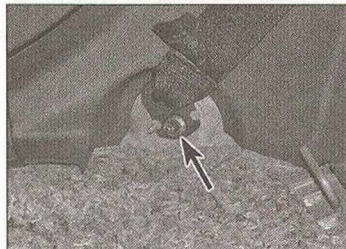
24.33 Undo the rear seat belt lower mounting bolt (arrowed)
