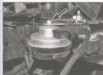
11.2 The horn(s) are located under the front bumper on the left-hand side
