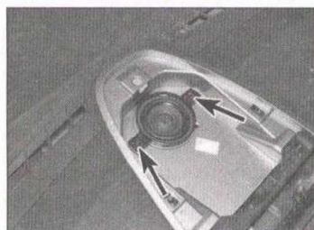
10.5a Undo the two screws (arrowed) securing the speaker to the centre switch/vent panel
