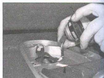
10.5b Lift out the speaker and disconnect the wiring connector
