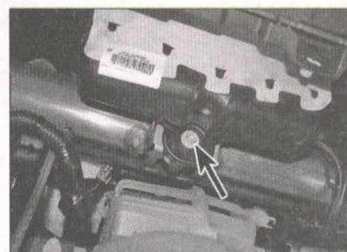
23.6 Undo the bolt (arrowed) securing the passenger's airbag to the fascia crossmember
