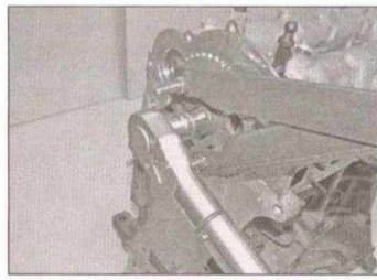
9.23 Hold the sprocket with the tool and tighten the retaining bolt to the specified torque
