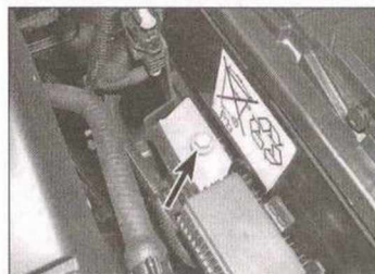
4.7 Unscrew the bolt (arrowed) and remove the battery retaining clamp
