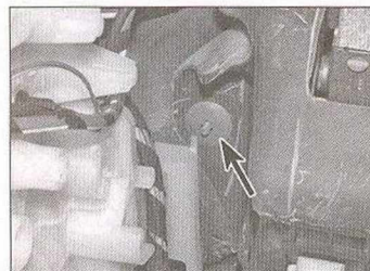
11.8b ... and left-hand plastic washer securing the foam sound deadening pad to the studs on the bulkhead
