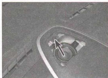
10.3 Undo the retaining screw (arrowed) at the front of the information display cover panel
