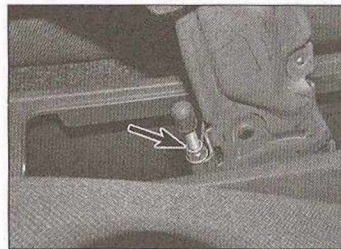
13.4 Fully slacken and remove the handbrake cable adjuster nut (arrowed)
