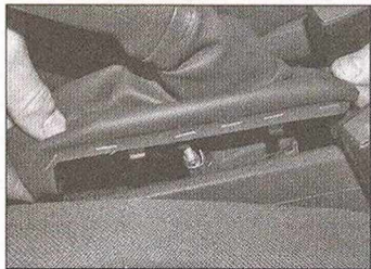
14.1 Unclip the handbrake lever gaiter from the centre console and fold it up the handbrake lever
