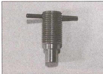
3.10a To make an alternative camshaft locking tool . . .
