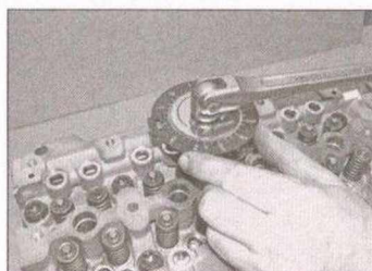
11.28 Tighten the bolts through the Stage 2 and Stage 3 angle using an angle-measuring gauge
