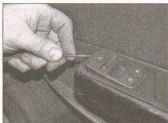
4.12 Carefully prise the electric window/mirror switch assembly out of the door inner trim panel
