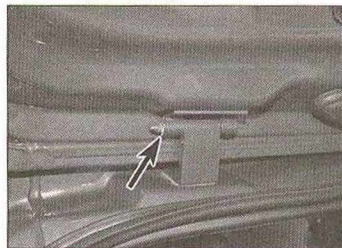
15.8 Extract the clips (arrowed) and carefully drive out the hinge pins from outside to inside
