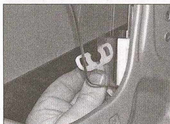
14.23a Release the two clips securing the window glass to the regulator ...
