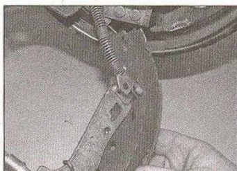
5.3e Similarly disengage the leading shoe from the abutment bracket and wheel cylinder, then turn the shoe assembly over for access to the rear
