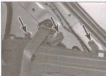
24.54 Undo the three screws (arrowed) along the upper edge of the trim panel
