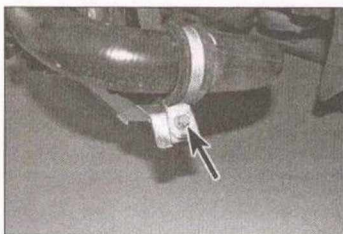
16.2b . . . then undo the bolt each side (arrowed) securing the charge air hose clamps to the radiator support crossmember
