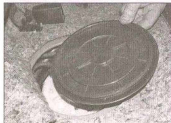
6.4 Carefully prise the plastic access cover from the floor
