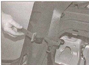
24.53 Undo the two bolts and remove the rear seat backrest locking bracket
