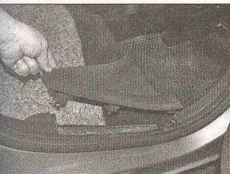
24.25 Lift the side sill rear trim panel upwards to release the clips and remove the panel
