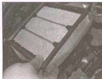
29.6 Lift out the air cleaner filter element
