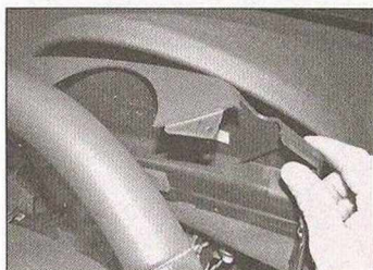
26.23 Lift the upper shroud off the steering column and remove it from the car
