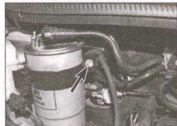
21.3a Undo the bolt (arrowed) securing the fuel filter mounting bracket clamp . . .
