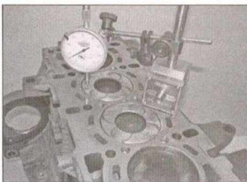
11.19 Using a dial test indicator to measure piston protrusion
