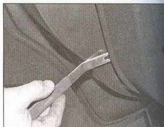
12.13 Using a wide-bladed screwdriver or removal tool, carefully prise the bottom and sides of the panel away from door
