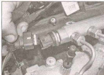
12.3a Disconnect the wiring connector at the fuel pressure sensor ...
