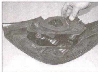
5.32b ... and withdraw the bulbholder from the light cluster
