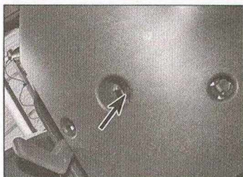
26.20 Undo the lower shroud lower retaining screw (arrowed)
