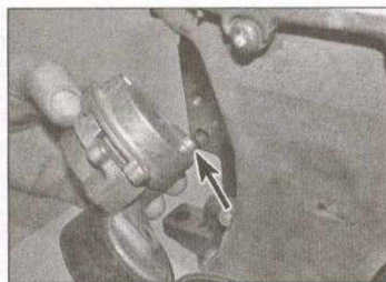
6.55 Refit the auxiliary drivebelt tensioner ensuring that the lug (arrowed) engages with the hole in the cylinder block
