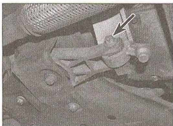
7.10 Undo the centre bolt (arrowed) from the torque link mounting
