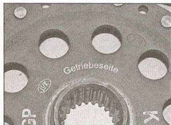
6.21 The lettering 'transmission side' or 'Getriebeseite' on the friction disc must point towards the transmission
