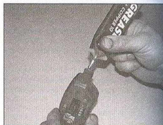
4.3i Apply a smear of high-temperature grease to the contact areas of the backing plates
