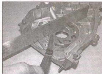
13.7 Checking the oil pump rotor endfloat
