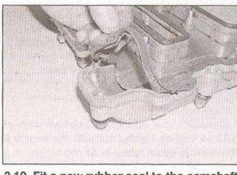
3.10 Fit a new rubber seal to the camshaft cover ensuring that it is correctly located in the cover groove
