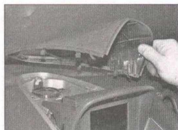
10.4b Once the side clips are released, move the panel forward to disengage the two lugs at the rear
