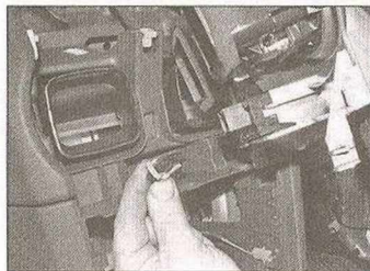
26.13b Disconnect the switch wiring connector and remove the switch/vent panel
