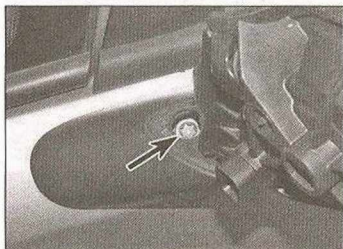
17.8a Undo the bolt (arrowed) securing the mirror body to the door ...
