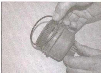
3.11a Renew the sealing ring on the oil filter cover ...
