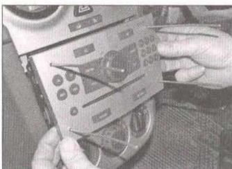
17.3 Removing the radio/CD player using welding rod to compress the internal clips
