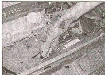
10.32 Undo the three bolts and remove the oil filter housing from the cylinder block
