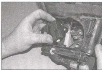
7.5a Rotate the headlight adjustment motor clockwise to free the motor from the headlight unit ...
