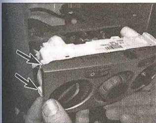
9.7b ... while at the same time pulling the assembly away from the fascia to release the two clips (arrowed) each side
