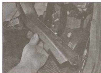
4.3 Remove the plastic expanding rivet and remove the footwell air duct
