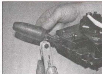
16.10 Use a 1.5 mm diameter rod to depress the internal retaining lug, and withdraw the switch stalk from the electronics module
