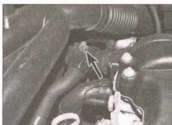
25.17b . . . and on automatic transmission models, unscrew the additional bleed screw (arrowed) located in the radiator top hose elbow
