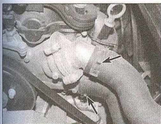
7.9a Release the clips (arrowed) and disconnect the hoses from the front ...
