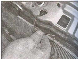
10.7b ... slide the other end off the release cable and remove the spring
