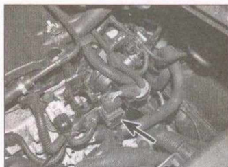
4 Check all multiplugs and wiring connectors for security.
