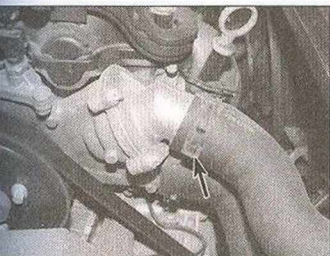
4.3 Release the clip (arrowed) and disconnect the hose from the thermostat housing cover – petrol engines
