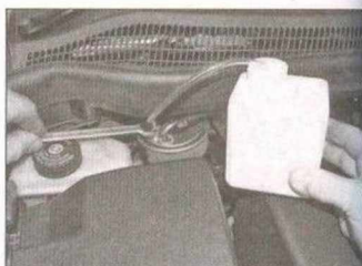
6.3 Unscrew the drain screw approximately two turns
