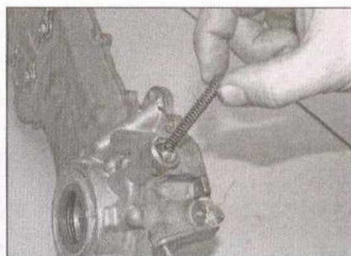
13.5b ... then withdraw the spring ...
