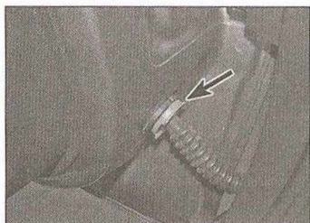
11.11 Disconnect the wiring connector (arrowed) from the front edge of the rear door window switch assembly from the door trim panel, then disconnect the wiring connector (see illustrations).
