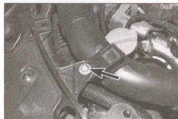
3.4a Undo the bolt (arrowed) securing the upper air inlet hose to the front body panel ...
