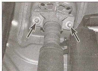
11.4 Undo the two bolts (arrowed) securing the shock absorber upper mounting to the underbody
