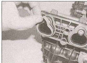
11.15 Fit new individual rubber seals to the grooves in the inlet manifold
