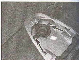
26.10a Undo the two screws (arrowed) securing the speaker to the centre switch/vent panel
