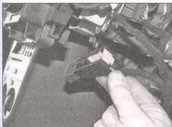
16.6 Disconnect the main wiring harness connector at the rear of the steering column electronics module
