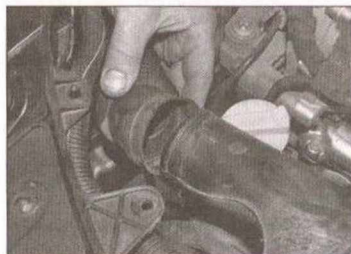
3.19b . . . and disconnect it from the connecting hose on the air cleaner
