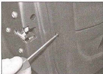
12.5b ... and rear screw securing the edge of the trim panel to the door
