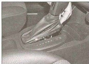
6.11 Unclip the selector lever gaiter from the selector lever cover and fold the gaiter up the lever
