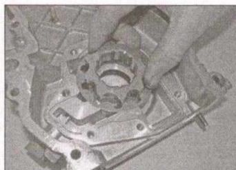
13.4a Remove the oil pump inner rotor ...
