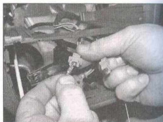
6.16 Pull the relevant heater control illumination bulb from the bulbholder
