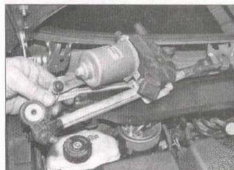
13.5b ... and withdraw the wiper motor and linkage assembly from the scuttle
