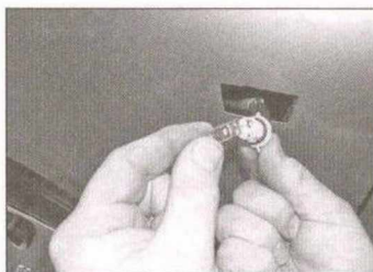
5.19b The bulb is a push-fit in the bulbholder
