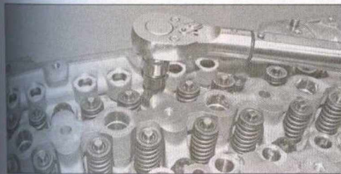
11.27a Working in sequence, tighten the cylinder head bolts to their Stage 1 torque, using a torque wrench
