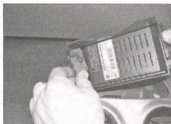
10.6b ... then disconnect the wiring connector and remove the unit
