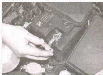
3 Check the security and condition of the battery connections.
