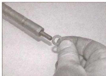
13.11 Remove the copper washer from each injector
