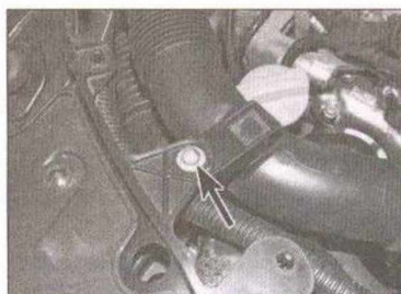
29.4a Undo the bolt (arrowed) securing the upper air inlet hose to the front body panel...
