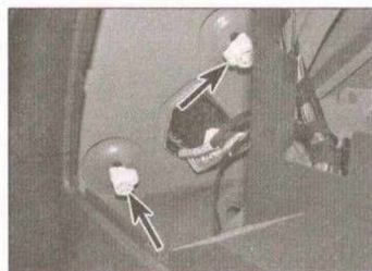
5.29 Slacken the two light cluster plastic retaining nuts (arrowed) and remove one of the nuts
