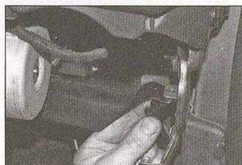
26.31a Extract the expanding rivet ...
