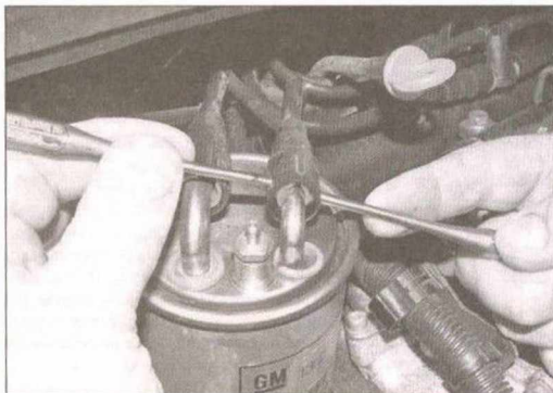
21.4 Using two screwdrivers to detach the fuel hose quick-release connectors
