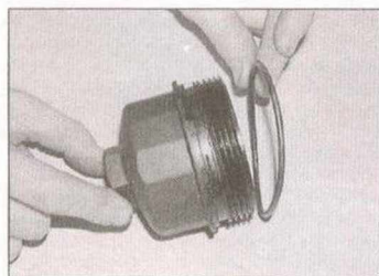
3.11a Fit a new sealing O-ring to the oil filter housing cap ...
