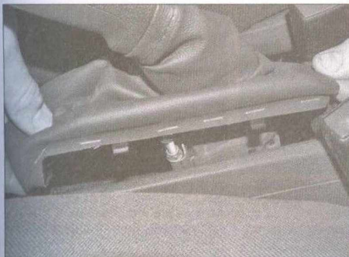
23.5 Unclip the handbrake lever gaiter from the centre console . . .
