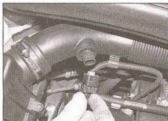
10.9 Disconnect the wiring connector from the inlet air temperature sensor
