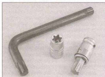
Torx key, socket and bit
