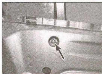
14.21a Undo the bolt (arrowed) securing the lower end of the window rear guide rail to the door ...
