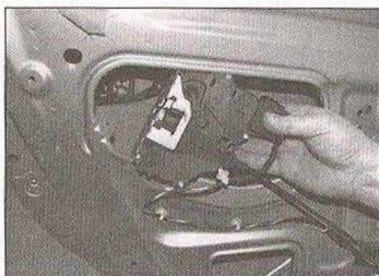
13.35a Withdraw the lock from its location . . .
