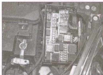
5 Check that all fuses are still in good condition and none have blown.
