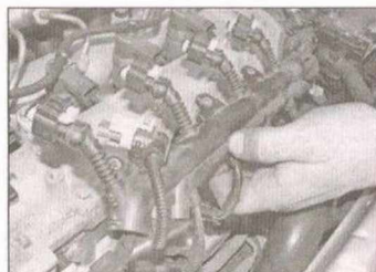
13.6 Disconnect the injector wiring, while moving the wiring harness guide forward
