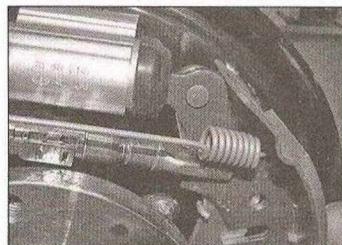
5.3u Engage the leading brake shoe with the abutment bracket and wheel cylinder then similarly engage the trailing shoe with the wheel cylinder . . .
