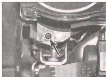
9.3c . . . and lower left-hand retaining screw (arrowed)
