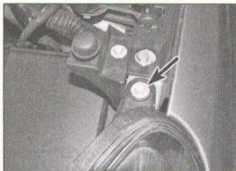
7.2b ... the upper retaining bolt (arrowed) ...
