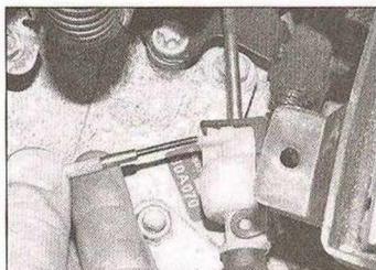
3.3 Using a small screwdriver, open the clamping piece on the selector cable adjuster as far as the notch
