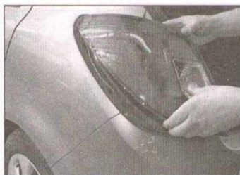
5.30 Hold the light cluster from the outside, remove the remaining nut and withdraw the cluster from the rear wing
