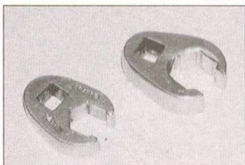
2.6 Two crow-foot adaptors will be necessary for tightening the fuel pipe unions
