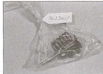
7.6 Place each valve assembly in a labelled polythene bag or similar container
