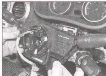
16.9b ... and withdraw the module from the steering column
