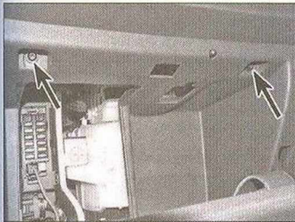
26.2a Undo the two glovebox upper retaining screws (arrowed) ...
