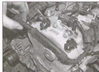
6.33 Release the wiring harness from the timing cover support clips
