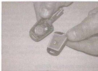
25.1 Prise the battery cover from the ignition key fob
