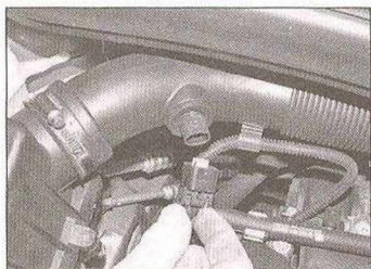
2.2 Disconnect the wiring connector from the inlet air temperature sensor
