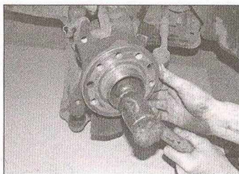
2.12a Tap the end of the driveshaft with a soft-faced hammer . . .
