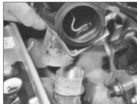
4.12 Do not lose hot air intake connector hose when removing air cleaner metal intake duct
