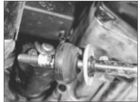
9.6 Fit flange washer, spacer and mounting bush onto tie bar . . .
