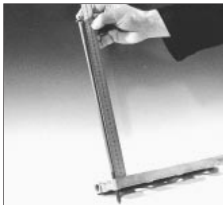
9.16 Checking length of cylinder head bolts
