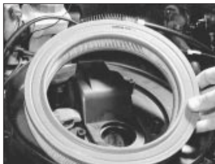
31.3 Ensure new filter element is correctly seated on refitting
