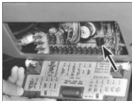
3.2 Remove fuses with plastic tweezers supplied (arrowed)
