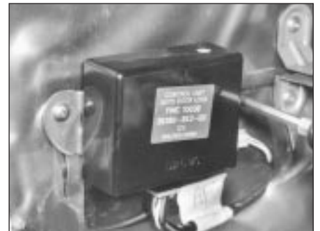
15.5 Central locking control unit must be removed when working on left-hand door
