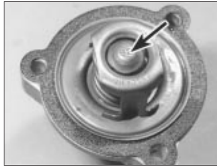
6.8 Note temperature specification stamped on thermostat end
