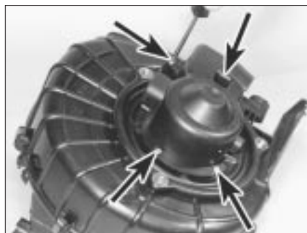
10.20a Remove motor cover retaining screws (arrowed)...
