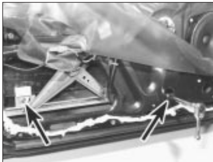
15.9 Undo window-to-regulator retaining bolts
