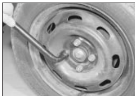
4 Use the wheel brace to slightly loosen the wheelnuts
