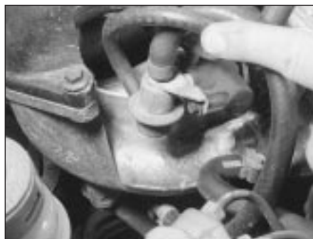
14.25 Fuel pressure regulator location - alloy inlet manifold
