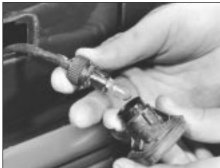
5.16 ... then withdraw lamp and pull out bulbholder
