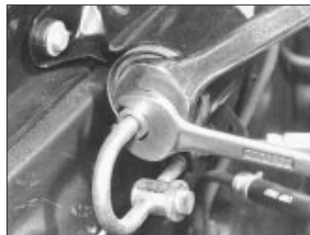
32.2 Use two spanners when slackening fuel filter unions - non catalyst model shown
