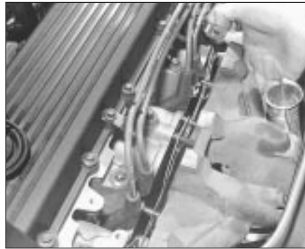
17.8a Refitting exhaust manifold with new gasket
