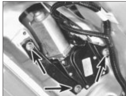
23.7 Tailgate wiper motor mounting bolts (arrowed)
