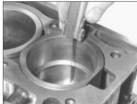
13.5b Measuring piston ring end gap
