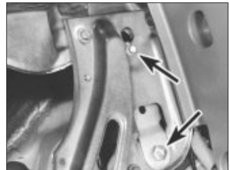
28.22 . . . and inertia reel retaining bolts (arrowed) - 4-door models
