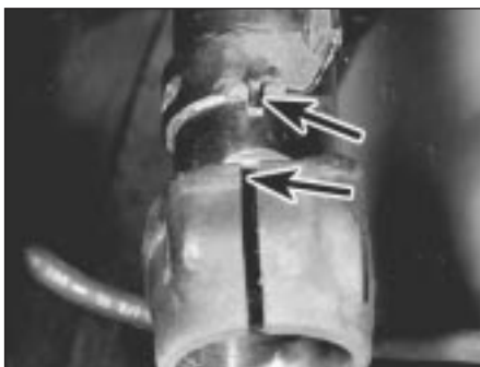
5.7 Align suspension strut lug with slot in swivel hub (arrowed)
