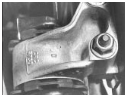
19.12 Check rubber washers are correctly installed before tightening through-bolt nut
