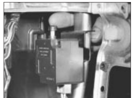
15.39 Reset fuel cut-off inertia switch by depressing plunger
