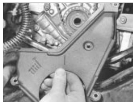
7.4 Removing timing belt lower cover
