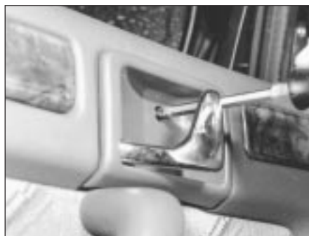
14.2a Undo retaining screw ...
