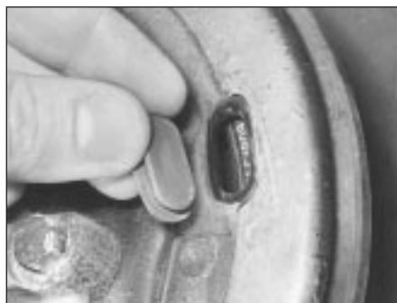
21.2 Remove grommet to check rear brake shoe friction material thickness
