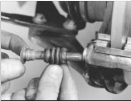
11.7 Check condition of guide pins and gaiters before refitting pads
