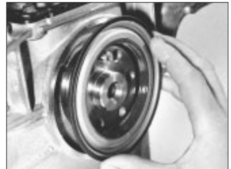
18.30a Fitting a new crankshaft left-hand oil seal
