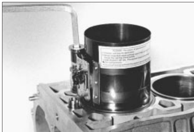
18.15b Using piston ring compressor to clamp piston rings
