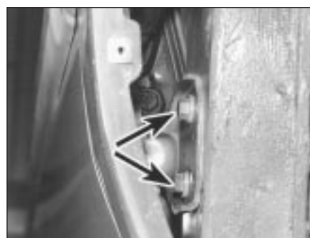
13.5 Remove wheel archliner to gain access to front door hinge retaining bolts (arrowed)
