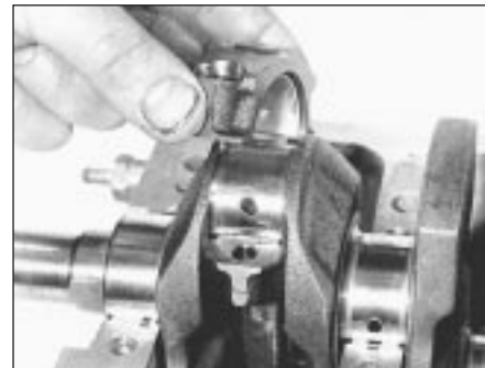
10.9 Removing No 1 cylinder big-end bearing cap and lower bearing shell
