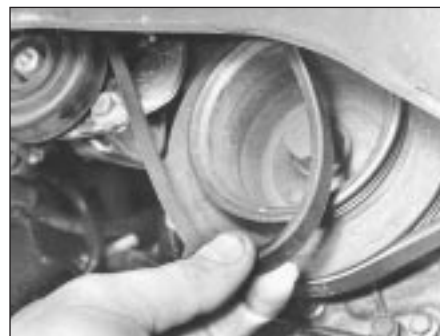
26.10 Power steering pump drivebelt removal
