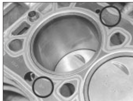
13.26b . . . so that TOP mark is upwards and FRONT arrow points to timing belt end
