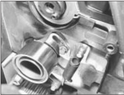
9.39 Ensure timing belt tensioner spring is correctly hooked onto pillar bolt
