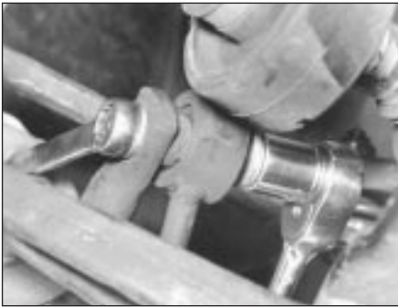
7.4 Slacken and remove anti-roll bar-to-connecting link bolts
