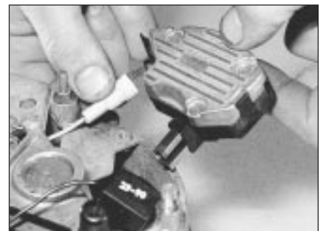
7.2 Remove voltage regulator/brush holder from alternator and disconnect wiring lead
