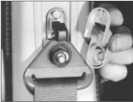
28.2 Removing cover to reveal front seat belt upper mounting nut
