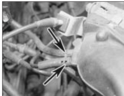
16.9 Disconnect breather hoses (arrowed) from manifold chamber
