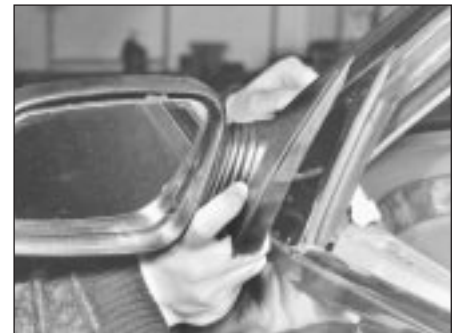
16.4b . . . and remove mirror assembly from door
