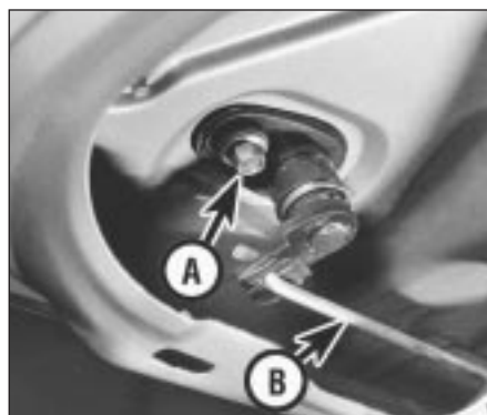
18.7 Boot lid lock cylinder retaining bolt (A) and operating rod (B)
