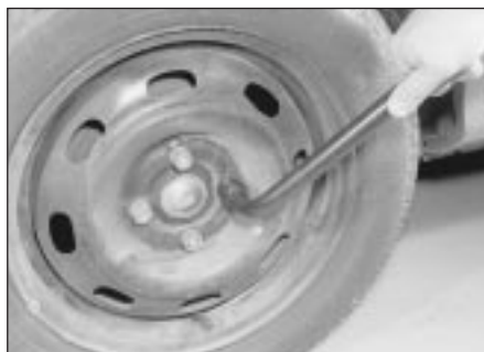
8 Fit the replacement wheel and tighten the nuts
