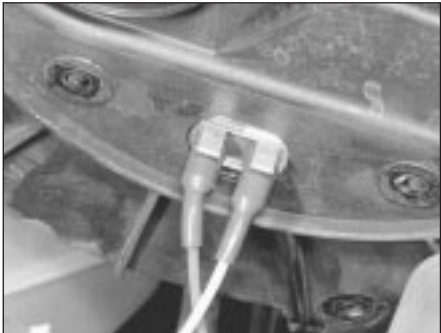
3.2 Note colour-coding of thermac switch vacuum pipes before disconnecting
