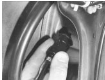
19.12 Disconnecting fuel filler release cable - 414 models
