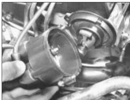
15.7 Distributor cap is retained by two offset screws
