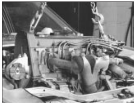
4.34 Lifting out engine/gearbox unit
