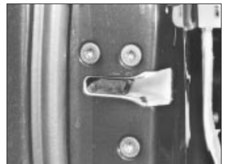
12.4 Door lock retaining screws (Torx type)
