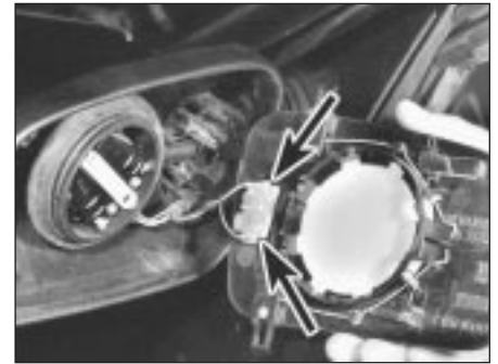
16.2b Disconnect wiring connectors (arrowed) and remove mirror glass - electrically-operated mirrors
