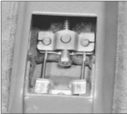
23.4b . . . to gain access to handbrake cable adjuster nut and equalizer mechanism
