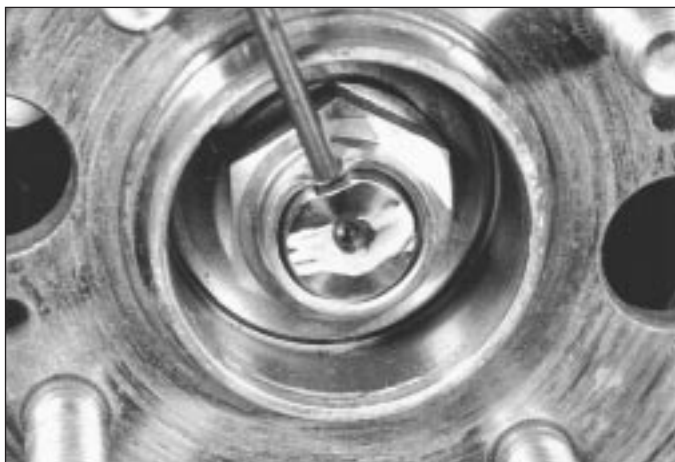
11.11 Stake hub retaining nut firmly into stub axle groove
