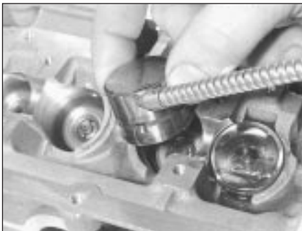
11.26 Lubricate hydraulic tappets thoroughly and refit correct way up - K8 engine
