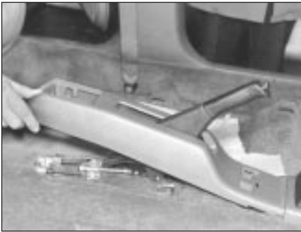
30.2b ... and remove centre console rear section (front seats removed for clarity)
