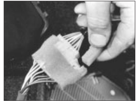
14.5 Disconnect wiring connectors as trim panel is removed - electrically-operated windows
