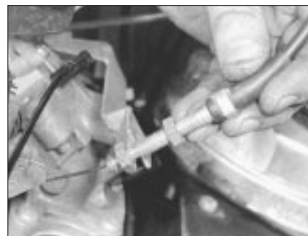
9.2 Disconnecting accelerator cable from carburettor
