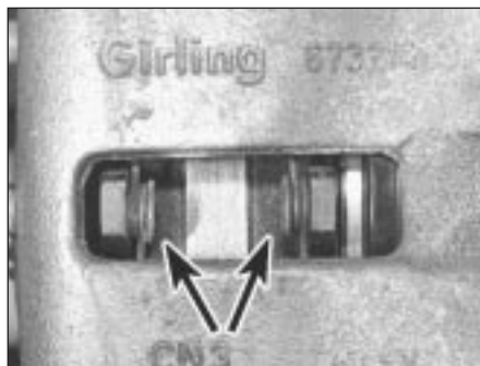
20.2 Front brake pad friction material (arrowed) can be checked through slot in caliper body
