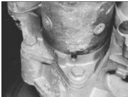
10.6a Starter motor lower mounting bolts viewed from underneath
