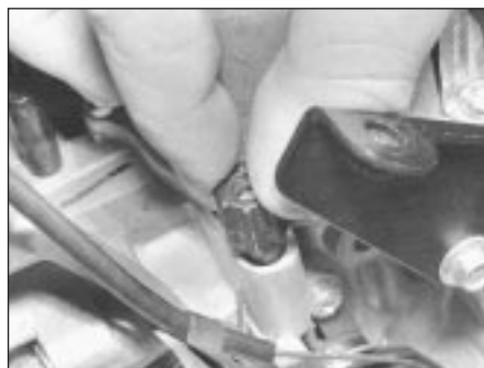
12.4 Turning idle speed adjusting knob to alter engine idle speed
