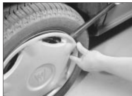
3 Remove the trim to expose the wheelnuts
