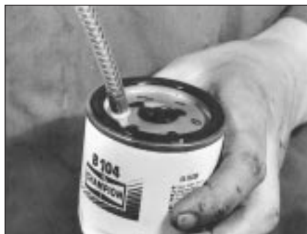
9.9 Applying a light coat of clean engine oil to oil filter sealing ring
