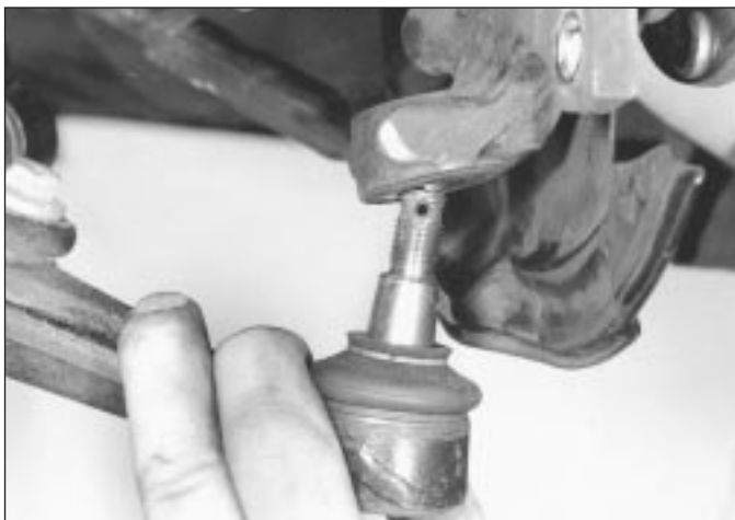
10.4a Release balljoint from swivel hub assembly . . .
