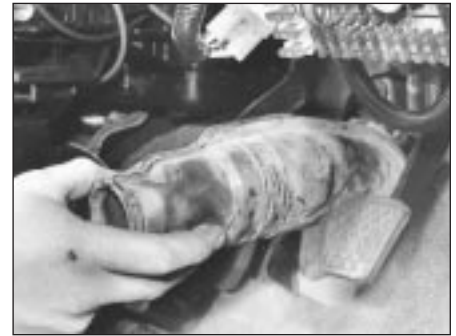
19.7b . . . and withdraw lower steering column cover
