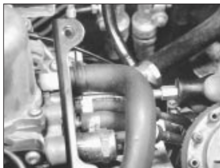
12.6 Adjusting idle mixture (air cleaner removed for clarity)
