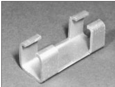
9.11a Camshaft locking tool cut from steel section ...
