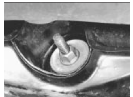
9.3 Tie bar retaining nut is accessed from front of subframe
