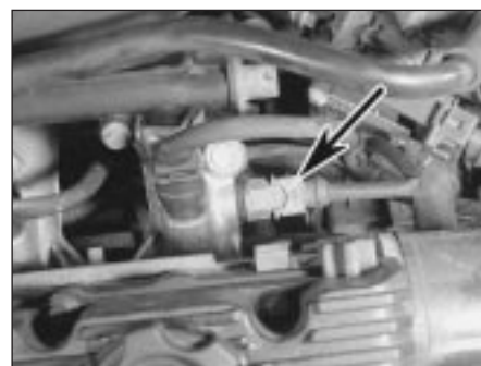
14.49 Intake air temperature sensor multiplug (arrowed)
