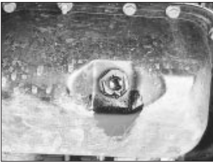
Engine oil may leak from the drain plug...
