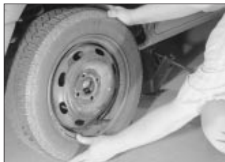
7 Remove the wheelnuts and lift off the wheel
