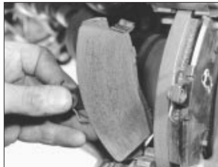
11.4 Removing pads with springs and shims
