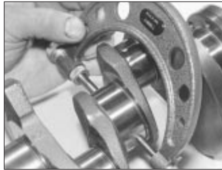
14.8 Measuring crankshaft journal diameter
