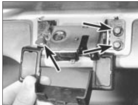
22.3 Remove plastic cover to gain access to tailgate lock retaining bolts (arrowed)
