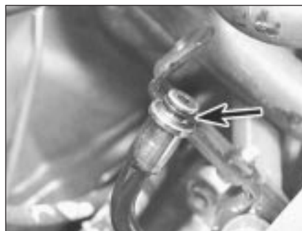
25.7 Always renew outlet pipe O-ring (arrowed)
