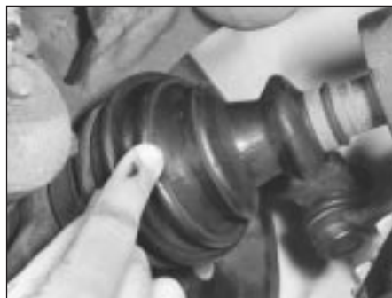
18.1 Checking driveshaft outer CV joint rubber gaiter
