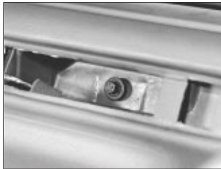
31.12a Facia centre mounting bolt is accessed via clock aperture
