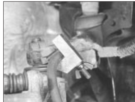
8.1 Using a brake hose clamp to minimise fluid loss
