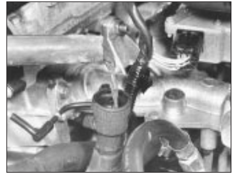
10.16 Filling cooling system slowly via filler stem
