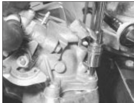
13.8a Unscrew upper-to-lower inlet manifold Torx screws . . .
