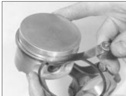
13.5a Measuring piston ring-to-groove clearance
