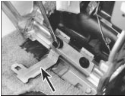
31.9 Slacken two facia mounting bolts and remove relay module mounting bracket (arrowed)
