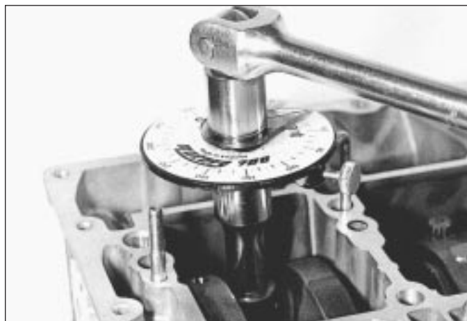
19.17b . . . then use angular torque gauge to tighten bolts through angle specified (second stage)
