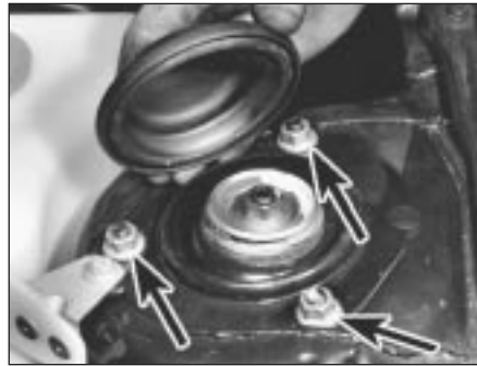
5.6a Remove rubber cover and strut upper mounting nuts (arrowed)
