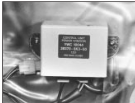
15.4 Control unit for electrically-operated windows must be removed when working on right-hand door
