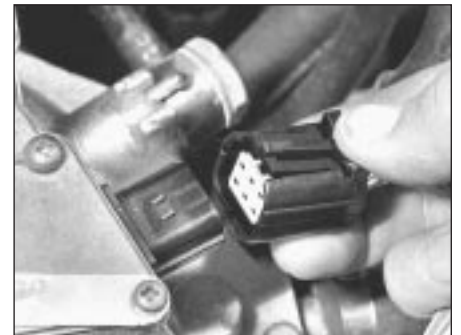
15.12 Disconnecting stepper motor wiring connector
