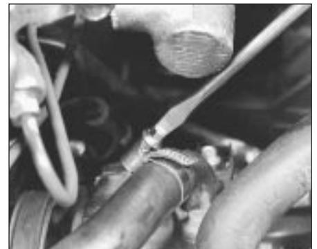
25.2a Slacken retaining clamp and disconnect inlet hose from pump
