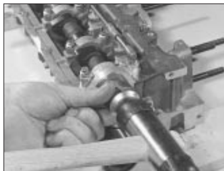
11.31 Fitting a new camshaft right-hand oil seal - K8 engine
