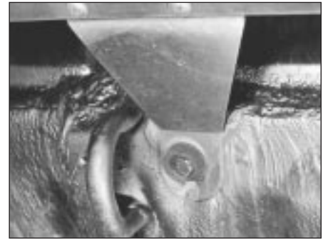
7.17 Rear bumper centre mounting bracket-to-body bolt - 414 models
