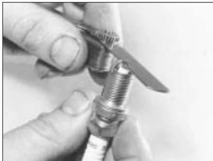
34.10a Measuring a spark plug electrode gap with a feeler gauge
