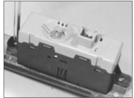
13.3 Removing clock retaining screws (remaining one arrowed)
