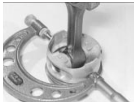
13.1 Measuring piston diameter
