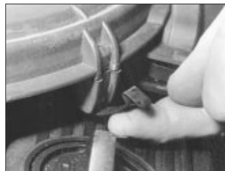
31.1a Release air cleaner assembly cover retaining clips . . .
