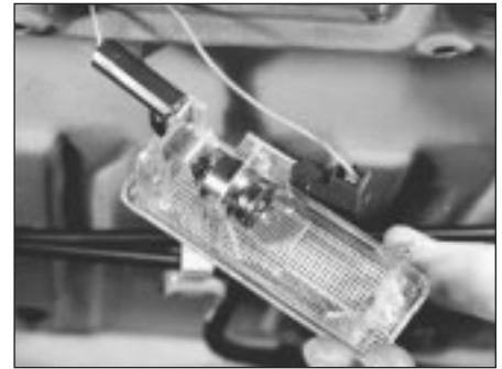
6.9 Luggage compartment lamp bulb is of bayonet type
