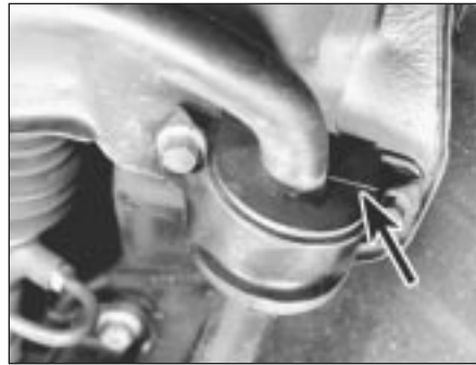
7.5 Correct position of anti-roll bar mounting bush split (arrowed)
