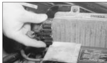
E The ECU wiring plugs may cause problems if dirty or not properly connected
