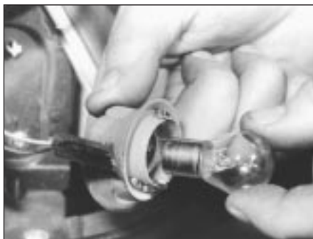
5.13 Indicator bulbs are of bayonet type
