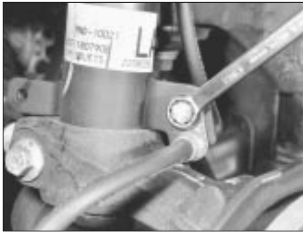
5.4 Removing bolt securing brake hose to suspension strut
