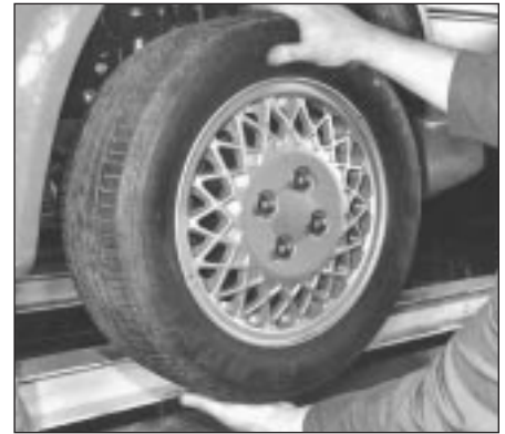
24.4 Rocking a roadwheel to check steering/suspension wear
