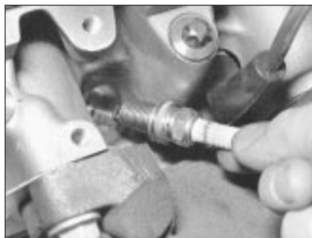
34.5a Spark plugs are easily accessed on K8 engine
