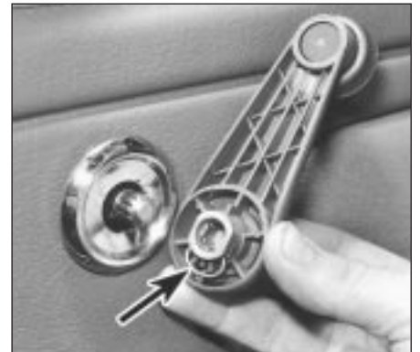
14.6 Fit horseshoe clip (arrowed) to handle before refitting handle to regulator
