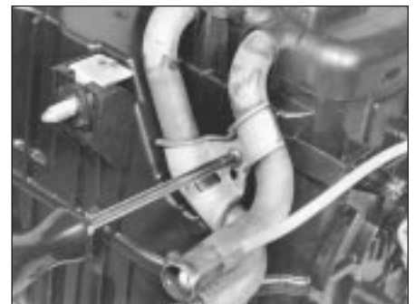
10.12 Undo retaining screw and remove matrix outlet pipe bracket
