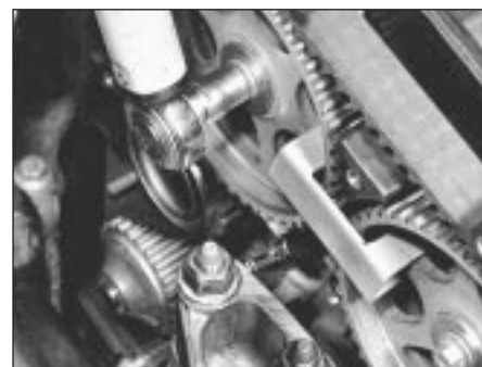
9.23b Locking camshafts in position with fabricated tool - K16 engine
