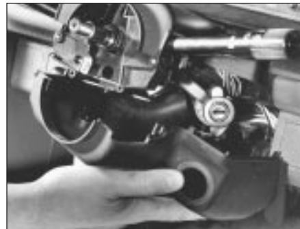
19.3c . . . and remove lower and upper shrouds
