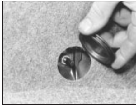
7.16 Remove rubber grommet to gain access to bumper mounting nut
