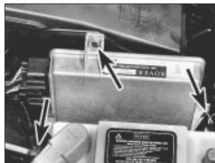
15.21b . . . then undo ECU mounting nuts (arrowed) and remove unit
