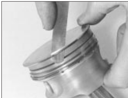
13.3 Removing piston rings with feeler blades
