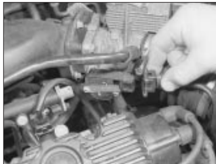
14.35 Disconnecting potentiometer multiplug - alloy inlet manifold
