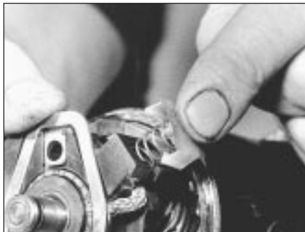
11.6b ... remove brush spring caps and springs ...
