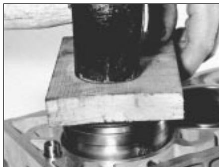
12.3 Tap liner onto locating shoulder - ensuring O-rings are not displaced
