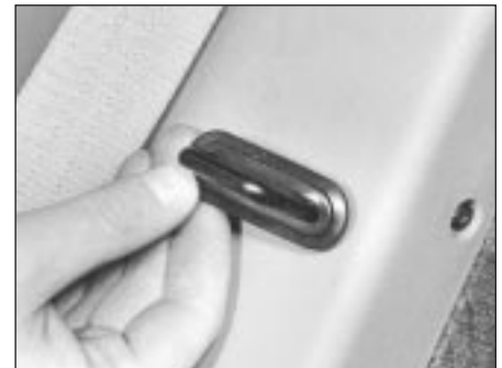
28.16b . . . and remove seat catch rubber seal
