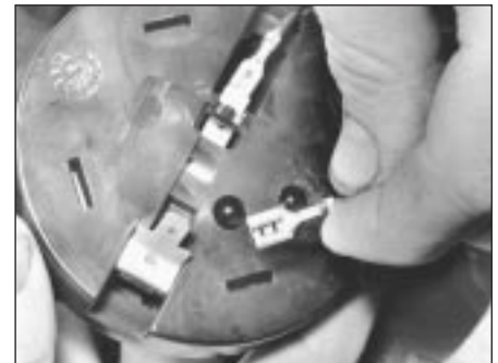
18.2b . . . and disconnect wiring from button terminals
