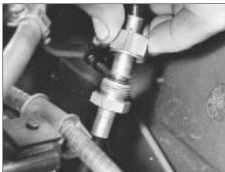
17.10 Slacken union nut and disconnect two speedometer cable sections
