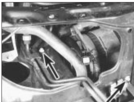
26.4a Power steering oil cooler upper mounting bolts (arrowed)
