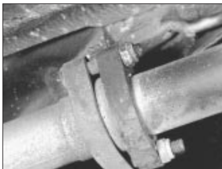
18.13 Tailpipe-to-intermediate flange joint
