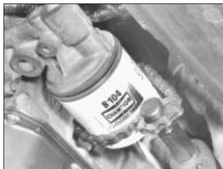
9.7 Using an oil filter removal tool
