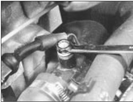
10.15a Unscrew cooling system bleed screw to allow trapped air to escape
