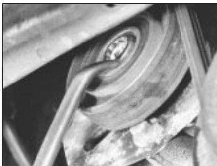
26.6a Slacken adjuster pulley spindle nut . . .
