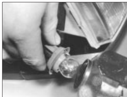
5.12 ... then withdraw indicator lamp and twist bulbholder free
