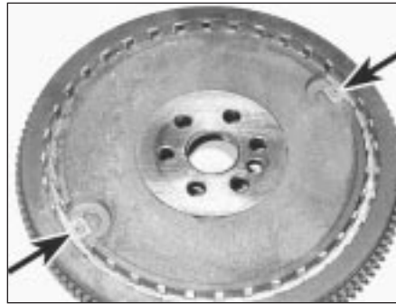
6.6 Reluctor ring-to-flywheel screws (arrowed)
