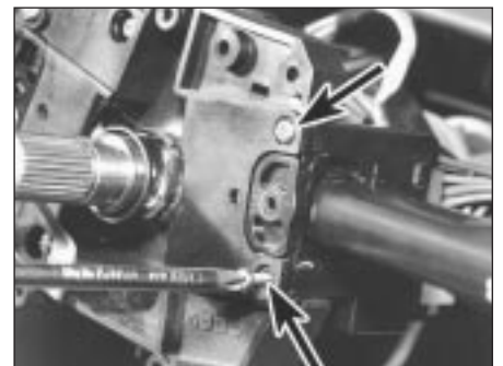
4.3a Individual combination switches can be removed by slackening retaining screws . . .
