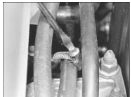
26.3 Slacken clamps and disconnect hoses from power steering oil cooler
