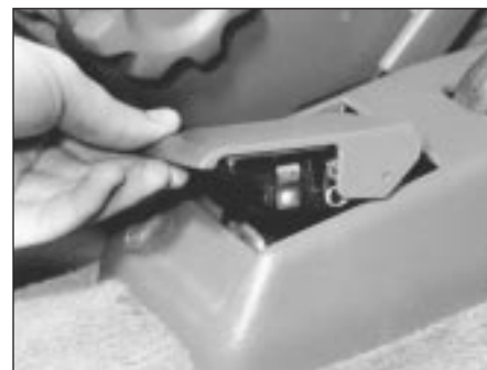
23.4a Remove ashtray from centre console . . .
