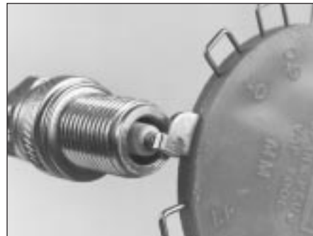
34.10c Adjusting a spark plug electrode gap with a special tool
