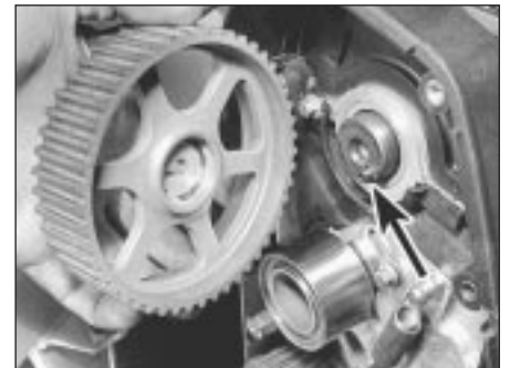
9.12 Removing camshaft sprocket (roll pin arrowed) - K8 engine
