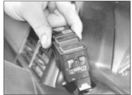
10.2b . . . then withdraw assembly and disconnect wiring connectors
