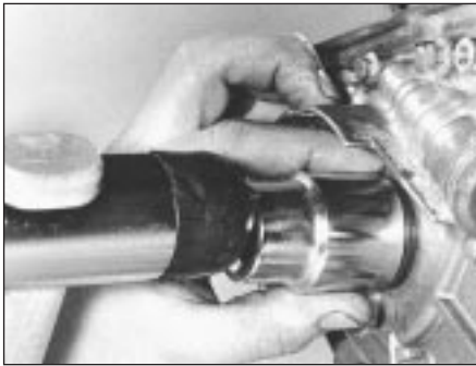
18.31b Fitting a new crankshaft right-hand oil seal
