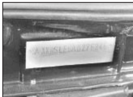
Vehicle identification number on engine compartment bulkhead
