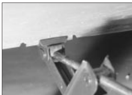
5 Locate the jack head in the correct jacking point
