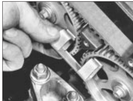
9.11b ... to fit sprocket spokes as closely as possible - K16 engine
