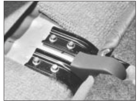
26.11 Rear seat back centre hinge retaining bolts - 214 models
