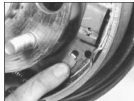
16.10 Ensure handbrake stop lever is correctly located
