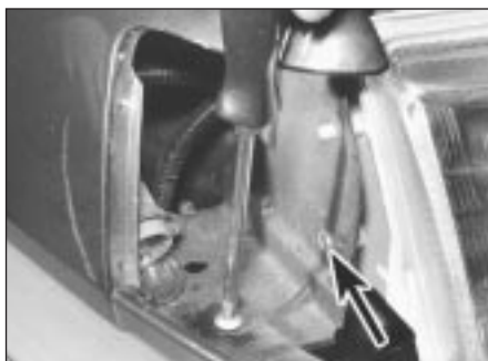
7.3a Remove headlamp retaining screws (remaining one arrowed) . . .
