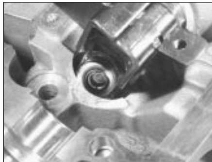
6.3a Using a valve spring compressor to release split collets
