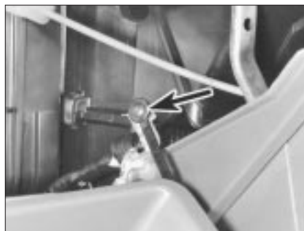
10.15 Glovebox damper retaining screw (arrowed)
