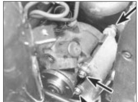
25.5a Unscrew power steering pump mounting bolts (three arrowed) . . .
