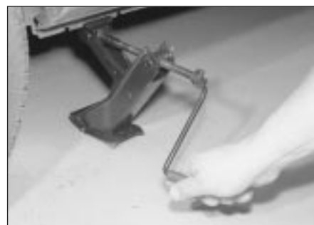
6 Raise the jack until the wheel is clear of the ground
