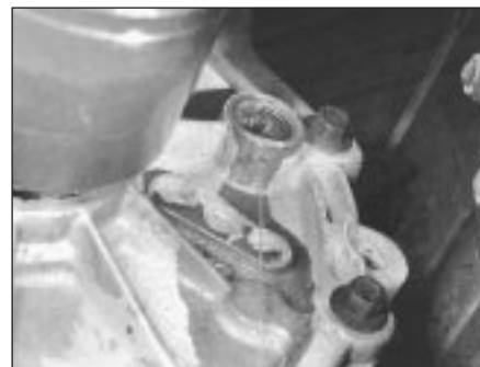
17.3 Gearbox oil level is correct when oil has just stopped trickling from filler/level plug hole
