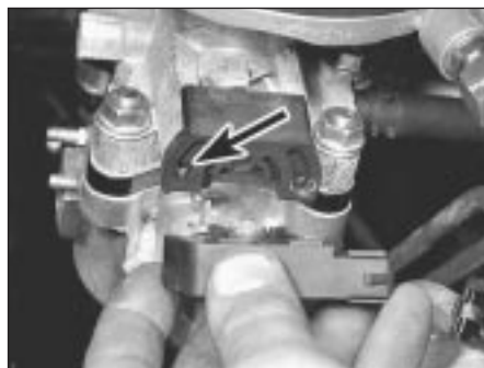
15.19 Ensure potentiometer tongue engages correctly with throttle lever (spacer arrowed)
