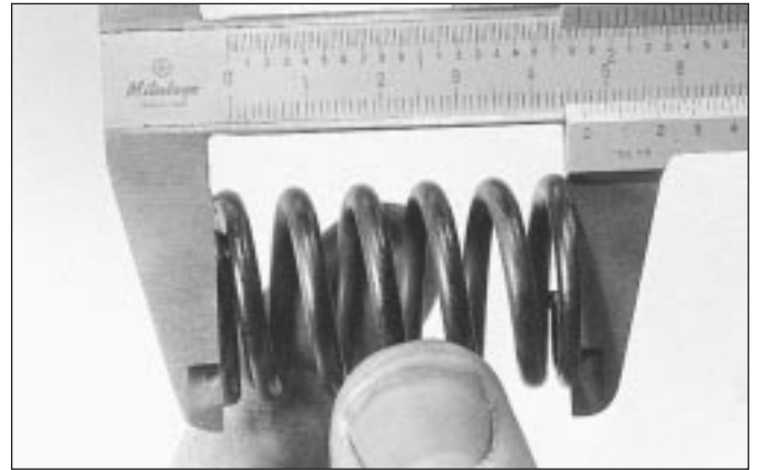
7.19 Measuring valve spring free length
