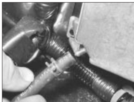
15.21a . . . and absolute pressure sensor vacuum hose from ECU . . .
