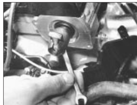
15.9 Removing distributor rotor arm grub screw - fuel-injected engines
