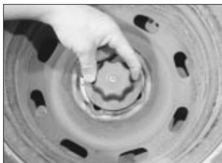
2 Unscrew the spare wheel retaining cap
