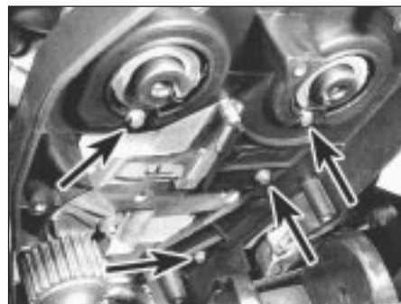
7.9b Timing belt upper left-hand (inner) cover fasteners (arrowed) - K16 engine
