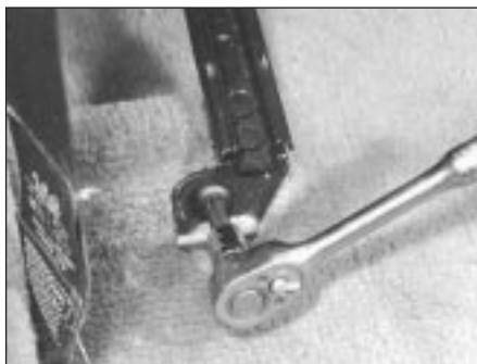
26.1 Front seat slides are secured to floor by Torx bolts
