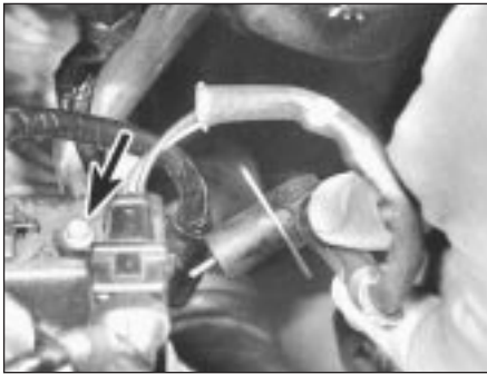
6.3 Removing crankshaft sensor (wiring lead screw arrowed)
