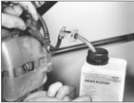
6.21 Using a one-way valve kit to bleed braking system
