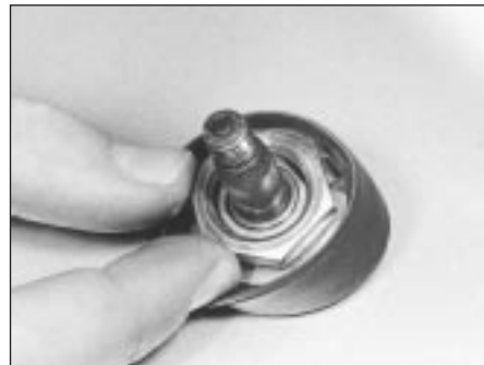
23.4a Unscrew wiper spindle retaining nut . . .
