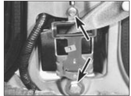
28.4 Front seat belt inertia reel retaining bolts (arrowed)
