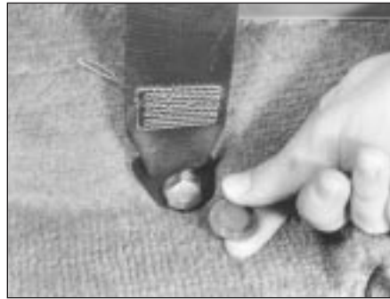
28.3 Prise off trim cap and remove front seat belt lower mounting bolt
