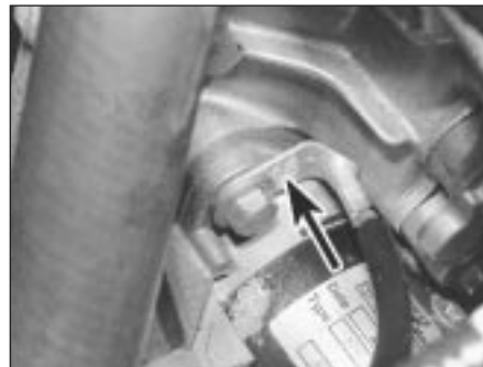
10.6b Starter motor upper mounting bolt and earth strap (arrowed) - viewed from above
