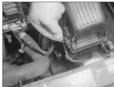
31.4a Release air cleaner cover securing clips . . .
