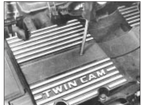
34.2 Remove spark plug cover . . .
