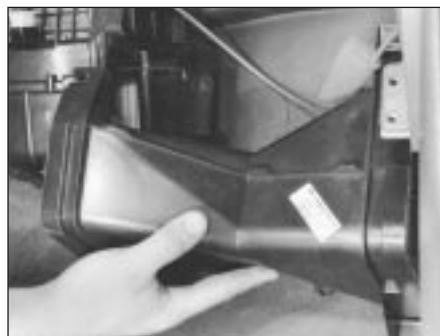
10.17 ... then remove blower motor-to-heater unit duct
