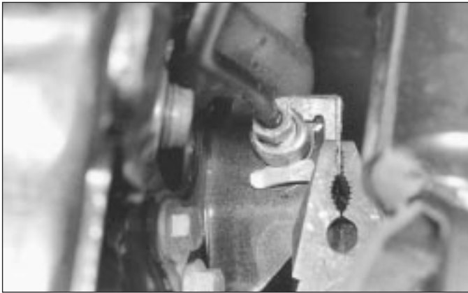
16.3 Remove retaining clip and free brake hose from trailing arm
