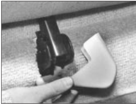
26.7 Remove seat cushion hinge covers to gain access to retaining bolts - 214 models
