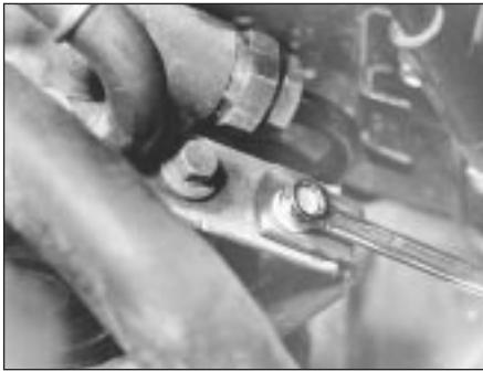
25.2b Remove outlet pipe bracket retaining bolt . . .
