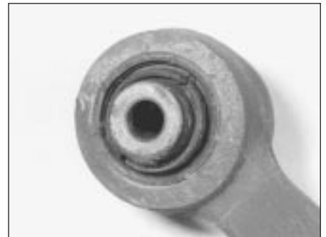
15.7 Examine lateral link bushes for signs of wear and renew if necessary
