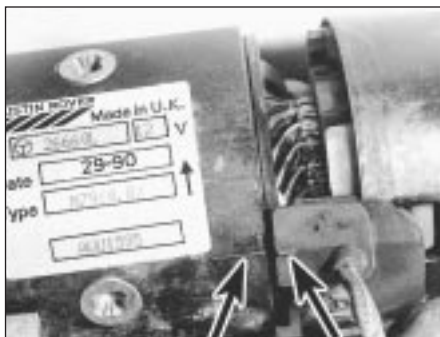
11.4a Note alignment marks between yoke and grommet ...
