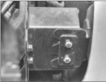
7.4 Front bumper mounting plate-to-bracket bolts
