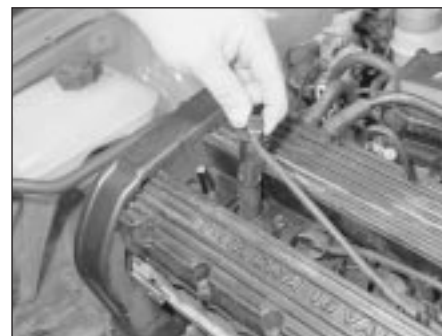
15.2 Pull each spark plug lead by gripping its end fitting
