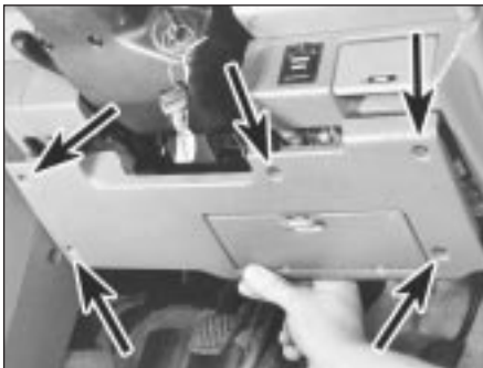
14.6 Remove retaining screws (arrowed) and withdraw right-hand lower facia panel
