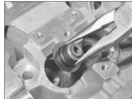
6.3b Extracting a valve spring bottom seat/stem seal
