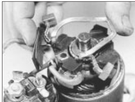
11.6c ... and remove positive brush assembly from motor
