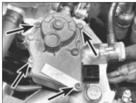
15.13a Undo stepper motor retaining screws (arrowed) . . .
