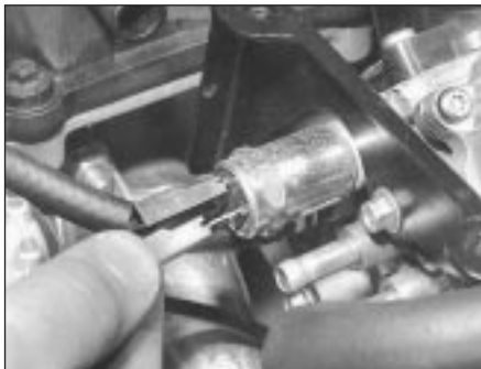
13.7 Note connections before disconnecting idle bypass solenoid wiring
