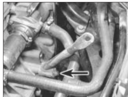
16.11b Inlet manifold support stay lower end bolt (arrowed)
