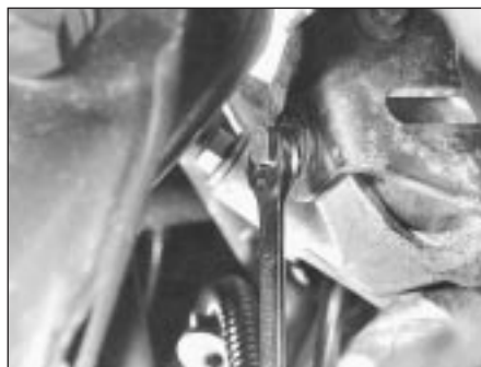
26.6b . . . and rotate adjuster bolt until power steering pump drivebelt tension is correct
