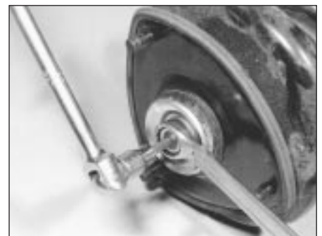
6.3 . . . and remove upper mounting nut whilst retaining piston with Allen key
