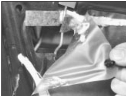
15.7 Carefully peel back polythene watershield to gain access to regulator components
