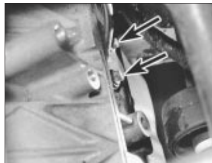
9.6a Dipstick tube mounting bolts (arrowed)
