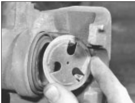
11.3 Removing circular shim from caliper piston
