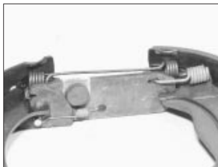
16.6 Correct fitted positions of adjuster strut and springs
