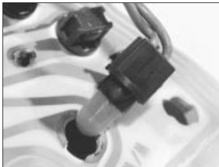
6.13a Instrument panel illumination bulbholder is a twist fit in panel . . .
