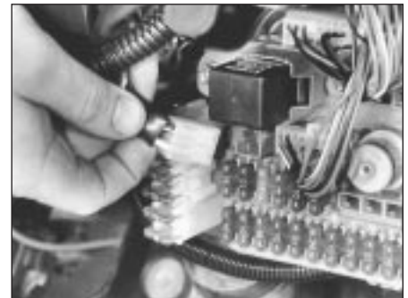
14.7b . . . and disconnect wiring connectors from front of fusebox
