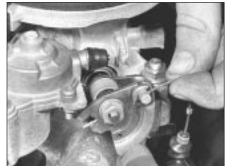
11.2 Disconnecting accelerator cable from throttle cam pulley
