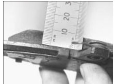
11.5 Measuring thickness of brake pad friction material
