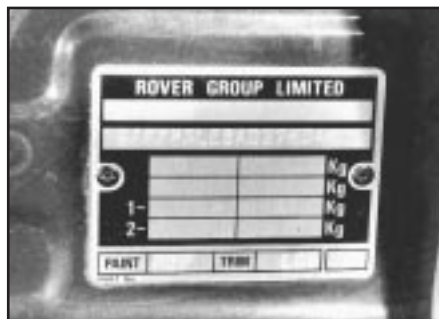
Vehicle identification plate on passenger door pillar
