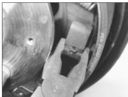
16.5b Remove brake shoe retainer springs...
