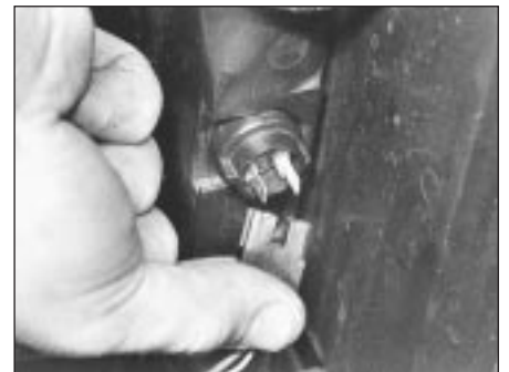
5.4b Disconnecting wiring connector from radiator switch
