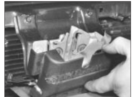
11.2 Remove plastic bonnet lock cover ...
