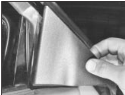
16.3 Remove mirror inner trim panel . . .
