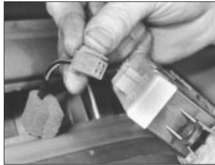
13.2b . . . and disconnect clock wiring connector
