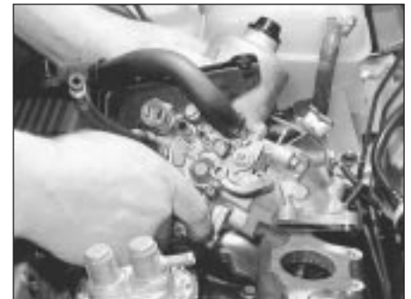
13.8b . . . and remove carburettor assembly
