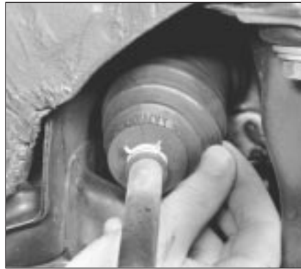
24.2 Checking a steering gear rubber gaiter
