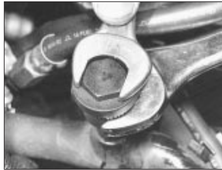
10.15b Unscrewing filler cap bolt whilst retaining filler stem with an open-ended spanner
