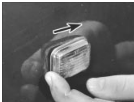
5.15 Push indicator side repeater lamp to right ...
