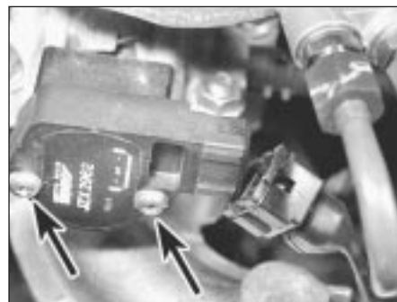
15.17 Disconnecting throttle potentiometer wiring connector (mounting screws arrowed)
