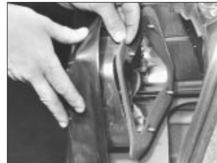
7.15 Withdraw rear lamp unit noting rubber seal
