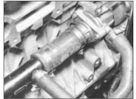
6.10 Thermostat housing and coolant hoses refitted
