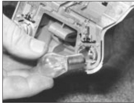
5.20c . . . whereas all other bulbs have bayonet type fitting
