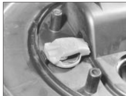
4.9 Thermac switch is clipped into air cleaner assembly
