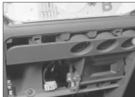
4.13c . . . and withdraw the switch panel surround
