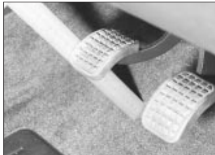
10.2 To check the clutch pedal stroke, measure the clutch pedal travel as described in the text
