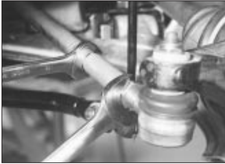
21.11 Adjusting the front wheel toe setting
