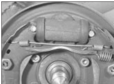
5.4 Upper return spring location (DBA Bendix type)
