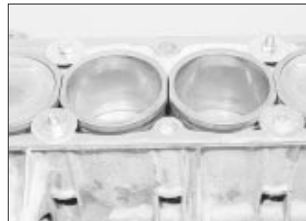
8.17 Cylinder liners clamped with washers and bolts
