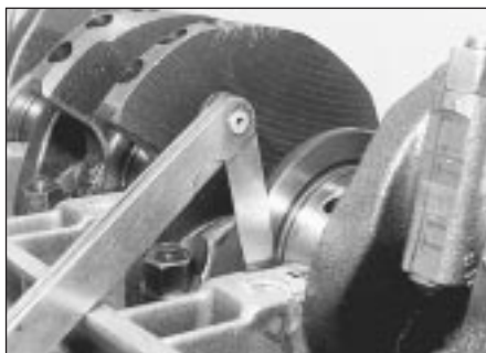
8.7 Checking crankshaft endfloat using feeler blades
