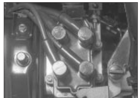
6.5 HT lead connections on the static distributorless ignition module
