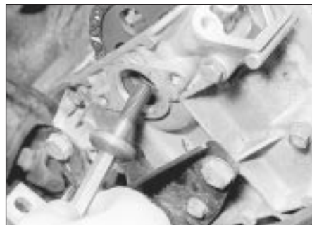
7.23 Unscrew and remove the camshaft sprocket bolt
