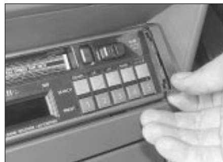
22.6 Removing the radio side trims on later models
