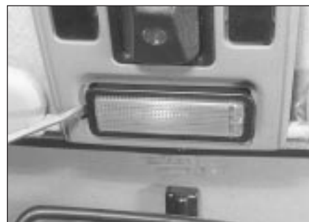
9.3 Prise out the interior light for access to the bulb
