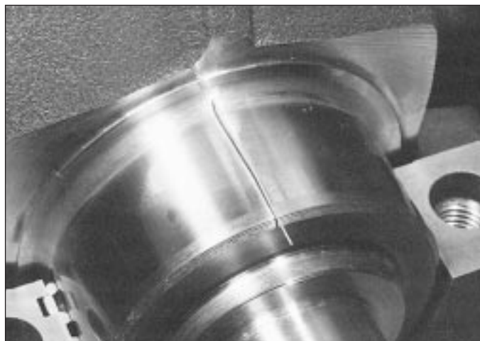
13.26 Plastigage in place on a crankshaft main bearing journal
