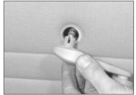
11.4 Removing the window regulator handle
