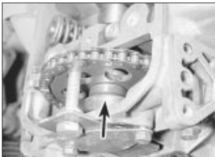
7.29 Slide the camshaft from the fuel pump eccentric (arrowed)
