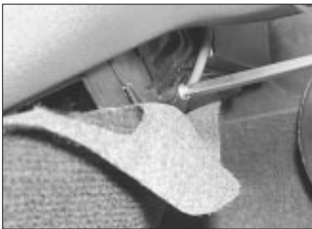
26.31 Prise out the console vent and remove the screw
