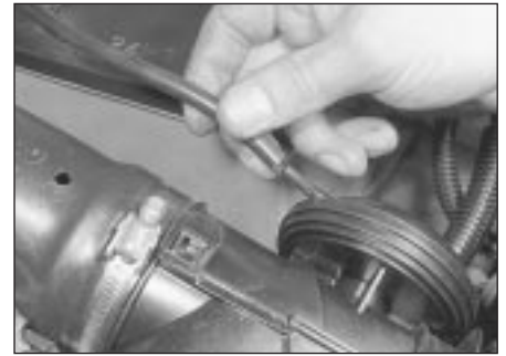
2.9 Disconnect the hose from the vacuum motor
