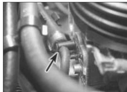
11.25 Vacuum hose connection to throttle body (arrowed)
