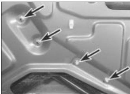
12.2a Window regulator mounting nuts (arrowed)
