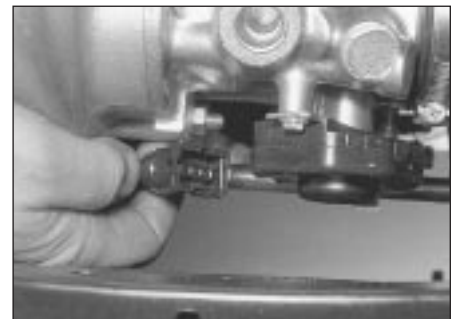
10.14 Removing the throttle switch connector
