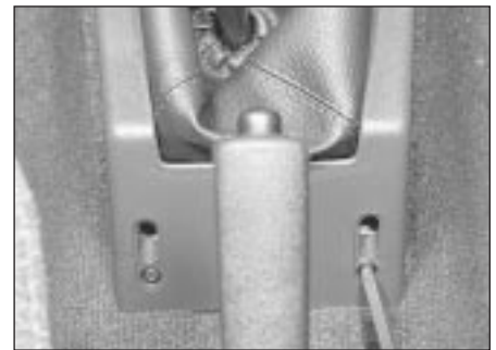
26.33 Remove the screws and slide the surround up the gear lever
