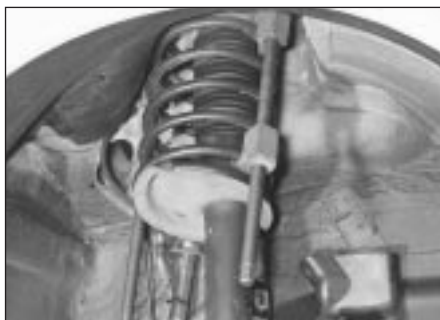
4.1 Coil spring compressors fitted to strut spring
