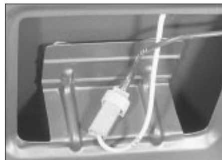
16.4a Tailgate wiper motor wiring connection . . .
