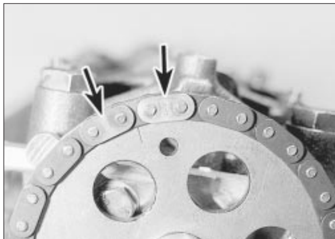
4.21 Camshaft sprocket timing mark (arrowed) positioned between two bright links (arrowed) on chain
