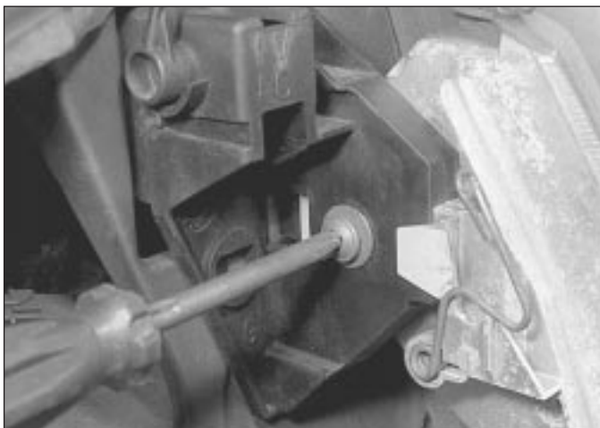
11.3a Remove the headlight adjustment assembly screw . . .
