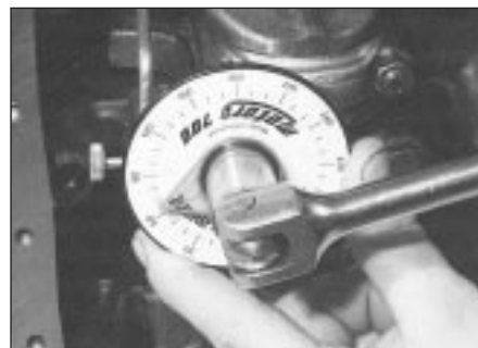
14.23 . . . and further, on XU series engines, through the specified angle using an angle tightening gauge
