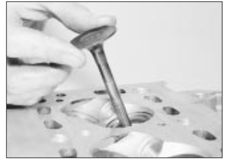
6.6 Withdraw the valve through the combustion chamber
