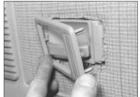
11.5 Removing the interior door handle surround
