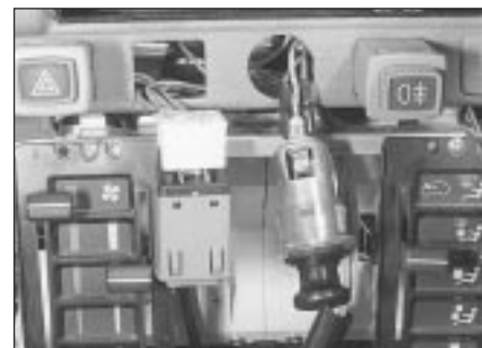
4.7 Heated rear window switch and cigar lighter removed from facia
