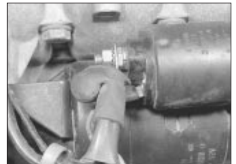
9.4 Starter motor solenoid wiring
