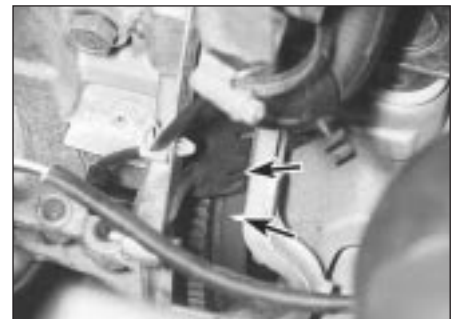
8.25b . . . to reveal the timing plate and flywheel timing mark (arrowed)
