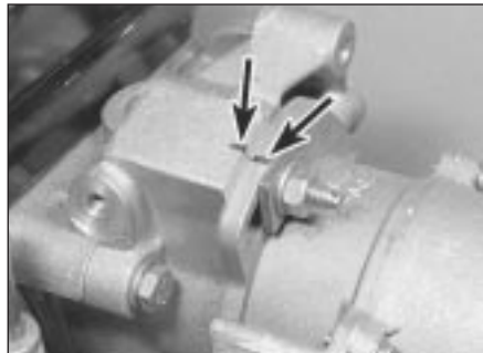
4.17 Mark the distributor and housing . . .
