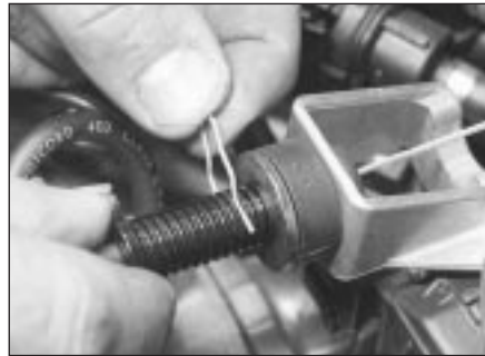
3.3 Adjust the throttle cable as described in text
