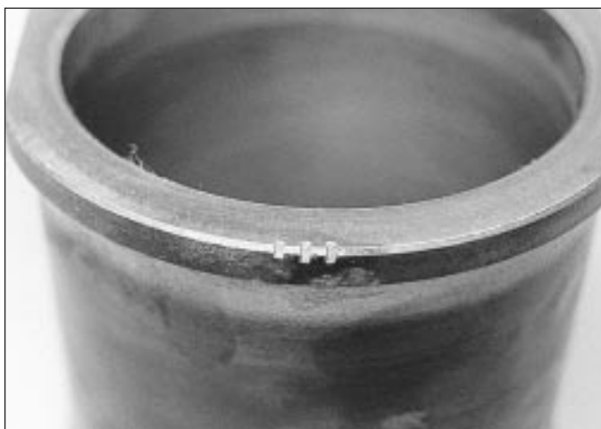
9.18 Cylinder liner size group marking
