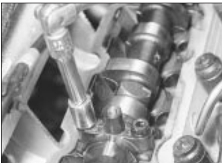
7.7 Progressively unscrew the camshaft bearing cap nuts . . .
