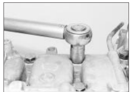
13.45 Tightening the main bearing/casing bolts
