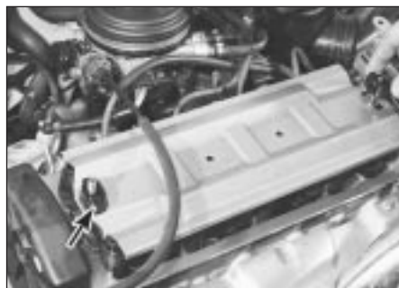
4.6a Lift off the spacers (second one arrowed) . . .
