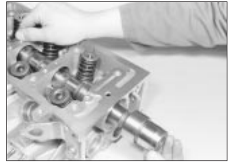
10.9b . . . and slide out the camshaft
