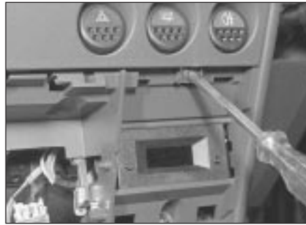
26.27b Remove the lower screws and withdraw the surround
