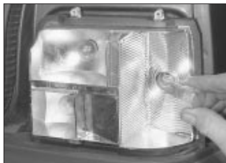
8.19 Removing a rear light cluster bulb
