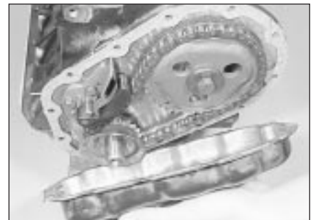
14.21 Refitting the timing cover
