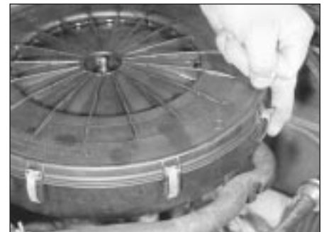
24.1b . . . and release the retaining clips . . .
