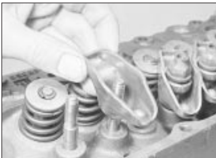
9.24a Fitting a rocker arm . . .
