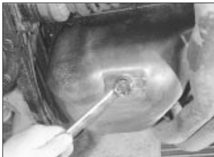
6.4 Removing the sump drain plug
