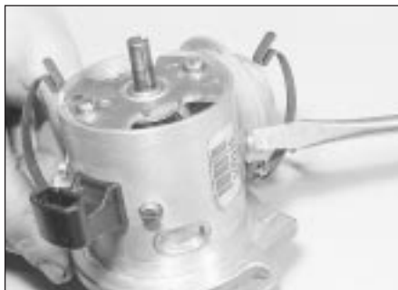
4.16a Removing a vacuum unit retaining screw
