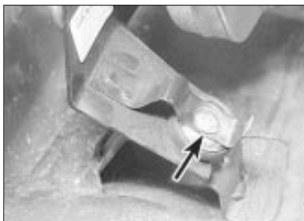
20.7 Wiper motor securing screw (arrowed)
