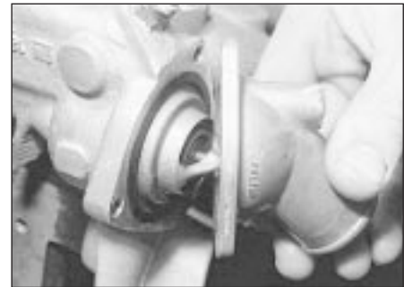
4.9a Removing the thermostat cover . . .
