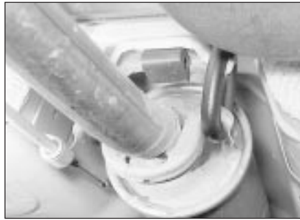
27.4b Exhaust system rubber mounting ring
