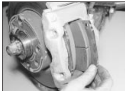
4.6 Removing the inboard pad
