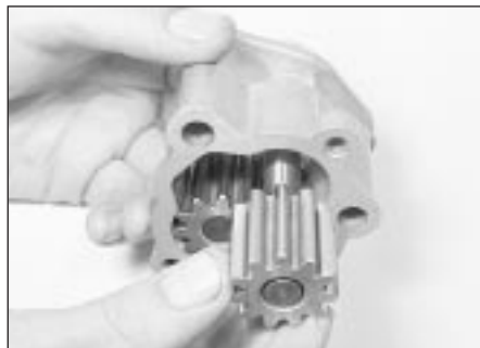
13.3a Removing the oil pump driving gear . . .
