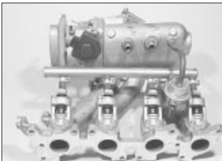
13.11b Inlet manifold showing injectors fuel rail and associated components
