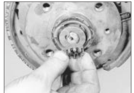
10.6b . . . the washer and the castellated nut
