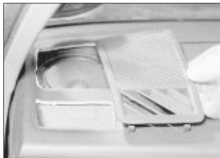
10.1 Removing an end grille and speaker
