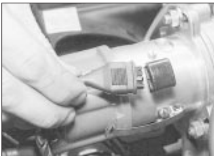
3.6a Unplugging the distributor LT connector (1.6 litre carburettor model shown)
