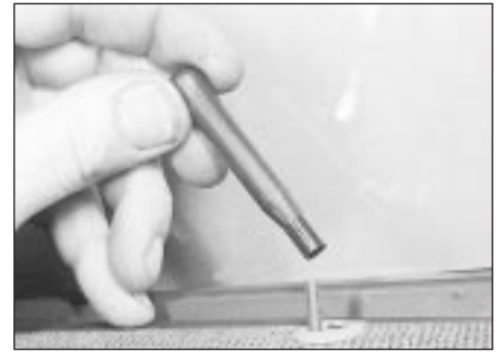
12.4 Unscrewing the lock button
