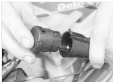
23.9a Engine wiring harness plug
