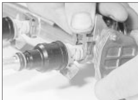
12.69a Remove the retaining clip
