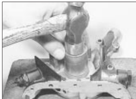
14.6 Fitting a new front oil seal
