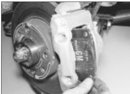
4.5 Removing the outboard pad
