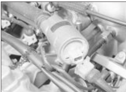
12.44a Disconnect the idle speed adjuster multi-plug . . .
