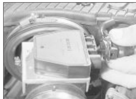
12.84 Disconnecting the multi-plug from the air mass meter
