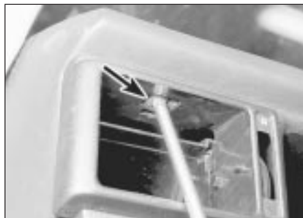
10.2 Removing a swivelling vent housing securing screw
