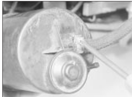
12.98b Disconnecting a hose from the canister
