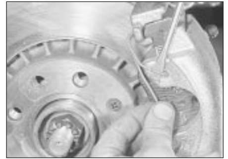
4.17 . . . then lever out the spring clip
