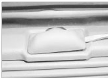
11.22 Prising out the number plate lamp
