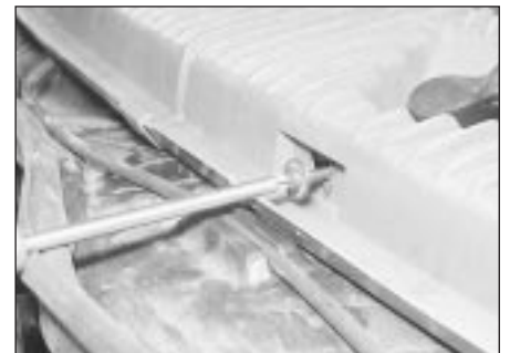
11.3b Wind deflector screw near the wiper
