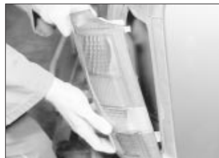
11.17b Removing a rear lamp lens
