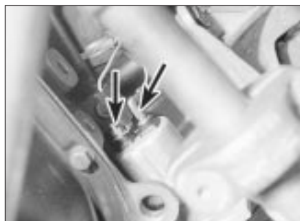
13.2 Oil pressure sender wires (arrowed)
