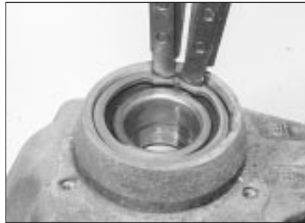
3.5b Removing a hub bearing circlip
