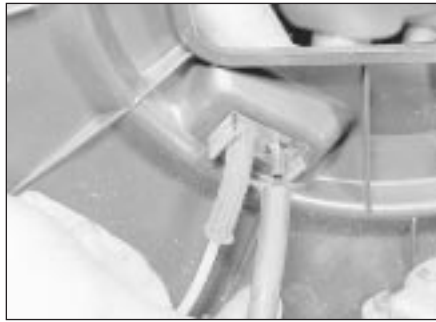
3.2b Air cleaner vacuum hose connection
