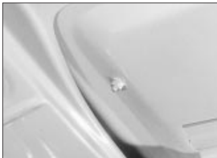
26.9 Boot lid handle retaining nut
