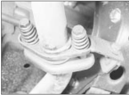
27.4a Exhaust system flexible joint
