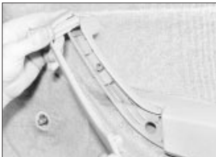
12.6a Removing the armrest screw cover
