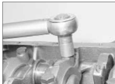
20.16b Tightening a main bearing cap bolt
