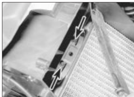
9.17b Heater matrix upper securing screws (arrowed)
