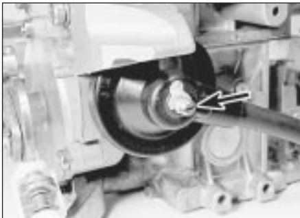
14.8a Choke valve gap adjustment screw (arrowed)
