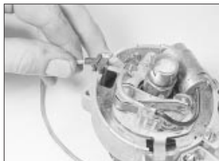
7.3 Removing the LT lead
