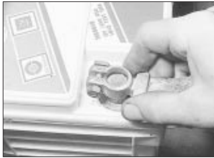
4.2 Disconnect the battery negative terminal first
