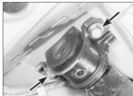
5.4 Control arm clamp bolts (arrowed)
