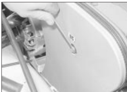
7.6a Removing a belt cover bolt . . .
