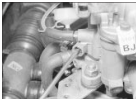
11.4c Adjusting the idle speed - Varajet carburettor
