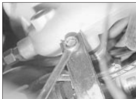
11.8 Unbolting the inlet manifold support bracket (seen from below)
