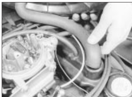
7.4 Removing the breather hose from the rocker cover
