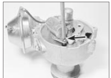
7.5 Undoing the condenser retaining screw
