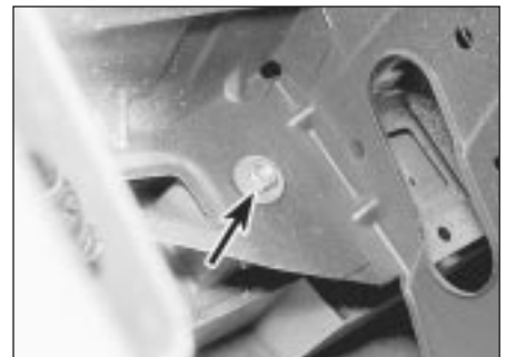
8.3 Front trim panel securing nut (arrowed)
