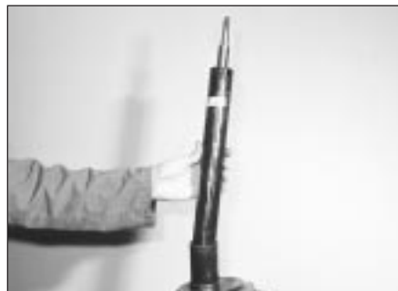
4.7 Removing the shock absorber cartridge
