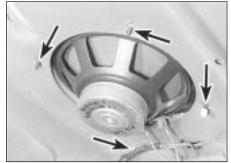
26.2b . . . the speakers are retained by four screws
