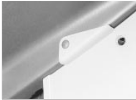
9.4b Heater control panel side screw
