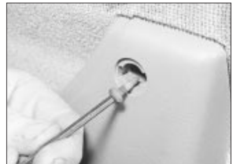
12.5b Removing a door pocket screw
