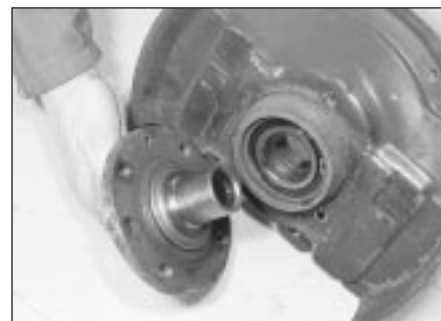
3.3b Hub removed from the carrier
