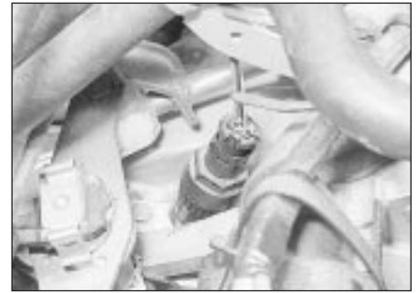
25.22 Speedometer sender (used with digital instrument panel)
