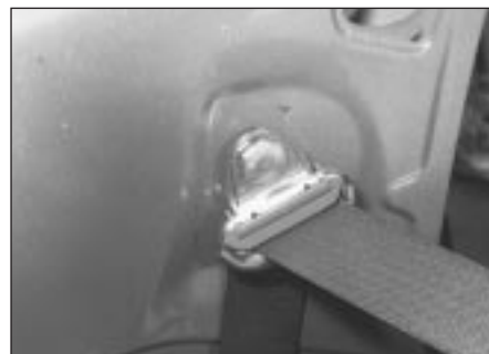
37.7b Rear seat belt upper mounting
