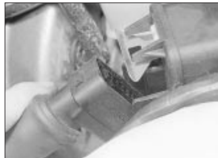
7.7 Disconnecting the control unit wiring plug - later 1.8 litre model
