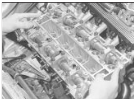
11.20 Lifting off the cylinder head
