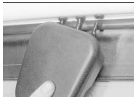
21.9 Removing the window-mounted motor
