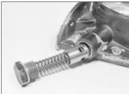
14.5 Oil pressure regulator valve components
