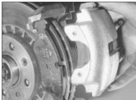
4.20 Lift the caliper off the disc . . .
