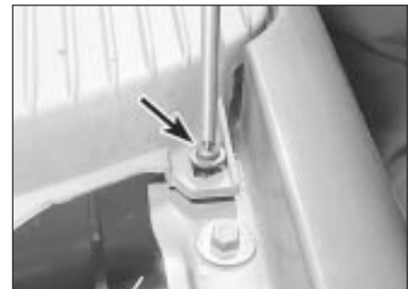
11.3a Wind deflector screw at the wing
