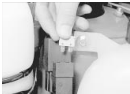
3.7b Removing the headlamp washer fuse
