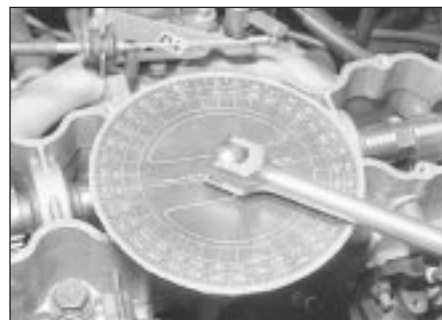
8.26b Using a marked card to measure angular rotation when tightening cylinder head bolts
