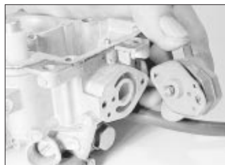
21.6 Removing the part-load enrichment device
