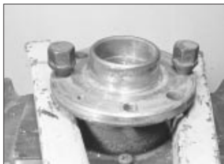
3.3a Removing the hub from the carrier
