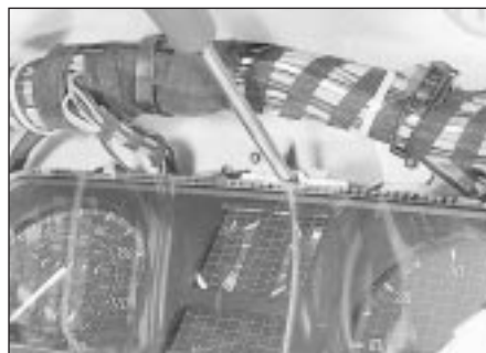
8.7a Removing the instrument panel securing screw
