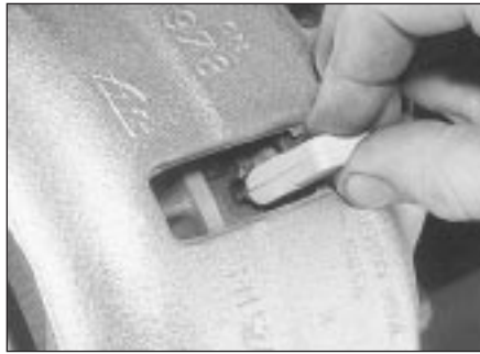
4.16 On later ATE type calipers, unclip the pad wear sensor . . .
