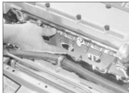
14.8 Fitting a new exhaust manifold gasket
