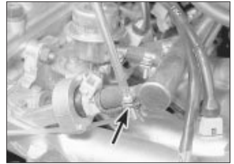
12.6 Slackening a fuel rail hose clamp
