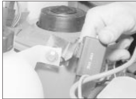
12.36a Removing the control relay and bracket
