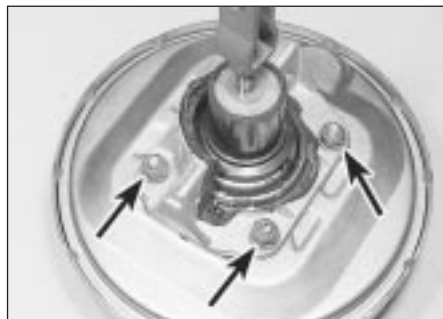
16.9 Three of the four servo-to-bracket nuts (arrowed) servo and bracket removed for clarity
