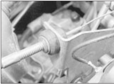
8.3 Accelerator cable bracket and bush
