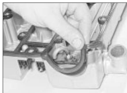
11.25 Fitting a new gasket to the camshaft cover
