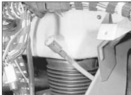
10.2 Speedometer cable at instrument panel end
