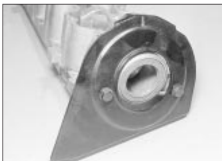
9.7 Camshaft belt cover backplate (1.3 litre engine shown)
