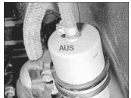
25.4 Fuel filter directional marking
