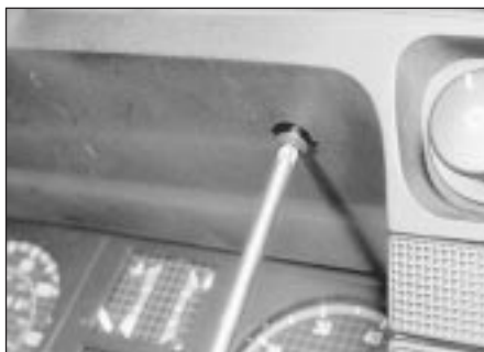
8.4 Removing an instrument panel surround screw
