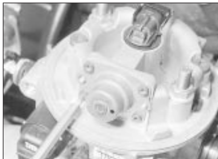
11.17a Undo the retaining screws ...
