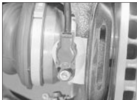
22.2b ABS front wheel speed sensor
