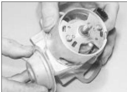
4.16b Removing the vacuum unit
