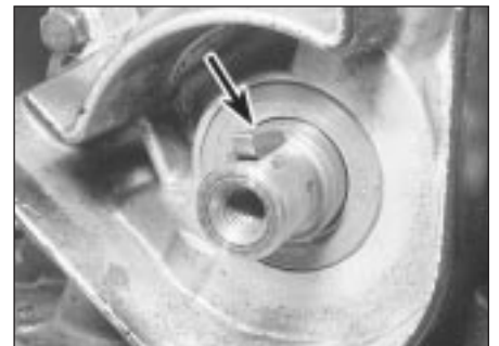
13.2b Woodruff key (arrowed) in crankshaft nose
