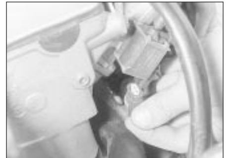
12.100 Disconnecting the vent valve multi-plug
