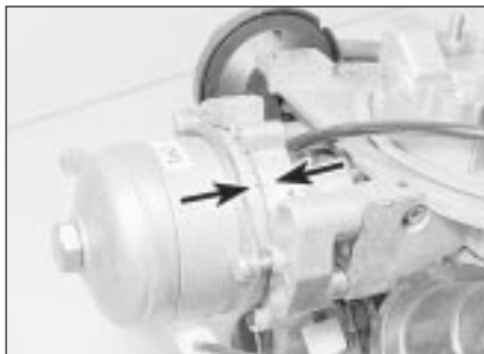
15.12 Choke cover alignment marks (arrowed)
