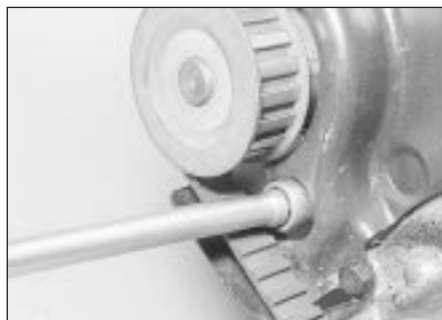
7.8 Slackening a water pump bolt
