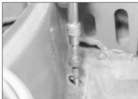
16.8 Removing a servo bracket screw
