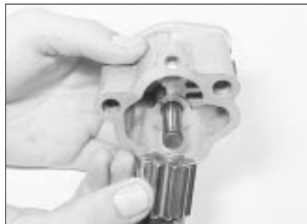
13.3b . . . and the driven gear
