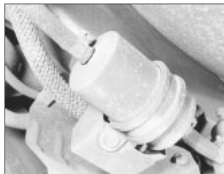
25.3 Fuel filter showing mounting and hose connections
