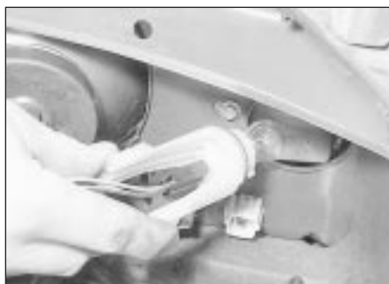
11.9 Removing a direction indicator bulb and holder
