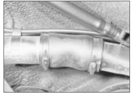
7.11 Fuel tank filler pipe-to-neck junction
