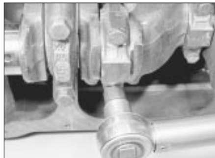
15.14b Tightening a big-end bearing cap bolt
