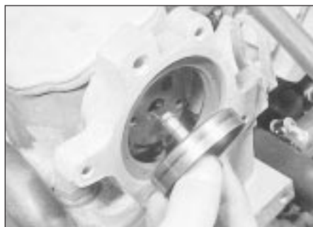
3.11a Extract the rotor hub . . .
