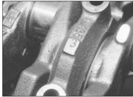
20.3 Identification number on No 3 main bearing cap
