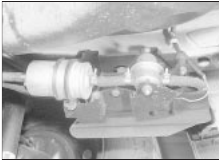
7.6 Fuel pump, damper and filter assembly
