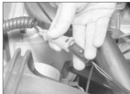
23.9b Dipstick sensor plug
