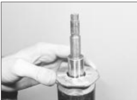
4.6b Removing the strut ring nut
