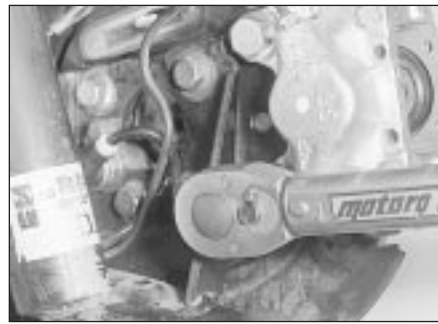
11.10 Tighten the rear caliper mounting bolts to the specified torque setting
