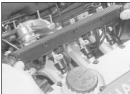
12.66b Lifting the wiring rail off the injectors
