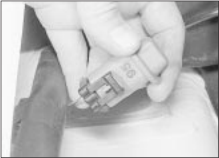
2.10 Octane plug in the "95" position - later 1.6 litre models
