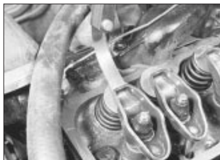
7.10 Checking a valve clearance
