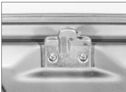
26.2 Boot lid lock securing screws
