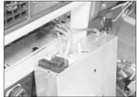
25.2b Removing the radio from its aperture
