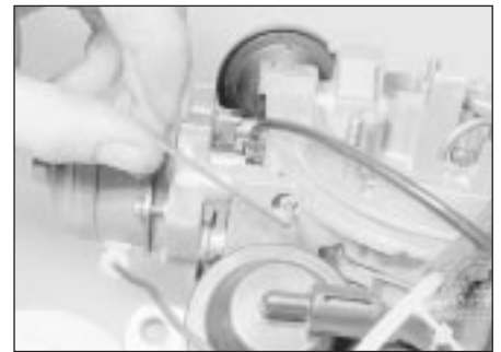
15.9b Choke pull-down adjusting screw
