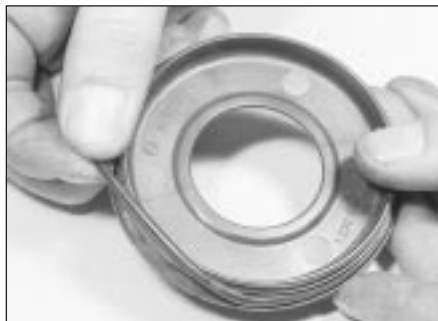
3.27 Renewing the insulator sealing ring
