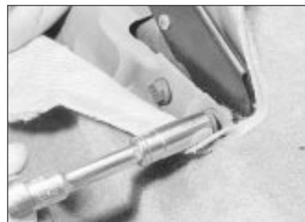
19.5 Unbolting the handbrake lever
