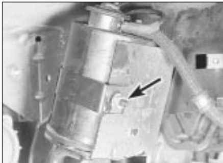
12.98a Canister clamp nut (arrowed)
