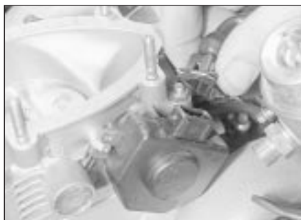
12.82 Disconnecting the throttle valve switch multi-plug
