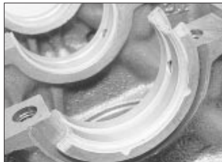
20.12 Centre main bearing shell, showing thrust flanges
