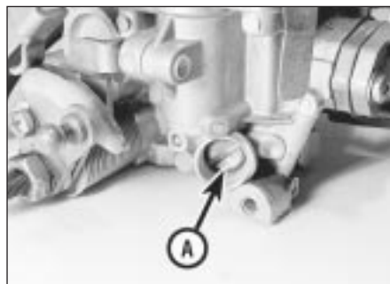
11.4d Idle speed adjusting screw (A) - 1B1 carburettor
