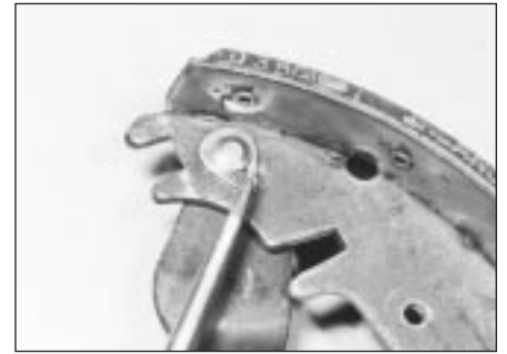
6.16 Handbrake lever secured by pin
