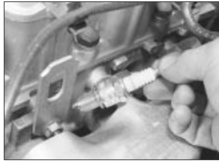
7.5 Removing a spark plug - 1.6 litre engine shown
