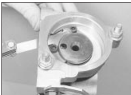
9.10 Checking the camshaft endfloat
