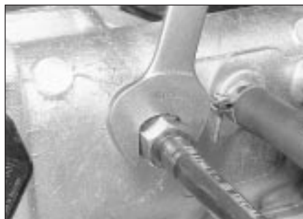
15.2 Brake servo vacuum connection at inlet manifold (fuel injection model)
