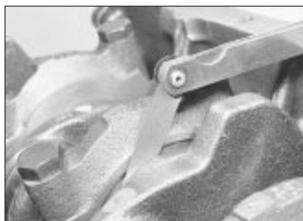
20.19 Checking crankshaft endfloat
