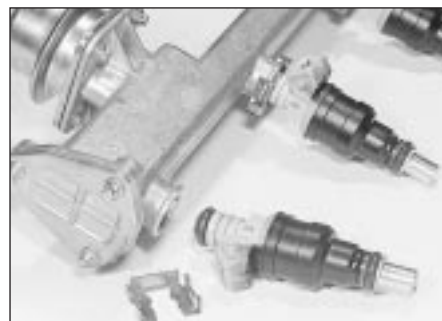
12.69b . . . and pull out the injector
