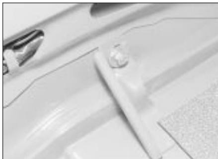
9.2 Rear trim panel securing nut
