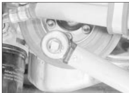
7.14 Tightening one of the crankshaft pulley screws
