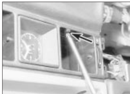
10.3 Removing a centre vent housing screw
