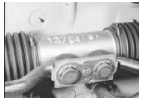
27.4 Tie-rod connection to steering rack
