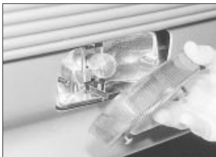
11.19 Removing a rear foglamp lens
