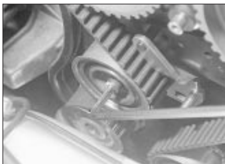
7.10 Slackening the camshaft belt tensioner screw
