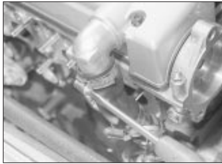
11.15 Disconnecting the large breather hose
