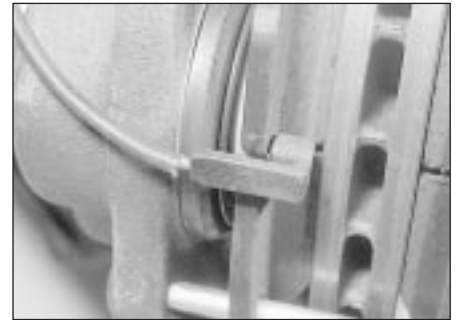
4.4b Wear warning sensor clipped to pad
