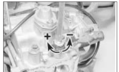
15.23 Accelerator pump delivery adjustment: + to increase, - to decrease
