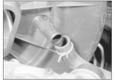
3.2c Air cleaner hose connection
