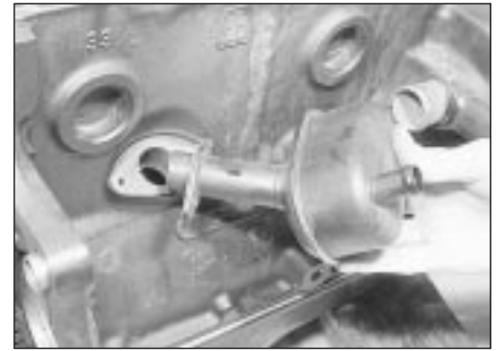
22.8 Crankcase ventilation system oil separator - 1.3 litre engine
