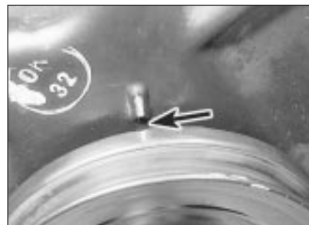
7.7 Ignition timing marks (arrowed) in alignment
