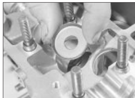
12.6e ... and the valve spring seat
