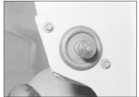
33.5a Seat backrest catch striker - Hatchback
