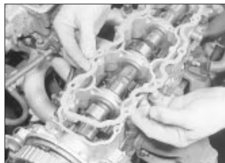
8.29a Fitting a new camshaft cover gasket
