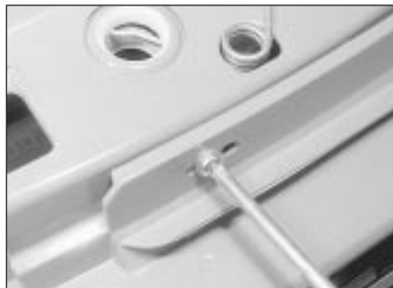
8.2 Undoing a front trim panel screw
