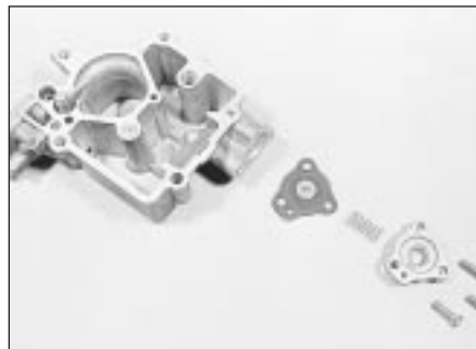
19.10 Enrichment valve components
