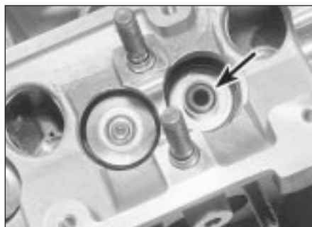
12.6d ... the valve stem oil seal (arrowed) ...
