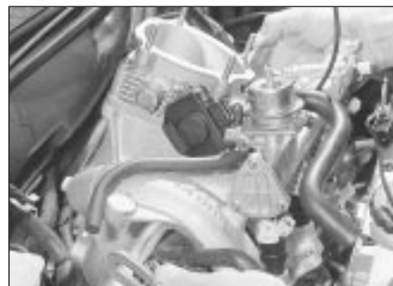
13.32 Removing the inlet manifold - 2. litre 16-valve model
