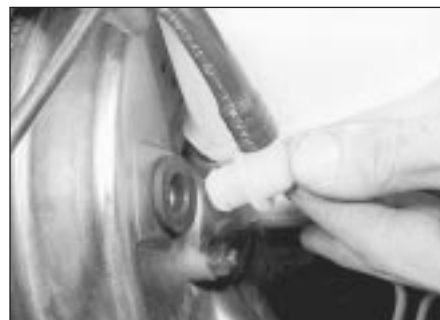
15.3 Brake servo vacuum connection at servo
