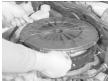
24.2a . . . then lift off the air cleaner lid . . .
