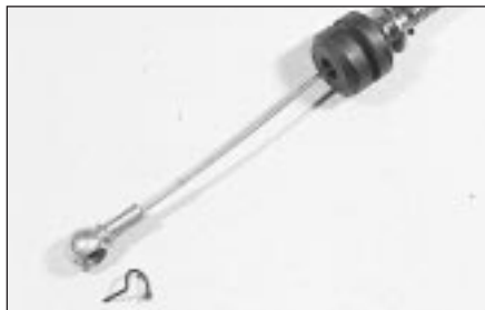
13.9 Accelerator cable at engine end
