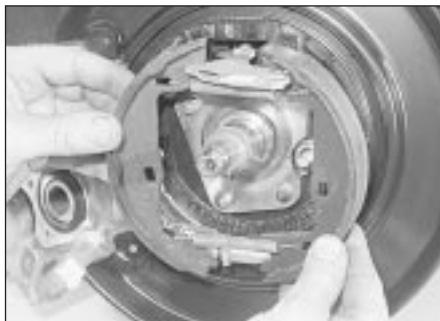
20.4 Removing the handbrake shoe assembly
