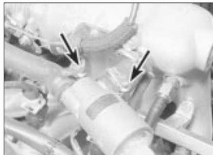
12.44b . . . and the air hoses (arrowed)
