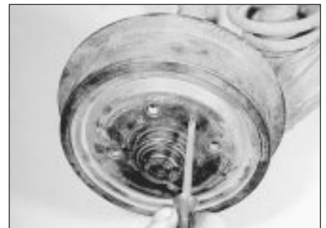
9.3a Removing a brake drum securing screw
