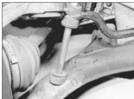
8.2 Front anti-roll bar end link
