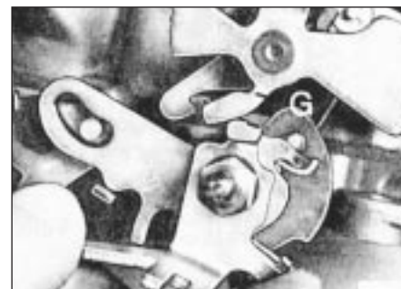
16.21 Full throttle opening adjustment - bend tang G to adjust choke gap
