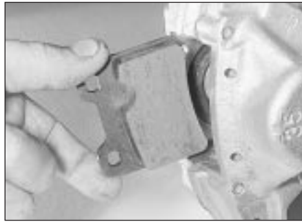
5.9a Fitting a rear pad
