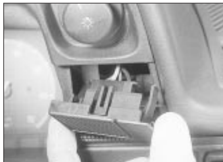
4.5 Removing a foglamp switch
