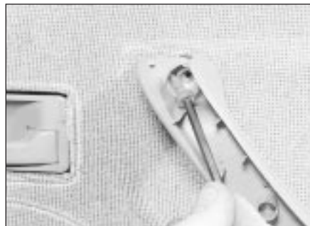
12.6b Removing an armrest screw
