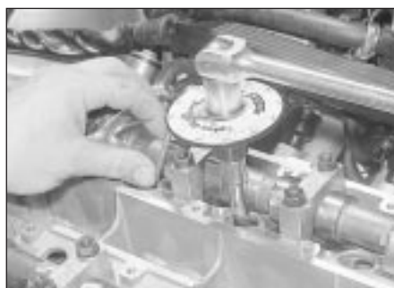
11.24b Angle tightening a cylinder head bolt
