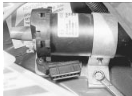
6.4a Removing a coil securing bolt
