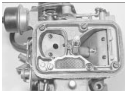
23.8 Varajet II carburettor top cover
