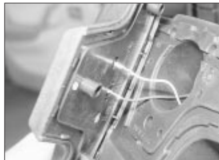
19.2 Removing the steering wheel central cap
