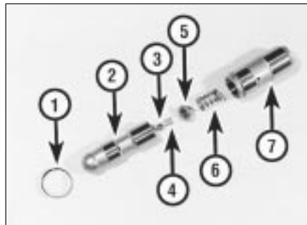
10.6 Hydraulic valve lifter components
