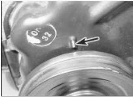
6.3 Ignition timing marks (arrowed) in alignment
