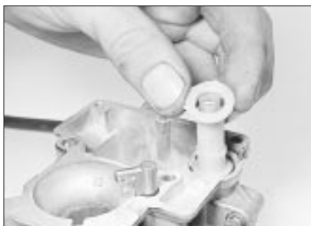
21.7a Removing the accelerator pump collar ...
