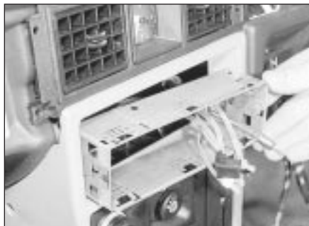
25.4 Removing the radio surround
