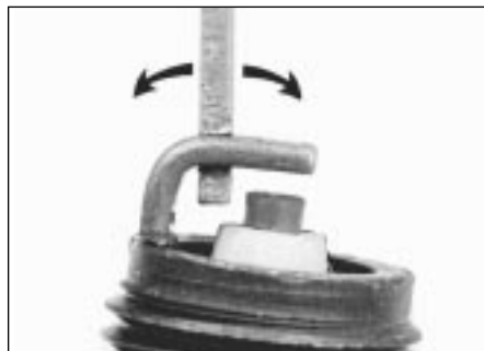
Adjusting spark plug gap
