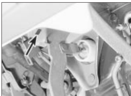
17.1 Stop-lamp switch 'keyhole' mounting (arrowed)
