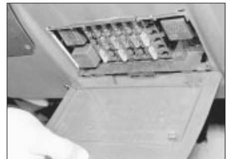
3.1 Removing the cover from the fuse/relay box
