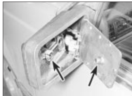
30.2b Engage the linkage and press the ball into the socket (arrowed)
