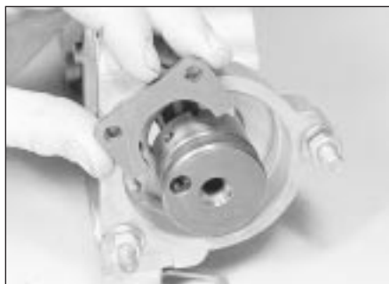
9.5b Removing the camshaft thrust plate
