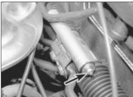
26.2 Steering damper securing nut (arrowed)
