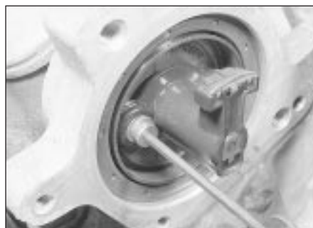
3.10a Undo the two Allen screws . . .
