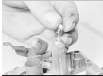
21.10 Removing the main jet
