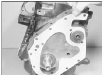
18.10 Fitting a new front plate gasket
