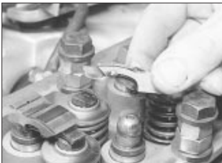
8.19 Removing a rocker arm
