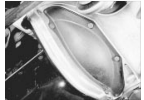
14.2 Clutch access plate
