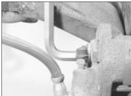
10.6b . . . then unscrew the caliper bolts . . .
