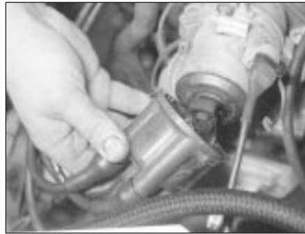
10.9a Remove the distributor cap . . .
