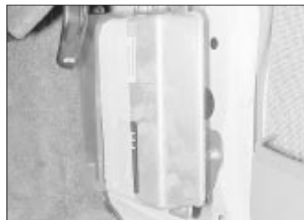
12.48 Motronic control unit location
