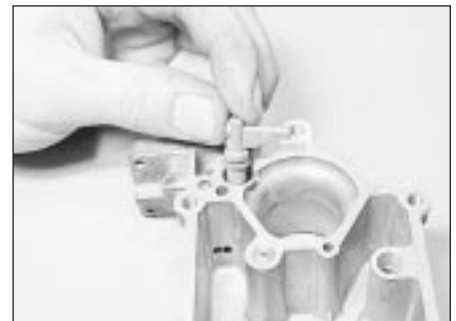
19.11 Removing the fuel discharge nozzle
