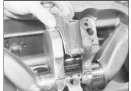
20.14 Fitting the centre main bearing cap
