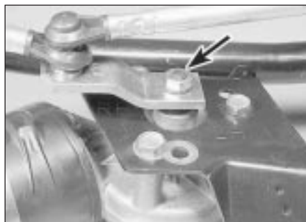
20.8a Wiper motor spindle nut (arrowed)
