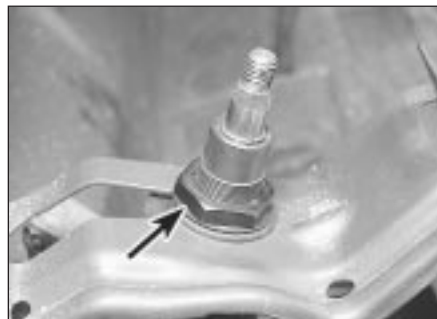
20.4 Wiper spindle clamp nut (arrowed)
