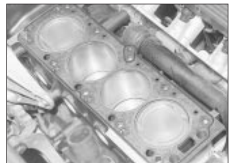
11.22 New head gasket in position
