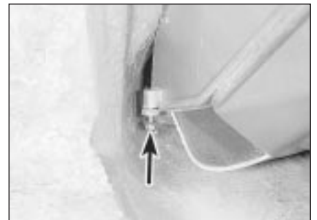
9.15b Air distribution housing lower screw (arrowed)
