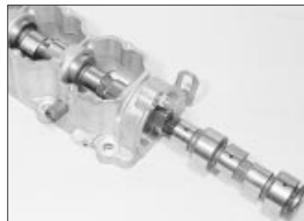
9.6 Removing the camshaft from the housing
