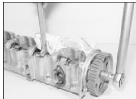
9.12b Tightening the camshaft sprocket bolt
