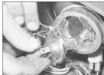
11.3 Removing a headlamp bulb
