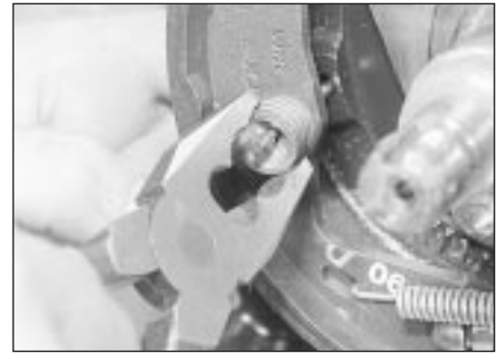
20.3a Removing a steady washer . . .
