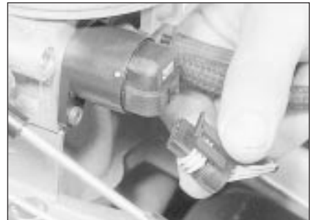
11.11a Detach the wiring connector ...
