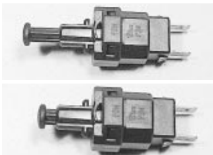
17.6 Stop-lamp switch plunger in extended position (top) and after fitting (bottom)
