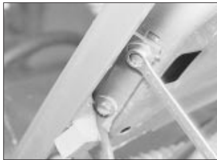
6.3 Removing a bonnet hinge bolt
