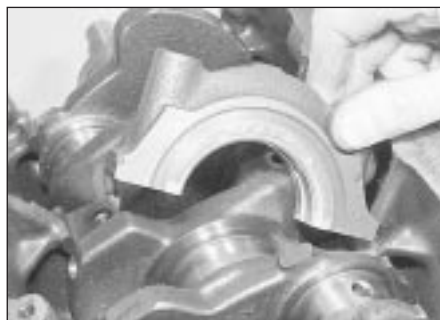
20.16a Fitting a main bearing cap
