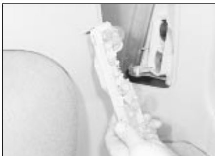
11.16b Rear lamp cluster bulbs and holder
