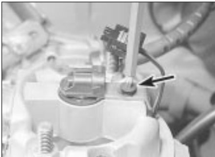
11.6b ... undo the retaining screw ...
