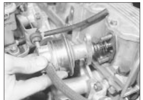
5.5 Removing the fuel pump (1.3 litre engine shown)
