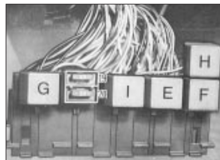
3.8b Fuse and relay identification (reverse side of fusebox)
