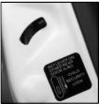
Your vehicle is equipped with rear door security locks that help prevent passengers from opening the rear doors of your vehicle from the inside. The rear security door locks are located on the inside rear doors.
