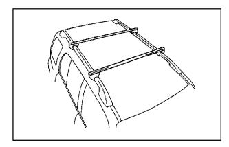
3. Mount the crossrails onto the side rails and adjust their position so the cargo can be mounted properly. Make sure the crossrails are not slanted.
