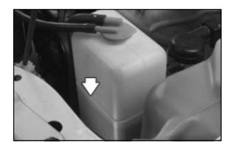
When the engine is cold, the coolant level should be at or above FULL. If it isn't, you may have a leak in the radiator hoses, heater hoses, radiator, water pump or somewhere else in the cooling system.
