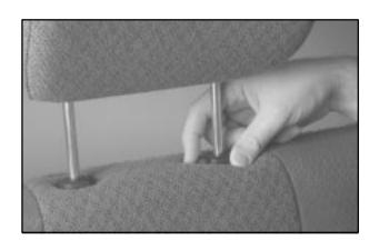
Remove the head restraint from the seatback by raising the head restraint fully. Push the release button and remove the head restraint from the seatback.
