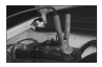
6. Connect the red positive (+) cable to the positive (+) terminal of the vehicle with the dead battery. Use a remote positive (+) terminal if the vehicle has one.
