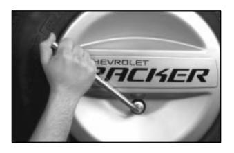
2. Using the wheel wrench, remove the wheel nut from the tire. Gently pry the spare tire cover off the wheel.
