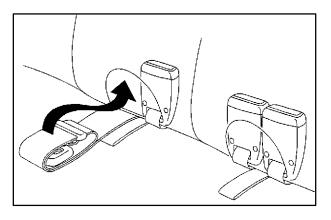
1. Fold the safety belt buckles and center safety belt (if equipped) into the pocket of the rear seatback.
