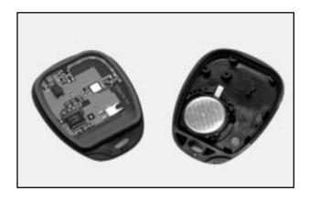
To replace the battery in the transmitter:
