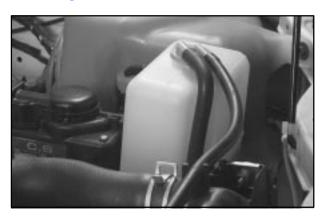
The vehicle must be on a level surface. When your engine is cold, the coolant level should be at LOW, or a little higher. When your engine is warm, the level should be up to FULL, or a little higher.
