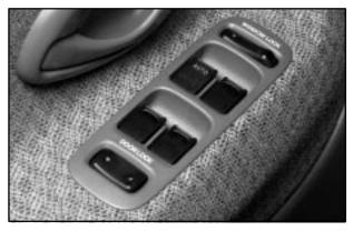
With power windows, switches on the driver's door operate each window when the ignition is on. Push down on the front of the switch to lower a window and lift up the front of the switch to raise a window.
