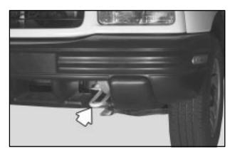
Your vehicle is equipped with recovery hooks. The recovery hooks are provided at the front and rear of your vehicle. You may need to use them if you're stuck off-road and need to be pulled to some place where you can continue driving.
