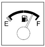
Your fuel gage shows about how much fuel is in your tank. When the gage first indicates "E" (empty), you still have about one or two gallons (4 to 8 L) of fuel left in your tank, but you need to get more right away.
