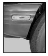
1. Remove the two screws holding the sidemarker lamp assembly using a Phillips screwdriver. The assembly should pull away from the vehicle.
