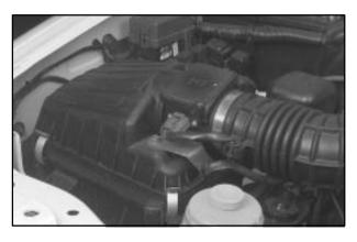
The engine air cleaner/filter is located on the passenger's side of the engine compartment toward the front of the vehicle.
