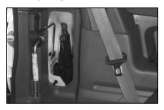
The jacking equipment you'll need is stored in the luggage compartment on the driver's side of the vehicle.
