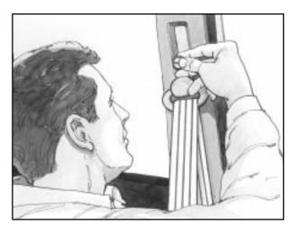
To move it down, pull out the knob and move the height adjuster to the desired position. You can move the adjuster up just by pulling out the knob and sliding the adjuster up. After you move the adjuster to where you want it, try to move it down without pulling out the knob to make sure it has locked into position.
