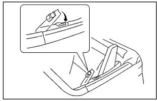
5. Reengage the latches by pushing down on the support arms at the hinges.
