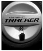
1. The spare tire is mounted on your tailgate. To remove the cover from the spare tire, insert your key into the wheel lock and pull the wheel lock off.
