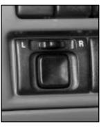
The switch to control the power mirrors is located on the lower left side of the instrument panel.
