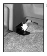
Remove the two attaching screws from each lower corner of the cargo area. Release the tension bows on both sides of the convertible top. See "Convertible Top" later in this section for more information.
