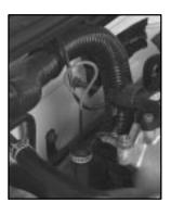
1. The automatic transmission dipstick is a red ring handle located in the rear of the engine compartment toward the center of the vehicle. Pull out the dipstick and wipe it with a clean rag or paper towel.
