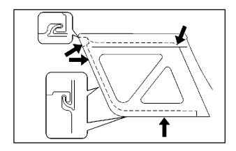
After completing installation, make sure that the front and bottom ends are securely hooked and the rear top end of the window is under the canvas top.
