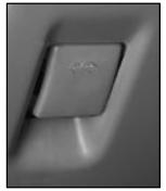
To open the hood, first pull the release handle located on the driver's side of the vehicle on the lower portion of the instrument panel.
