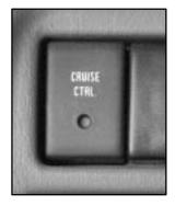
Press the CRUISE CTRL. switch on the instrument panel to turn the system on. The indicator light on the switch will come on.
