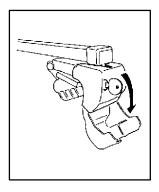
Turn the screw cover lock to the unlocked position and lower the cover.
