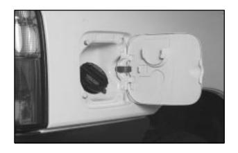
The cap is behind a hinged door on the passenger's side of your vehicle. On some models, you may need to use the vehicle's key to unlock the fuel door.
