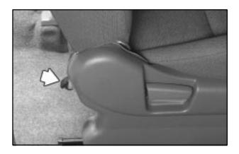
To get out, push the release pedal on the rear of the passenger's side front seat.
