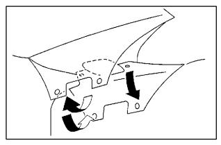
Unfasten the snaps that secure the canvas top to the roof. The snaps are located on either side of the dome lamp. Reattach the snaps which hold the sunroof canvas in place.
