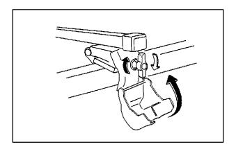
4. Tighten the screws securely, taking care not to overtighten them. Then raise and lock the screw covers.
