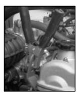
9. The other end of the negative (-) cable doesn't go to the dead battery. It goes to a heavy, unpainted metal part on the engine of the vehicle with the dead battery.
