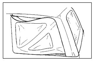
Make sure the plastic clip at the top front corner of the canvas top is unfastened. Then start by zipping the zipper about 3 inches (8 cm), to hold the window in place. When zipping, place the rear bottom corner of the window inside the rear part of the vehicle body to help support the window while you engage the zipper end.
