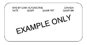
The other label is the Certification label, also found on the driver's door lock pillar. It tells you the gross weight capacity of your vehicle, called the Gross Vehicle Weight Rating (GVWR). The GVWR includes the weight of the vehicle, all occupants, fuel and cargo. Never exceed the GVWR for your vehicle, or the Gross Axle Weight Rating (GAWR) for either the front or rear axle.
