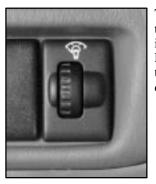
The thumbwheel controls the brightness of your instrument panel lights. Rotate the wheel upward to brighten the lights or downward to dim them.
