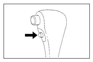
The overdrive off switch is located on the left side of the shift lever. By operating the overdrive off switch, the four-speed automatic transmission (three-speed plus overdrive) can be converted to a three-speed automatic transmission. While in the three-speed mode, the transmission will not shift into the overdrive position.
