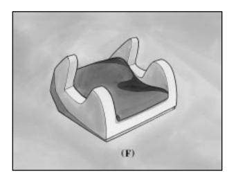
A booster seat (F) is designed for children who are about 40 to 60 lbs., or even up to 80 lbs. (18 to 27 kg, or even up to 36 kg), and about four to eight years of age. A booster seat is designed to improve the fit of the vehicle's safety belt system. Booster seats with shields use lap-only belts; however, booster seats without shields use lap-shoulder belts. Booster seats can also help a child to see out the window.
