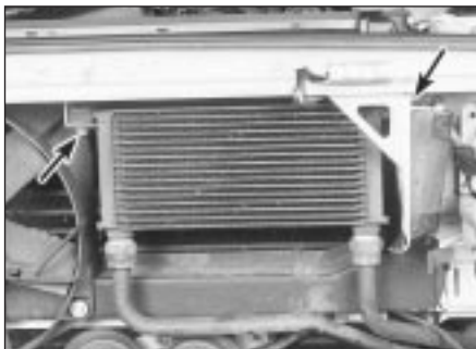
6.3 Remove the mounting nuts (arrowed) to take the oil cooler out
