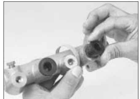
6.7r Refit the grommets
