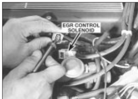
6.8 Check for battery voltage to the EGR control solenoid
