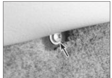
29.5 Detach the screws (arrowed) along the lower edge of the seat cover
