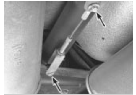
11.5 To disconnect the intermediate cable, remove the cotter pins, washers and clevis pins (arrowed) from the adjuster lever and the yoke
