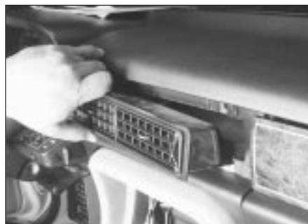
24.7 After removing the centre trim panel, detach the air conditioning duct
