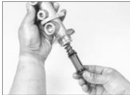
6.7h Remove the secondary piston
