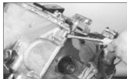
12.4 Pry at the recess in the front of the sump to break the gasket seal - insert a putty knife, if necessary, between the sump and engine block
