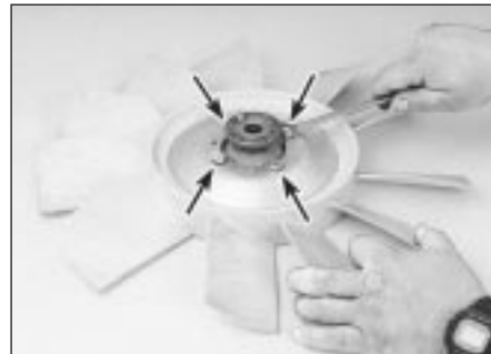
4.12 Separate the fan clutch from the fan by removing the four bolts (arrowed)
