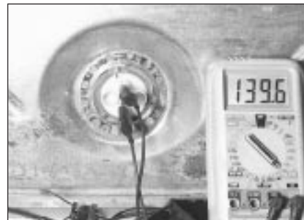
5.4 Connect the probes of the ohmmeter to the fuel level sender unit terminals and check the resistance of the float assembly
