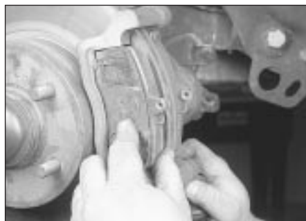
3.5f Remove the outer brake pad
