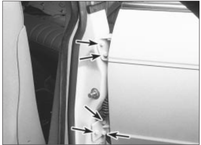
19.7b Open the front door to access the rear door hinge-to-body bolts (arrowed)
