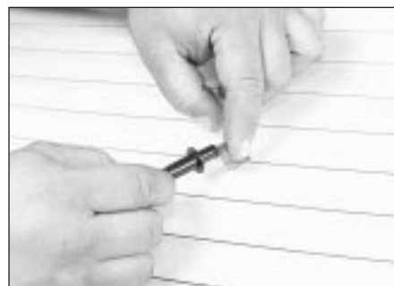
16.4 When measuring the voltage at the heated rear window grid, wrap a piece of aluminium foil around the negative probe of the voltmeter and press the foil against the element with your finger
