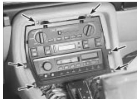
12.3a Remove these six screws (arrowed) to release the control panel/radio assembly from the console
