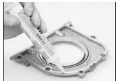
15.5 Apply RTV sealant to the sealing surface
