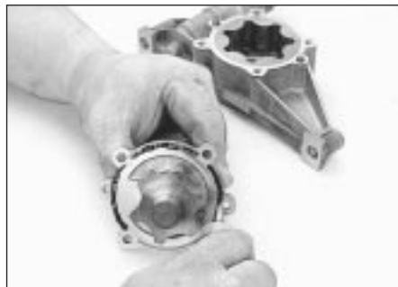
13.14 Apply a thin coat anaerobic sealant (Loctite 510 or 518) to the pump cover sealing surface
