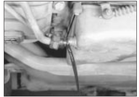
26.6b Detach the tube and let the remaining fluid drain
