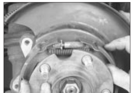
12.5r Pull the shoes apart and refit the adjuster mechanism
