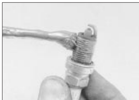
4.10 Apply a coat of anti-seize compound to the spark plug threads
