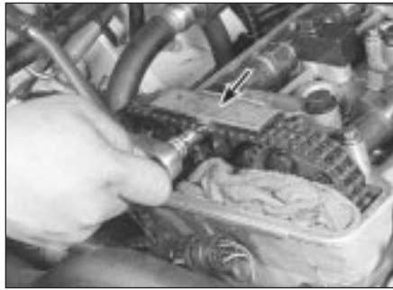
10.13 Remove the two bolts and the upper timing chain guide (arrowed)
