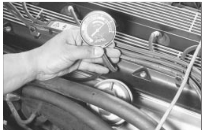
6.6 Check for vacuum to the EGR valve from the throttle body
