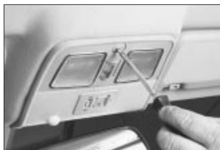
24.13 Remove the plastic screw, then pull the overhead console down and unplug the electrical connectors
