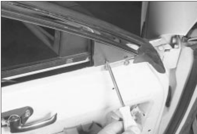
23.2 Remove the trim cover retaining screws
