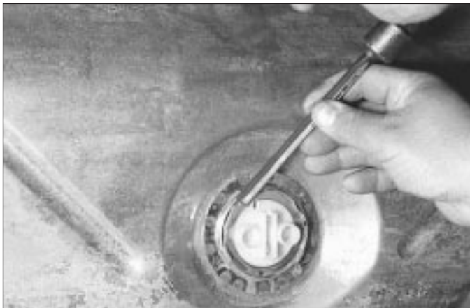
5.10 Use a brass punch and remove the lock ring by tapping on it in an anti-clockwise direction
