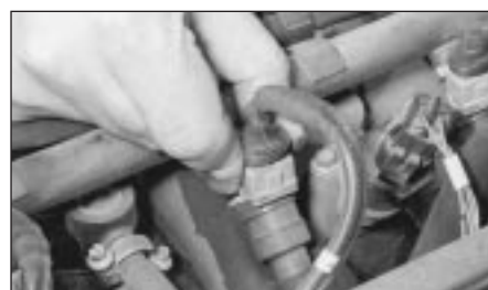
D Check that the wiring connectors are securely connected to the injectors and various fuel system sensors and switches.
