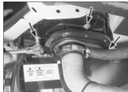
7.7a Remove bolts (arrowed) that retain the fuel filler assembly to the body and slide the assembly down the filler neck of fuel tank
