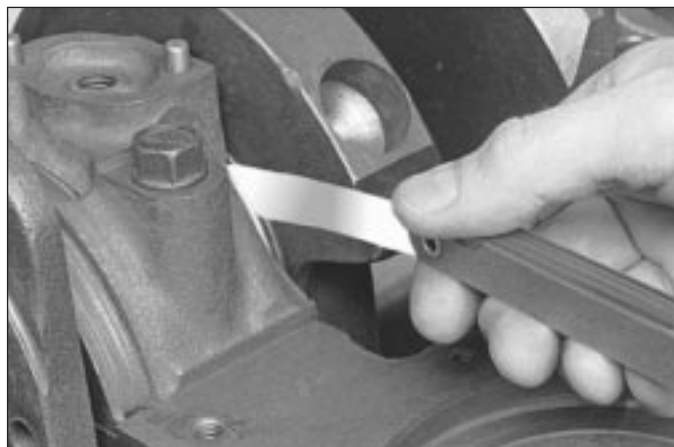
14.3 Checking crankshaft endplay with a feeler gauge
