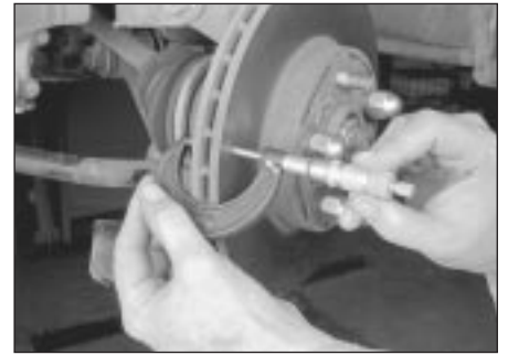
5.5a The disc thickness can be checked with a micrometer
