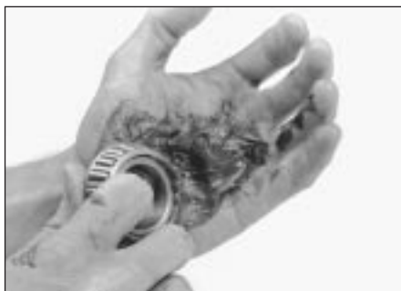
22.15 Work the grease completely into the bearing rollers
