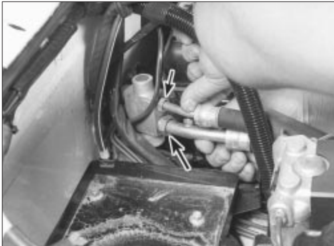
13.9 Feel the inlet (small arrow) and outlet (large arrow) pipes at the bulkhead leading to the air conditioning evaporator (battery removed here for clarity only)
