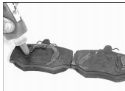
3.5k Apply anti-squeal compound to the new brake pads
