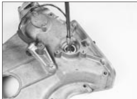
8.28a Drill a small hole in the intermediate shaft seal, thread a sheet metal screw into it and use a small slide-hammer pull the seal out of the cover
