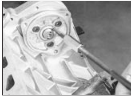
9.4 Remove the auxiliary shaft seal with a small slide-hammer puller
