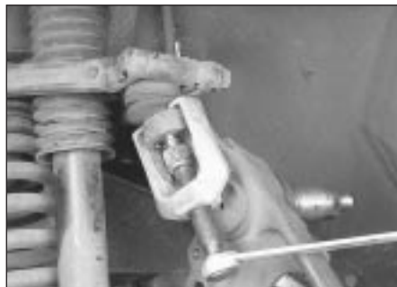
5.7 To detach the upper balljoint from the steering knuckle, loosen the ballstud nut, fit a small puller and break the ballstud loose from the knuckle
