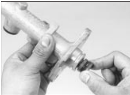
6.7g Remove the primary piston
