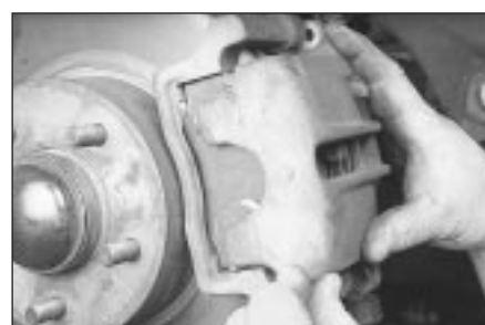
3.5o Refit the caliper, then tighten the mounting bolts to the specified torque
