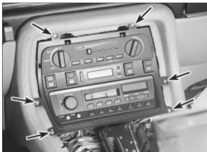
13.3 Remove the retaining screws (arrowed) and pull the radio/control panel out enough to unplug the connectors
