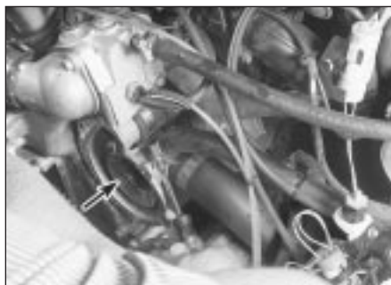
8.8a Once the water pump is removed, the rear housing (arrowed) is held in place only by the hoses - check them for leakage and condition whenever the pump is disturbed
