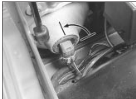
17.9 Disconnect the electrical connector and rotate the bulb assembly 1/4-turn anti-clockwise
