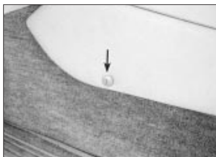
24.9 Remove the plastic screws (arrowed) from each side of the console
