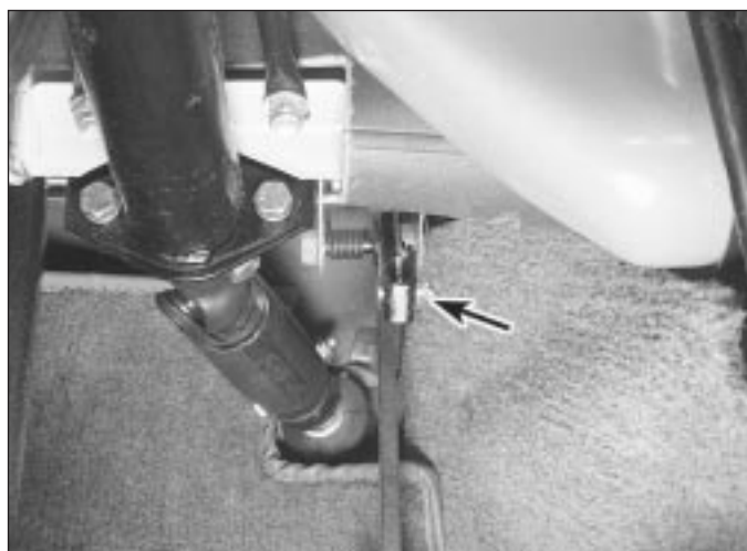
10.4 Remove circlip (arrowed) and separate cable from the accelerator pedal by pulling the pin from the pedal assembly
