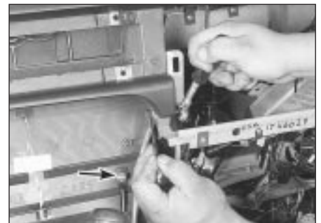
17.9b Black case-support rods are held with nuts (arrowed), the gold dash-support rods are retained by a bolt/nut to the dash
