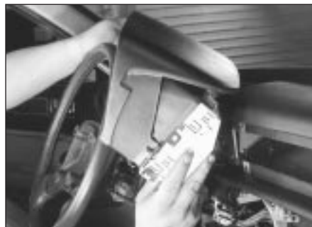
25.5 Pull outward on the instrument cluster housing and unplug the electrical connectors from the backside
