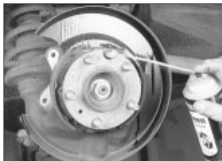
12.5a Wash down the handbrake assembly with brake cleaner before dismantling
