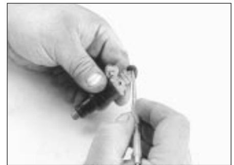
13.38b Pick out the old injector seal but make sure the injector body is not damaged in the process
