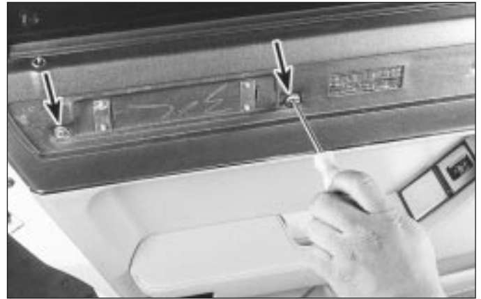
18.5 Detach the screws located behind the wood finisher panel, then remove the upper portion of the door trim panel
