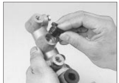
6.7c Remove the grommets, noting the position of each one
