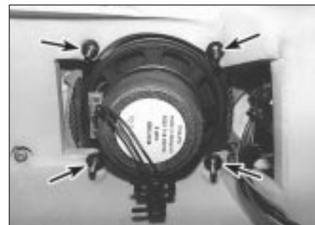
13.6 Remove the nuts from the retaining studs (arrowed) to remove the speaker
