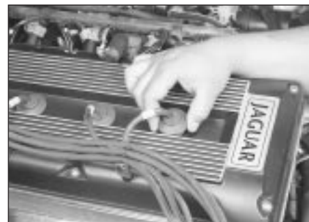
4.6 When removing the spark plug leads, grasp only the boot and use a twisting/pulling motion
