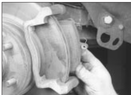
3.5g Remove the inner brake pad
