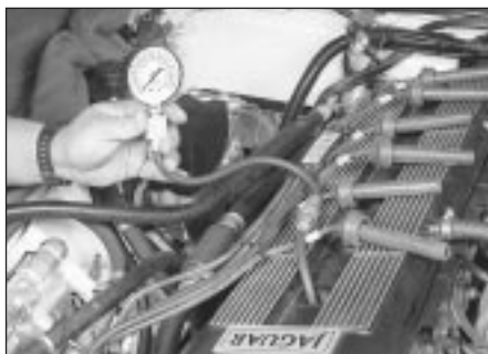
4.6 A compression gauge with a threaded fitting for the spark plug hole is preferred over the type that requires hand pressure to maintain the seal - be sure to block open the throttle valve as far as possible during the compression check!
