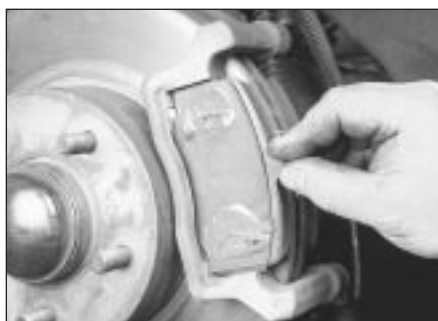
3.5n Refit the outer pad
