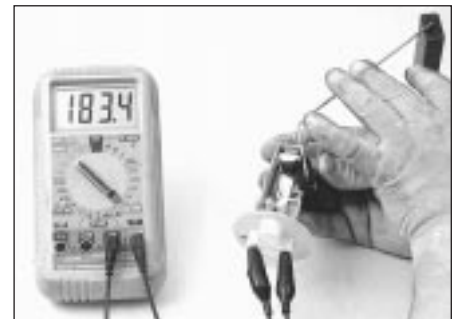
5.8 An accurate check of the sender unit can be made by removing it from the fuel tank and observing the resistance with the float down (empty) and then extended (full)
