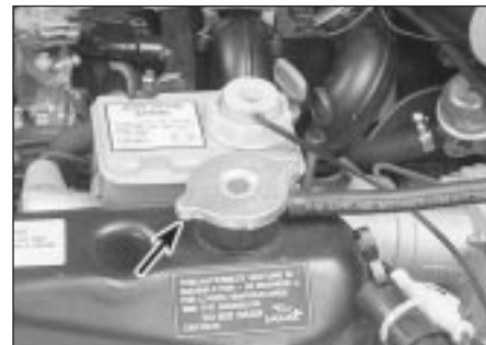
30.3 Push the expansion tank pressure cap downward and rotate anti-clockwise - never remove it when the engine is hot!
