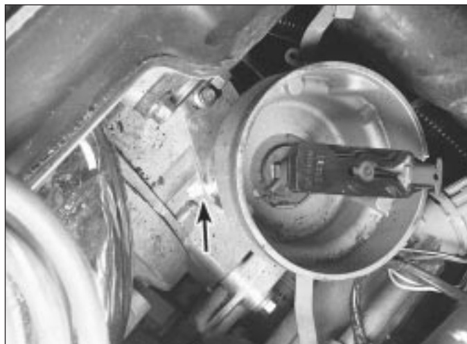
9.5b Paint or scribe another mark across the cylinder head and the distributor body (arrowed) to ensure that the distributor is aligned correctly when it is reinstalled
