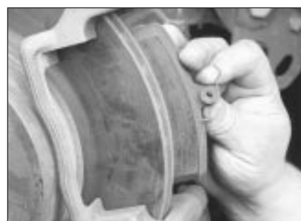
3.5m . . . then refit the inner pad onto the caliper bracket
