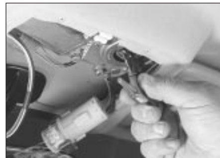
27.9 To close the sunroof manually, insert the T-handle spanner in the motor shaft and rotate it clockwise
