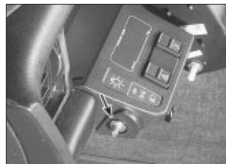
10.3 Detach the headlight switch knob, then remove the hex nut securing the switch to the instrument panel (arrowed)
