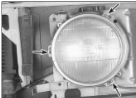
17.4 Loosen the retaining ring screws (arrowed) a few turns - rotate the retaining ring anti-clockwise to remove it
