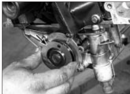
13.17 Refit the original shim pack (arrowed) if the original pump is being used - if a new pump is being installed, refit a 0.38 mm (0.015-inch) shim pack
