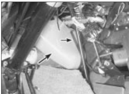
17.5 Left duct (large arrow) can be removed by pulling off the clip (small arrow) - right duct pulls out without a clip
