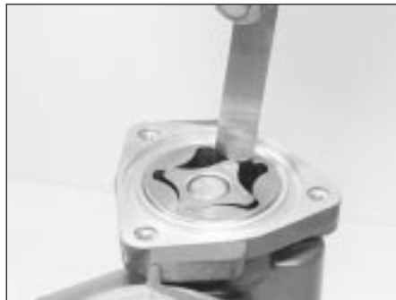
16.4B Checking the inner rotor-to-outer rotor clearance
