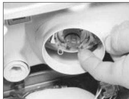
5.2B . . . compress the clips . . .
