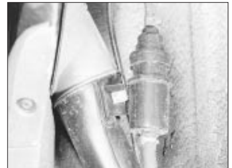
10.3 Roll-over valve location on fuel filler pipe
