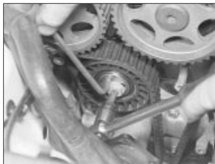
10.12 Slacken tensioner bolt, and use Allen key to rotate tensioner away from timing belt
