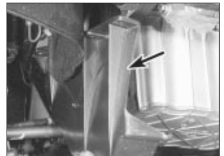
11.3 Removing the auxiliary drivebelt lower cover (arrowed) from inside the wheel arch
