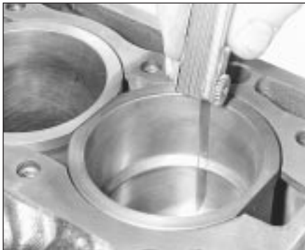
19.3 With the ring square in the bore, measure the end gap with a feeler gauge
