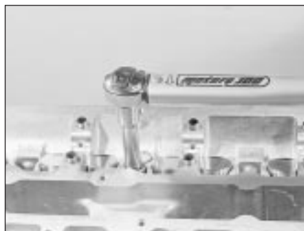
14.30B Tightening cylinder head bolts (Stages 1 and 2) using torque wrench . . .
