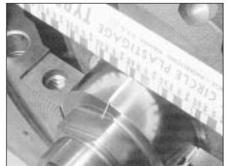
20.15 Compare the width of the crushed Plastigage to the scale on the envelope to determine the main bearing oil clearance (always take the measurement at the widest point of the Plastigage). Be sure to use the correct scale; Imperial and metric scales are included
