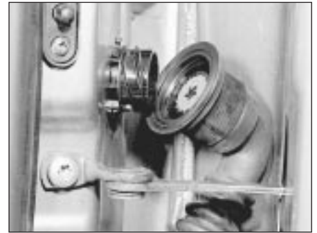
16.1 Disconnect the wiring multi-plug connector
