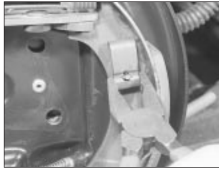
6.3 Removing a shoe steady spring
