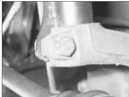
2.9A Remove the suspension strut-to-spindle carrier clamp bolt . . .
