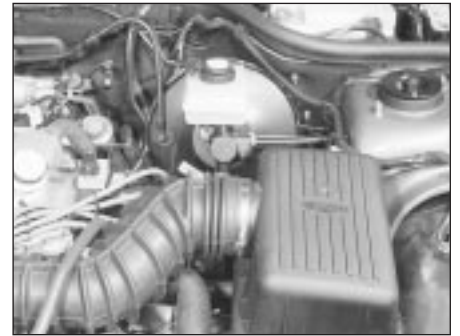
4.8 General view of the air filter (A) and air duct (B) fitted to the 1.6 litre EFI engine
