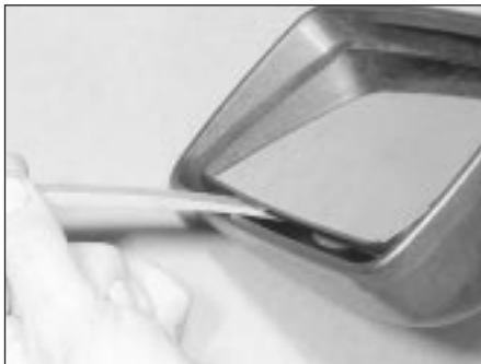
17.1A Prise free the door mirror glass...
