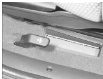
Chassis number etched into the floor to the right-hand side of the driver's seat
