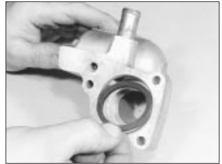
4.6C . . . and where applicable, remove the O-ring seal
