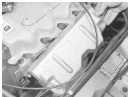
7.1B Hot-air shroud removal from the 1.6 litre EFI fuel injected engine
