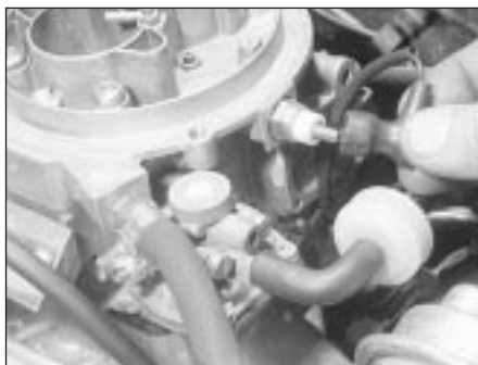
23.5A Disconnecting the lead from the anti-dieselling (fuel-cut off) solenoid
