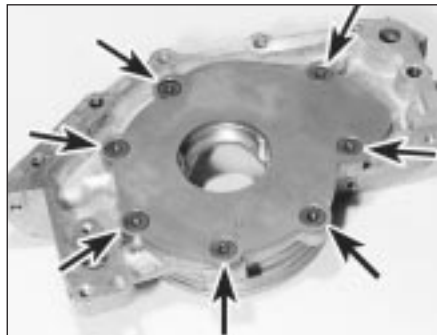
17.2 Oil pump cover plate retaining screws (arrowed)
