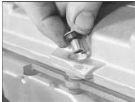
5.9 Ensure rubber seal is fitted to each cover bolt spacer, as shown
