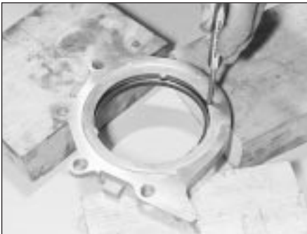
17.13 . . . and ensure that carrier is properly supported when driving out used oil seal - note notches provided in carrier for drift
