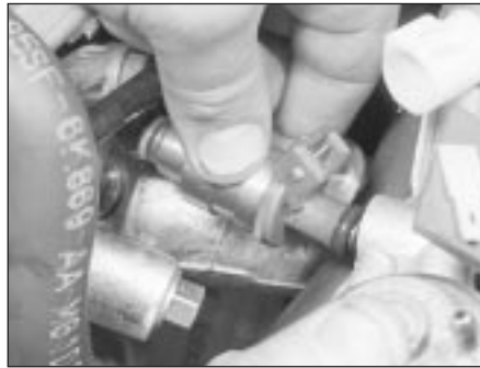
16.13B . . . release each injector . . .
