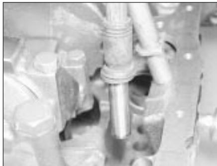
11.8 Tappet withdrawal using a valve grinding tool suction cup
