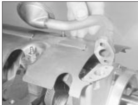
16.16 Use new gasket when refitting oil pick-up pipe to pump
