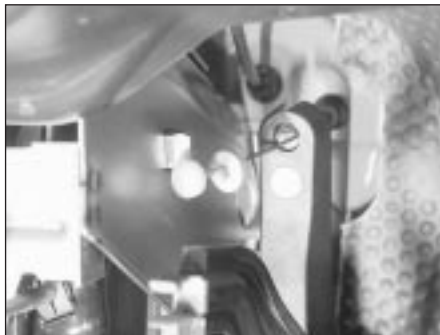
3.2 Disconnecting the accelerator cable from the pedal
