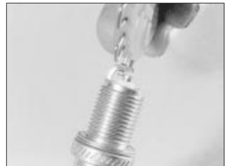
27.13 To change the gap, bend the outer electrode only, and be very careful not to crack or chip the porcelain insulator surrounding the centre electrode
