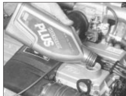
3.6C Topping-up the engine oil level (Zetec engine)
