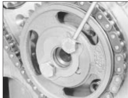
13.15 Bend locktabs against the camshaft retaining bolt heads to secure
