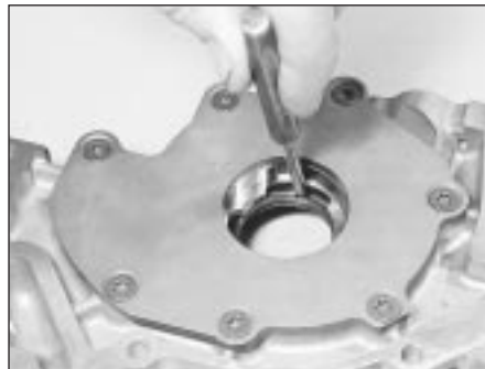
17.2 Driving out crankshaft right-hand oil seal
