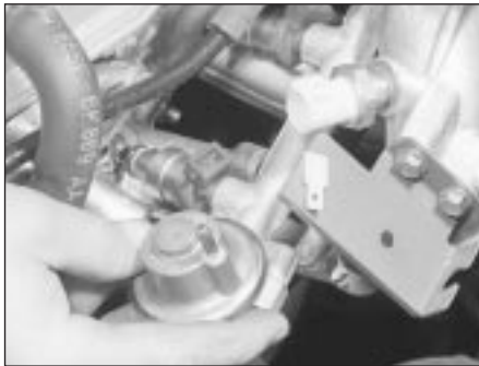
16.13C . . . and withdraw the fuel rail and injectors
