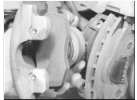
2.17D . . . then withdraw the caliper from the anchor bracket and disc
