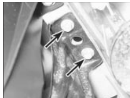
7.8 Radiator retaining bolts (arrowed)
