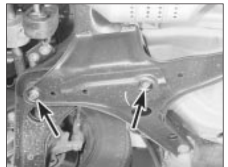
9.3 Suspension arm-to-subframe retaining bolts (arrowed)
