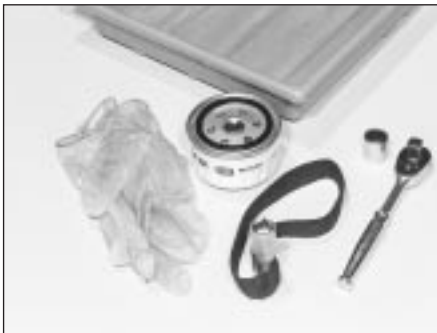
16.2 These tools are required when changing the engine oil and filter
