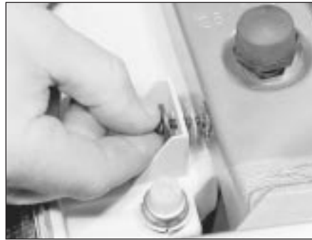
7.7B Headlight retaining screw showing washer arrangement
