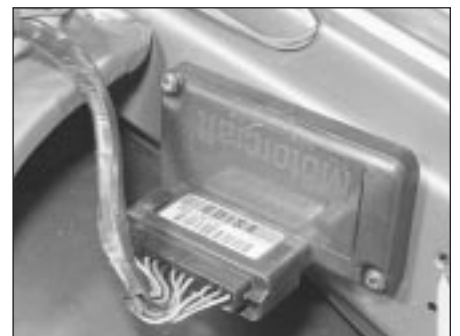
8.3 Ignition module and wiring connection on the 1.6 litre EFi fuel-injected engine
