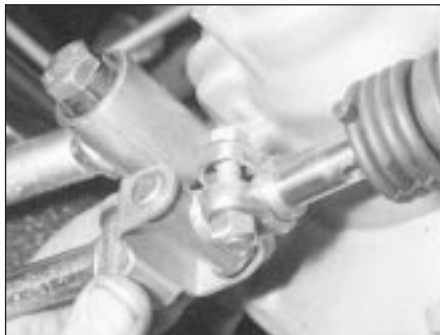
6.24A Disconnect the gearchange linkage ...
