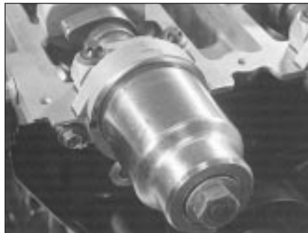
12.5 Using socket and toothed pulley bolt to install camshaft oil seal
