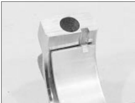
21.3 Tab on each big-end bearing shell must engage with notch in connecting rod or cap
