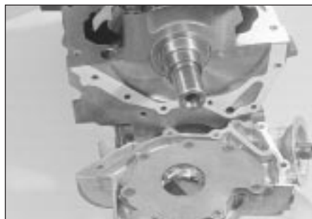
16.12 Use new gasket when refitting oil pump
