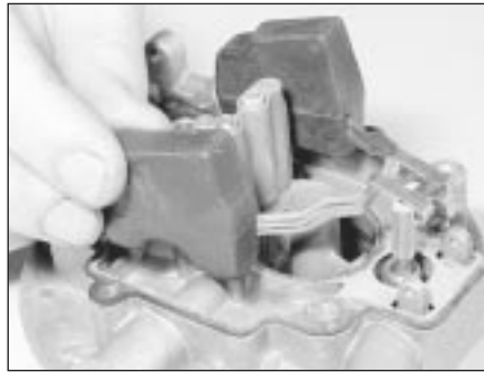
14.6B ... then detach the float and needle valve
