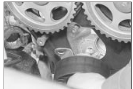
11.3 Removing timing belt tensioner
