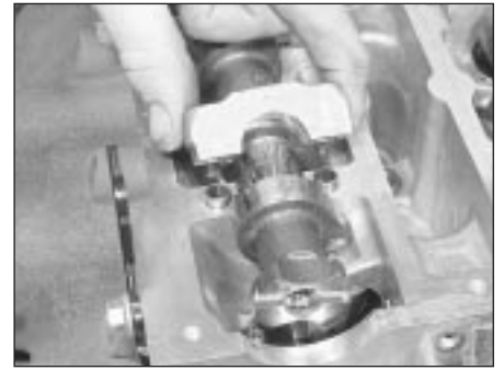
13.5A Note locating dowels when removing camshaft bearing caps
