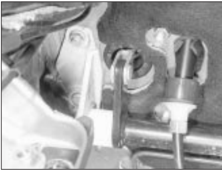
15.5 Brake system cross-link mounting to the bulkhead
