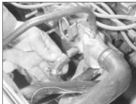
4.3B Detaching the heater hose from the thermostat housing (CVH engine)
