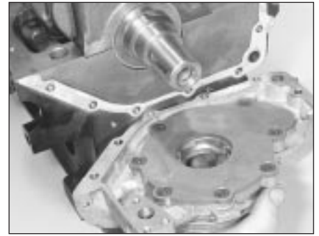
16.9A Refit the oil pump
