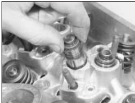
13.6A Removing a hydraulic tappet
