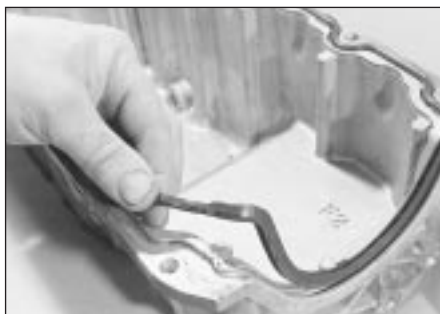
15.11 Ensure gasket is located correctly in sump groove
