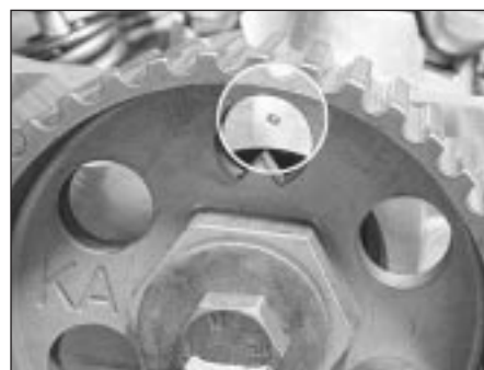
4.6B Camshaft sprocket timing mark aligned with the TDC mark on the front face of the cylinder head
