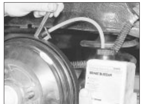
17.22 Bleeding a front brake using a one-way valve kit
