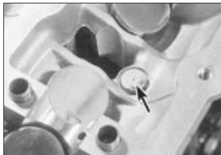
8.24 Cylinder head oil-retaining valve (arrowed)
