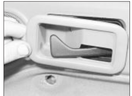
10.3B ... and remove the bezel
