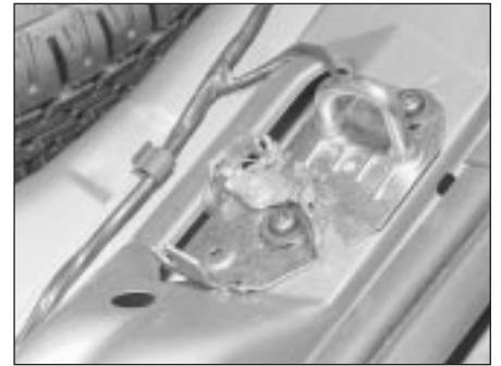
23.6A Undo the retaining screws . . .
