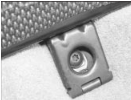
32.3 Rear seat cushion retaining screw (Saloon)
