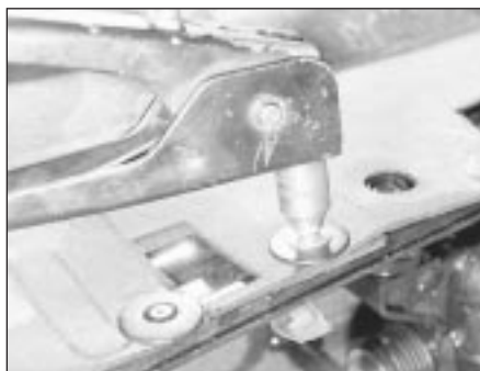
7.12 Pop-riveting the anti-splash shield to the radiator
