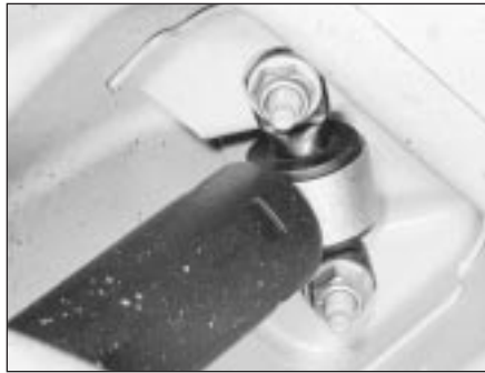
16.4 Rear shock absorber upper mounting (Estate models)
