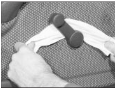
10.1A Release the regulator retaining clip as shown ...
