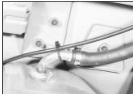
8.5 Fuel filler pipe connection to the fuel tank. Note the handbrake cable locating strap
