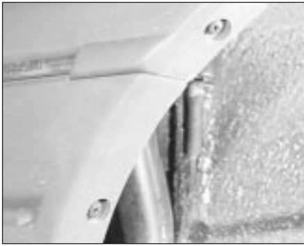
6.8 Rear bumper retaining screws
