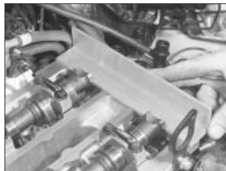
10.8 Fit camshaft-aligning tool to ensure engine is locked with Nos 1 and 4 cylinders at TDC
