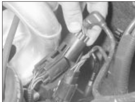
14.9A Unplug engine wiring loom connector alongside the inlet manifold
