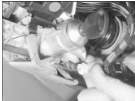
21.6 Detach the bonnet release cable from the lever
