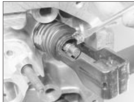
10.11 Insert the split collets into the groove in the valve stem
