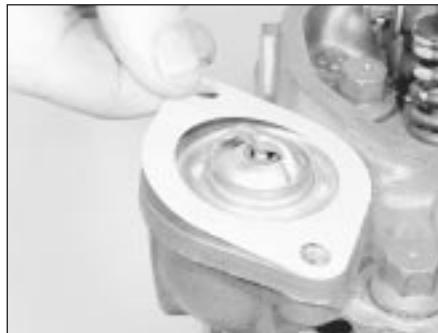
4.18 Use a new gasket when refitting the thermostat housing
