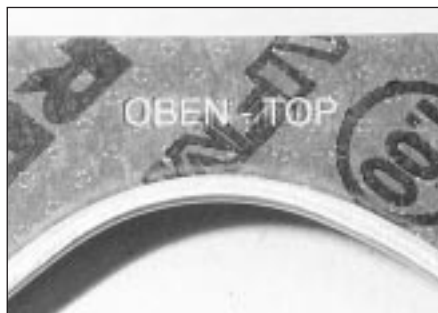
10.22A Cylinder head gasket top-face marking ("OBEN")
