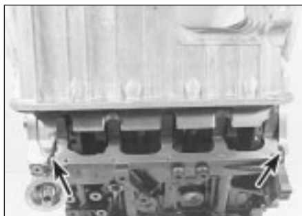
15.13A Apply sealant (arrowed) as directed when refitting sump
