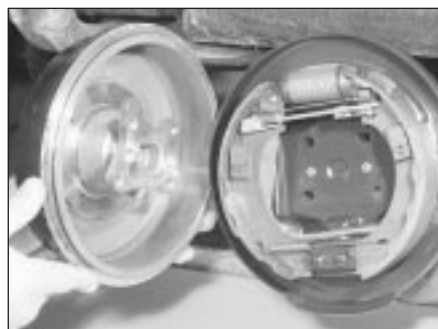
5.2B Removing the rear brake drum/hub
