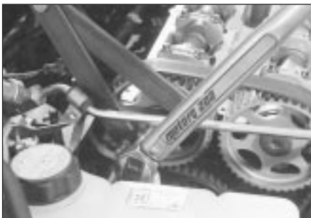
10.23 Using forked holding tool while camshaft toothed pulley bolt is tightened
