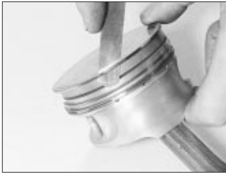
15.2 Using feeler gauge blades to remove piston rings
