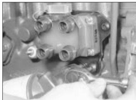
6.10A Unbolting the ignition coil from the HCS engine
