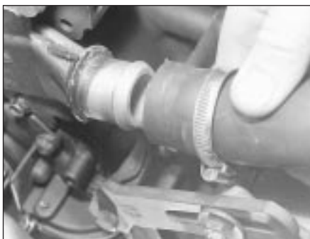
9.4 Detach the coolant hose from the water pump
