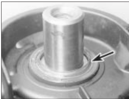
16.9B With the oil pump refitted, remove the protective guide (arrowed)
