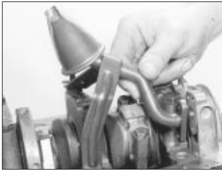
16.4 Removing the oil inlet pipe
