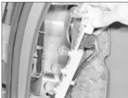
5.34 Rear light cluster removal on Estate models
