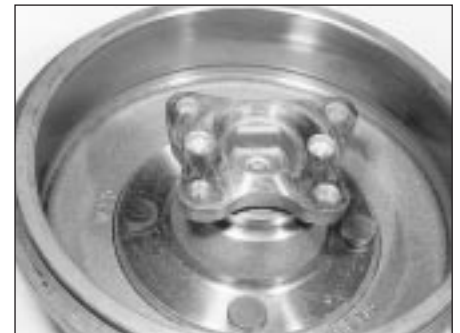
5.6 Examine the inside surfaces of the brake drum for signs of excessive wear and/or cracks
