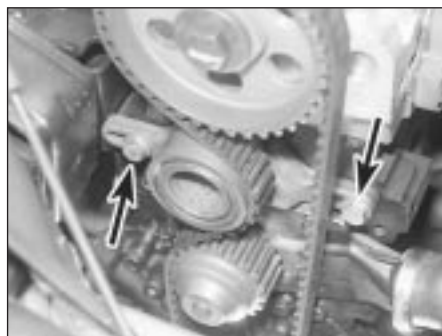
10.4 Timing belt tensioner retaining bolts (arrowed)
