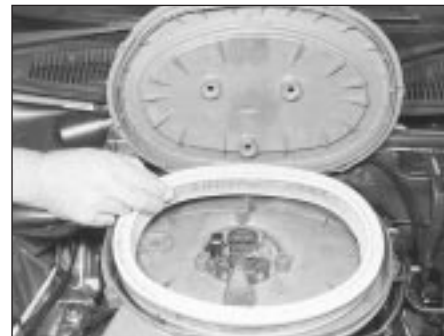
29.1C . . . then lift off the cover and withdraw the element
