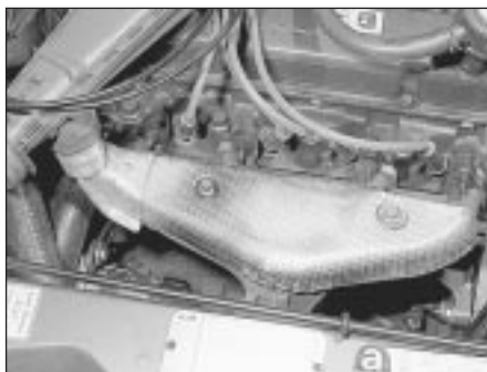
8.1 Exhaust manifold shroud/heat shield
