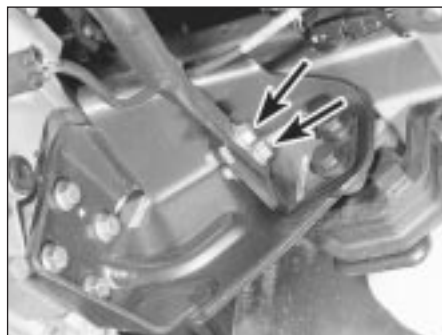
5.33 Remove the brace between the transmission left front mounting bracket and the transmission flange
