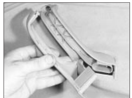
10.2A Remove the door handle trim capping ...
