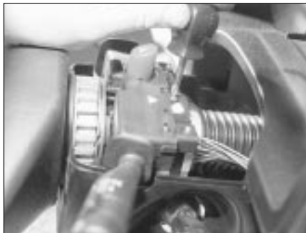
4.8A Undo the retaining screw . . .
