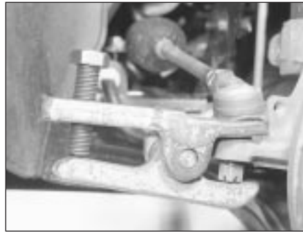
28.3 Balljoint separator tool in position. Note that the nut should be left loosely in position when the thread of the joint is to be protected for re-use
