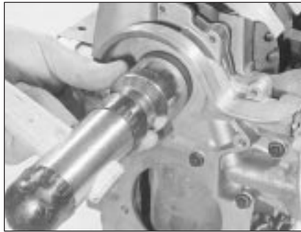
17.6 If seal is tapped into place as shown, exercise great care to prevent seal from being damaged or distorted
