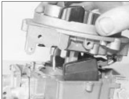
17.2B ... and remove the carburettor upper body
