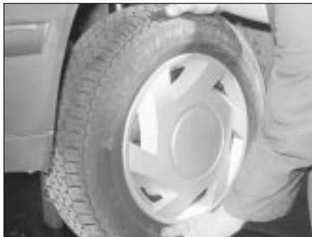
19.4 Checking for wear in the front suspension and hub bearings
