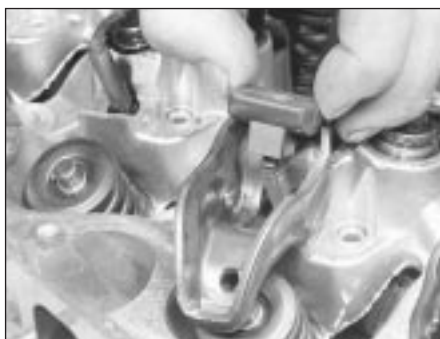
13.5B ... withdraw the guide ...
