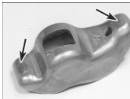
13.19 Inspect the rocker arm contact points indicated for excessive wear
