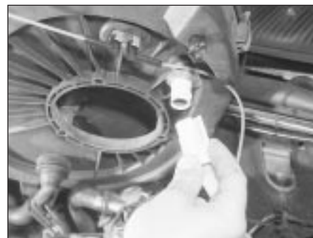
2.4C Disconnecting the intake air temperature sensor connector (CVH engine)
