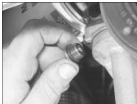
16.9A Unscrew threaded plug - seen through right-hand wheel arch . . .
