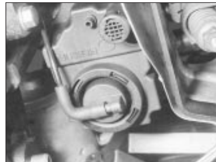
6.27 Disconnect the vacuum hose from the base of the filter housing ...
