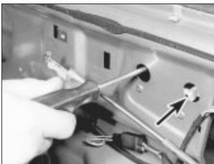
11.3 Undo the glass-to-regulator screws through apertures shown
