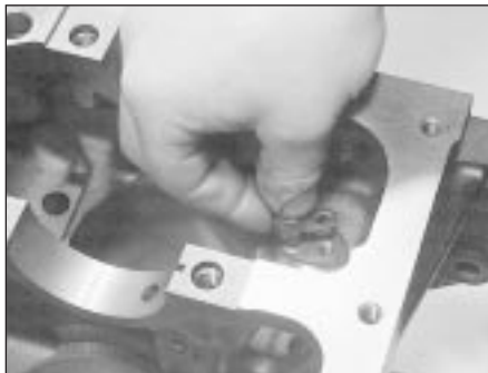
14.1A Unbolt blanking plugs (where fitted) to clean out oilways . . .
