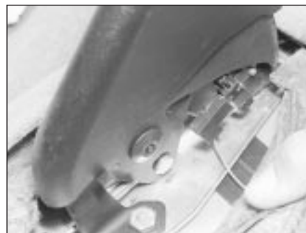
4.31 Handbrake warning light switch
