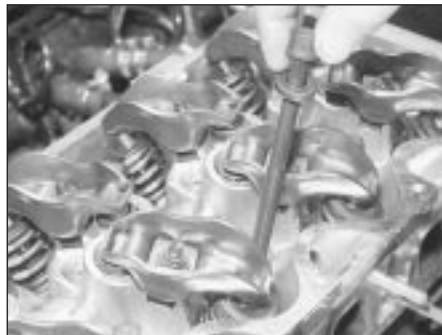
14.23B Insert the new cylinder head bolts
