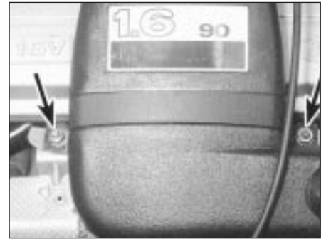
4.25 Undo the two nuts (arrowed) and lift off the air inlet duct retaining strap
