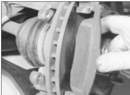
2.18A Withdraw the outer pad from the anchor bracket . . .
