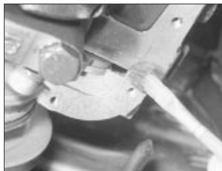
15.11B Applying sealant to the oil pump-to-crankcase joint
