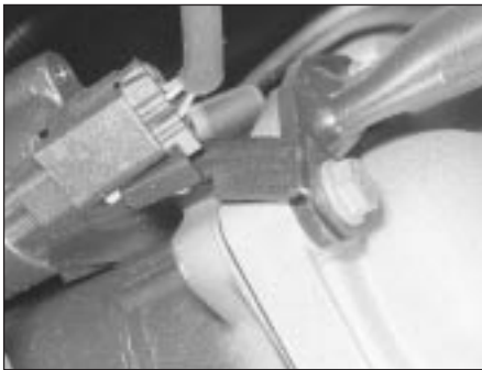
17.4D Oxygen sensor wiring multi-plug connector and location bracket
