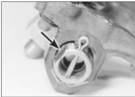
9.8 Flat on the rocker shaft (arrowed) to same side as rocker arm adjusting screws
