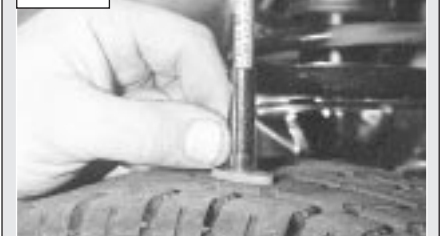
Tread wear can be monitored with a simple inexpensive device known as a tread depth indicator gauge.
