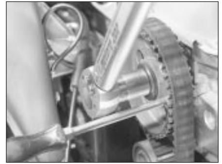
11.13B . . . and tighten the retaining bolt to the specified torque whilst retaining the sprocket as shown
