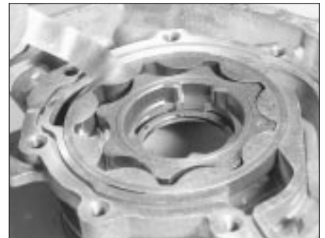
17.3A Outer rotor-to-oil pump body clearance check
