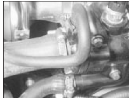
14.14 Disconnect all coolant hoses from thermostat housing
