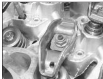
13.5A Undo the rocker arm retaining nut ...
