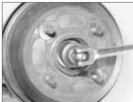
11.8 . . . unscrew the hub nut . . .
