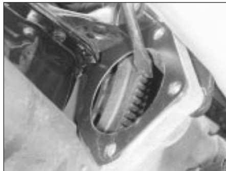
8.6 Using a suitable bar to lock the flywheel ring gear
