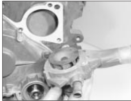
8.9 Refitting the water pump to the engine. Note the new gasket
