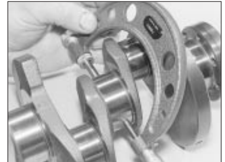
16.5 Measure the diameter of each crankshaft journal at several points, to detect taper and out-of-round conditions
