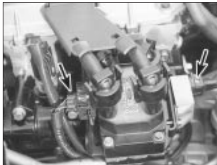
14.9B Unplug connectors (arrowed) to disconnect ignition coil wiring
