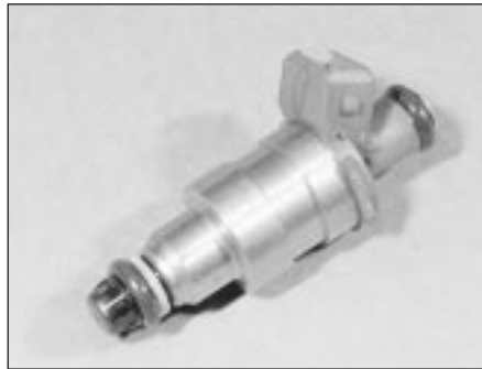
16.15 Fuel injector with new seals fitted
