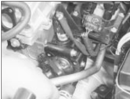
4.8 Unscrew the retaining bolts, and remove the water outlet from the thermostat housing
