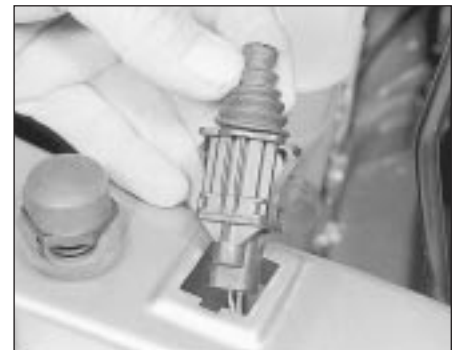
26.12 Bonnet alarm switch removal (anti-theft alarm system)
