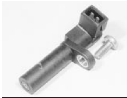
10.5 Crankshaft speed/position sensor shown removed from engine
