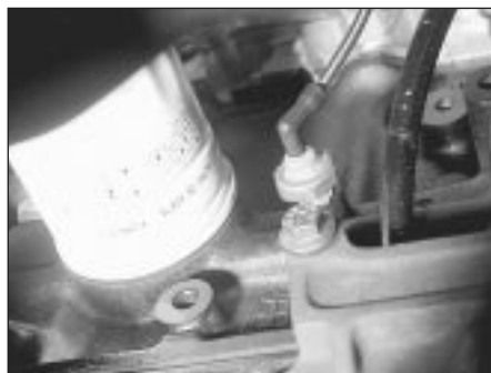
5.12B . . . the oil pressure switch . . .
