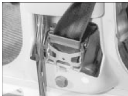
33.11 Inertia reel unit and retaining bolt
