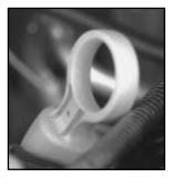
The transaxle fluid dipstick handle is the red loop near the back of the engine.
