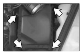
To check or replace the air filter, remove the four screws and lift the cover.
