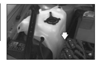
When the engine is cold, the coolant level should be at or above the COLD mark on a cold engine. The coolant level should be at or above the HOT mark on a hot engine. If it isn't, you may have a leak in the radiator hoses, heater hoses, radiator, water pump or somewhere else in the cooling system.
