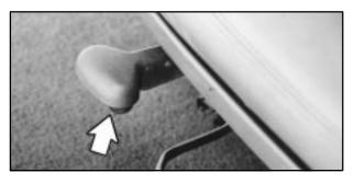
Lift the handle to tilt the seat up or down.
