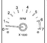
The tachometer displays the engine speed in thousands of revolutions per minute (rpm).
