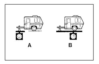
If you're using a weight-carrying hitch, the trailer tongue (A) should weigh 10 percent of the total loaded trailer weight (B). If you have a weight-distributing hitch, the trailer tongue (A) should weigh 12 percent of the total loaded trailer weight (B).
