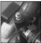
3. After the engine cools, open the coolant air bleed valve or valves.
