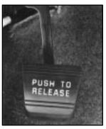
To set the parking brake, hold the regular brake pedal down with your right foot. Push down on the parking brake pedal with your left foot.
