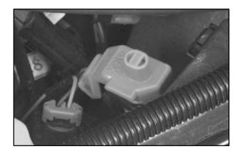
5. Find the positive (+) and negative (-) terminals on each battery. Your vehicle has a remote positive (+) jump starting terminal. The terminal is on the same side of the engine compartment as your battery. You should always use the remote positive (+) terminal instead of the positive (+) terminal on your battery. To uncover the remote positive (+) terminal, lift the red plastic cap.
