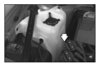
The vehicle must be on a level surface. When your engine is cold, the coolant level should be at the COLD mark or a little higher. When your engine is warm, the level should be up to the HOT mark or a little higher.
