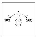
You have a gage that shows the engine coolant temperature. If the gage pointer moves into the red area, your engine is too hot!
