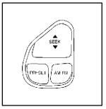
**SEEK:** Press the up arrow to tune to the next radio station and the down arrow to tune to the previous radio station.
