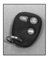
Press UNLOCK once to unlock the driver's door. Press UNLOCK again within five seconds to unlock all remaining doors; pressing UNLOCK will also cause the vehicle's interior lamps to come on for a period of time.
