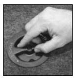
The equipment you'll need is in the trunk. Pull the carpeting from the floor of the trunk. Turn the center nut on the compact spare cover counterclockwise to remove it. Then lift and remove the cover.
