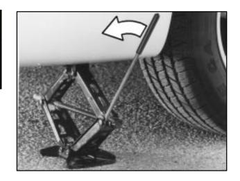
9. Lower the vehicle by turning the jack handle counterclockwise. Lower the jack completely.
