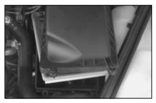
Pull out the filter. Be sure to install the air filter and put the cover back on tightly when you are finished.
