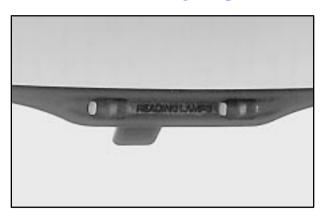
These lamps go on when you open the doors. When the doors are closed, turn the lamps on and off with the switches.
