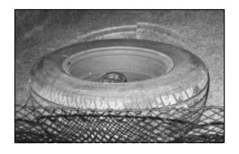
Put the bolt through one of the wheel nut holes, install the retainer over the bolt, then install the wing nut. Put the spacer and nut next to the tire in the well. Store the cover as far forward as possible. The compact spare is for temporary use only. Replace the compact spare tire with a full-size tire as soon as you can. See "Compact Spare" in the Index. See the storage instructions label to store your compact spare in the trunk properly.
