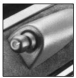
The power mirror control is located on the driver's side door. Turn the control counterclockwise to adjust the driver's side mirror or clockwise to adjust the passenger's side mirror. Then move the control in the direction you want to move the mirror.
