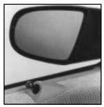
Adjust the passenger's side mirror by hand. To adjust the driver's side mirror, move the knob in the direction you want to move the mirror.
