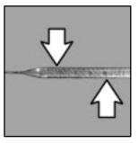
Pull out the dipstick and clean it with a paper towel or cloth, then push it back in all the way. Remove it again, keeping the tip down, and check the level.
