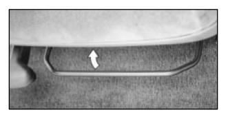
The driver's seat may have a bar and a handle under the front edge of the seat. Lift the bar to unlock the seat and to slide it forward and backward. Try to move the seat with your body to be sure the seat is locked into place.
