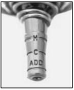
When the engine compartment is hot, the level should be at the H mark. When it's cold, the level should be at the C mark. If the fluid is at the ADD mark, you should add fluid.
