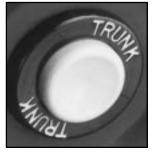
Press the button under the instrument panel on the driver's side. Your transaxle shift lever must be in PARK (P) for the remote trunk release button to work.
