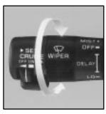
You can control the windshield wipers by turning the band marked WIPER.
