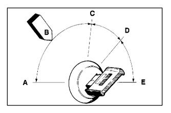
**ACC** (**A**): The accessory position lets you use things like the radio and windshield wipers when the engine is off. To use ACC, push in the key and turn it toward you. Your steering wheel will stay locked.
