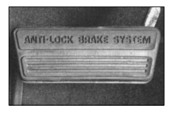
If your vehicle has anti-lock brakes, the brake pedal will say so.
