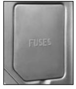
Some fuses are in a fuse block on the passenger's side of the instrument panel. Pull off the cover labeled FUSES to expose the fuses.
