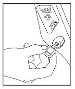
1. Open the rear door. Use a key to move the lever all the way up.
