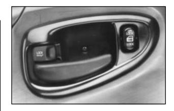
From the inside, push the lever to lock the door manually. To unlock, pull the lever in the opposite direction.
