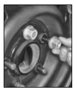
8. Put the spare tire on and then reinstall the wheel nuts with the rounded end of the nuts toward the wheel. Tighten each nut by hand until the wheel is held against the hub.
