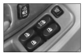
Switches on the driver's door armrest controls operate each of the windows when the ignition is in ON or ACC. In addition, each of the passenger's doors has a window switch for its own window.
