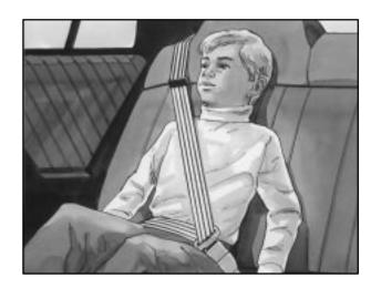
Buckle, position and release the safety belt as described in "Rear Seat Outside Passenger Positions" earlier in this section. Make sure that the shoulder belt crosses the shoulder.
