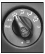
The rear window defogger uses a warming grid to remove fog from the rear window. Press the area labeled PUSH to turn the defogger on.
