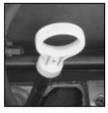
The engine oil dipstick handle is the yellow loop near the front of the engine.
