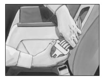
4. Tilt the latch plate to adjust the belt if needed.
