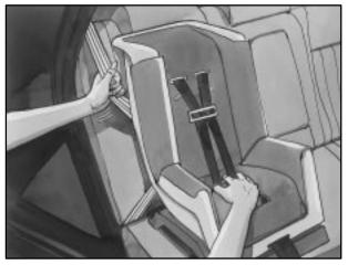
• If your vehicle has the child restraint locking feature on the shoulder belt retractor, pull the rest of the shoulder belt all the way out of the retractor to set the lock.
