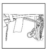
Your vehicle is equipped with auxiliary power leads. These leads can be used to power aftermarket electrical equipment added to your vehicle.
