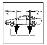
3. Position the jack under the vehicle and raise the jack lift head until it fits firmly into the notch in the vehicle's frame nearest the flat tire.
