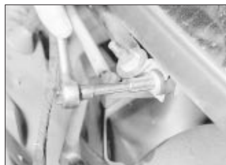
38.5A Unscrew the windscreen wiper motor/linkage assembly securing bolts . .
