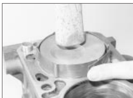
32.15 Tapping a piston into its bore - 2.0 litre SOHC engine
