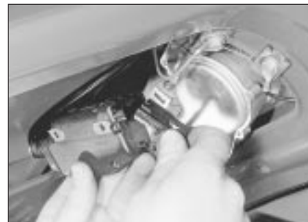
46.18 Disconnecting the wiring plug from the tailgate lock operating motor - Hatchback model
