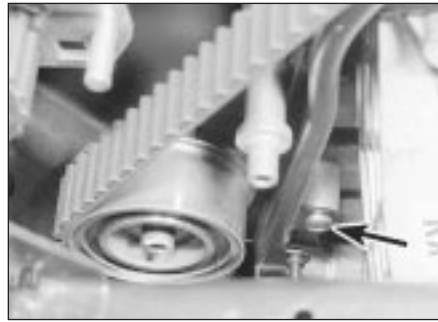
4.19B Rear timing belt cover lower right-hand securing bolt
