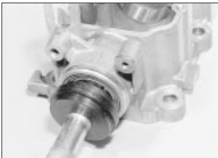
18.11A Fitting a new camshaft front oil seal using a special tool - 2.0 litre engine
