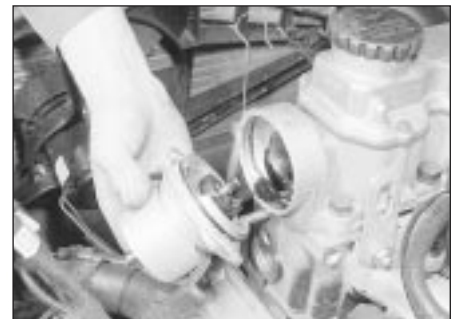
18.7C . . .and withdraw the distributor
