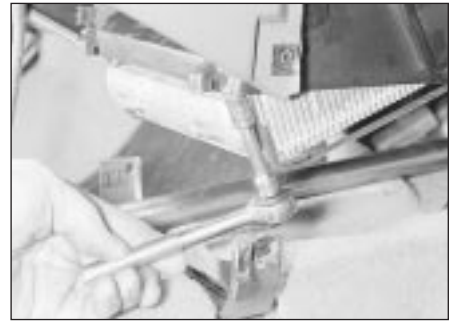
17.5 Unscrewing a heater matrix securing strap screw
