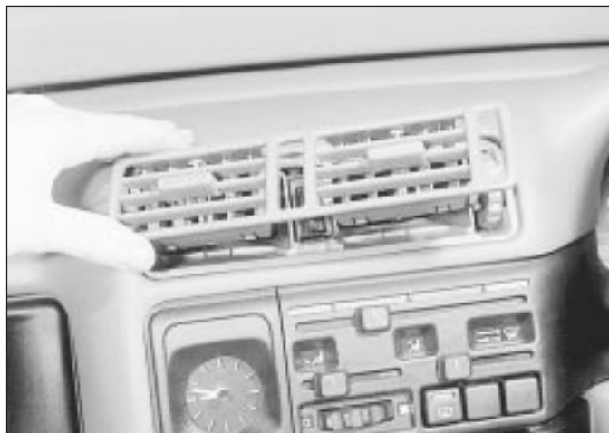
19.2B . . . to release the centre facia ventilation nozzles
