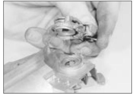
20.3B . . . and recover the lever assembly
