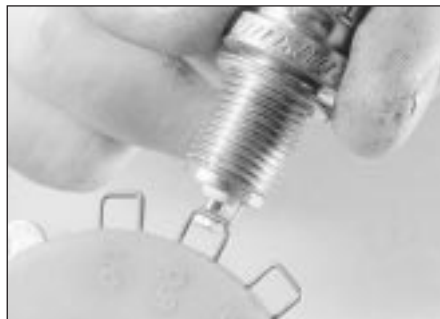
30.9B Measuring the spark plug gap with wire gauge
