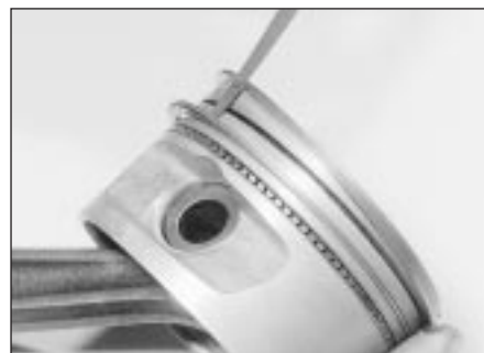
33.5A Using a feeler blade to aid removal of a piston ring - 2.0 litre SOHC engine
