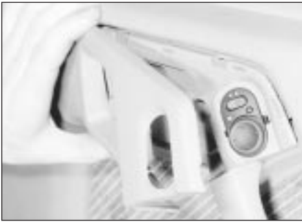
17.3 Remove the plastic surround from the door interior handle
