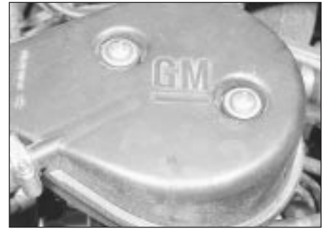
5.4B Do not overtighten the air box screws
