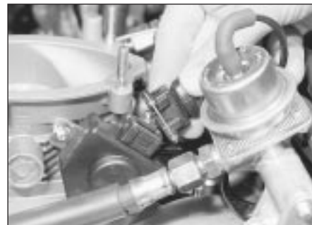
23.8 Disconnecting the throttle position sensor wiring plug - DOHC model
