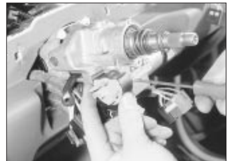
4.6 Removing an ignition switch securing screw
