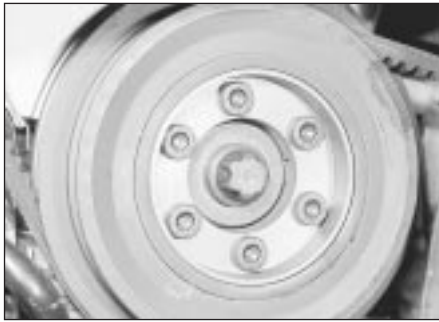
4.7 Crankshaft pulley and securing bolts viewed through right-hand wheel arch
