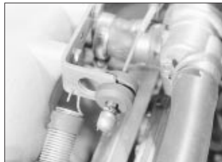
19.7 Throttle cable end grommet in bracket on inlet manifold
