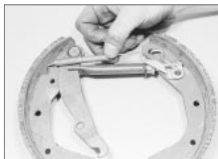
6.22B Fitting the upper return spring to the shoes
