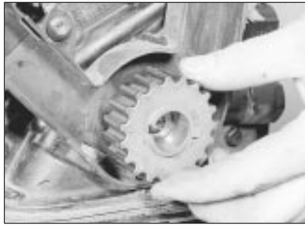
11.21 Crankshaft sprocket fits with flange and pulley locating lug outermost - 1.6 litre engine
