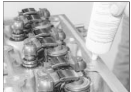
20.35 Apply sealing compound to the cylinder head top mating face
