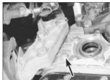
33.2B Transmission oil level plug (arrowed) - F16 type transmission (viewed from below, with driveshaft removed)
