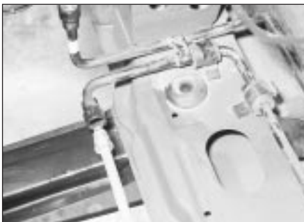
42.2 Power steering fluid cooler pipe unions in engine compartment - 2.0 litre SOHC model
