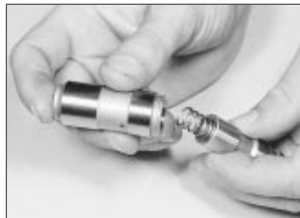
24.10B . . . then slide the plunger and spring assembly into the cylinder
