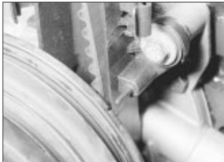
11.7B ...and notch in crankshaft pulley aligned with pointer on rear timing belt cover - 2.0 litre engine
