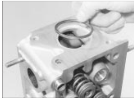
23.9 Renewing the thermostat housing sealing ring - 2.0 litre engine
