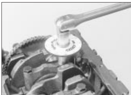
34.27B . . . then through the specified angle - 2.0 litre SOHC engine
