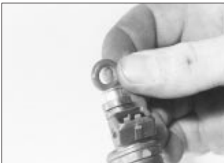
28.9 Fit new seals to the injectors
