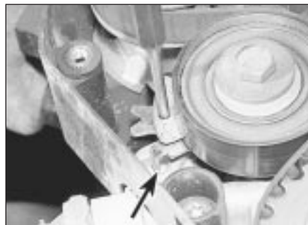
12.2 Using a close-fitting drift to lock the tensioner. Note baseplate lug engaged in oil pump housing (arrowed)
