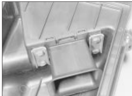
25.3 Airflow meter securing bolts and reinforcing plates, and air funnel
