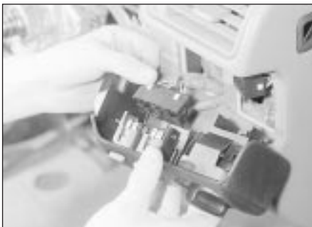
37.22 Disconnecting the wiring plugs from the lighting switches
