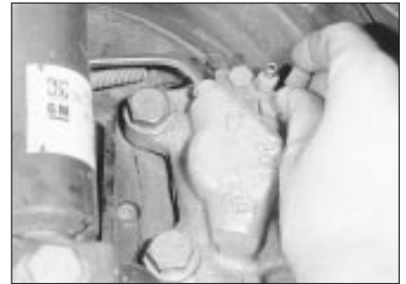
3.5 Removing the dust cap from a rear caliper bleed screw - models with ventilated discs
