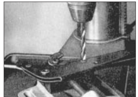
28.13 Drilling out the handbrake lever pawl pivot pin
