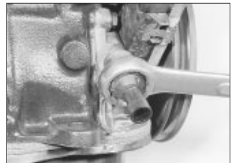
14.4 Unscrewing the oil pressure warning lamp switch - SOHC model (engine removed)
