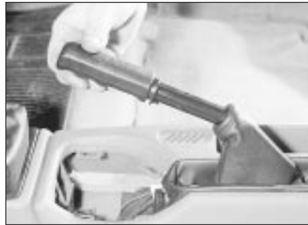
38.3 Pull the grip from the handbrake lever
