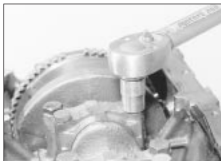
32.18A Tighten the big-end cap bolts to the specified torque . . .
