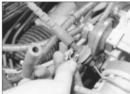
11.2A Extract the throttle cable end clip . . .
