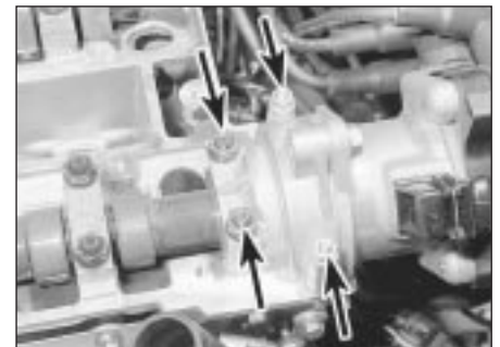
7.4 Exhaust camshaft rear bearing cap securing nuts (arrowed)
