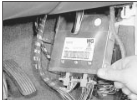
35.3 Withdrawing the fuel injection/ignition system ECU
