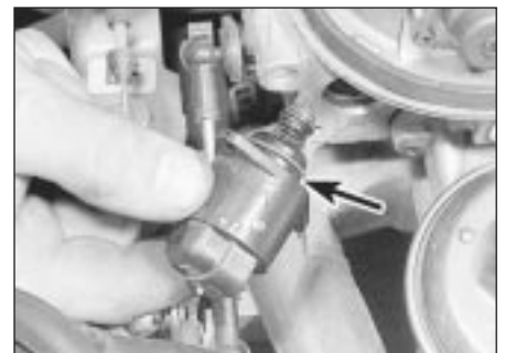
33.4B . . . to remove the stepper motor - renew sealing ring (arrowed)
