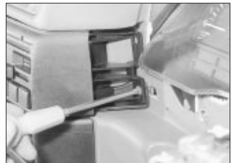
16.4B . . . and the remaining screw from the right-hand end of the panel
