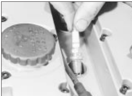
37.2 Removing a spark plug - DOHC model
