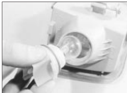
34.10 Withdraw the front indicator lamp bulbholder (lamp removed) . . .
