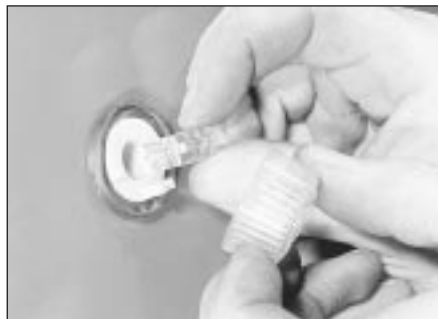
34.14 Removing a front indicator side repeater lamp bulb
