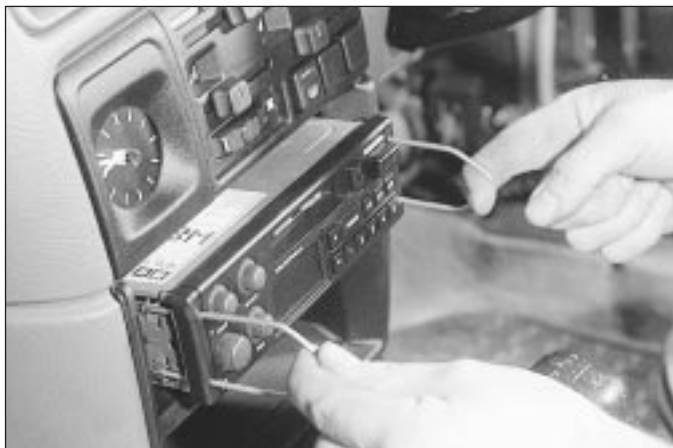
50.4 . . . and withdraw the radio/cassette player using the special tools
