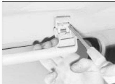
39.2 Removing a grab handle securing screw
