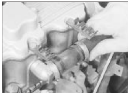
20.19A Disconnecting the crankcase breather tube stub hose - 2.0 litre engine
