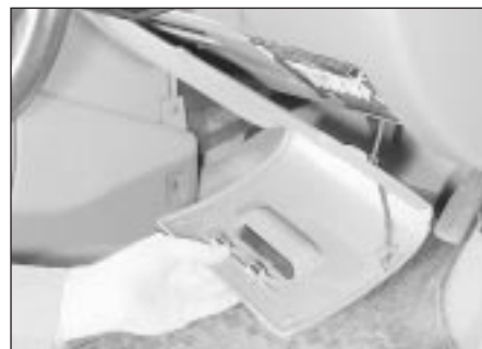
37.5B . . . then withdraw the lower facia panel
