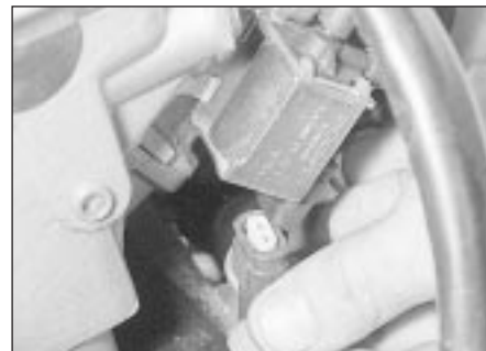
1.6 Disconnecting the fuel tank vent valve wiring
