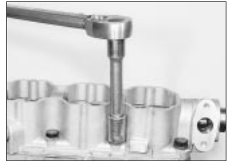
20.37B Tighten the cylinder head bolts to the specified torque . . .
