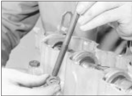
20.36 Fit new cylinder head bolts, ensuring that the washers are in place
