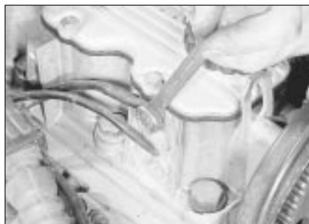
20.10 Unbolting the fuel injection wiring harness earth leads from the camshaft housing - 2.0 litre engine
