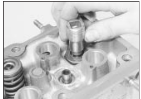
22.14B . . . and push onto the spring seat using a socket
