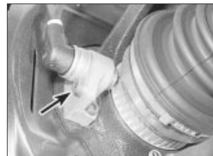
21.4 ABS front wheel sensor securing bolt (arrowed) - DOHC model
