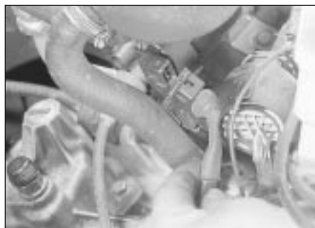
16.3 Disconnecting the coil LT wiring plug - 2.0 litre model
