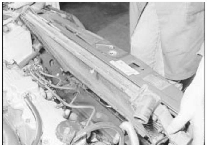
6.7B Withdrawing the radiator - 2.0 litre SOHC model
