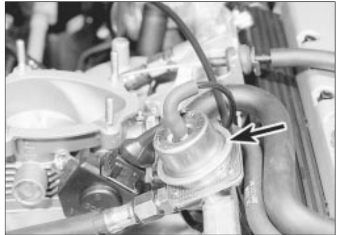
21.17 Fuel pressure regulator (arrowed) - DOHC model
