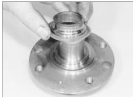
2.4 Removing the half inner bearing race from the hub
