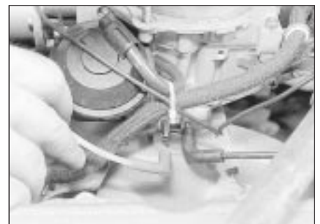
13.6 Disconnecting the air box vacuum pipe from the carburettor - 1.6 litre model
