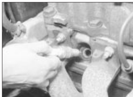
30.3 Removing a spark plug
