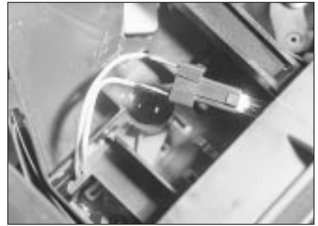
24.20 Heater control panel illumination lamp bulbholder withdrawn
