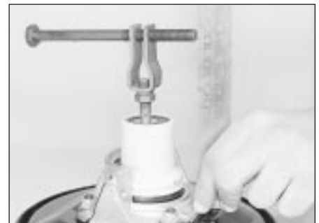
19.15 Measuring the servo operating fork dimension using a bolt inserted through the pivot pin hole
