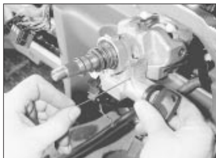
33.11 Removing the lock cylinder - adjustable tilt steering column
