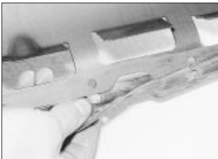
29.13 Locate a new rubber gasket over the sump baffle flange - 2.0 litre engine
