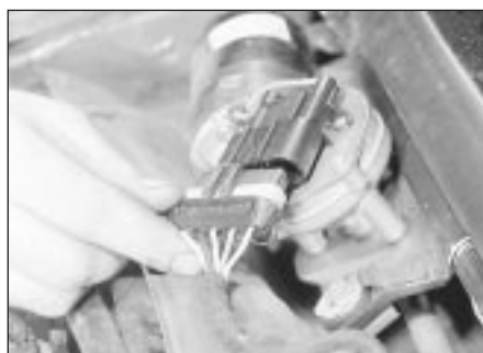
38.4 Disconnecting the windscreen wiper motor wiring plug
