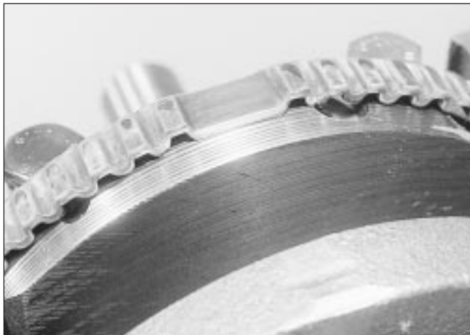
35.9 Check the condition of the TDC sensor wheel teeth at the front of the crankshaft - 2.0 litre SOHC engine
