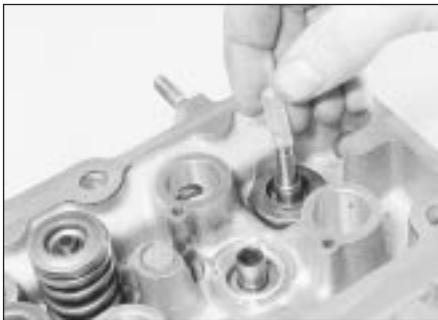
22.13 Slide the oil seal fitting sleeve down the valve stem . . .
