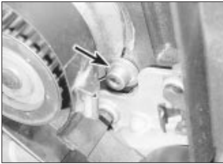
11.4 Coolant pump securing bolt (arrowed) - 2.0 litre SOHC model
