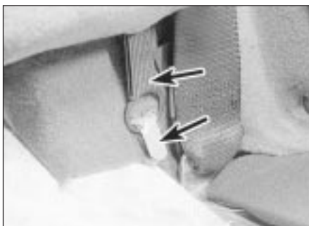
40.19 Seat back-to-body panel securing strap and lug (arrowed)
