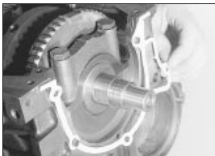
30.7 Fit a new oil pump gasket to the cylinder block - 2.0 litre engine
