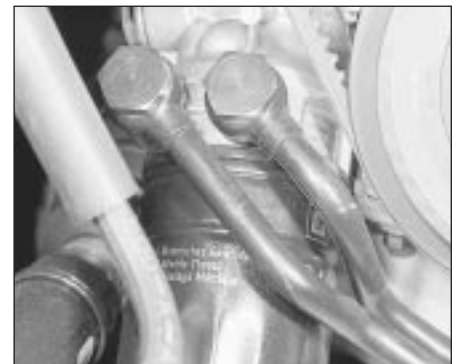
14.2 Oil cooler pipe unions at oil pump
