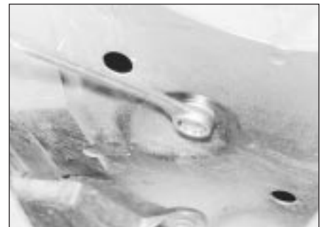
28.4 Unscrewing the right-hand front bumper securing bolt (air cleaner removed)
