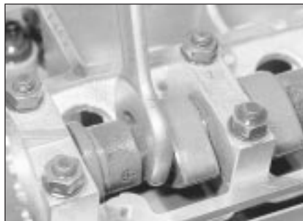
4.14 Spanner positioned to counterhold exhaust camshaft
