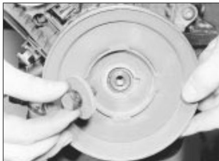
11.24A Refitting the crankshaft pulley - 1.6 litre engine
