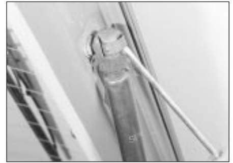
15.2 Prising the spring clip from a tailgate strut balljoint
