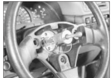
30.7 Two legged puller fitted to remove steering wheel
