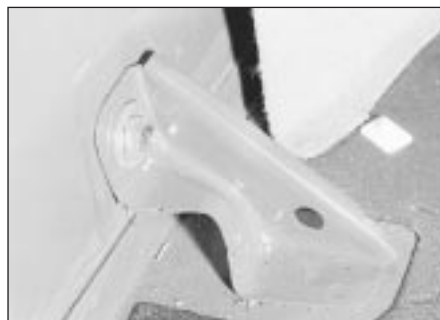
28.8B . . . to expose the bumper securing nuts
