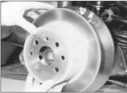
10.18 Withdrawing the rear brake disc - DOHC model
