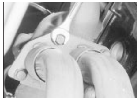
14.11 Unscrewing a downpipe-to-exhaust manifold bolt - SOHC models
