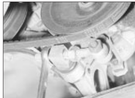
18.4 Adjusting the length of the power steering pump threaded rod
