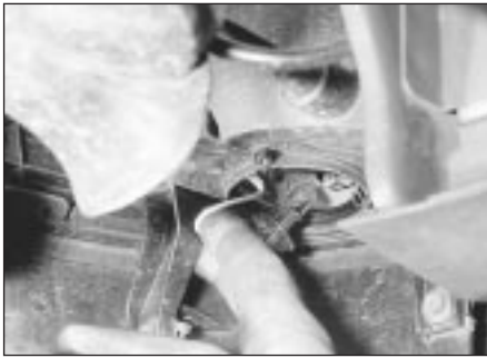
34.19 Withdrawing a foglamp bulb
