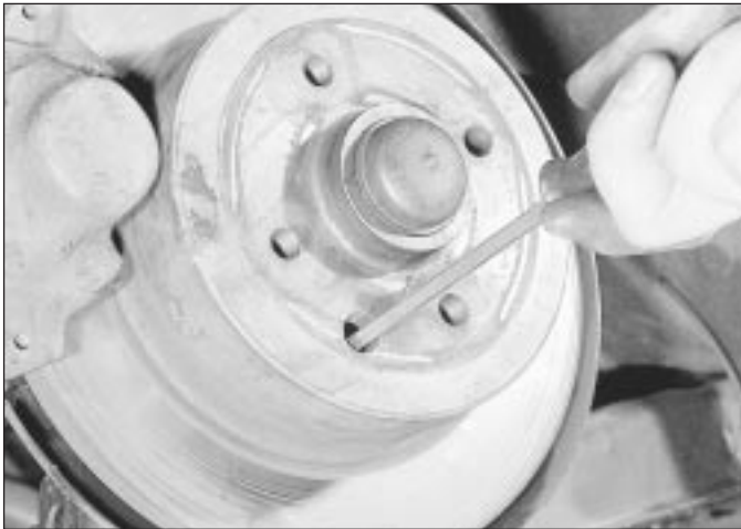
26.14 Using a screwdriver to turn the handbrake adjuster wheel - model with rear disc brakes
