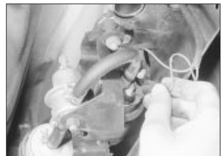
12.4 Disconnecting a fuel pump wiring plug - 'out of tank', fuel pump model
