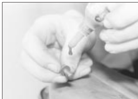
29.17A Coat the sump securing bolts with thread-locking compound before fitting
