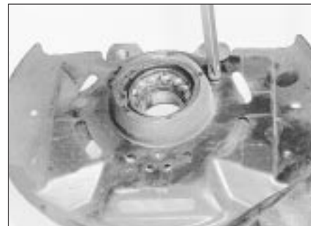
2.5 Removing a brake disc shield securing screw
