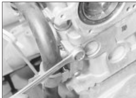
20.19B Unbolting the crankcase breather tube bracket from the cylinder head - 2.0 litre model
