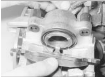
4.24 Removing the inboard pad from the caliper piston - models with ventilated discs
