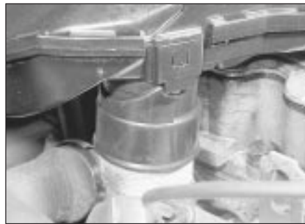
3.3 The air cleaner body locates over the hot air hose
