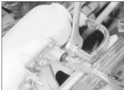
38.5 Disconnecting the brake servo vacuum hose - SOHC models
