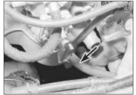
26.5 . . .and the camshaft cover breather hose (arrowed) from the inlet manifold - 1.6 litre model
