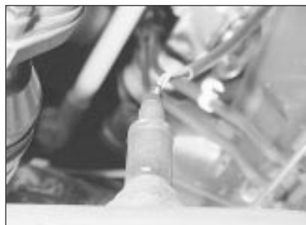
12.6 Oxygen sensor location in front section of exhaust system - DOHC models
