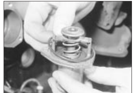
9.15B . . .and recover the O-ring - 2.0 litre SOHC model
