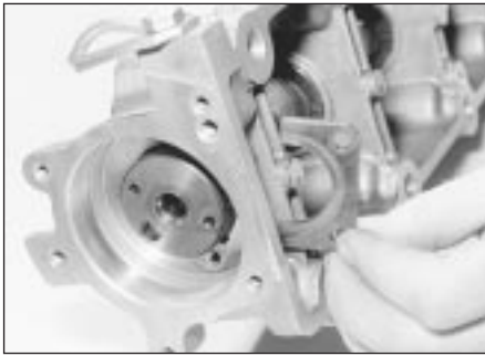
18.5 Removing the camshaft thrustplate - 2.0 litre engine
