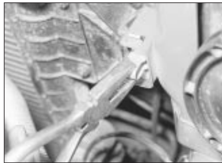
6.6 Compressing a radiator securing clip - 2.0 litre SOHC model
