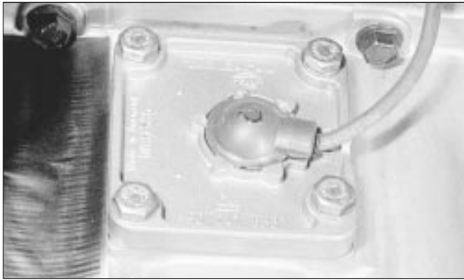
21.18 Engine oil level sensor - DOHC model
