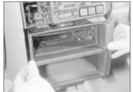
37.29B Manipulating the radio/oddmments tray from the fascia
