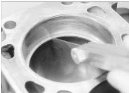
33.6 Measuring a piston ring end gap using a feeler blade
