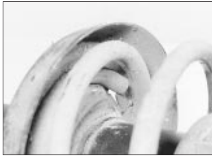
4.22 Lower end of spring rests against lug (arrowed) on lower spring seat
