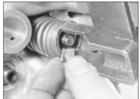
22.17 Retain the split collets with a little grease
