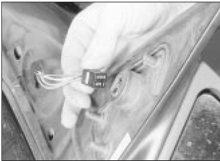
27.7B Withdraw the mirror and disconnect the wiring plug
