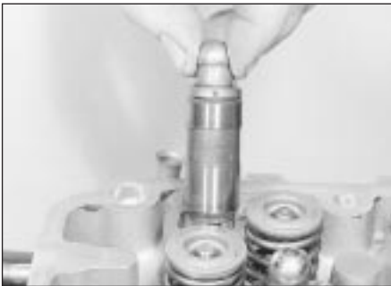
20.26 Lift the hydraulic valve lifters from the cylinder head - 1.6 litre engine
