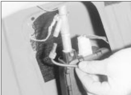
47.4B Disconnecting the aerial lead - electric aerial
