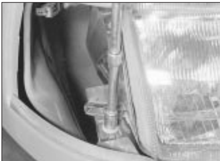
25.5A Unscrewing the lower headlamp securing screw
