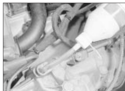
33.3B Topping-up the transmission oil level - F13 type transmission
