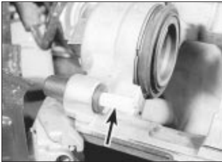
8.20A Extract the nylon compression sleeve (arrowed) . . .
