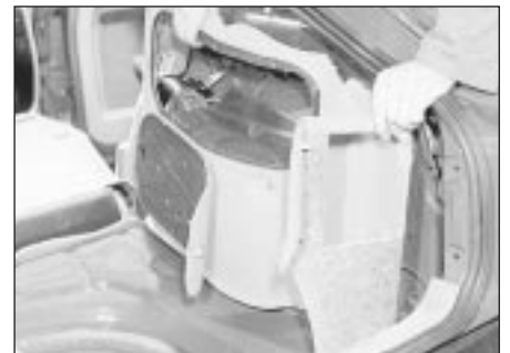
36.19B Withdrawing the lower rear quarter trim panel - Hatchback model
