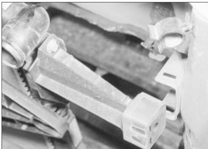
6.7A Radiator freed from top right-hand mounting - 1.6 litre model
