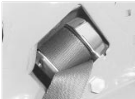
41.13 Rear seat belt inertia reel unit location - Hatchback model
