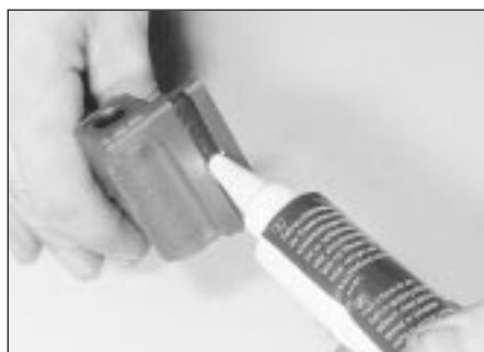
34.25A Fill the side grooves of the rear main bearing cap with RTV jointing compound . . .
