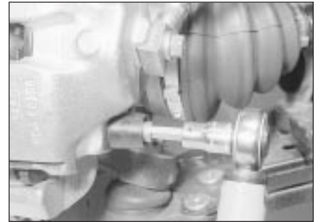
4.29 Tightening a caliper guide bolt - models with ventilated discs
