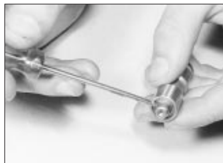
24.9B Locate the cap flange in the plunger groove
