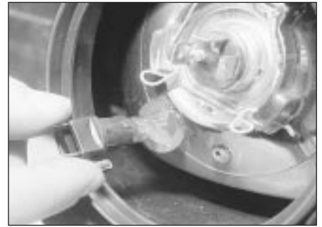
34.6 Pull the sidelamp bulbholder from the headlamp . . .
