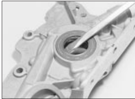
31.9A Prise out the old crankshaft front oil seal . . .
