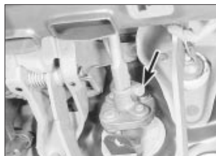
32.4 Steering shaft flexible rubber coupling. Upper pinch-bolt arrowed
