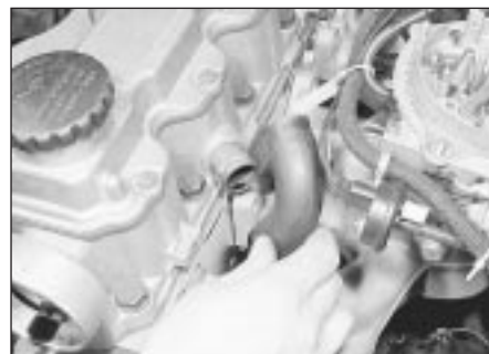
20.11 Disconnecting the crankcase breather tube stub hose - 1.6 litre engine
