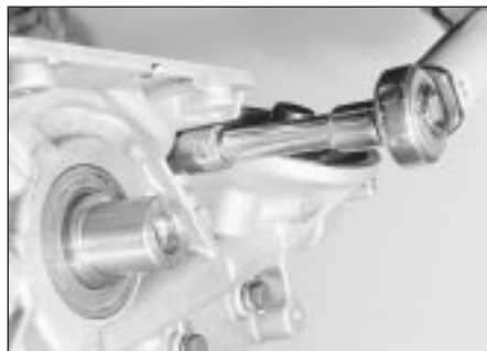
30.9C Tighten the oil pump securing bolts to the specified torque - 2.0 litre SOHC engine
