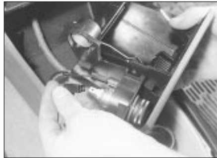
38.11 Disconnecting the wiring plugs from the cigarette lighter
