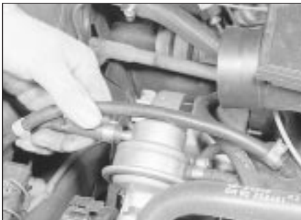
7.14A Disconnecting a fuel hose from the fuel pump - 1.6 litre model
