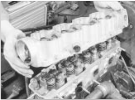
20.24 Lifting the camshaft housing from the cylinder head - 1.6 litre engine
