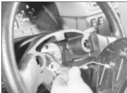
30.3 Disconnecting the horn push pad wiring
