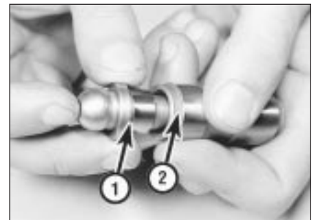
24.11 Slide the collar (1) over the top of the plunger and engage with the groove (2) in the cylinder
