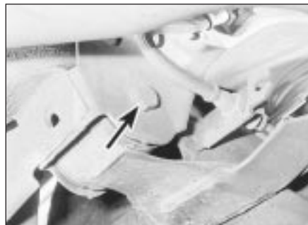
17.9 Trailing arm securing bolt (arrowed)
