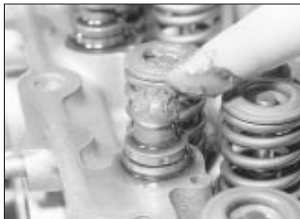
20.33 Lubricate the valve lifter contact faces with molybdenum disulphide grease
