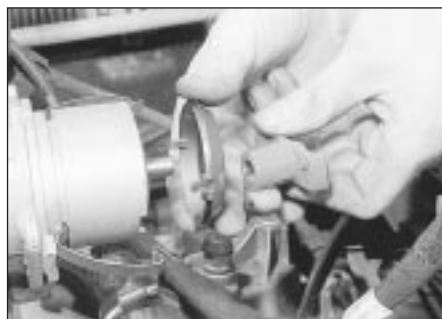
17.5 Removing the rotor arm and plastic shield - 1.6 litre model (Bosch distributor)
