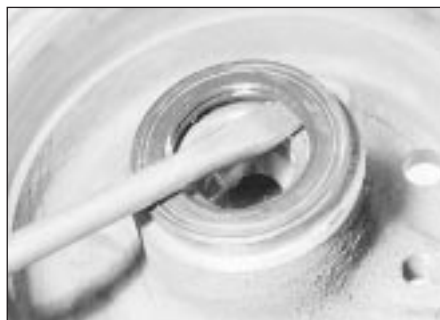
11.4 Prise the oil seal from the inner end of the hub - model with rear disc brakes
