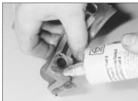
34.25B . . . and the lower surfaces with sealing compound - 2.0 litre SOHC engine
