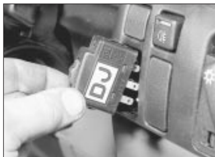
27.4 The headlamp aim adjustment switch - 1992-on models
