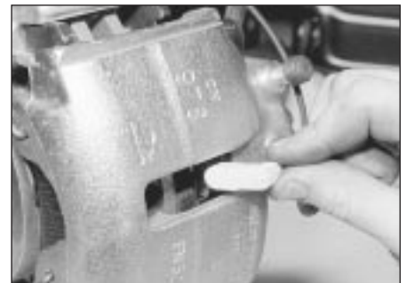
4.21 Withdrawing the pad wear sensor from the inboard pad - DOHC model
