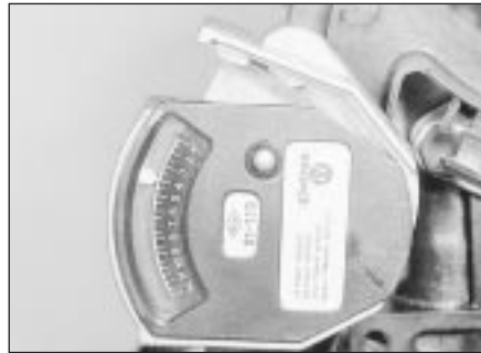
11.35 Note the reading on the scale of the tension gauge - 1.6 litre engine
