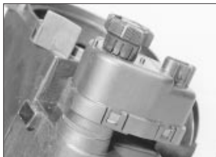
26.2A Headlamp aim adjustment motor (headlamp removed)
