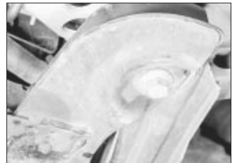
3.10B Front subframe rear securing bolt which also secures rear end of lower arm
