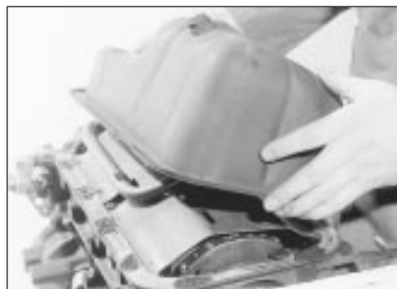
29.17B Refitting the sump - 2.0 litre engine
