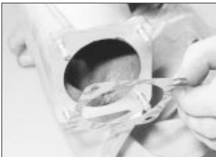
31.15 Refit the throttle body, using a new gasket
