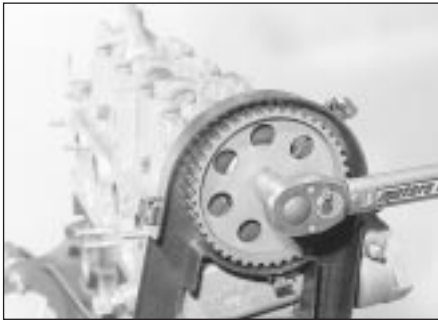
11.22B ... and tighten the securing bolt to the specified torque - 2.0 litre engine
