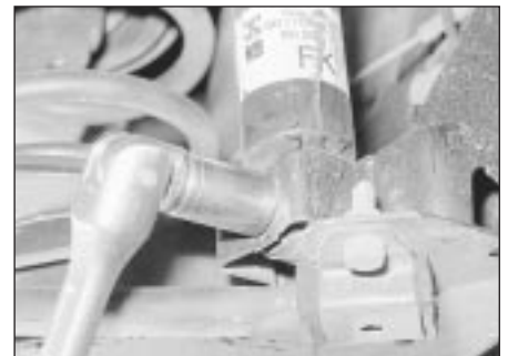
14.7 Unscrewing a rear shock absorber lower mounting bolt - SOHC models
