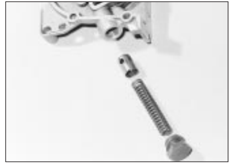
31.7 Oil pressure relief valve components - 2.0 litre SOHC engine
