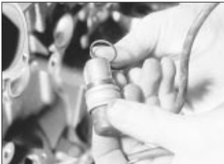
24.18 Examine the crankshaft speed/position sensor sealing ring - 1.8 litre model
