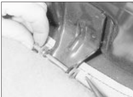
40.7 Removing a rear seat cushion hinge pin - SOHC models
