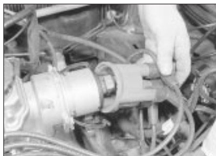
17.3A Removing the distributor cap - 1.6 litre model (Bosch distributor) . . .
