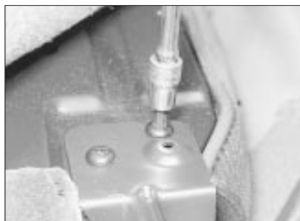
40.21 Extracting a hinge-to-seat back securing screw
