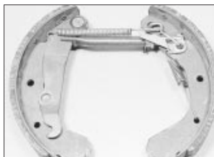
6.22C Adjuster lever spring fitted to leading shoe
