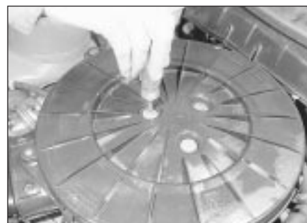
27.3 Air cleaner-to-carburettor mounting cap nuts
