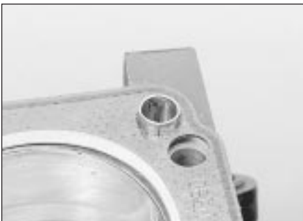
20.31B Cylinder head gasket correctly located over dowel in cylinder block
