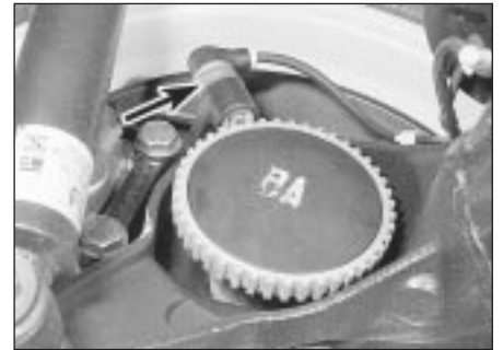
21.14 ABS rear wheel sensor (arrowed) - DOHC model
