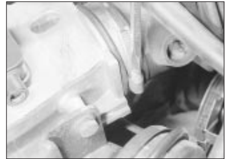
4.2 Loosening the air trunking clamp screw at the airflow meter
