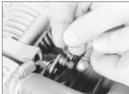
19.4 Disconnecting the throttle cable end from the throttle valve lever - SOHC model
