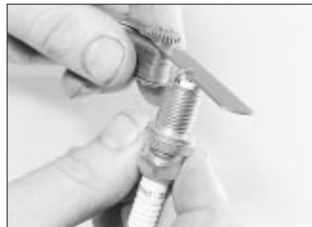
30.9C Measuring the spark plug gap with feeler blade
