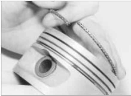
33.5B Removing the centre section of the oil control ring - 2.0 litre SOHC engine
