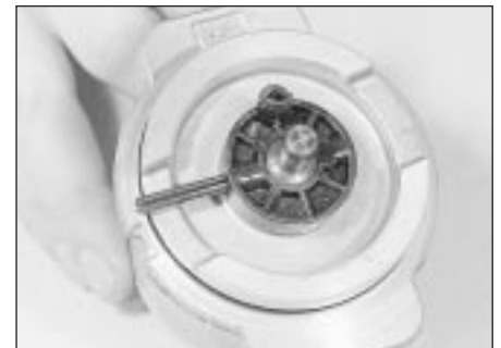
20.12 Removing the drive collar roll pin - 1.6 litre models (Bosch distributor)
