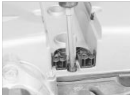
4.12 Unscrewing a camshaft cover securing bolt
