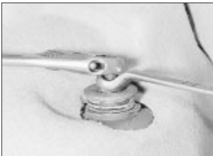
14.4 Unscrewing a rear shock absorber top mounting nut - Hatchback model
