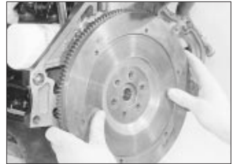
25.5 Removing the flywheel - 1.6 litre engine
