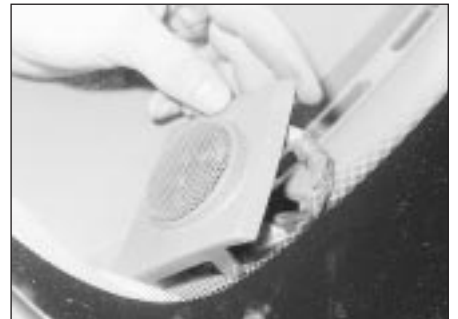
49.2 Removing a facia-mounted speaker (viewed through windscreen)
