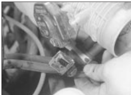
23.2 Disconnecting the throttle position sensor wiring plug - early SOHC models
