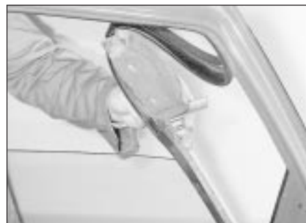
25.13B . . . then withdraw the guide rail from the door
