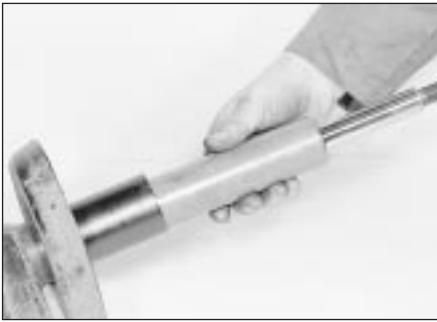
4.17B ... and withdraw the shock absorber cartridge
