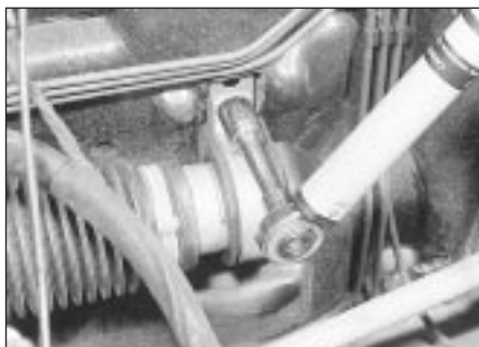
37.13 Tightening a steering gear mounting bolt
