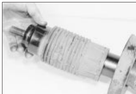
4.15 Slide off the bellows and the rubber buffer
