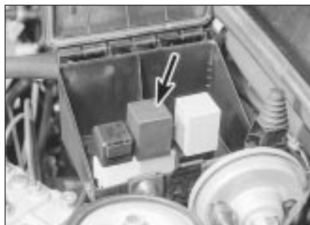
23.9 ABS surge arrester relay (arrowed)
