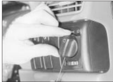
7.2 Using a thin rod to depress the lightning switch knob retaining clip
