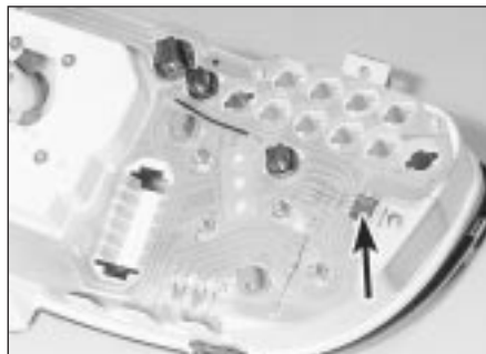
19.5 Instrument panel voltage stabiliser (arrowed)
