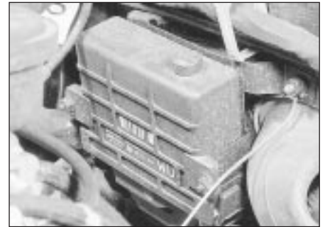
23.6 MSTS-i module location - 1.6 litre model
