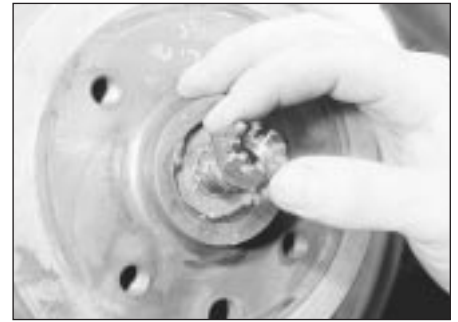
13.17B . . . and the hub nut - model with rear disc brakes
