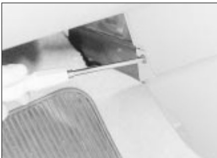
38.13 Unscrewing a side centre console-to-facia securing screw
