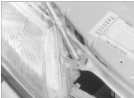
25.5B Unscrewing an upper headlamp securing screw
