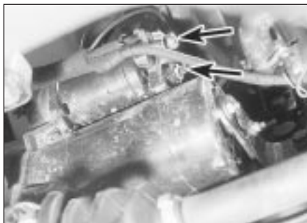
14.4 Starter motor and solenoid viewed from underneath the vehicle. Solenoid wiring connections arrowed
