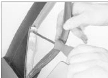
25.12 Unscrewing the window rear guide rail securing screw
