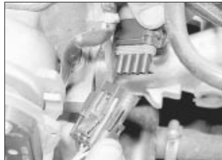
18.3B Disconnecting the distributor wiring on the C16 NZ engine
