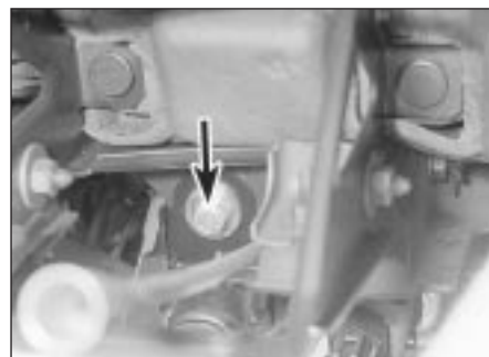
33.13 Steering column to dashboard mounting bracket bolt (arrowed)
