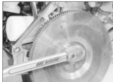
25.13B Tighten the flywheel securing bolts to the specified torque . . .
