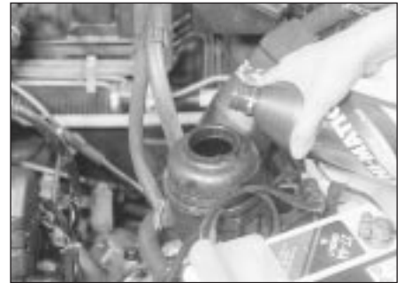
17.2 Topping-up the power steering fluid level
