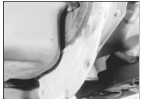
7.20 Removing the transmission bellhousing cover plate
