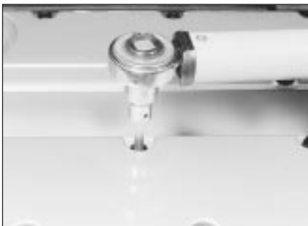
4.24 Tightening a camshaft cover securing bolt
