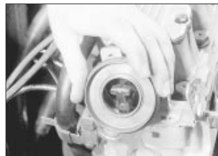
17.9 Removing the plastic shield from the rotor arm housing - 2.0 litre model
