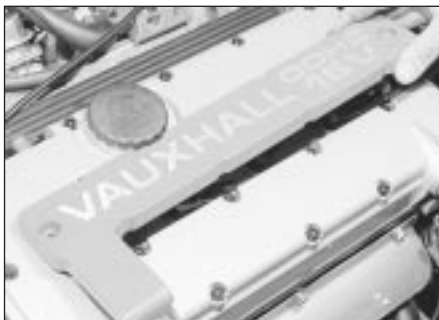
4.11 Removing the spark plug cover
