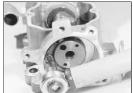
18.13 Tightening a camshaft thrustplate securing bolt - 2.0 litre engine
