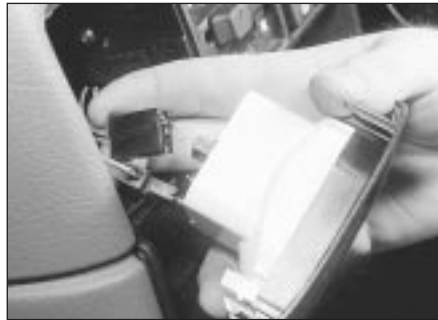
16.3 Disconnecting the wiring plugs from the clock
