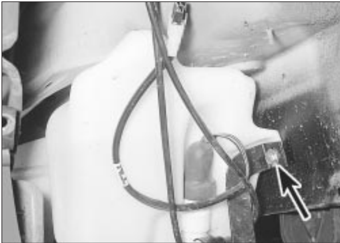
41.17 Horn/washer fluid reservoir support bracket securing bolt (arrowed) - model with headlamp wash
