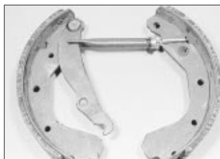
6.22A Right-hand adjuster strut correctly fitted to shoes
