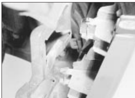
28.5 Front bumper retaining clips released from body
