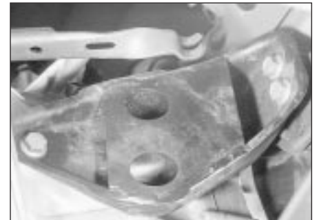
8.12 Left-hand transmission mounting viewed from underside of vehicle
