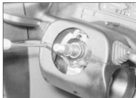
37.9B . . . then remove the front column shroud securing screws
