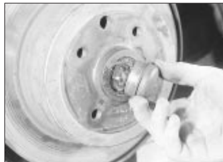
10.2 Removing the dust cover from the rear hub - model with rear disc brakes
