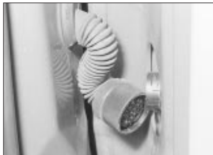
16.3 Disconnect the wiring connector from the front edge of the door
