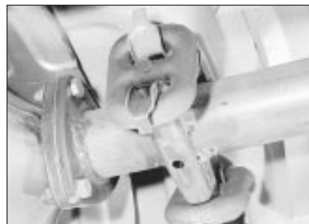
14.28 Exhaust centre section forward rubber mountings - DOHC models
