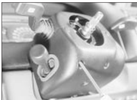
37.10A Remove the three lower column shroud securing screws . . .
