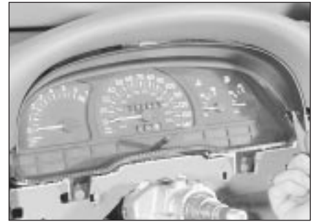
37.17 Withdrawing the instrument panel upper trim panel
