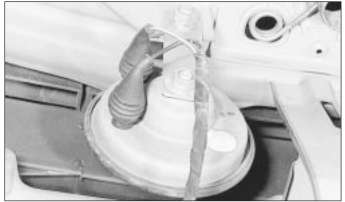
22.5 Horn viewed from behind with radiator removed - single horned model
