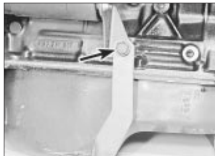
14.5 Starter motor mounting bracket/exhaust bracket securing bolt (arrowed) - 1.6 litre model
