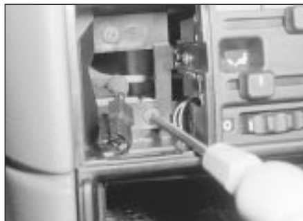
16.4A Remove the two heater control panel securing screws from the clock/trip computer aperture . . .
