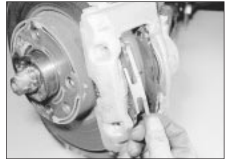
4.7 Removing an anti-rattle spring - models with solid discs
