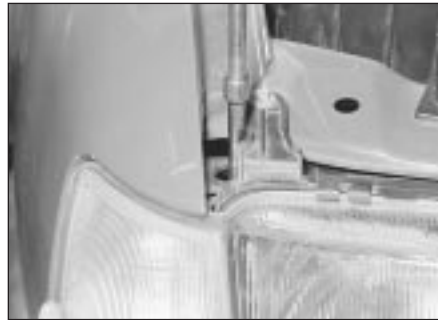
29.2 Unscrewing the front indicator lamp unit securing screw
