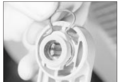
17.2 Window regulator handle securing clip
