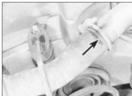
14.26 Exhaust centre section-to-rear section clamp (arrowed) - SOHC model
