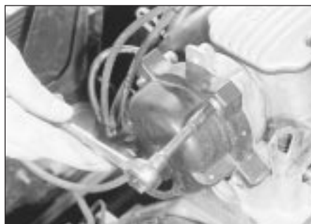
17.8 Unscrewing a distributor cap securing screw - 2.0 litre model
