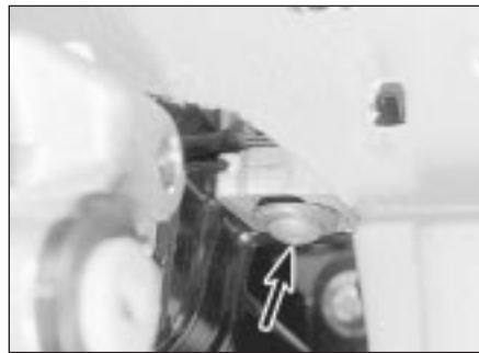
33.14 Column upper mounting shear head bolt (arrowed)
