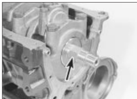
30.9A Oil pump inner gear must engage with hexagon flats on crankshaft (arrowed) on 1.4 and 1.6 litre engines . . .
