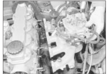
26.11 Withdrawing the inlet manifold - 1.6 litre model
