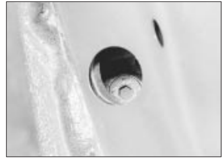
19.10B . . . to expose the servo securing bolts
