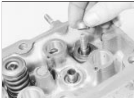
22.14A . . . then fit the valve stem oil seal . . .
