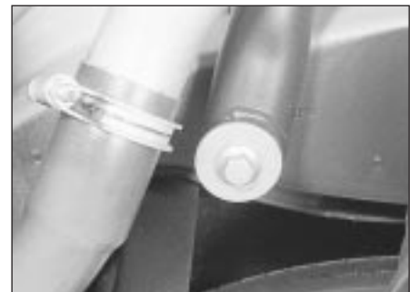
26.9 Rear suspension crossmember rear tube securing bolt - DOHC model
