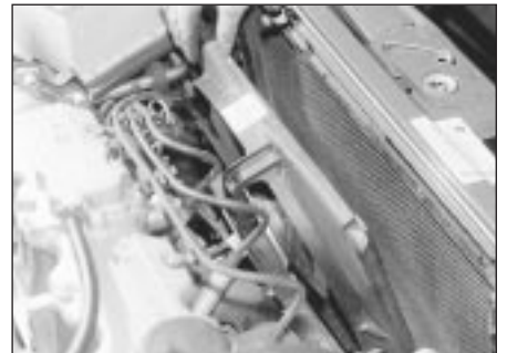
12.3 Withdrawing the fan shroud assembly - 2.0 litre SOHC model
