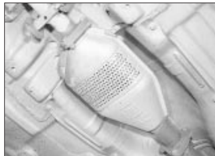
10.9 The catalytic converter is protected by heat shields
