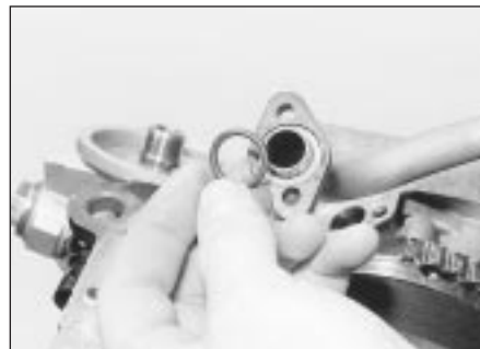
29.15A Fit a new O-ring to the oil pick-up pipe . . .
