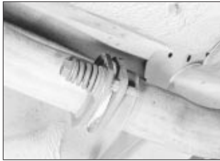
14.9 Exhaust front section flexible joint - SOHC models
