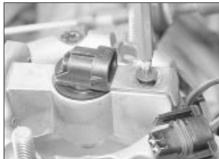
29.5 Unscrewing the injector retainer Torx screw
