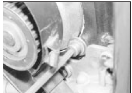
11.8 Loosening a coolant pump securing bolt - 2.0 litre engine
