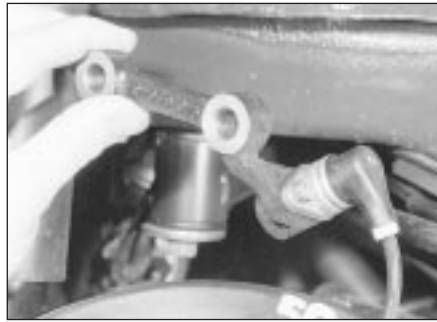
9.5B . . . which also secures the ABS sensor bracket - DOHC model
