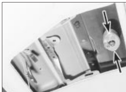
34.23 . . . to expose the crank drive - securing screws arrowed
