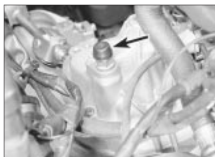
33.3A Transmission breather/filler plug (arrowed) - F16 type transmission
