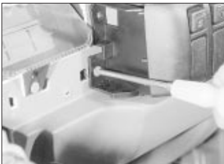
37.20 Removing the lower left-hand lighting switch panel securing screw
