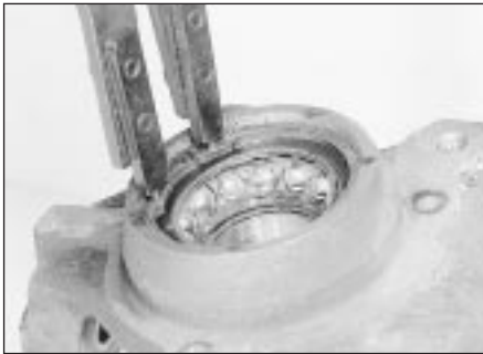
2.6 Extracting the outer bearing retaining circlip
