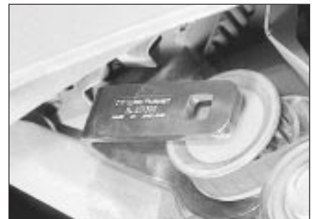
12.8 Using a special spanner to adjust the timing belt by moving the coolant pump
