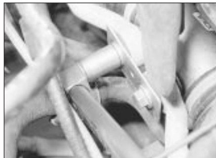
37.4B . . . then unscrew and remove the tie-rod to steering gear bolts
