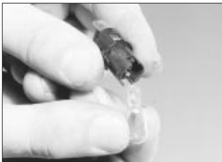
34.07 . . . then pull the bulb from the bulbholder
