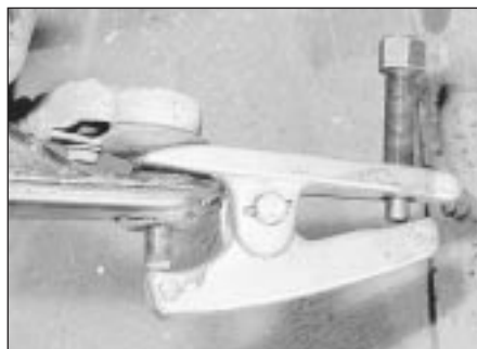
43.04 Disconnecting the tie-rod end to suspension strut balljoint
