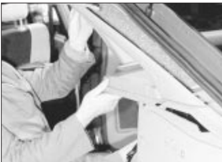
36.17 Withdrawing the upper rear quarter trim panel - Hatchback model
