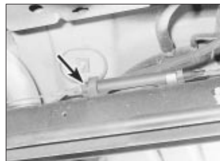
26.4 Handbrake cable adjuster. Knurled nut arrowed - all SOHC models
