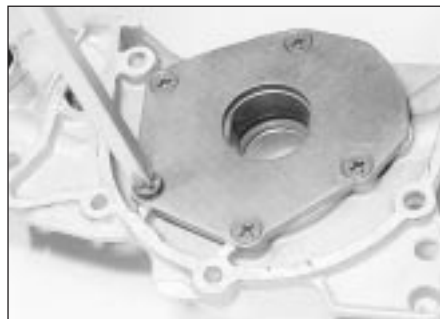
31.2 Removing an oil pump rear cover securing screw - 2.0 litre SOHC engine
