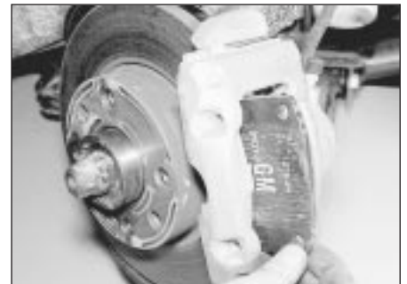
4.8 Withdrawing the outboard disc pad - models with solid discs
