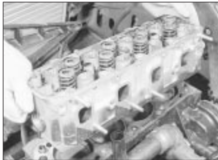
20.27 Lifting the cylinder head from the cylinder block - 1.6 litre engine
