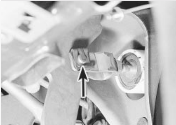
29.4 Brake servo fork-to-pedal pivot pin spring clip (arrowed)
