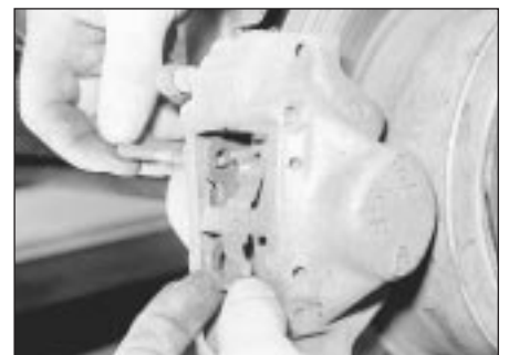
5.5 Removing a rear disc pad retaining pin anti-rattle spring
