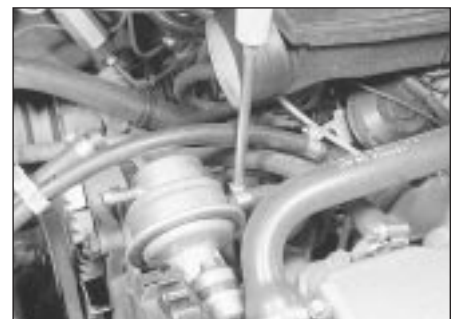
6.3 Disconnecting a fuel hose from the fuel pump - 1.6 litre model
