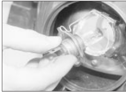
34.3B . . . and withdraw the headlamp bulb
