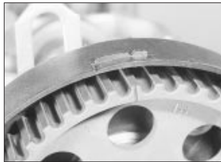
11.7A Camshaft sprocket TDC mark aligned with notch in rear timing belt cover ...
