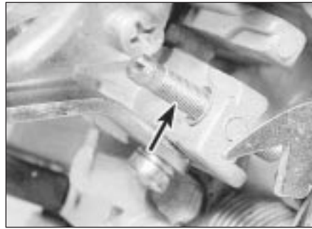
14.3 Carburettor idle speed adjustment (throttle stop) screw (arrowed)
