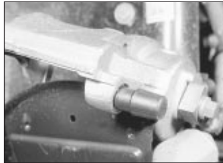
8.20B . . . then withdraw the caliper locating pin rubber - model with solid discs
