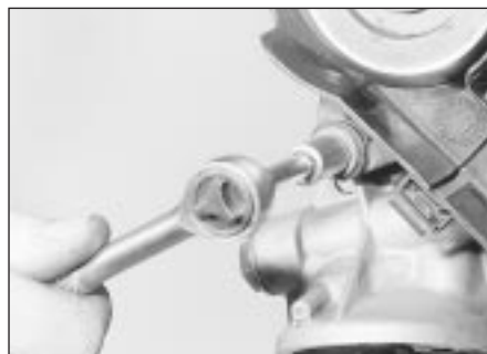
11.18 Unscrewing the coolant pump rear belt cover securing bolt - 2.0 litre engine
