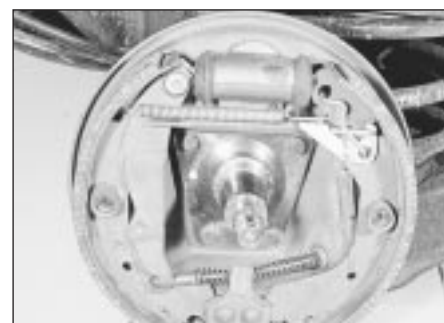
6.24 Rear brake components correctly assembled (hub removed for clarity)
