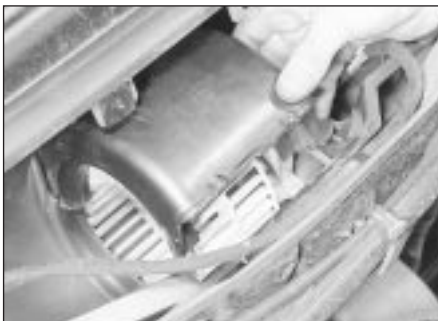
18.4 Unclip the cover from the heater blower motor
