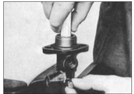
16.25 Depressing the secondary piston while extracting the stop screw - ATE type master cylinder
