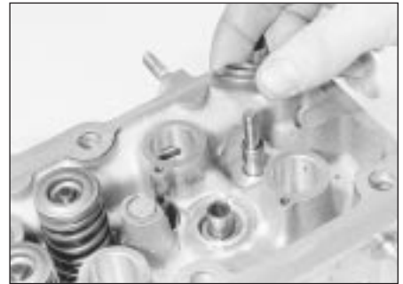
22.12 Fit the valve seat (exhaust valve shown)
