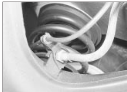
26.5 Brake fluid line/ABS sensor wire bracket and locking clip on semi-trailing arm - DOHC model
