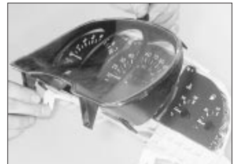
19.8 Removing the instrument panel shroud
