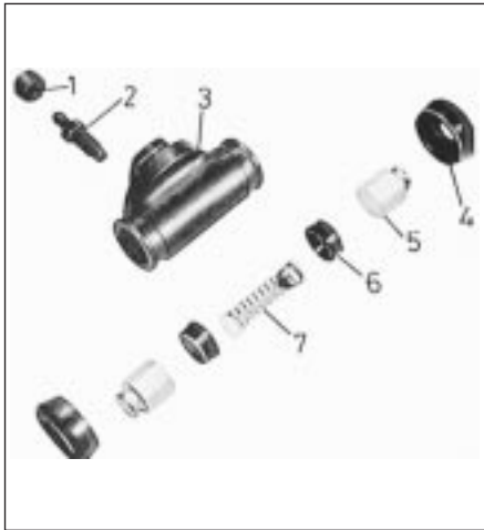
12.13A Exploded view of a rear brake wheel cylinder
