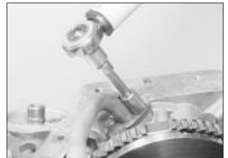
29.15B . . . and tighten the securing bolts to the specified torque - 2.0 litre engine
