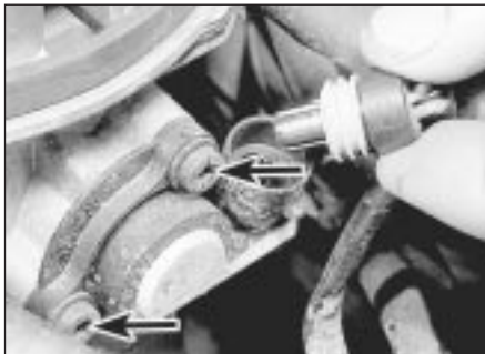
34.2 Disconnecting the throttle potentiometer wiring plug - note the mounting screws (arrowed)
