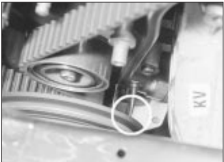
4.6B ...and notch in crankshaft pulley aligned with pointer on rear timing belt cover (circled)
