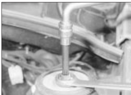
4.7 Unscrewing the suspension strut top mounting nut
