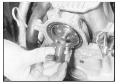
17.10B . . .and withdraw the rotor arm - 2.0 litre model
