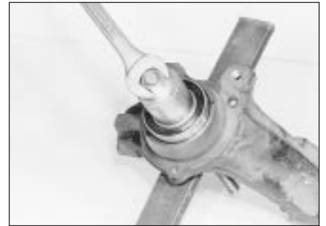
2.9 Fitting a new front wheel bearing using a socket, nut, bolt, washers, and length of bar
