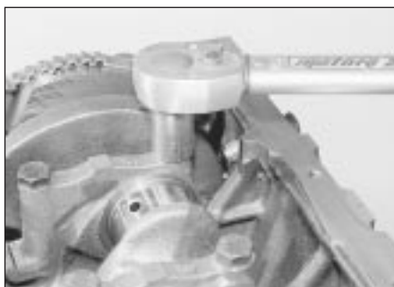
34.27A Tighten the main bearing cap bolts to the specified torque . . .
