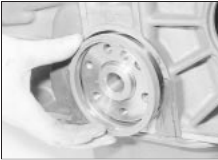
28.4 Fitting a new crankshaft rear oil seal - 2.0 litre engine
