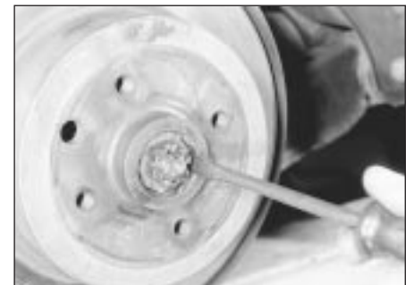
10.5 Loosen rear hub nut until spacer washer can be moved with a screwdriver - model with rear disc brakes
