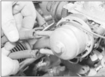
7.11A Disconnect the coolant hoses from the automatic choke housing . . .
