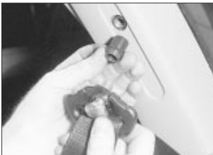
41.9 Removing a rear seat belt upper mounting from the body pillar - Hatchback model
