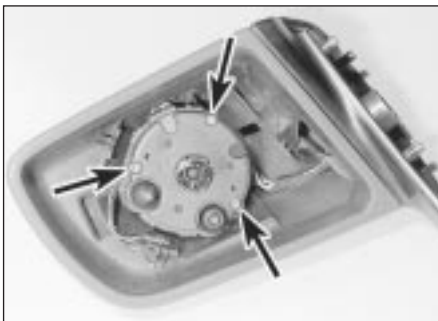
27.10 Mirror motor securing screws (arrowed)
