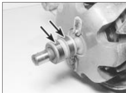
11.4 Alternator slip rings (arrowed) - Delco-Remy alternator
