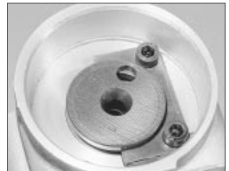
18.4 Camshaft thrustplate and securing bolts - 1.6 litre engine
