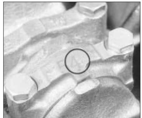
32.3 Big-end cap centre punch identification marks (circled). Note that lug on bearing cap faces flywheel end of engine - 2.0 litre SOHC engine
