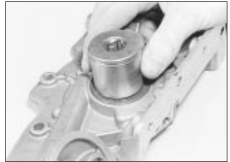
31.9B . . .and fit the new seal using a socket - 2.0 litre SOHC engine
