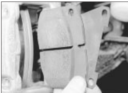
4.9 Withdrawing the inboard disc pad and shim - models with solid discs
