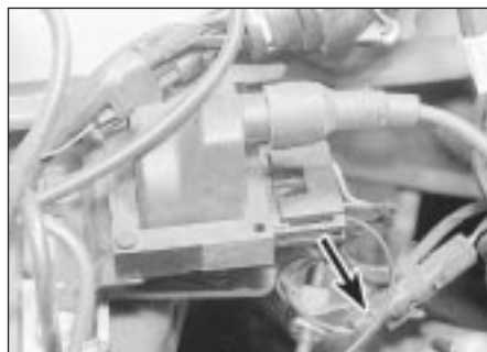
16.1 Ignition coil - 1.6 litre models - note ignition timing basic adjustment coding plug (arrowed)
