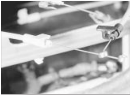
16.5 Heater control cables disconnected, showing cable end securing clips
