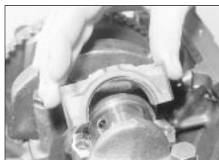
32.17 Fitting a big-end bearing cap - 2.0 litre SOHC engine
