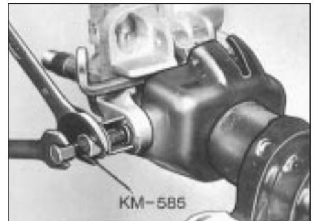
34.19 Extracting the bearing housing fulcrum pins using special tool KM-585 - adjustable tilt type steering column
