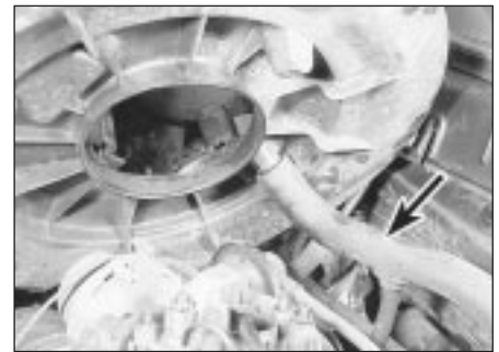
3.4 Disconnecting the crankcase ventilation hose (arrowed)
