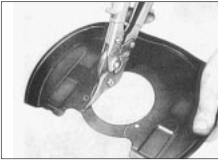
14.4 Cutting a section of metal from a new front brake disc shield prior to fitting
