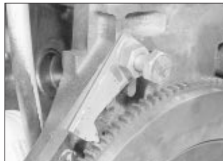
25.13A Tool for locking flywheel fitted to engine-to-transmission bolt hole - 1.6 litre engine
