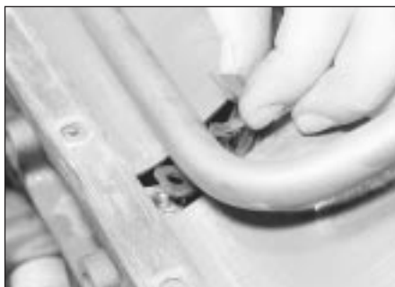
29.16 Refitting the oil pick-up pipe bracket - 2.0 litre engine
