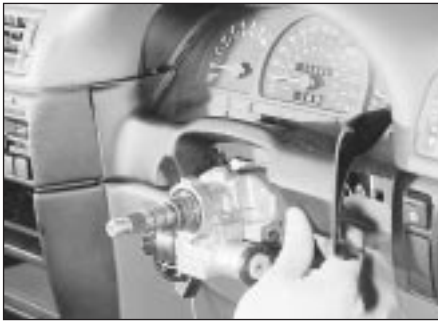
37.13 Removing the instrument panel lower trim panel
