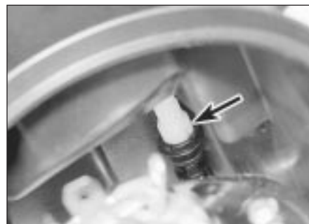
26.2B Headlamp aim adjuster balljoint (arrowed)
