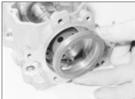
18.11B Fitting a new camshaft rear oil seal - 2.0 litre engine
