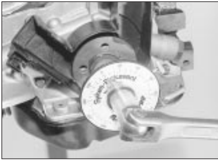
11.20F ...then through the specified angle - 2.0 litre engine
