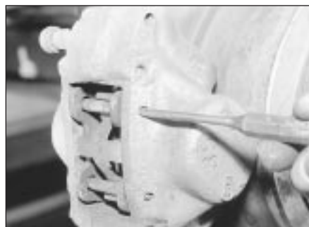
5.4 Driving out a rear disc pad retaining pin
