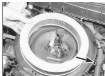
27.4 Removing the air cleaner element - note clip for crankcase ventilation hose (arrowed)
