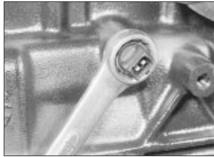
24.11 Unscrewing the MSTS-i oil temperature sensor - 1.6 litre model (engine removed)
