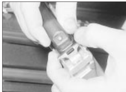
22.4B . . . and release the wiring plug retaining clip - ABS-2E system
