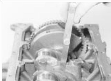
34.30B . . . or a feeler blade - 2.0 litre SOHC engine
