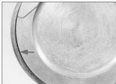
32.14A Piston crown arrow must point towards timing belt end of engine - 1.6 litre engine
