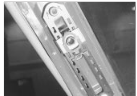
41.15 Upper rear quarter trim panel removed, to expose upper seat belt mounting height adjuster
