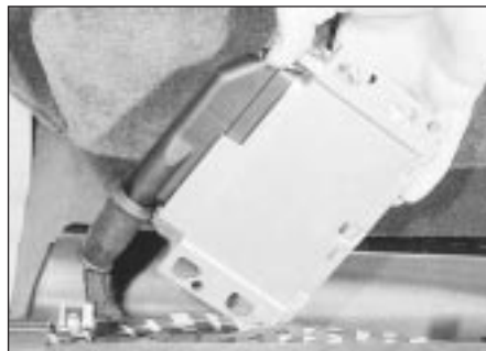
22.4A Lift out the ABS control module . . .
