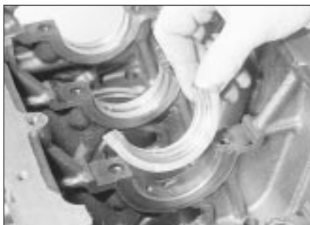
34.19 Fitting a central main bearing shell. Note thrust flanges - 2.0 litre SOHC engine
