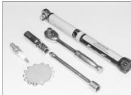
30.9A Tools required for spark plug removal, gap adjustment and refitting
