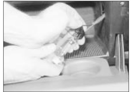
37.34 Prise out the glovebox lamp and disconnect the wiring
