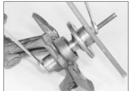
2.12 Drawing the hub into the bearing using improvised tools
