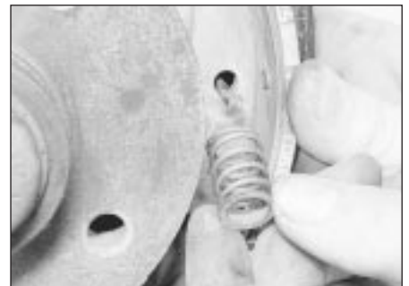
6.9B . . . then withdraw the cup and spring
