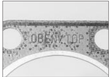
20.31A Cylinder head gasket "Oben/TOP" markings
