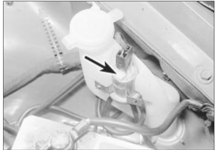
43.1 Headlamp washer fluid non-return valve (arrowed)
