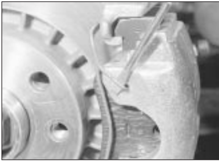
4.22 Prising out the disc pad retaining clip - models with ventilated discs
