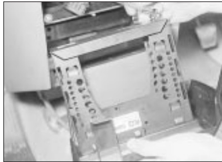
37.30B . . . then disconnect the wiring and aerial plugs
