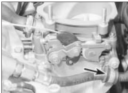
31.23 Remove the fuel hose bracket (arrowed) from the throttle body - DOHC models
