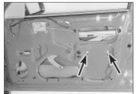
25.5 Window lower guide rail securing screws (arrowed)
