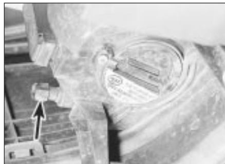
31.7 Foglamp aim adjustment screw (arrowed)
