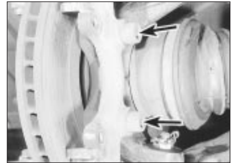
8.31 Caliper bracket securing bolts (arrowed) - model with ventilated discs
