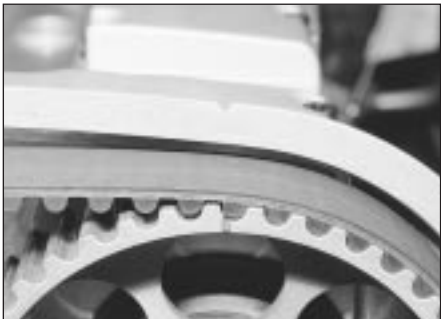
4.6A Camshaft sprocket TDC mark aligned with notch in camshaft cover
