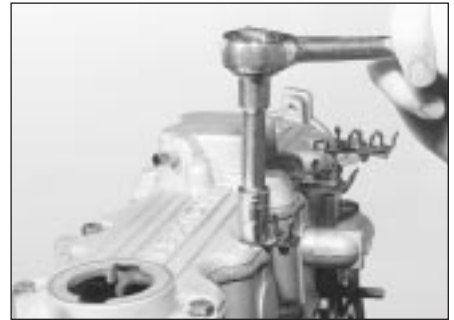
11.22D ... fit the cover and tighten the bolts. Note position of HT lead brackets
