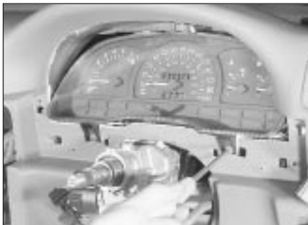
18.4 Unscrewing a lower instrument panel securing screw
