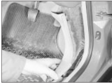
36.5 Removing the driver's footwell side trim panel
