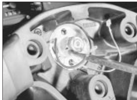
30.4 Prising back the tabs on the steering wheel retaining nut lockwasher
