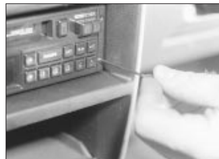
50.3 Unscrew the grub screws . . .
