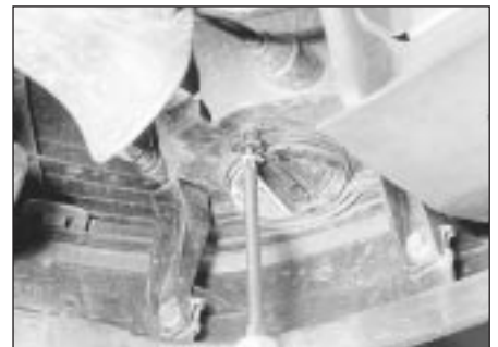
34.18 Removing a front foglamp cover securing screw
