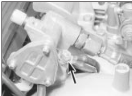
28.24 Earth leads secured to fuel rail stud (arrowed) - DOHC model
