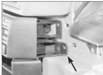
37.29A Right-hand securing lug (arrowed) behind heater control panel
