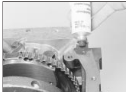
29.12B Applying sealing compound to the joint between the oil pump and cylinder block - 2.0 litre engine
