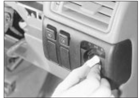
7.3A Press the switch securing clips towards the switch spindle . . .
