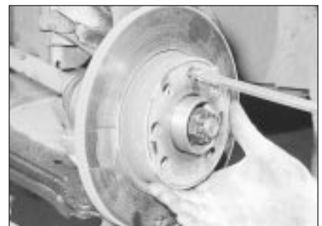
10.12 Removing a disc securing screw - SOHC model
