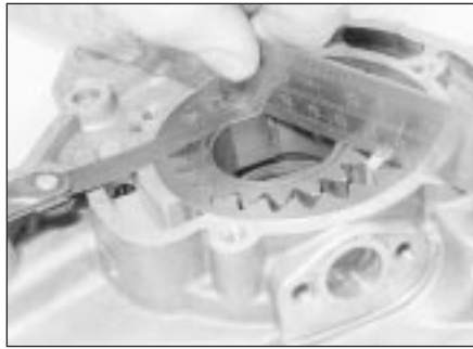
31.4 . . .and between the edges of the gears and the housing - 2.0 litre SOHC engine
