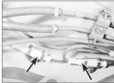
21.12 ABS rear wheel sensor wiring connectors (arrowed) on rear underbody - DOHC model
