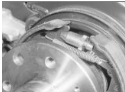
7.26 Handbrake shoe adjuster and upper return spring correctly fitted - DOHC models
