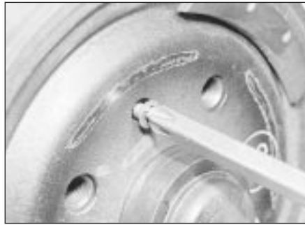
6.6A Extracting a brake drum securing screw
