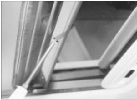
34.2A Extract the four securing screws . . .
