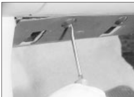
37.2 Releasing a footwell trim panel securing clip
