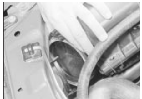
34.2 Removing the cover from the rear of the headlamp
