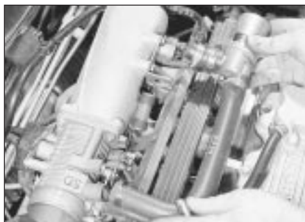
22.4 Withdrawing the idle speed adjuster complete with hoses - SOHC model (except with Multec systems)
