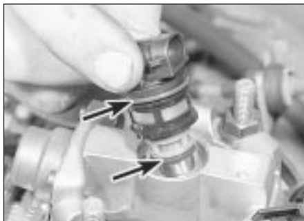
29.6 Renew injector sealing rings (arrowed)
