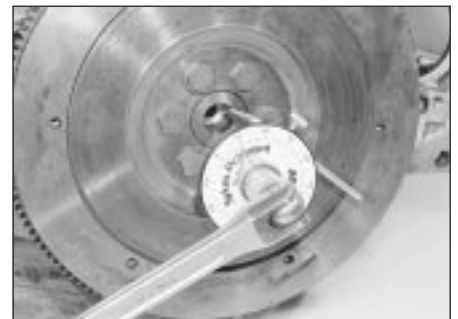
25.13C . . . and then through the specified angle - 1.6 litre engine
