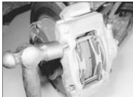
4.15 Fitting a disc pad retaining pin - models with solid discs
