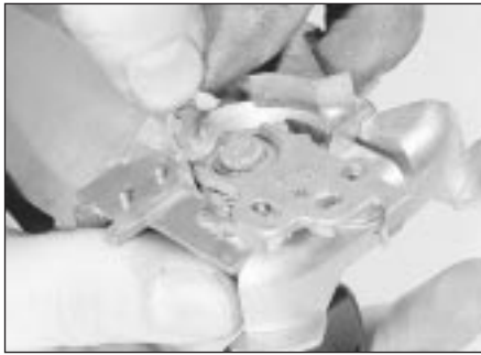
20.2 Extract the circlip from the end of the lock cylinder . . .
