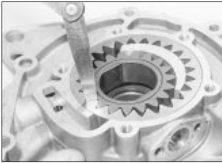
31.3 Check the clearance between the inner and outer gear teeth . . .
