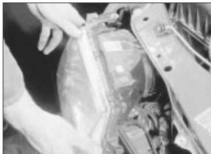
25.5C Withdrawing a headlamp unit
