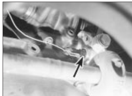
14.2 Oil pressure warning lamp switch (arrowed) viewed from underneath vehicle - SOHC model
