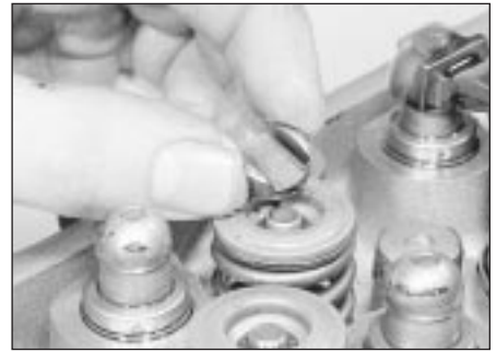
20.25B . . . and their thrust pads from the cylinder head - 1.6 litre engine
