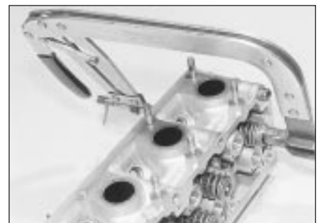
22.3 Valve spring compressor tool fitted to No 1 exhaust valve - 2.0 litre engine
