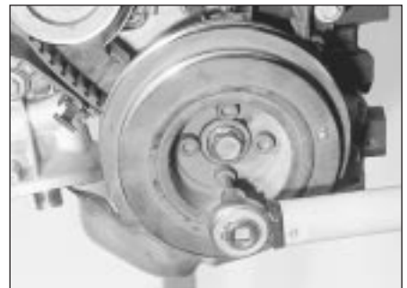
11.24B Tightening a crankshaft pulley securing bolt - 2.0 litre engine
