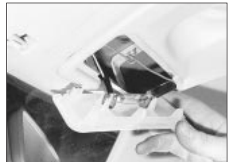
23.2 Withdrawing the courtesy lamp
