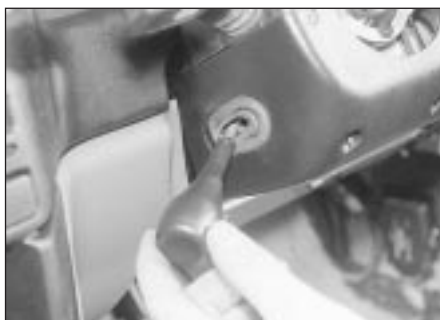
37.7 Removing the column adjuster lever
