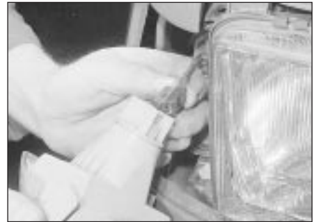
29.3 Disconnecting the front indicator lamp unit wiring plug
