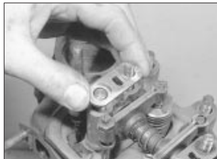
7.15a Recover the pedestal plate (where fitted) . . .
