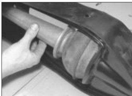
15.3 Remove the rear rubber cone spring strut . . .
