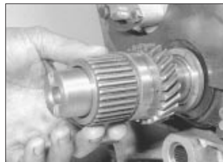
5.30 Slide on the primary gear ...
