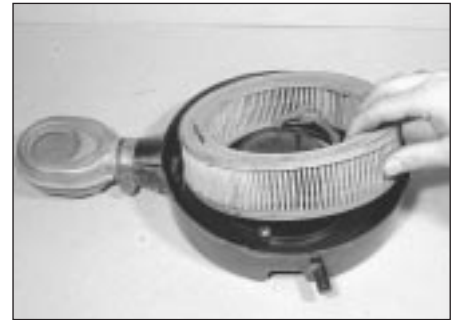
30.6b . . . and lift out the element
