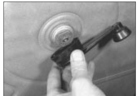
6.2b . . . and the window regulator handle
