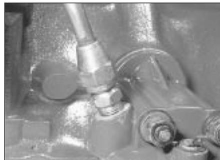
15.2b . . . and pipe nut attachment at the filter housing
