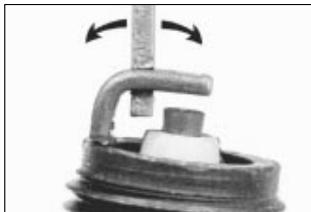
Adjusting spark plug gap
