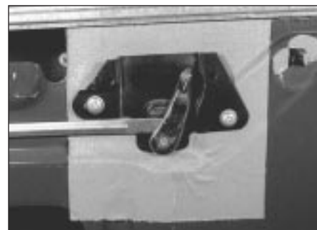
10.3 . . . the interior lock control retaining screws . . .
