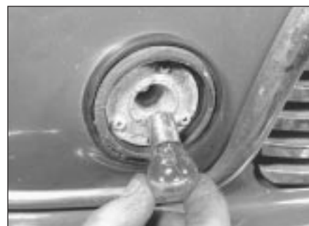
5.28 Push and turn the bulb anti-clockwise to remove
