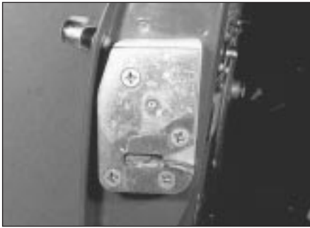
10.4 ... and the door lock retaining screws
