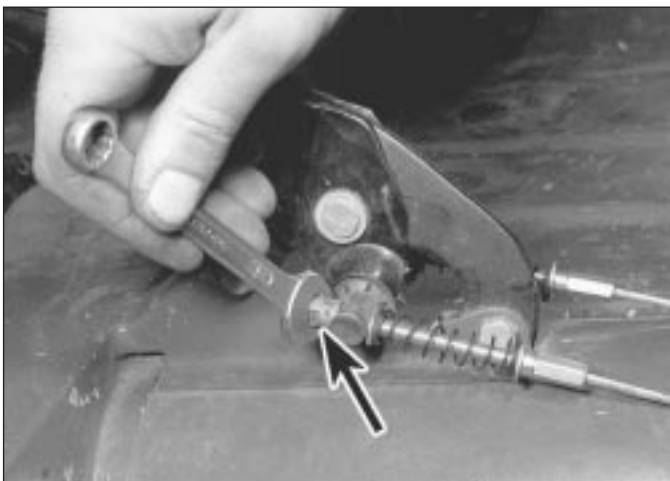
4.5a Handbrake adjustment on models with twin cables
