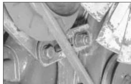
8.6 Dynamo adjusting arm nut located below the water pump
