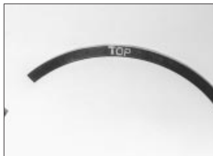
16.3 Piston ring identification markings
