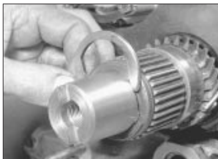
5.31b ... and the C-shaped washer
