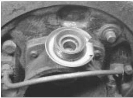
5.11a Fit the lockwasher ...
