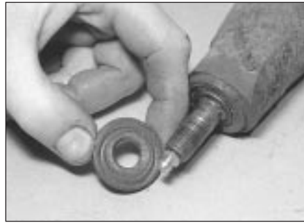
19.12b . . . and thrustwasher . . .
