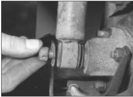
17.3 Remove the shock absorber lower ...
