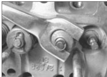
8.4a Compress the valve springs with a spring compressor and lift off the split collets . . .
