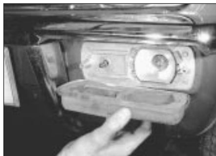
5.24 Undo the two screws and lift off the lens
