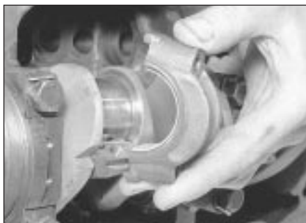
11.3 Removing a connecting rod big-end cap
