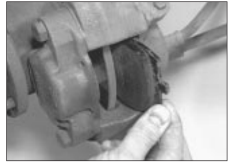
7.3b . . . then withdraw the two brake pads
