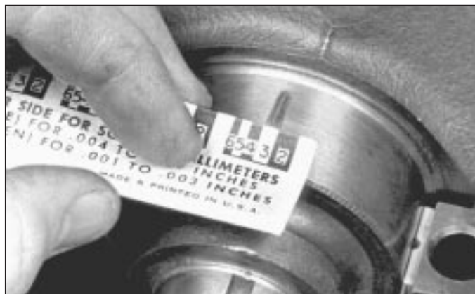
17.11 Measuring the width of the deformed Plastigage using the card gauge supplied
