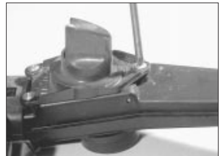
3.12 Removing the air cleaner intake duct adapter
