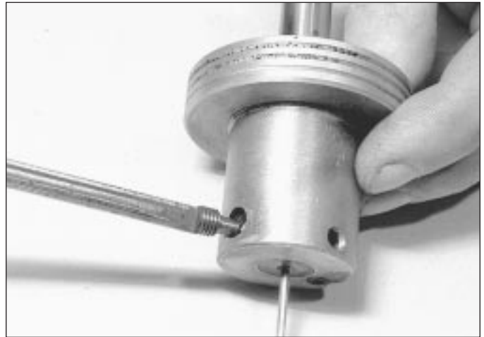
13.35b . . . and secure with the retaining screw
