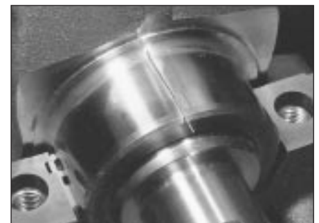
17.7 Plastigage in place on main bearing journal
