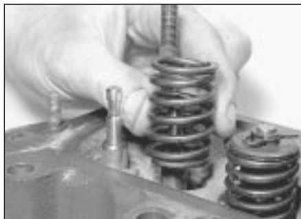
8.4b . . . Then remove the compressor, valve cap and spring
