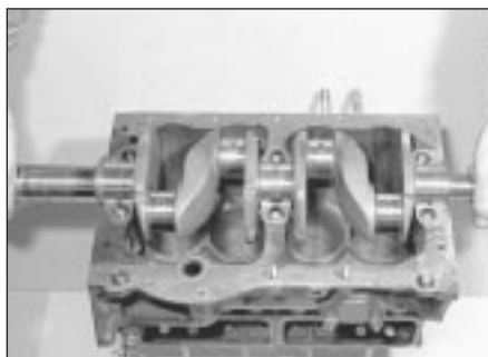
12.10 Carefully lift out the crankshaft
