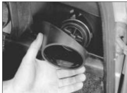
13.1b . . . and lift away the binnacle
