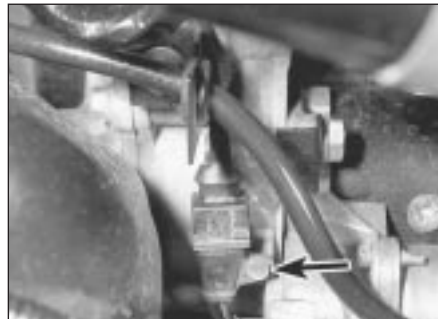
11.3 Crankshaft sensor wiring connector retaining bolt (arrowed) - manual transmission models
