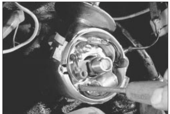
5.7 Adjusting the contact breaker points
