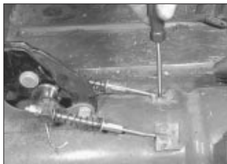
21.5b . . . and unscrew from above
