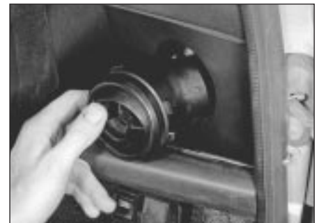
13.2 Turn the air vent anti-clockwise to remove
