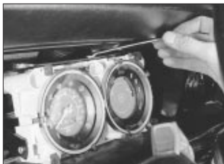
15.27b ... and upper retaining screws
