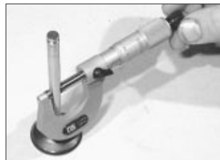
8.17 Measuring the valve stem diameter
