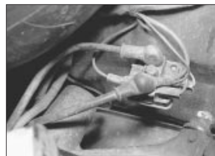
16.2 Electrical connections at the starter solenoid
