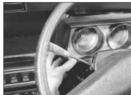
15.25 Remove the instrument cluster nacelle
