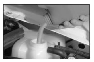
Fill the coolant surge tank with the proper mixture, to slightly above the FULL COLD/FROID line on the side of the coolant surge tank.
