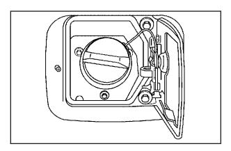
The tethered fuel cap is located behind a hinged fuel door on the passenger's side of the vehicle. To open the fuel door, push inward on the forward edge of the fuel door until the rear edge can be pulled outward.
