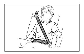
Buckle, position, and release the safety belt as described in *Rear Seat Passengers on page 1-22*. Make sure that the shoulder belt crosses the shoulder.
