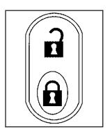
The power door lock switches are located on the front doors.
