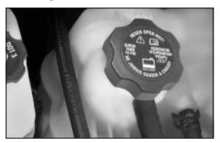
The coolant surge tank and pressure cap are located on the driver's side of the vehicle, toward the rear of the engine compartment. See *Engine Compartment*Overview on page 5-12 for more information on location.
