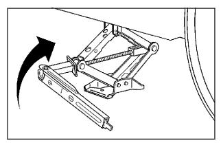
Raise the vehicle by turning the wheel wrench clockwise. Raise the vehicle far enough off the ground for the compact spare tire to fit under the vehicle.
