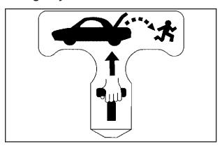
Notice: Do not use the emergency trunk release handle as a tie-down or anchor point when securing items in the trunk as it could damage the handle. The emergency trunk release handle is only intended to aid a person trapped in a latched trunk, enabling them to open the trunk from the inside.
