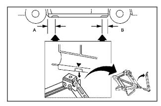
Find the jacking location using the diagram above and corresponding hoisting notches located in the plastic molding. The notches in the plastic molding are marked with a triangle shape to help you find them.
