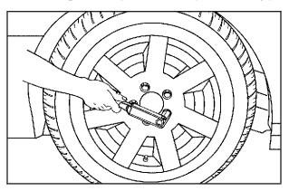
Loosen the wheel nuts, but do not remove them yet, using the wheel wrench. Turn the handle about 180 degrees, then flip the handle back to the starting position. This avoids taking the wrench off the lug nut for each turn.
