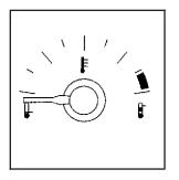
This gage shows the engine coolant temperature. If the gage pointer moves into the shaded area, the engine is too hot.
