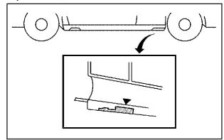
Locate the rear lifting points using the diagram shown above and corresponding hoisting notches located in the plastic molding. The notches in the plastic molding are marked with a triangle shape to help you find them. The rear lifting location is about 7 inches (17.8 cm) from the front edge of the rear wheel well.
