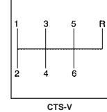
These are the shift patterns for the six-speed manual transmissions.
