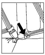
Insert a tool with a small tip into the slot as shown to unlatch the seatbelt buckle. Then move the belt to the side so it is not in your way.
