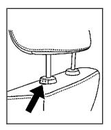
The front seat head restraints can be adjusted up and down. Pull up on the head restraint to raise it. Press the button located at the bottom of the head restraint and push the head restraint down to lower it.
