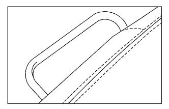
Your vehicle may have manual seats. To adjust the seat, lift the bar under the front of the seat to unlock it. Slide the seat to where you want it and release the bar. Try to move the seat back and forth with your body to be sure the seat is locked in place.
