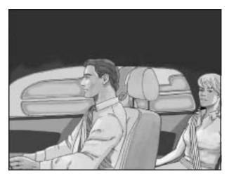
The roof-mounted side impact airbag for the front passenger and the passenger directly behind the front passenger is in the ceiling above the side windows.
