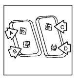
These are the controls for the message center. They are located on the left spoke of the steering wheel.
