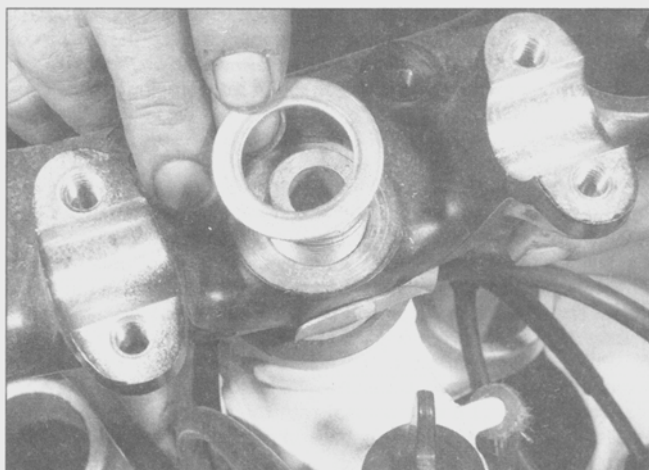
5.6c Lift off the washer ...
