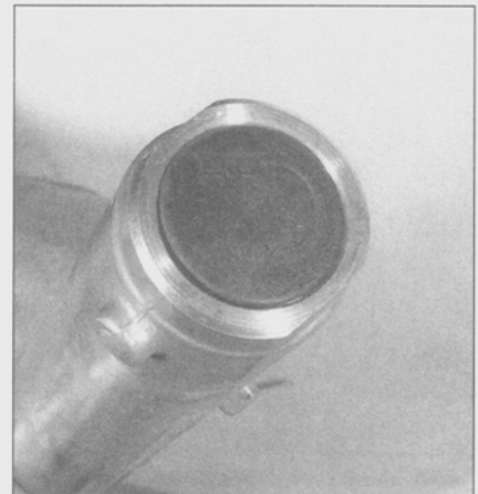
4.26a Remove the bottom cover from the fork leg
