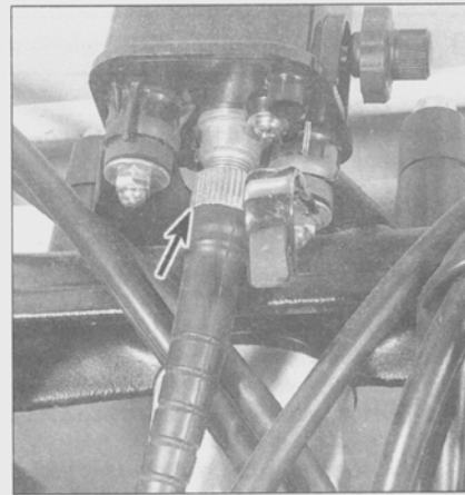
11.4 Unscrew the knurled nut (arrow) and detach the cable from the meter (XR600R trip odometer shown)
