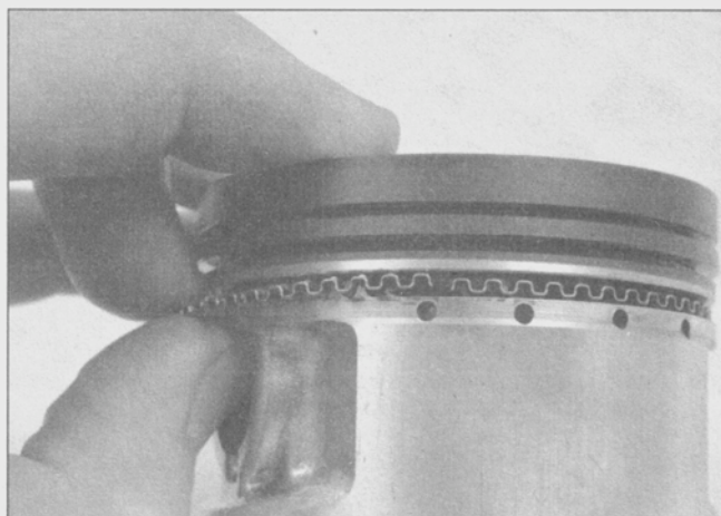
15.7a Installing the oil ring expander - make sure the ends don't overlap
