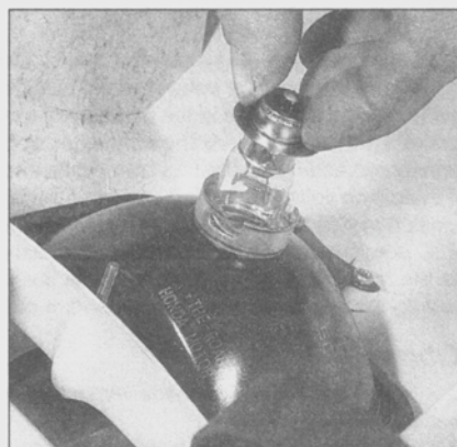
6.8 Rotate the bulb to align its tabs with the slots and pull it out
