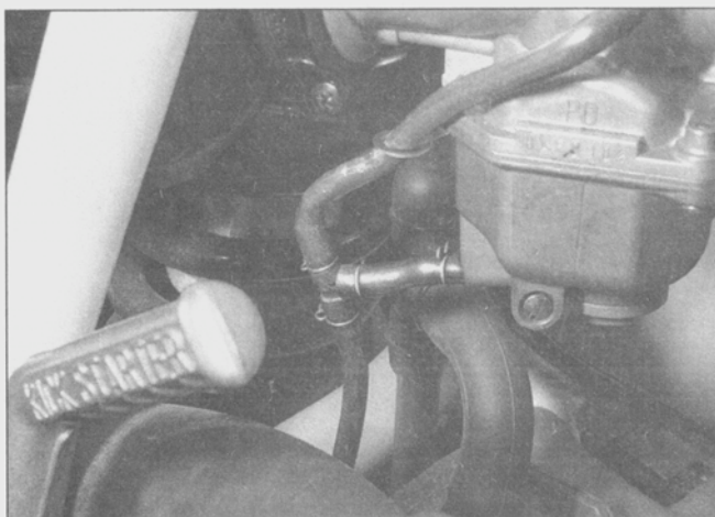
13.1b There's a drain hose and a vent hose connected to the bottom of the float chamber
