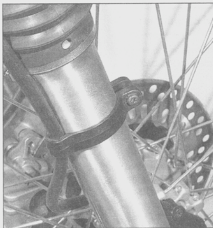
11.3 Detach the cable retainer from the fork leg
