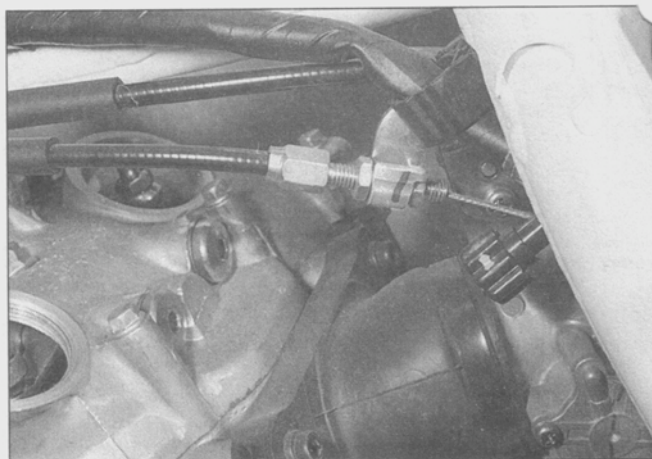
8.5 Major throttle cable adjustments are made at the adjuster near the carburetor
