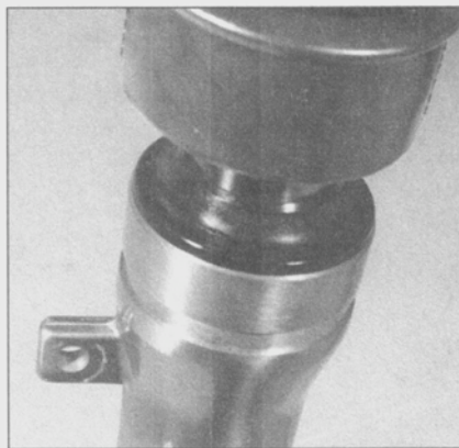
4.14 Push the dust seal down until it seats in the outer fork tube
