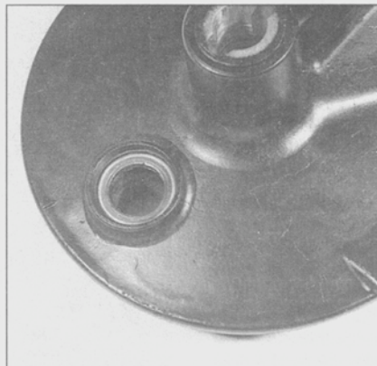
5.12a Replace the brake cam seal if it's worn or damaged
