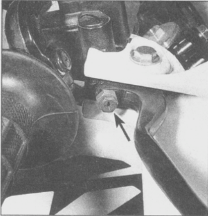
5.3 Front brake lever freeplay on later models is adjusted by loosening the locknut and turning the screw (arrow)
