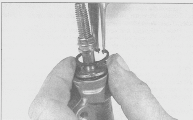
7.10a Remove the snap-ring from the master cylinder bore and withdraw the piston assembly and spring
