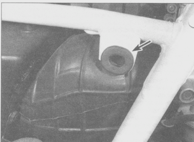
5.1b . . . and carefully pull the lugs free of the grommets (arrows)
