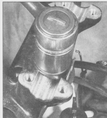
5.6a Loosen the steering stem nut with a socket . . .
