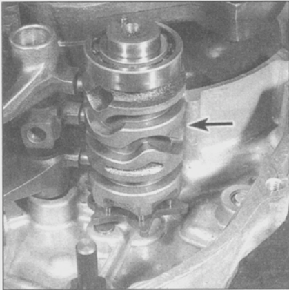
25.7 Lift out the shift drum (arrow)
