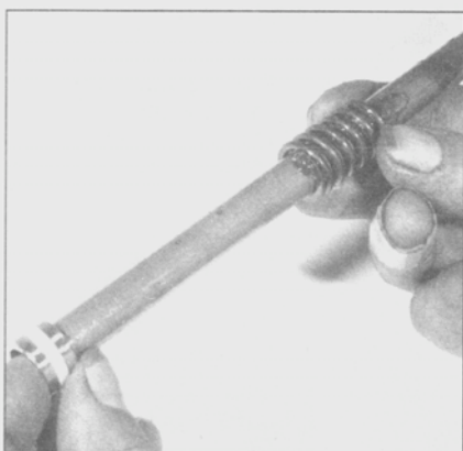
4.6 Replace the Teflon ring on the damper rod if it's worn or damaged
