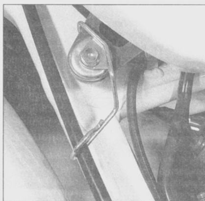
2.6 Remove the mounting bolts at the front (there's one on each side)
