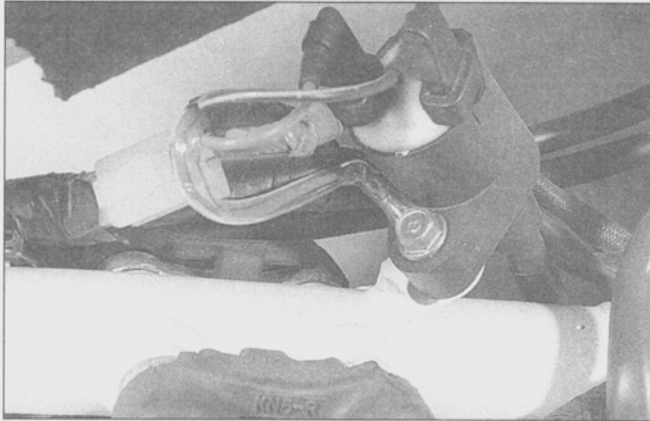
19.9 The ignition coil is mounted beneath the fuel tank
