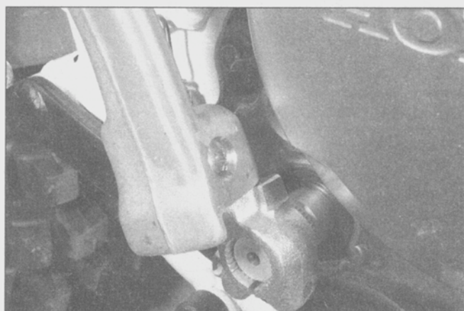
21.2 The pedal is secured to the lever by a screw
