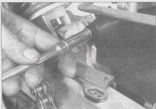
8.4a Unbolt the upper chain guard from the swingarm . . .
