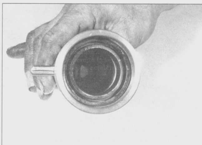
4.2k Pry the oil seal out of its bore; be careful not to scratch the seal's seating area in the fork tube
