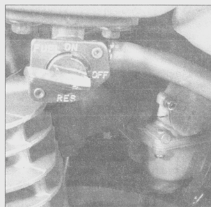
2.7 Disconnect the fuel line from the tap
