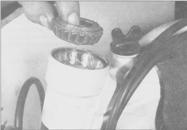
5.9 Lift the upper bearing out of the steering head
