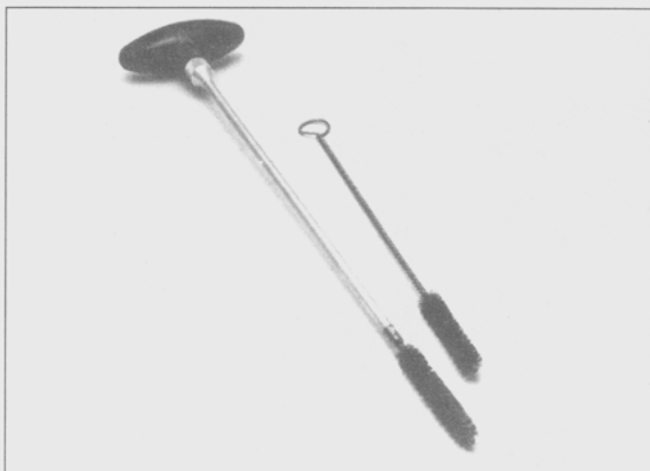
6.2 A selection of brushes is required for cleaning holes and passages in the engine components
