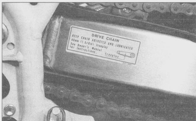
2.1a Decals on the motorcycle include maintenance information such as drive chain adjustment . . .
