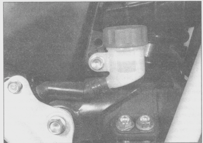
7.6b The fluid reservoir is secured by a single bolt
