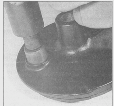
5.12b Pry out the old seal, then press a new one in with a socket the same diameter as the seal
