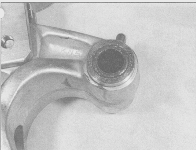
6.11c . . . and inspect the needle bearings
