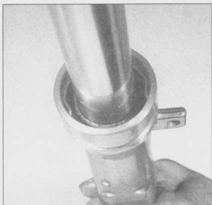
4.13 Make sure the retaining ring seats in its groove
