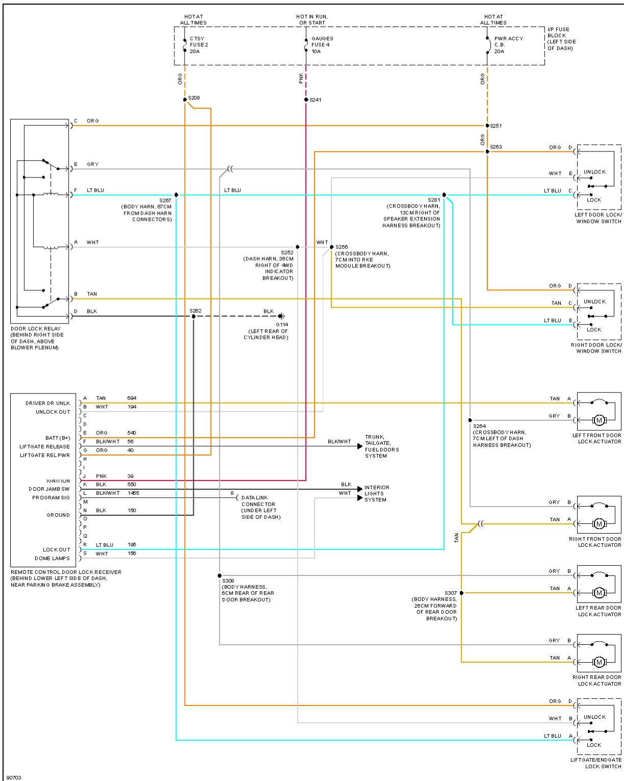
**Fig. 28: Keyless Entry Circuit**
