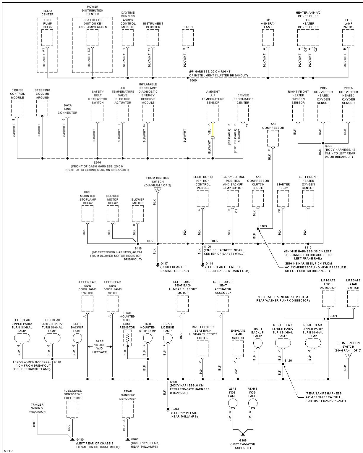
**Fig. 13: Ground Distribution Circuit (2 of 2)**
