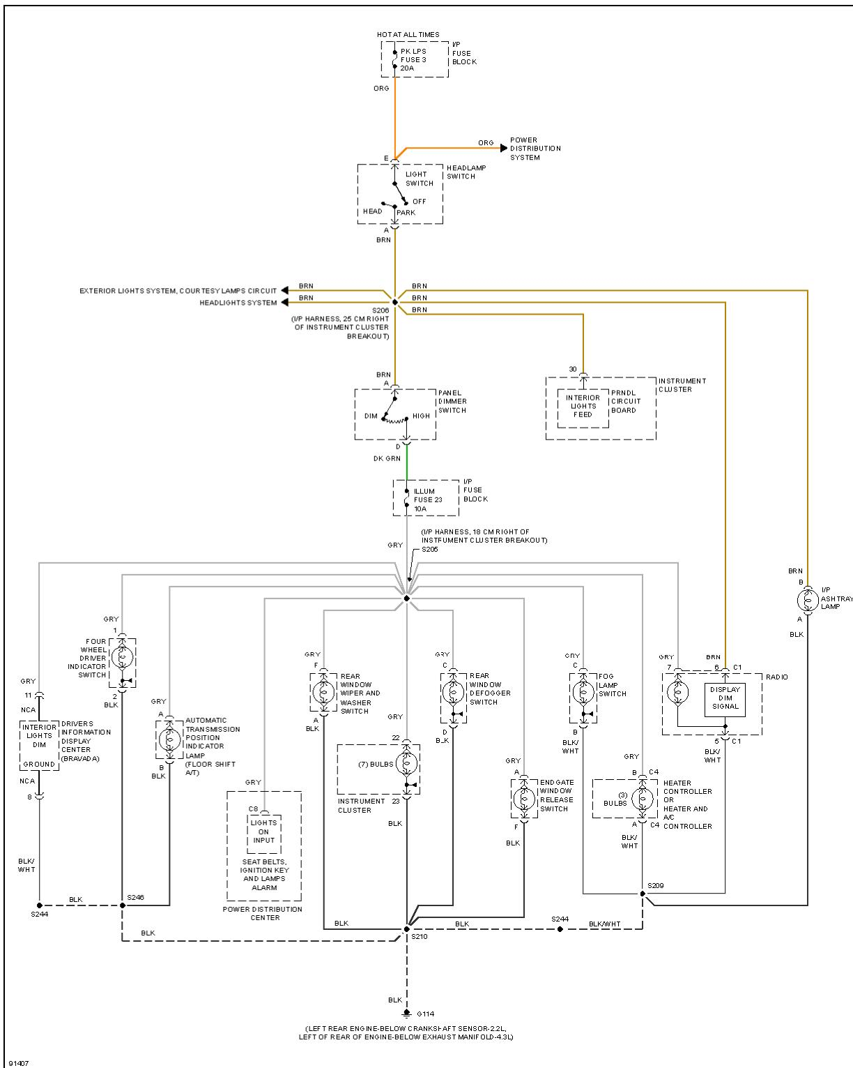
**Fig. 22: Instrument Illumination Circuit**
