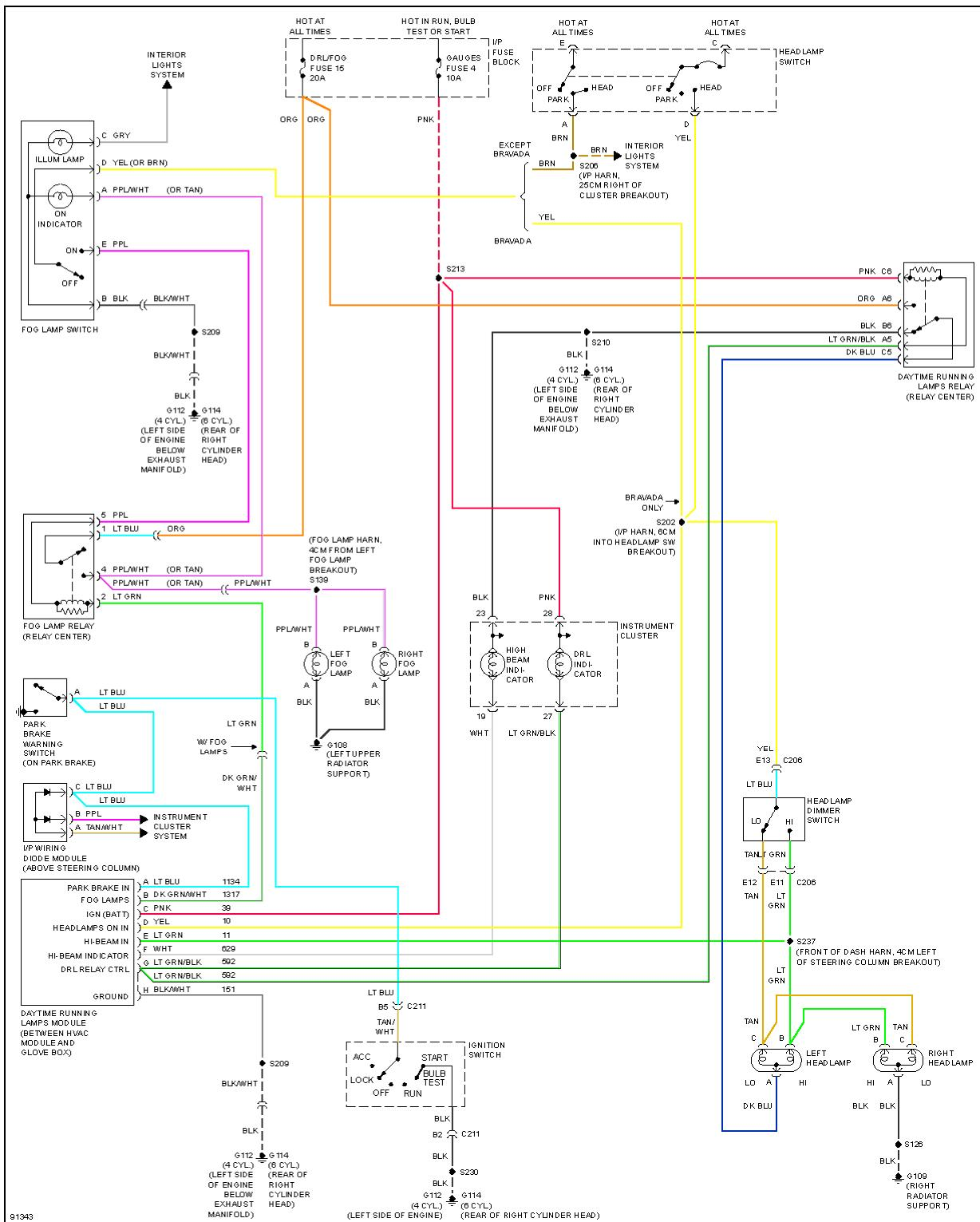
**Fig. 15: Headlight Circuit, W/ Sealed Beam Headlamps**
