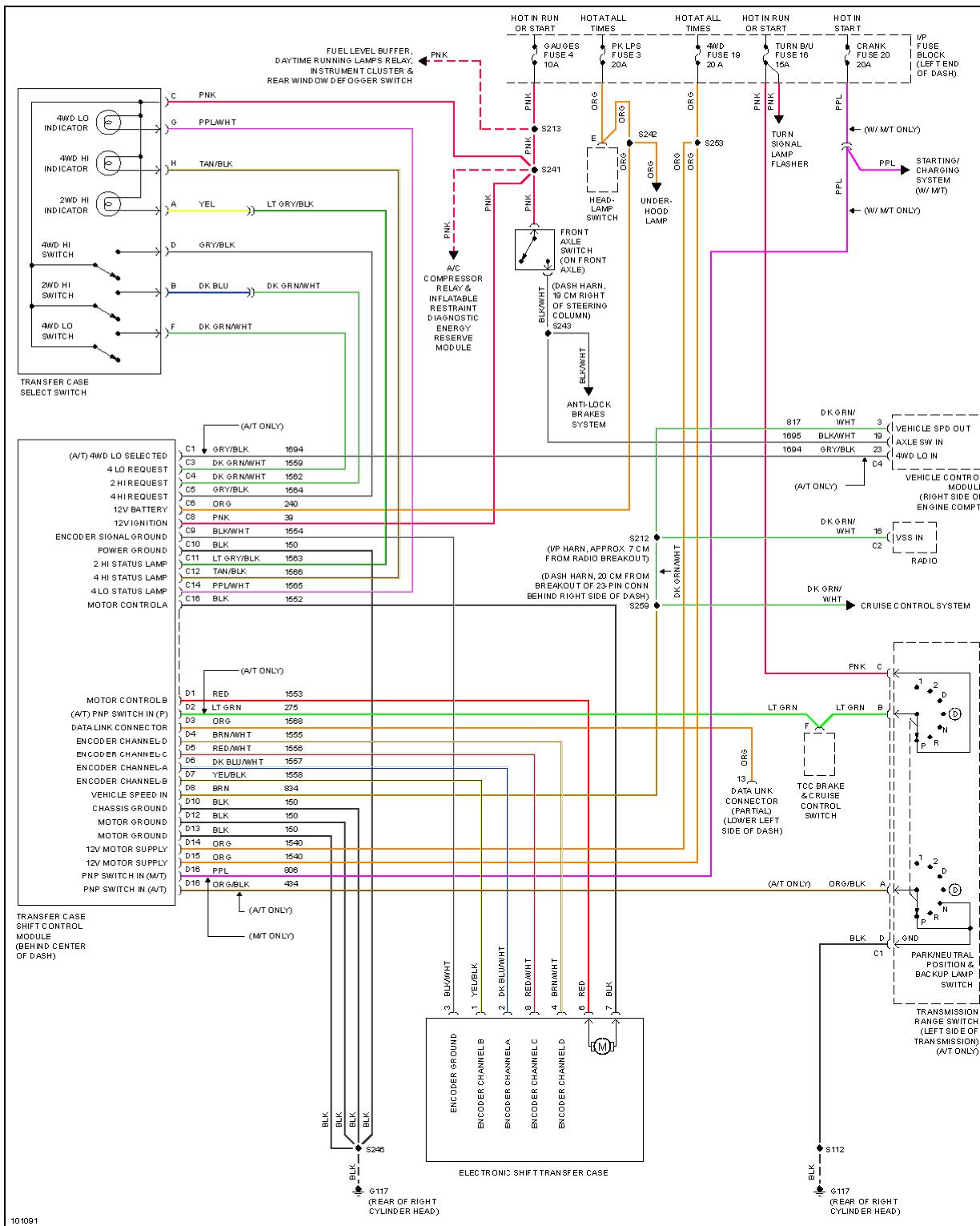
**Fig. 41: Electronic Transfer Case Circuit**
