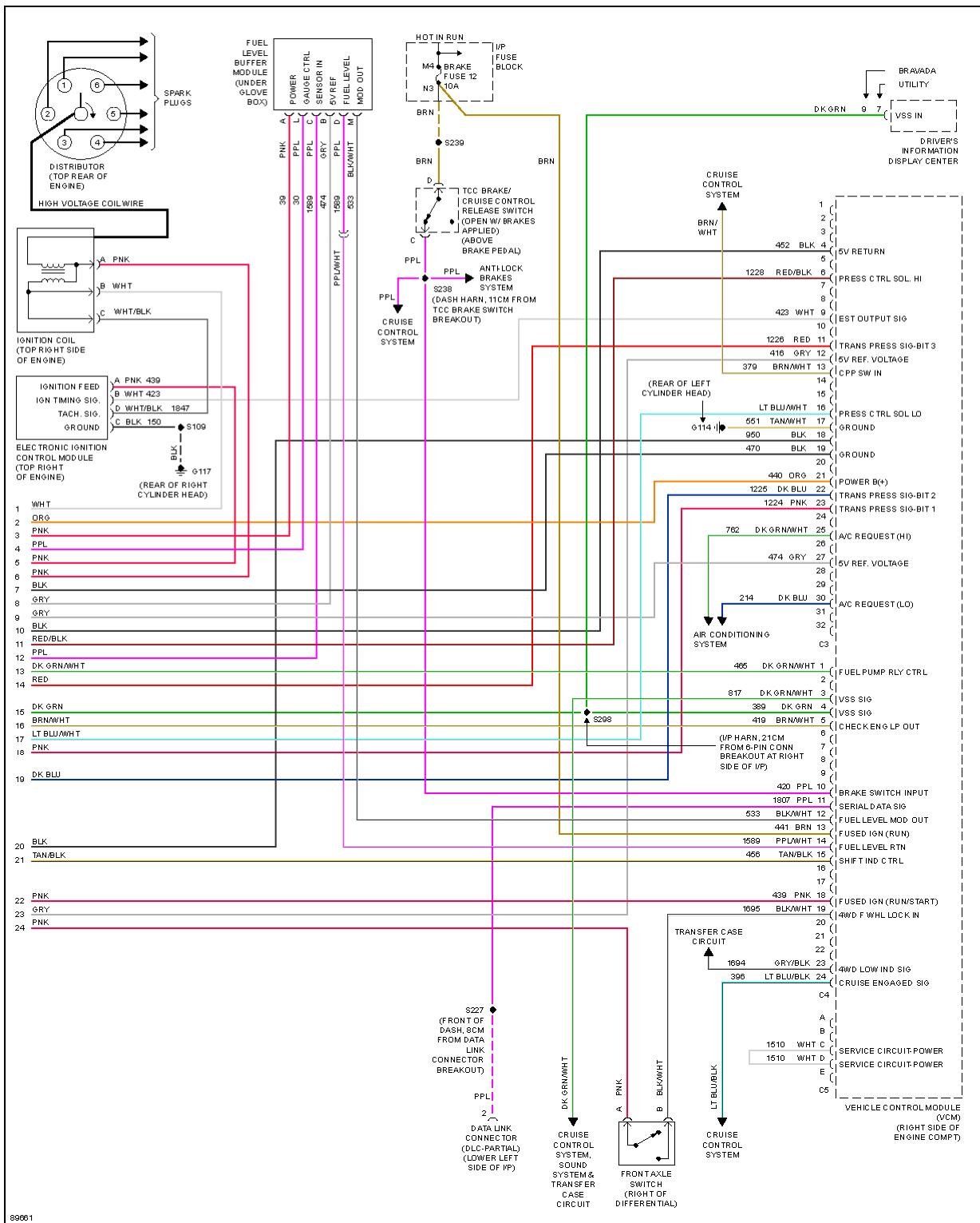
**Fig. 9: 4.3L (VIN W), Engine Performance Circuits (4 of 4)**
