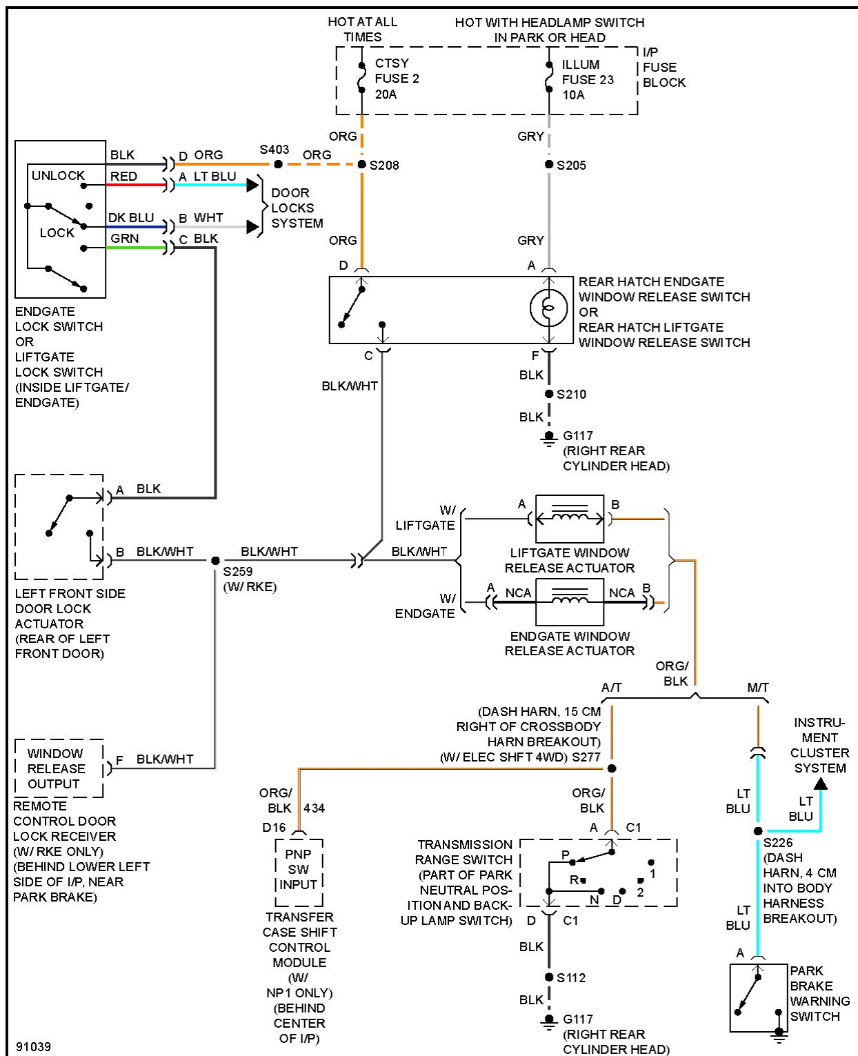
**Fig. 42: Rear Glass Release Circuit**
