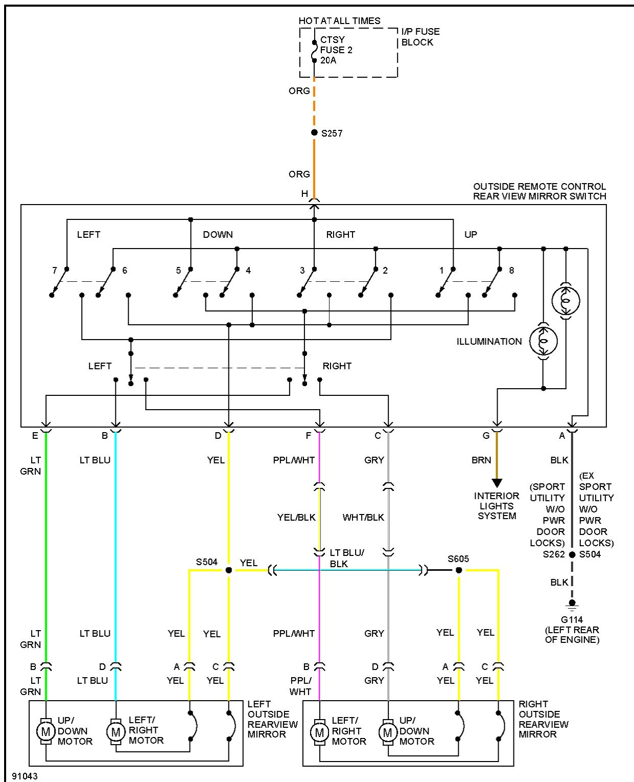
**Fig. 29: Power Mirror Circuit**
