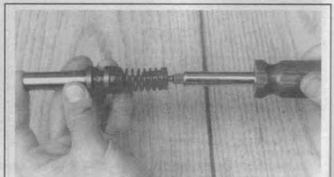
Fig. 19 Remove the screw to the secondary spring in order to disassemble piston B and piston A and the rest of the assembly
