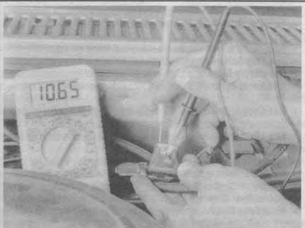
Fig. 9 This voltage drop test revealed high resistance (low voltage) in the circuit
