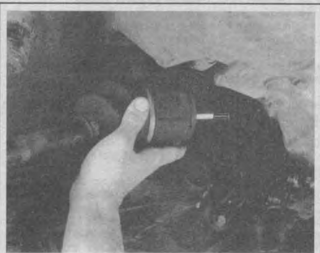
Fig. 54 Removing the inner CV-joint from the differential case
