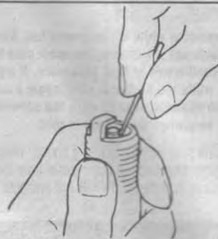
Fig. 10 Clean between the outer shell and insulator with a stiff wire
