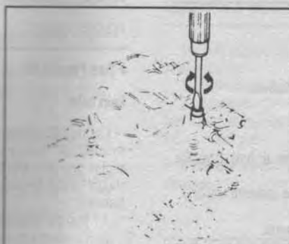
Fig. 15 If the fuel level is not centered in the level window, turn the adjusting screw
