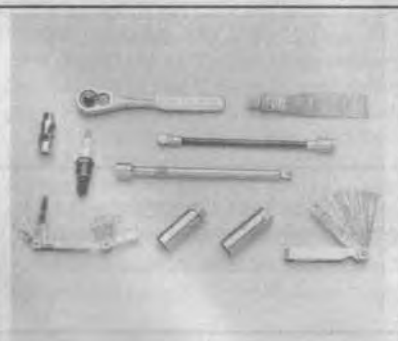
Fig. 7 A variety of tools and gauges are needed for spark plug service
