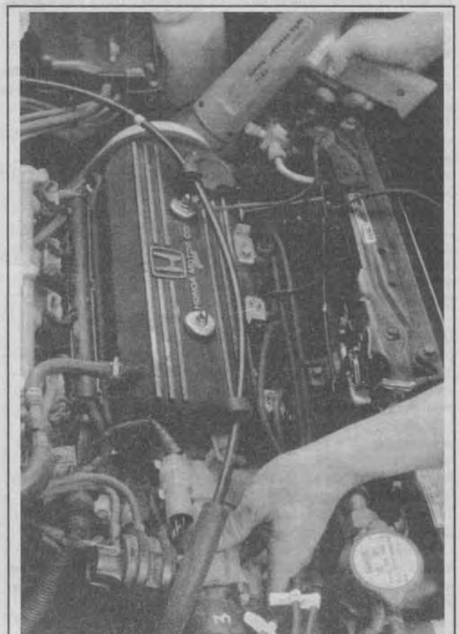
Fig. 62 To check the timing, rotate the distributor until it is within specification
