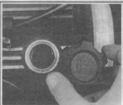
Fig. 87 The oil filler cap screws in atop the valve cover
