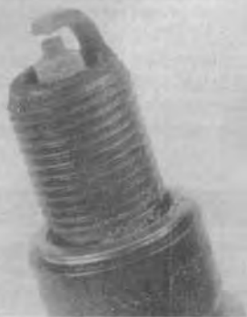
Fig. 6 This plug can be cleaned and re-used
