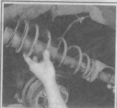
Fig. 44 Once completely detached remove the shock absorber from the car
