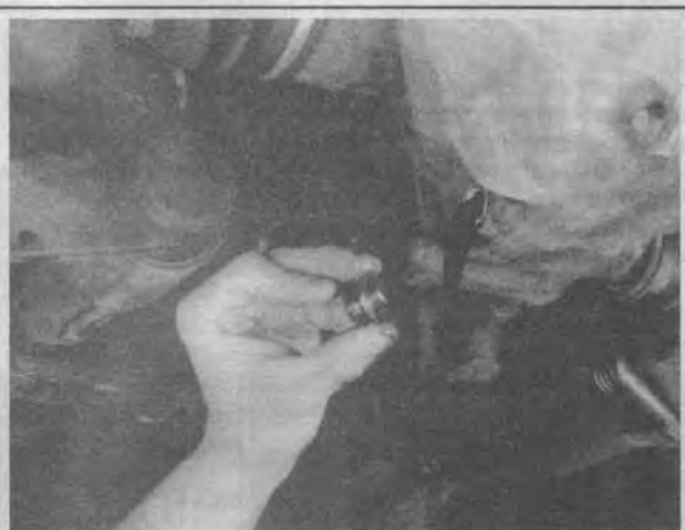
Fig. 90 Use inward pressure while unscrewing the drain bolt, then quickly pull away to avoid the hot oil
