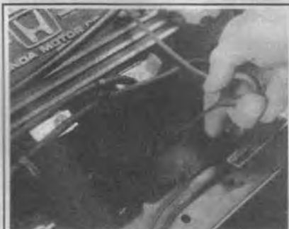
Fig. 80 The dipstick to check the motor oil level is usually brightly colored and prominent for easy identification
