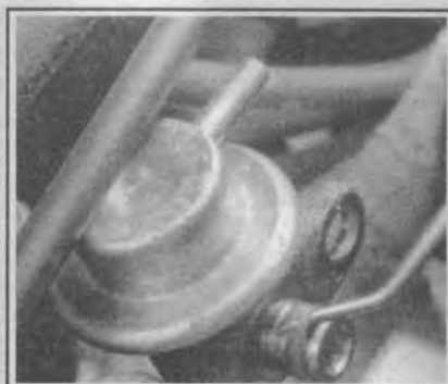
Fig. 68 Replace this O-ring before re-installation
