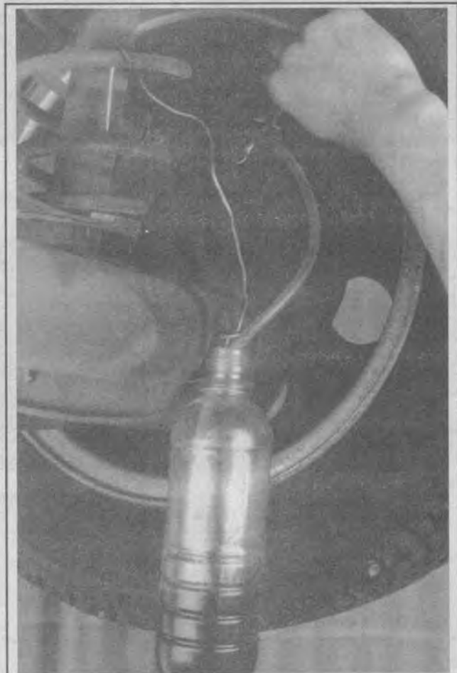
Fig. 23 Here is the quintessential homemade brake bleeder setup: a used plastic bottle, a clean hose submerged in the fluid and a stiff wire to securely fasten the arrangement to the underside of the car near the brakes
