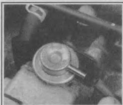
Fig. 66 Grasp and carefully pull the vacuum line from the fuel pressure regulator
