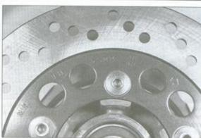
4.4 The minimum thickness is stamped into the disc
