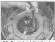
19.9a Thread a 6 mm bolt into the collar and pull it out . . .
