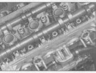
9.27a Make sure the bearing cap dowels are in place . . .
