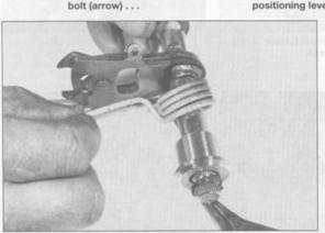
21.15a Remove the snap-ring, bushing and return spring from one end of the shift shaft, and the collar and shift arm from the other end
