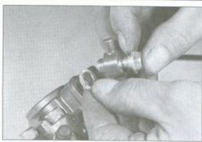
2.2b Separate the hose from the caliper; there's a sealing washer on each side of the fitting
