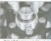
15.4a Lift the spacer out of the wheel
