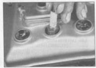
3.2e If the spark plug didn't stay in the wrench rubber insert, lift it out once it's loose . . .
