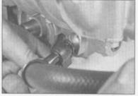
16.5b ... and pull the hose out of the engine; its O-ring should be replaced
