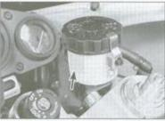
The fluid level is visible through the master cylinder reservoir. Make sure that the fluid level is above the Lower mark on the reservoir.
