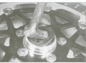
15.4b A screwdriver can be used to pry out the seal if you don't have a removal tool like this one
