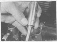
3.1 A 16 mm plug socket is required for spark plug removal
