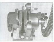
2.24 Leave enough space between the brake pads for the disc
