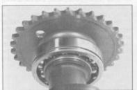
9.22 Check the ball bearing at the end of each camshaft for looseness, roughness or noise
