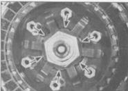
19.21 Use a new nut to secure the clutch hub; torque limiter spring tangs (arrows) must engage as shown
