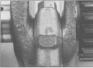
26.2 Using a hammer and punch, make matching number marks on the connecting rod and its cap
