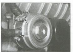
10.9 Loosen the clamps (arrows) and disconnect the coolant hoses
