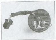
16.3c Remove the terminal screws and disconnect the wires
