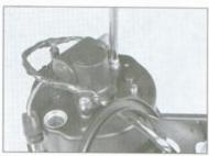
16.12a Remove the screws and lift off the gear housing . . .
