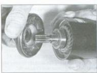
27.2b . . . and lift the cover off the pinion gear end of the starter
