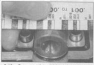
9.13a Compare the width of the crushed Plastigauge to the scale printed on the Plastigauge container
