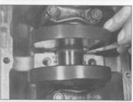
25.1b Measure crankshaft end play with a feeler gauge between the no. 2 bearing web and the crankshaft
