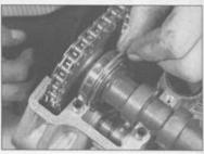
9.27b ... and install the bearing retainer rings
