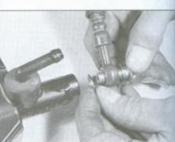
6.3 Disconnect the banjo fitting from the master cylinder; there's a sealing washer on each side of the fitting
