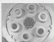
19.18 Check the pressure plate bearing and push piece for wear or damage
