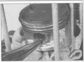
14.3b Using needle-nose pliers remove the piston pin circlips
