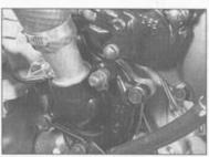
29.24a To bleed the cooling system, remove the rubber cap from the bleed valve (L model shown) . . .
