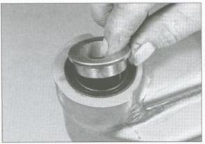
11.3 Remove the collar(s) from the grease seal(s)
