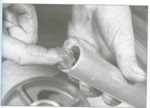
15.31a Apply a coat of grease to the inside of the spacer . . .
