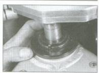
3.24 Install the lockwasher, making sure it engages the notches in the nut
