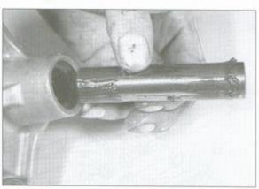
8.10b ... and remove the sleeve from each bearing
