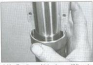
6.36e Tap the seal into place until it seats in the fork tube (tool disassembled for clarity)
