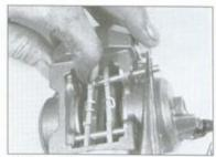
3.10b ... and pull out the retaining pin
