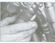
13.5b ... and slide the holders off the studs
