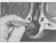
13.3 Lift out the cam chain front guide
