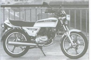
One of the two-stroke engined KH and KE range - the KH125EX
