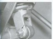
7.9b Remove the nut (arrow) and bolt from the lower end of the shock absorber
