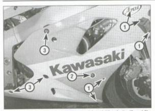
2.6 The fairing is secured by screws (1) and Allen bolts (2 and 3); install the center Allen bolt (2) first
