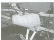
2 ... and under the right rear side cover on J, K, L and M models. The reservoir tank marks should be visible from below and to the rear of the cover.
