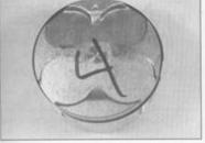
14.3a Mark the top of each piston with its cylinder number
