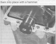
25.21 The ribs on the crankcase end seal must seat in the case groove
