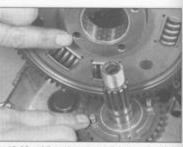
19.23a Align the sprocket pins with the holes in the back of the clutch housing.
