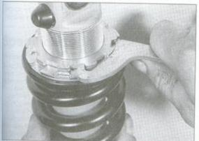
15.5 Loosen the locknut with a special wrench then loosen the adjusting nut until the spring extends completely
