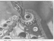
27.10b ... and the alternator driven sprocket ...
