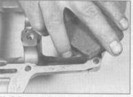
22.15 Remove all traces of sealant from the mating surfaces with a sharpening stone
