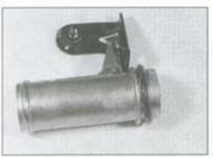
8.23 The coolant tube O-ring should be replaced whenever the tube is removed from the pump cover
