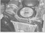
10.8 Stuff a clean rag into the chain cavity (arrow) so nothing is dropped into it
