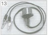
A buzzer is useful for voltage checks
