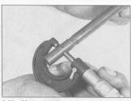
9.39a Measuring the rocker shaft diameter
