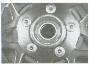
15.9 With the bearing in position, install the snap-ring and make sure it's securely seated in its groove
