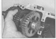
29.2b ... and driveshaft out of the casing
