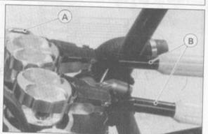
13.11 You can guide the cylinder block over the pistons with a screwdriver, but it's a good idea to use ring compressors
