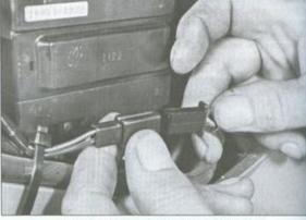
14.6 Disconnect the fuel pump connector (L model shown)
