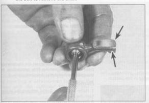
9,39b Check the cam contact and valve contact surfaces (arrows) for wear and damage; measure the inside diameter of the rocker arm with a small hole gauge . . .
