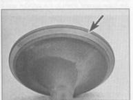
12,24a After lapping, the valve face should exhibit a uniform, unbroken contact pattern (arrow) . . .
