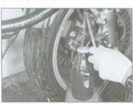
10.5c Connect a plastic tube to the bleed valve and place the other end in a container
