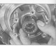
19.25a Install the clutch hub and splined spacer
