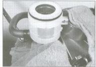
5 Reinstall the rubber diaphragm and retainer, Install the cap retainer and the cap and tighten its screw securely, but do not overtighten it. Wipe any spilled fluid off the reservoir body.
