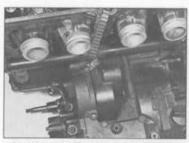
9.7 Wire the cam chain up so it doesn't slip down off the crankshaft sprocket
