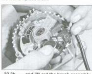
32.3b . . . and lift out the brush assembly (749 cc shown)
