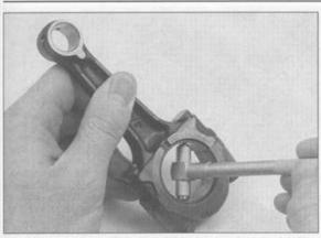
26.20a Measure the diameter of the connecting rod with a telescoping gauge then measure the gauge
