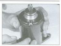
27.19c Line up the screw hole in the pinion gear end cover with the marks on the starter housing
