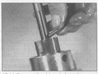
17.11 Remove the drive pin from the pump shaft
