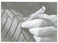
Measure the tread depth at the center of the tire using a tread depth gauge.
