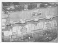
13.5 Lift the cylinder block off the crankcase
