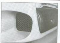
5.5b . . . and pull the duct with its screen out of the fairing
