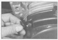
19.3b ... taking note of any hose brackets or wiring harness retainers ...
