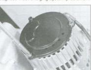
32.2 Remove the end cover from the alternator (749 cc shown)
