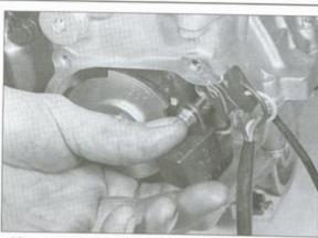
4.9c . . . pull the pick-up coil out and detach the grommet from the crankcase
