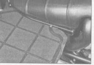
19.6b ... and slide the element out of the air filter housing
