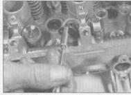
12.7c ... the valve spring retainer ...
