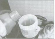
4 Add new, clean brake fluid of the recommended type until the level is above the inspection window. Don't mix different brands of brake fluid in the reservoir, as they may not be compatible.
