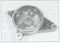
27.13a Inspect the bushing in the brush end housing . . .
