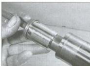
6.31 Lift the cartridge out of the fork
