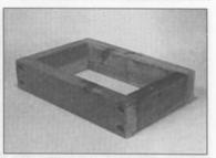
6.3 An engine stand made from short lengths of 2 x 4 lumber and lag bolts or nails
