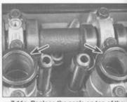
7.11a Replace the seals on top of the camshaft brackets (arrows) if deteriorated or damaged . . .
