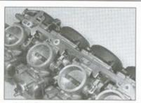
8.14b Be sure to reinstall the plastic washers on both sides of the shaft
