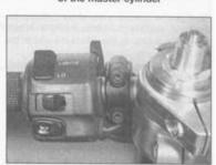
20.19 The UP mark on the master cylinder clamp must be upright
