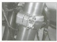
4.7 Loosen the lower triple clamp bolts (arrows)
