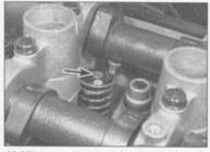
23.30b ... and remove the valve adjusting shim (arrow) with a magnet
