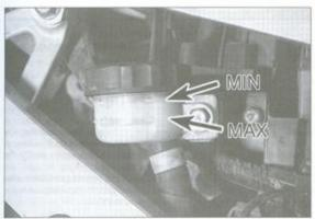
Rear brake fluid reservoir location – H models. Unscrew the cap and add fluid as described for the front brake.
