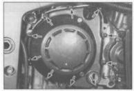
19.3a Remove the clutch cover bolts (arrows) . . .
