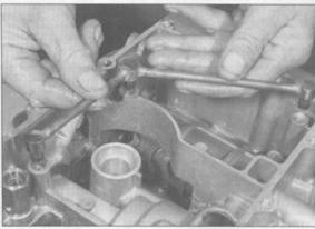
16.13 Work the three O-rings clear of the crankcase passages and lift the oil pipe out
