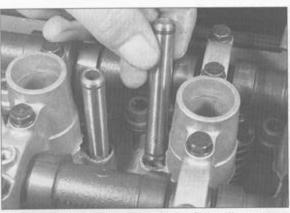
7.11b ... and replace the air suction tube O-rings if necessary (L3 models use two O-rings at the bottom end of each tube)
