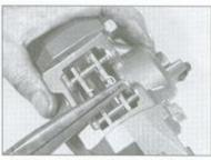
3.10a Pull out one of the retaining pin
