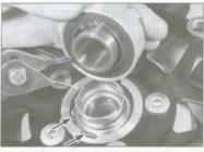
15.3a Lift out the speedometer drive unit and remove the snap-ring (arrows) . . .
