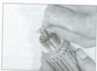
27.4 Note the location and number of any shims on the armature
