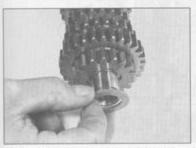
31.3a Remove the thrust washer . . .
