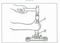
3.21 Drive the lower bearing onto the steering stem with the special Kawasaki tools
