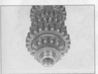
30.3 Remove the thrust washer and second gear
