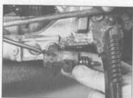
5.20b ... and remove the sidestand switch from the stand bracket
