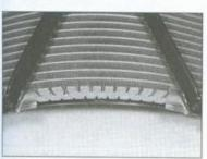
4.7a Remove two bolts at the bottom of the fan bracket . . .
