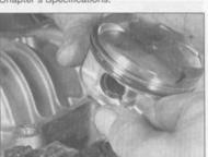
14.3b Wear eye protection and pry the circlip out of its groove with a pointed tool
