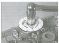
Angle-tightening cylinder head bolts
