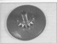
28.15 Check the idler gear for worn or damaged teeth and for looseness on its shaft
