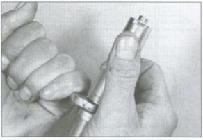
6.5b . . . then unscrew the preload adjuster from the piston rod
