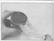
14.6 Remove the piston rings with a ring removal and installation tool
