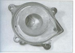
8.20 The cover O-ring should be replaced if there's any doubt about its condition
