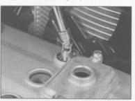
7.8a Remove the valve cover bolts . . .
