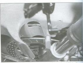
8.5 Rotate the fender/mudguard forward and lift it off
