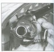
6.15 Reinstall the ground (earth) wire connector when installing the thermostat cover (J, K, L and M models)
