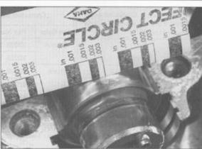
25.10 Measuring the width of the crushed Plastigauge
