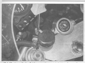
20.4 Master cylinder fluid reservoir cap retainer and mounting bolt
