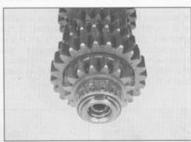
30.2b . . . then remove the snap-ring and bearing
