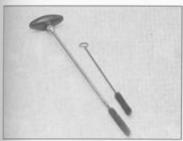
62a A selection of brushes is required for deaning holes and passages in the engine components
