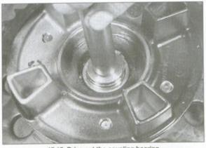
15.18 Drive out the coupling bearing
