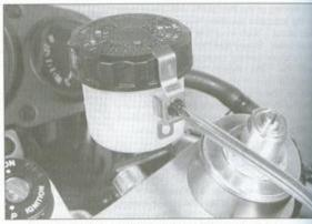
6.2a Remove the screw and take off the cap retainer . . .
