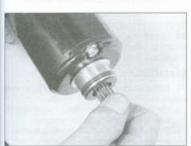
27.20b . . . and install them in the starter; make sure the O-ring is in position on the end of the starter
