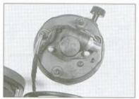
16.11b . . . and pull out the bulb sockets
