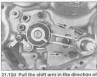
21,12d Pull the shift arm in the direction of the arrows to clear the shift drum cam
