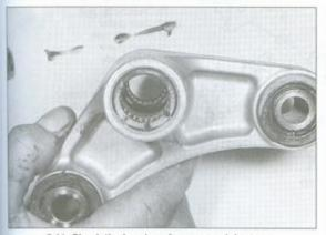
8.11 Check the bearings for wear and damage
