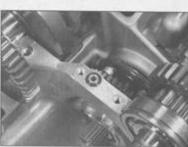
22.16 Install the oil nozzle and a new O-ring
