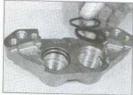
2.11 Remove the dust seals and piston seals with a wood or plastic tool
