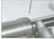
6.25 Insert a screwdriver between the dust seal and fork tube and pry the seal out
