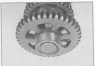
30.14a Slide off the bearing outer race . . .
