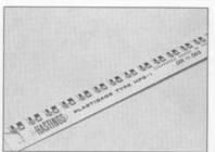
6.2b Type HPG-1 Plastigauge needed to check main bearing, connecting rod bearing and camshaft oil clearances
