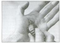
3,20 Work the grease completely into the rollers
