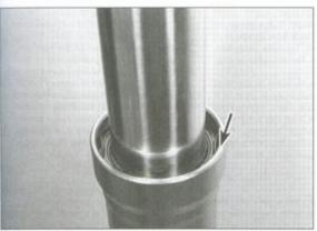
6.26 Pry the oil seal retaining ring (arrow) out of its groove
