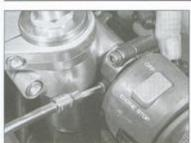
6.4 Remove the mounting bolts and separate the clamp from the cylinder body
