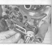
21.13b ... and take the external shift linkage out of the crankcase Caution: Don't pull the shift rod out of the
