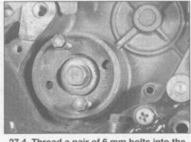
27.4 Thread a pair of 6 mm bolts into the holes in the pulley then tighten them against the case to push the pulley off
