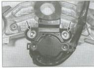
19.6 Drill out the self-shearing screws (arrows) and remove them with a screw extractor
