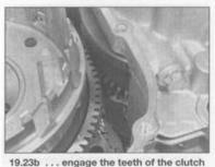
housing gear with the crankshaft primary gear
