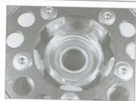
15.30 Make sure the bearing is fully seated and the snap-ring groove is exposed
