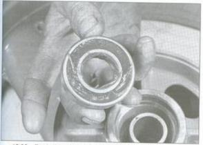
15.32a Pack the open side of the bearing with grease . . .
