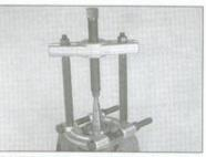
5.3 This bearing puller clamps behind the bearing and pressure is applied to the shaft end to draw the bearing off
