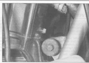
29.13 A coolant drain plug is located on each front corner of the cylinder block
