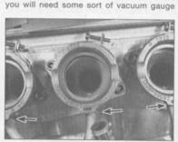
5.6a Disconnect the hoses (if equipped) from the vacuum fittings - L models (shown) are on the bottom of the intake manifold boots; H and J models are on the top . . .
