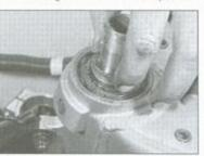
3.22a Install the upper bearing and the O-ring
