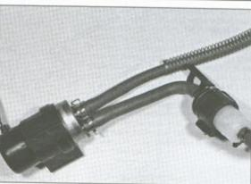
14.7b Fuel pump and filter details (L models)
