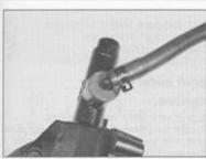
20.6 Remove the rubber cap, snap-ring, fluid feed fitting and O-ring
