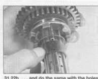
31.22b ... and do the same with the holes for the third-fourth gear bushing
