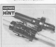
When disassembling the transmission shafts, place the parts on a long rod or thread a wire through them to keep them in order and facing the proper direction.
