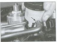
6.2b . . . remove the reservoir mounting screw; disconnect the hose at the reservoir end (arrow) . . .
