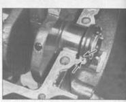
25.23 Make sure the ribs on each seal seat in the grooves in the case (arrows)
