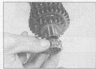
31.2c . . . and the needle roller bearing
