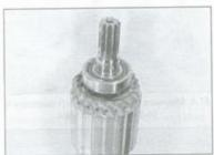
27.12 Check the armature bearing for roughness, looseness or loss of lubricant
