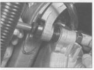
5.30 Install both front mounting bolts and their locknuts and tighten them slightly
