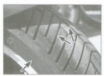
3 Tire tread wear indicators bars and location marking on the sidewall (arrows).
