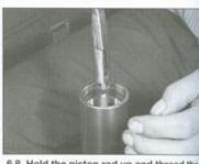
6.8 Hold the piston rod up and thread the nut all the way onto it
