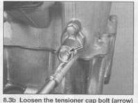
8.3b Loosen the tensioner cap bolt (arrow) and the mounting bolts . . .
