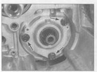
17.9a Remove the oil pump mounting bolts (arrows)
