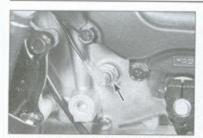
22.1 The neutral switch is mounted on the left side of the engine (749 cc engine shown)
