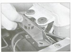
2.10e ... on L and M models, remove the tank mounting bracket
