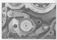
21.13a Remove the nuts (arrows) that secure the gear and neutral positioning levers . . .
