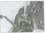
16.9a Remove the tachometer mounting nuts . . .
