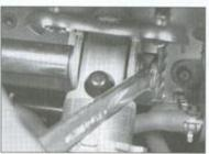
7.9c Hold the upper bolt with a wrench and remove the nut . . .
