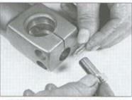
6.30b . . . then unscrew the bolt and remove its sealing washer
