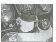
The clutch fluid reservoir is located above the left front fork. The fluid level is visible through the reservoir. Make sure that the fluid level is above the Lower mark on the reservoir. If the level is low, the fluid must be replenished.
