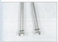
27.20a Make sure the O-rings are in position on the long screws . . .
