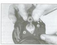
16.12d ... and lift the gear off the shaft
