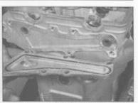
16.6b . . . then take the cover off; use a new O-ring on installation
