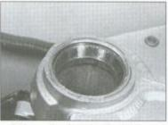
3.14c . . . then inserting the drift from below to drive out the upper race
