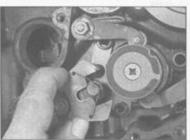
21.12a Compress the shift mechanism arm until the tips are clear . . .
