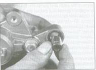
2.7b ... and check the bushing for wear or damage
