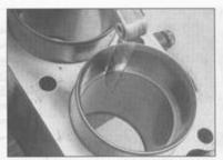
15.3 Check the piston ring end gap with a feeler gauge
