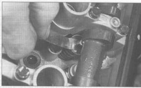
23.24 Insert a feeler gauge between the rocker arm and cam lobe to measure the clearance
