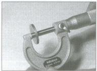
Tappet shims are measured with a micrometer
