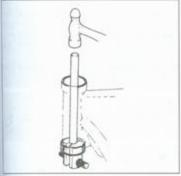
3.14a Driving out the lower bearing race with the special Kawasaki tool...
