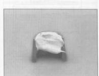
12.27 A dab of grease will hold the keepers/collets in place while the spring compressor is released
