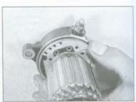
27.18b ... until the end of the armature shaft seats in the cover bushing
