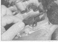
7.10 Lift the valve cover gasket off the cylinder head
