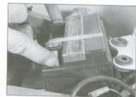
3.5b , . . and lift the battery out
