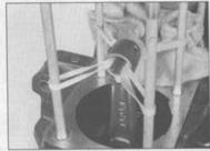
14.4 Use rubber bands to keep the connecting rods from flopping around after the pistons are removed
