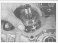
27.13 Remove the thrust collar from behind the transmission mainshaft
