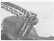
25.22 Be sure to drape the chain over the crankshaft sprocket
