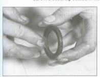
15.11 Apply a coat of grease to the lip of the seal
