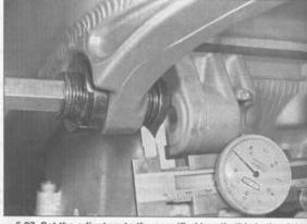
5.27 Set the adjusters to the specified length; this is the right front adjuster...
