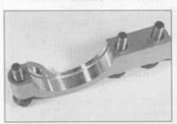
9.24 Check the cam bearing surfaces in the cap and head to make sure they're clean
