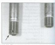
10.22 The rear axle has a cotter pin hole in the end (arrow); the swingarm pivot shaft doesn't
