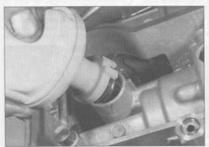
16.12 Work the strainer loose from the crankcase; on installation, align its notch with the cast tab on the crankcase
