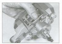
3.12a Pull the clip out of the other retaining pin . . .
