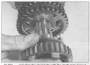
31.22d ... and align the steel balls with the shaft slots (arrow) when installing the gear
