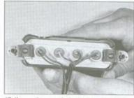
17.4b . . . then work the bulb socket(s) free of the assembly to expose the bulbs
