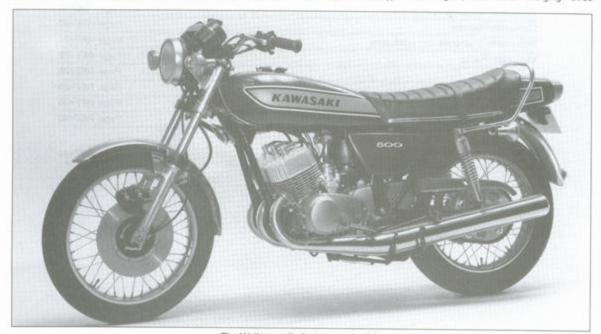
The H1 three cylinder two-stroke 500
