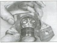
2.18b Remove the piston from the bore
