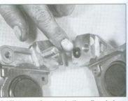
2.17b ... and separate the caliper halves; replace the O-ring with a new one
