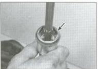
6.29a The special tool fits into the hex in the top of the cartridge (arrow)
