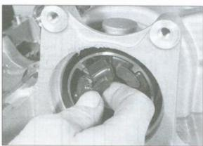
31.12 Replace the rubber damper segments if worn, brittle or deteriorated
