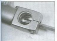
6.30a Insert an Allen wrench into the damper rod bolt . . .
