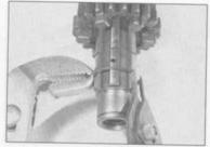
30.5b . . . holding the back of the snapring with pliers to prevent it from twisting
