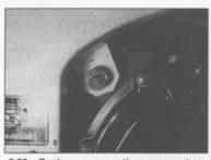
5.22a Engine rear mounting upper nut on right side . . .
