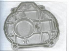
4.14 On J, K, L and M models, replace the cover O-ring if its condition is in any doubt
