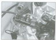
23.6 The sidestand switch is secured by two screws (arrows)
