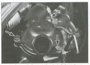
6.4 Remove the thermostat housing bolts (arrows) . . .
