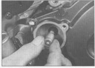
19.4d The clutch pushrod can be removed from the opposite side of the engine if the slave cylinder has been removed
