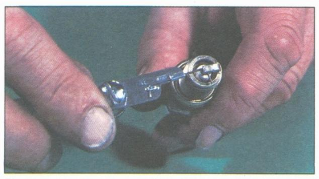
Electrode gap check - use a wire type gauge for best results
