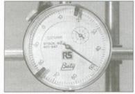
3.17 Dial gauge reading of 1.48 mm
