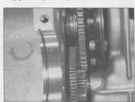
28.19b The idler gear should mesh with the starter clutch like this when installed
