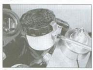
2 If the level is low, remove the cap retainer screw . . .
