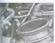
12.15 Apply a thin coat of engine oil to the rim of the air intake duct
