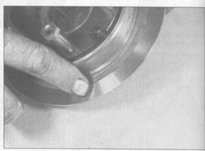
19.10b Replace the clutch hub if its friction surface is worn or damaged
