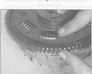
19.16b Replace the clutch housing if the springs are broken or the gear teeth are worn or damaged
