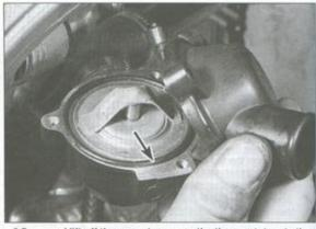
6.5 . . . and lift off the cover to expose the thermostat; note the O-ring (arrow)
