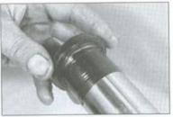
6.36d Wrap the groove in the fork tube with tape to prevent the seal from being out
