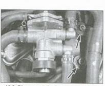
16.3 Disconnect the hoses, remove the mounting bolts (arrows) and lift the vacuum switching valve out
