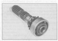
27.18 Inspect the starter idler shaft splines and sprocket; if the bearing is worn or damaged, have it pressed off
