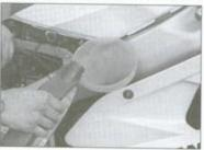
. . . and add enough oil of the recommended grade and type to bring the level up to the Maximum mark, o not overfill.
