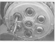
19.4a Remove the pressure plate bolts . . .
