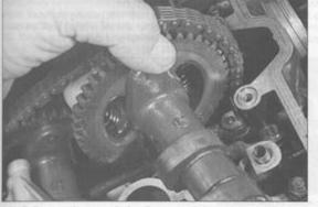
9.6a Pull up on the cam chain, disengage it from the sprocket and guide the camshaft out
