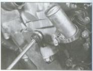
8.16a Remove the screw that secures the brace to the air baffle . . .
