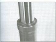
6.36g Seat the dust seal in the outer fork tube
