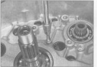
30.2a Remove the Allen bolt . . .
