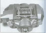
3.18 The ends of the pad springs should fit under the retaining pins like this
