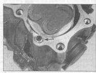
13.5a Dowel pin for the cylinder block at each front corner of the crankcase (arrow)
