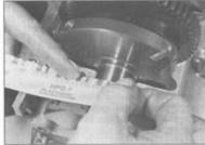
25.10 Measure the width of the crushed Plastigauge with the scale on the envelope
