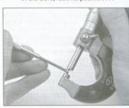
3.10 . . . then measure the gauge with a micrometer
