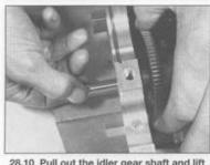
28.10 Pull out the idler gear shaft and lift out the gear
