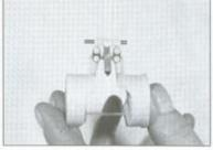
7.6c . . . and lift out the float, together with the needle valve
