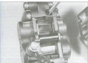
3.2 Remove the screws and lift off the pad cover
