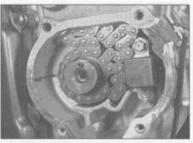
9.9b . . . if the chain is allowed to drop and bunch up like this, turning the crankshaft could cause damage
