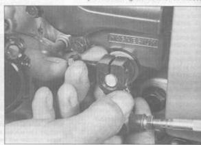
21.3 Remove the bolt and slip the lever off the shaft
