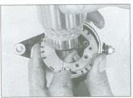
27.18a Hold the brushes back with a finger and start the armature into the brush end cover. . .
