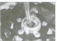
15.5 Drive the bearings from the hub with a brass drift
