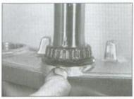
3.16 Remove the lower bearing and grease seal from the steering stem only if they're to be replaced
