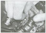
6.5 Disconnect the brake light switch connectors from the switch
