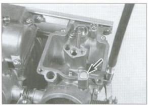
7.10a The pilot screw on US models is beneath a plug (arrow)
