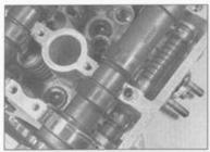
9.15 Lay a strip of Plastigauge on the camshaft journal, parallel to the camshaft centerline
