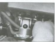
7.9d . . . then pull out the bolt and lower the shock absorber away from the bike
