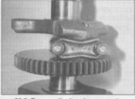
26.3 Remove the bearing cap nuts
