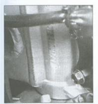
The frame number is stamped on the steering head . . .
