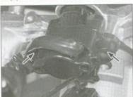
19.4 The ignition switch is secured by a pair of self-shearing screws (arrows)
