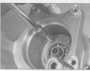
28.9 Remove the Allen bolts and take off the bearing holder
