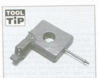
A simple spark gap testing fixture can be made from a block of wood, two nails, a large alligator clip, a screw and a piece of wire
