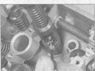
12.7b . . . compress the spring and remove the keepers (collets)
