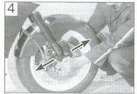
Checking the steering head bearings for freeplay
