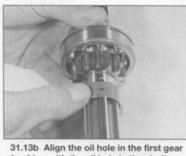
bushing with the oil hole in the shaft . . .
