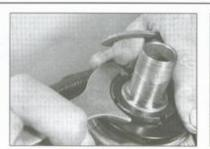
undo the nut with a spanner wrench (C-spanner) . . .
