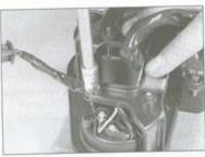
16.3a Remove the temperature gauge mounting nuts . . .
