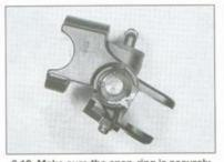
6.12 Make sure the snap-ring is securely seated in its groove
