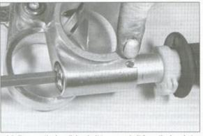
2.9 Remove the handlebar bolt to separate it from the bracket; note the alignment pin and the notch it fits into
