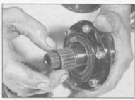
28.13d .. . and the needle roller bearing ...
