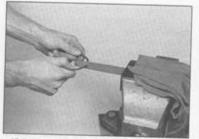
15.5 If the end gap is too small, clamp a file in a vise and file the ring ends to enlarge the gap slightly
