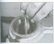
314b . . . or by inserting a drift from above to drive out the lower race . . .
