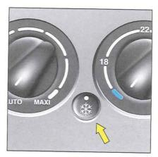
Note: A normal consequence of having the air conditioning turned on is that water condenses on the surface of the air conditioner. This drains out through a hole provided at the base of the windscreen and may form a puddle under the car when parked.
