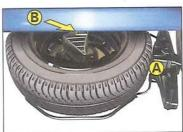
The wheel brace is stowed on the left hand side of the boot.
