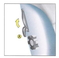
To return the seat to its normal position, push the backrest back so that it locks, and slide the seat back to its initial position.
