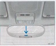
Fig. 29 Retrovisor interior antideslumbrante
