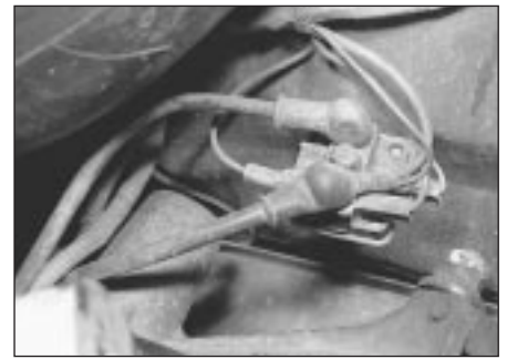
16.2 Electrical connections at the starter solenoid
