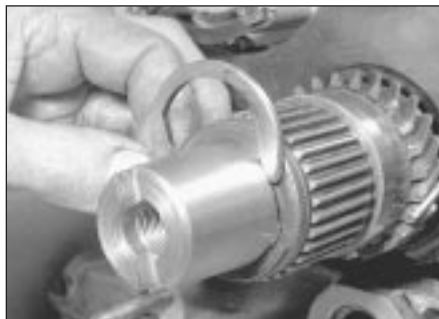
5.31b ... and the C-shaped washer
