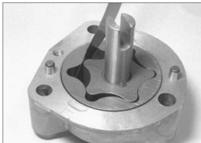
10.5a Measuring the oil pump rotor lobe clearance . . .
