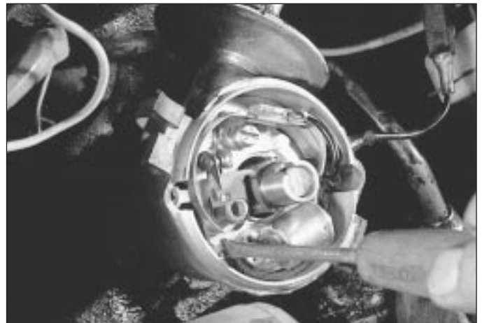
5.7 Adjusting the contact breaker points
