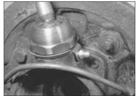
5.12b ... screw in the grease nipple ...
