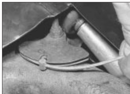
10.7 Removing the handbrake cable from the moving sector
