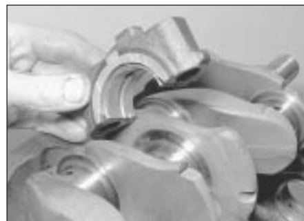
12.8 Main bearing cap with thrustwashers in position
