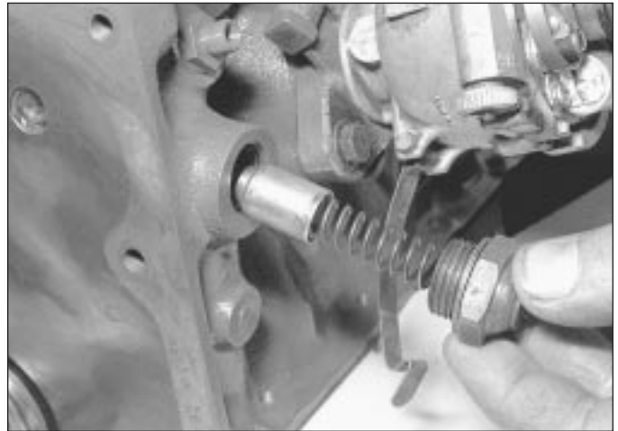
14.2 Removing the oil pressure relief valve
