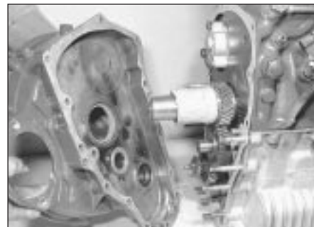
5.35 Refitting the flywheel housing
