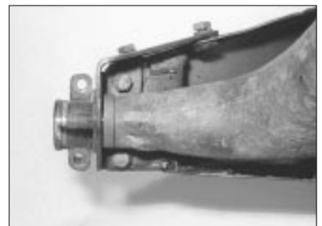
19.9 Rear radius arm outer bracket retaining bolts (subframe shown removed)
