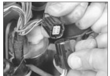
8.4 Disconnecting the exhaust system Lambda sensor wiring connector
