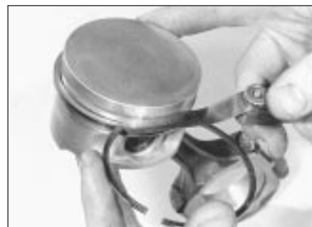
11.17 Measuring the piston ring-to-groove clearance
