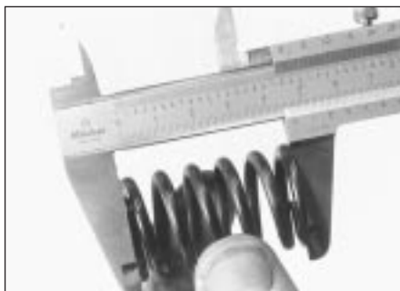
8.25 Measuring valve spring free length
