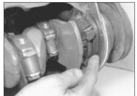
5.25 Fitting a new front oil seal . . .
