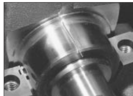
17.7 Plastigage in place on main bearing journal
