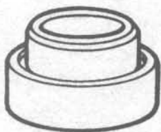
12.3 A special tool is recommended for front crankshaft seal installation
