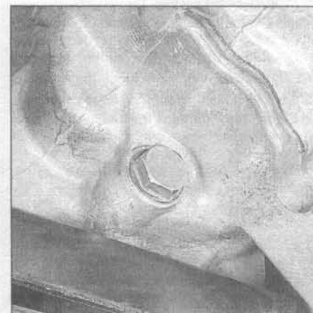
37.3 Manual transmission drain plug (4WD model shown)
