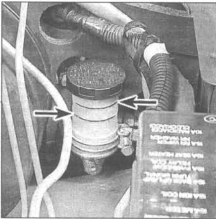
4.19b The clutch fluid level must be kept between the upper and lower marks on the fluid reservoir - unscrew the cap to add fluid
