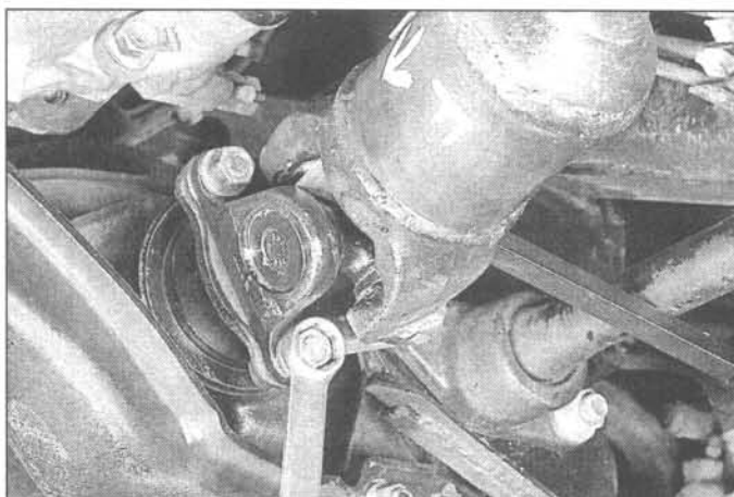
12.3 Lock the driveshaft so it can't turn, and remove the bolts
