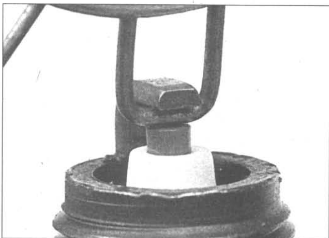
43.5a Spark plug manufacturers recommend using a wire-type gauge when checking the gap - if the wire does not slide between the electrodes with a slight drag, adjustment is required
