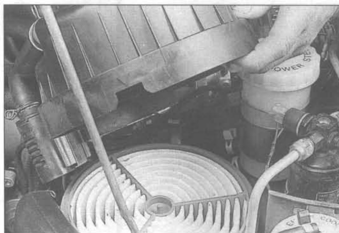
29.9 With the hoses still attached, pull the cover up, then lift the element out of the housing
