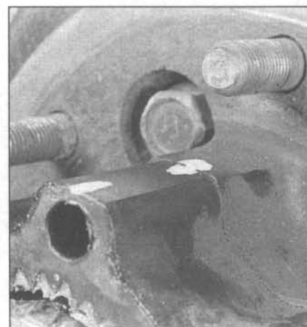
18.5a Mark the relationship of the housing ...
