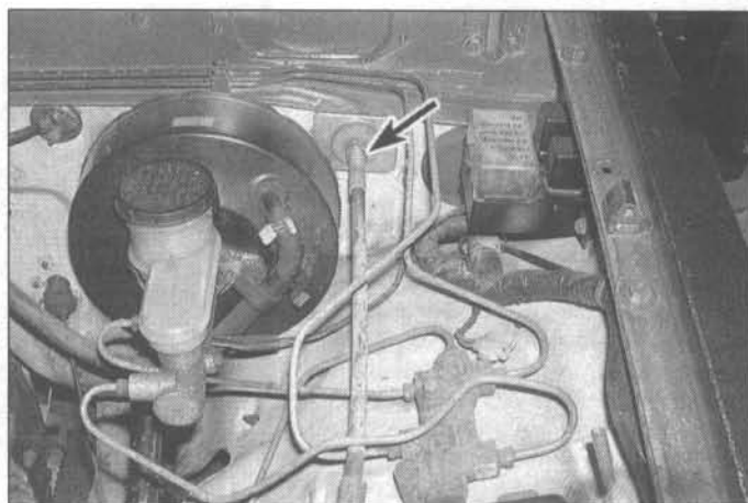
19.4 On cable-operated models, adjust the clutch to achieve the specified play between the nut (arrow) and the rubber cushion
