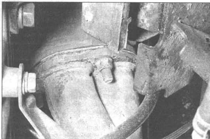
19.4 Apply penetrating oil to the exhaust pipe flange nuts before attempting to remove them
