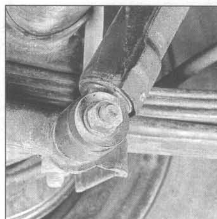
10.3 The lower mounting nut on the rear shock absorber
