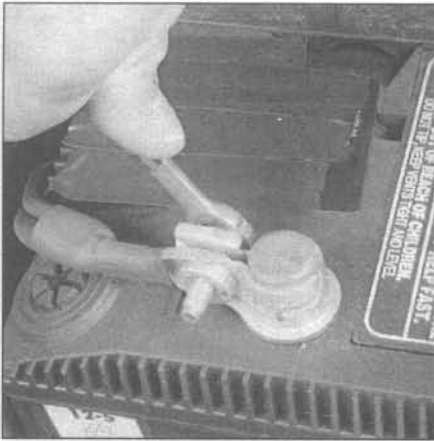
8.6 Removing a cable from the battery post with a wrench - sometimes a special battery pliers is required for this procedure if corrosion has caused deterioration of the nut hex (always remove the ground cable first and hook it up last!)
