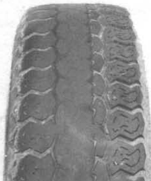
INCORRECT TOE-IN OR EXTREME CAMBER
