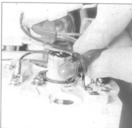
12.4 After removing the instrument cluster, turn the bulb holders, lift them out and withdraw the bulbs
