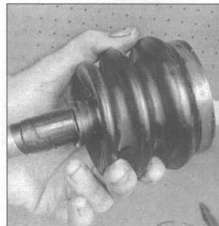
20.14 Wrap the splined area of the axle shaft with tape to prevent damage to the new boot
