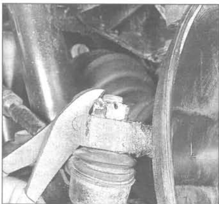
13.10a Use wire cutters or pliers to remove the cotter pin
