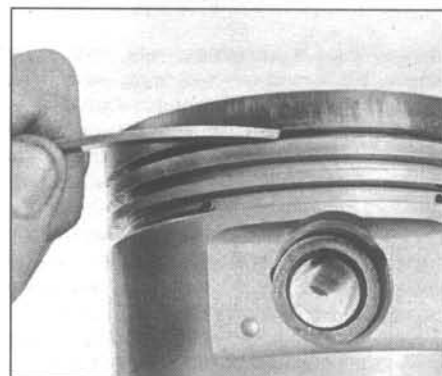
17.4b ... or a section of a broken ring
