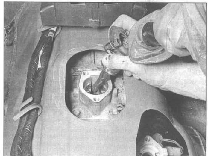
3.4 Lift the shift lever straight up and out of the transmission - be careful not to lose the spring
