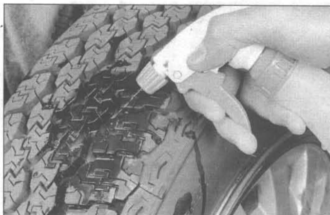
7.4b If the valve core is tight, raise the corner of the vehicle with the low tire and spray a soapy water solution onto the tread as the tire is turned - slow leaks will cause small bubbles to appear
