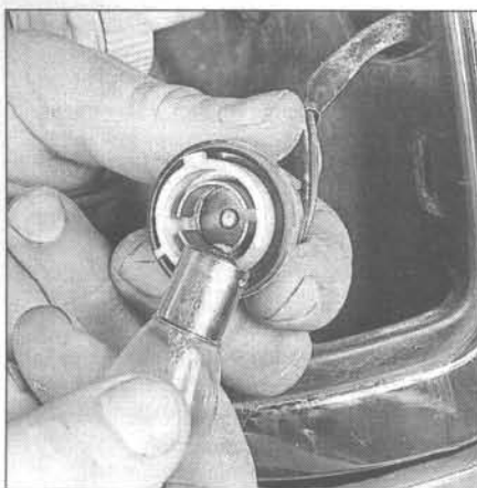
12.3a Push the bulb in, rotate it counterclockwise and withdraw it from the housing
