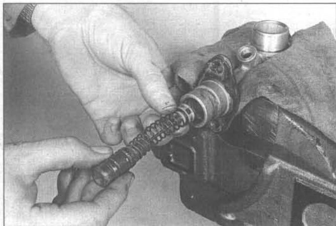
7.5 Remove the piston and spring from the bore of the master cylinder; note that the seal lip faces forward, toward the front of the master cylinder
