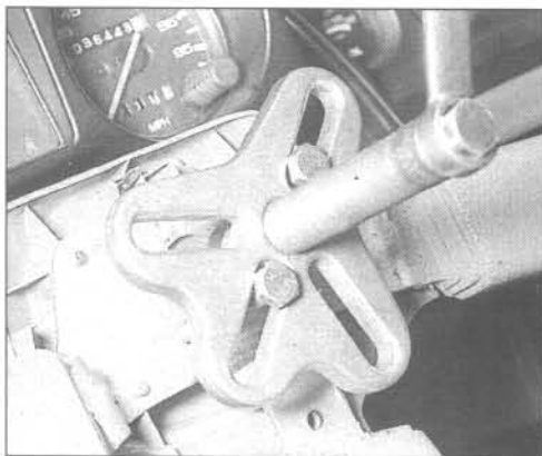
12.4 Remove the steering wheel from the shaft with a puller – DO NOT hammer on the shaft!
