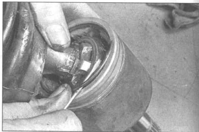
20.4 Pry the circlip from the outer race with a screwdriver
