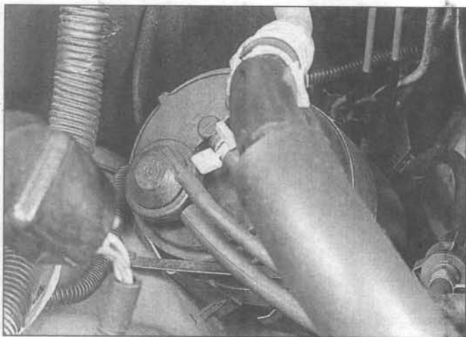
33.2 The charcoal canister is attached to the firewall on the passenger side of the engine compartment - check the canister housing and hoses for damage
