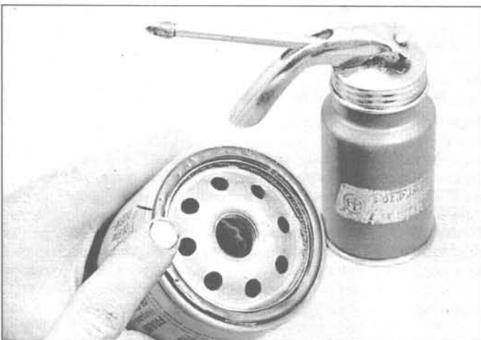
13.18 Lubricate the rubber gasket with clean oil before installing the filter on the engine
