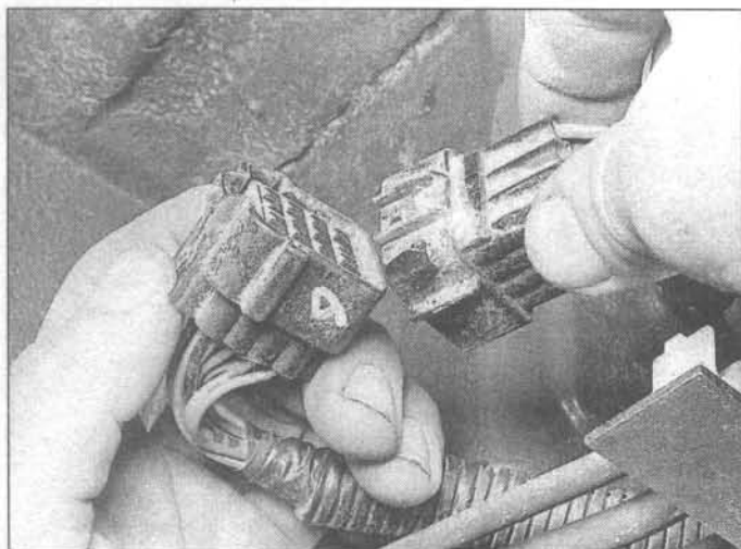
5.4 Disconnect the fuel tank electrical connector
