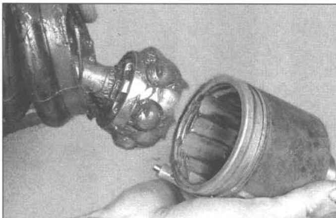
20.5 With the retainer removed, the outer race can be pulled off the bearing assembly
