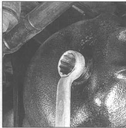
22.2 Use a box-end wrench to remove and install the differential plugs to avoid rounding off the hex
