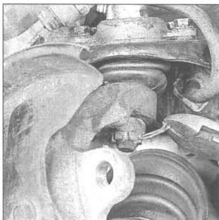
8.6a Use wire cutters or pliers to remove the cotter pin
