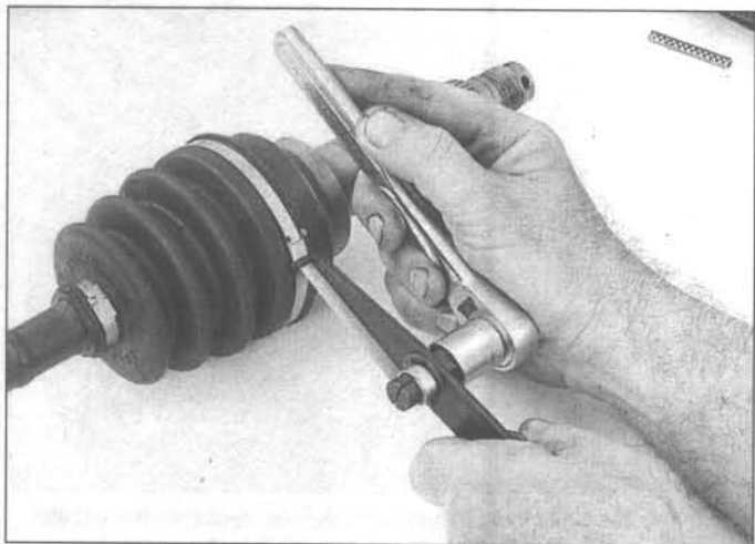
20.16a Secure the boot clamps with a special banding tool such as the one shown here (available at most auto parts stores): install the clamp, thread it onto the tool, pull the clamp tight . . .
