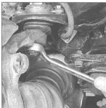
8.6b Unscrew the balljoint nut two turns
