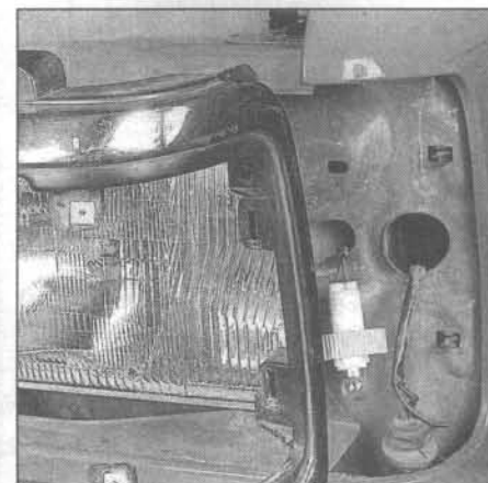
10.8b . . . disconnect the bulbs and pull the housing forward for access to the headlight bulb
