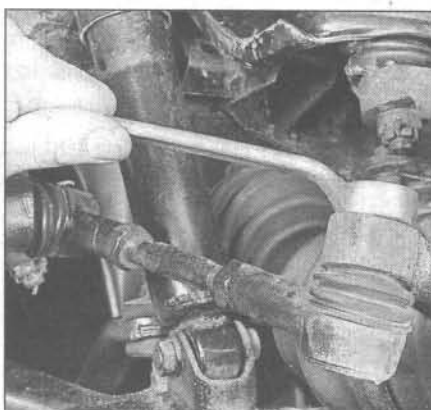
13.10b Unscrew the tie-rod end nut at the steering knuckle
