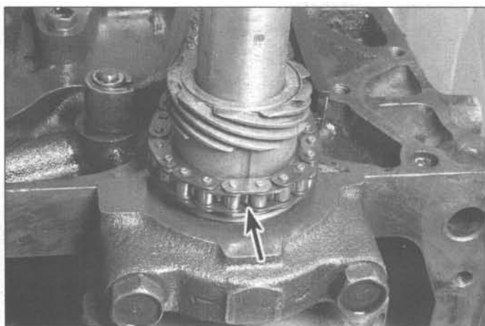
16.11 With the camshaft timing sprocket mark at top dead center, position the crankshaft sprocket and chain timing marks (arrow) as shown
