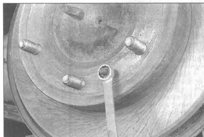
4.8 On rear discs, separate the brake disc from the hub by threading a bolt into the hub
