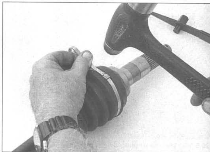
20.16b . . . peen over the locking tabs . . .
