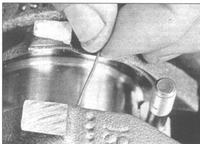
24.13 Lay the Plastigage strips on each rod bearing journal, parallel to the crankshaft centerline
