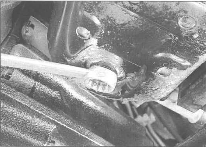
13.9 The engine oil drain plug is located at the rear of the oil pan (four-cylinder engine shown) - it's usually very tight, so use a box-wrench or six-point socket to avoid rounding off the hex
