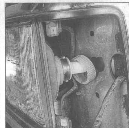
10.9 Unscrew the retaining collar and slide it back so the bulb can be pulled out of the housing
