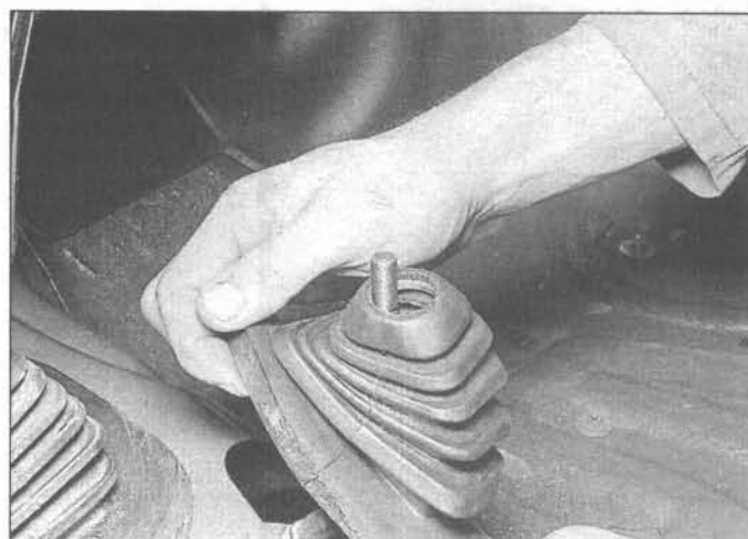
2.2b ... and pull the shift boot out of the body opening
