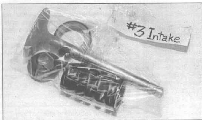
8.2 Have several plastic bags ready (one for each valve) before disassembling the head - label each bag and put the entire contents of each valve assembly in one bag as shown
