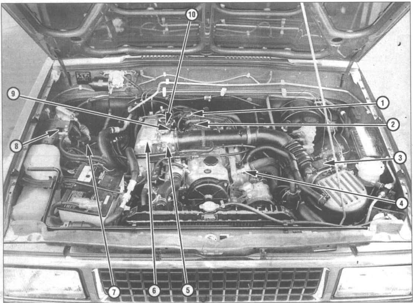
1.8 Multi-port (I-TEC) fuel injection system component locations
