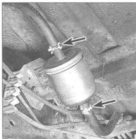
30.7 Detach the hoses (arrows), then unbolt the fuel filter from the bracket (fuel injected models)
