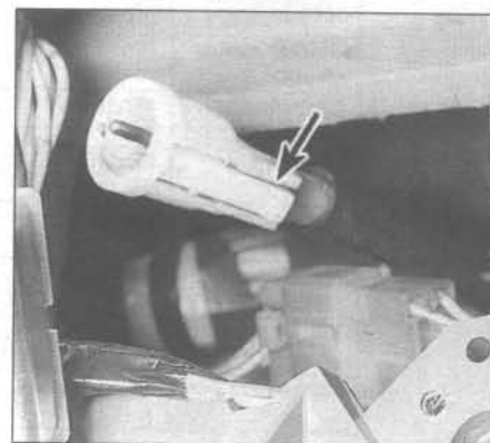
14.4 Press on the release lever (arrow) and detach the speedometer cable from the cluster
