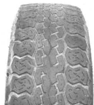
FEATHERING DUE TO MISALIGNMENT
