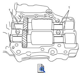
**4)** Install balancer shaft cover to oil pump housing.
