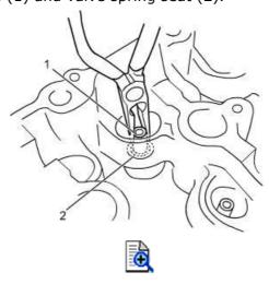
**7)** Use special tool to remove valve guide from combustion chamber side to valve spring side.
