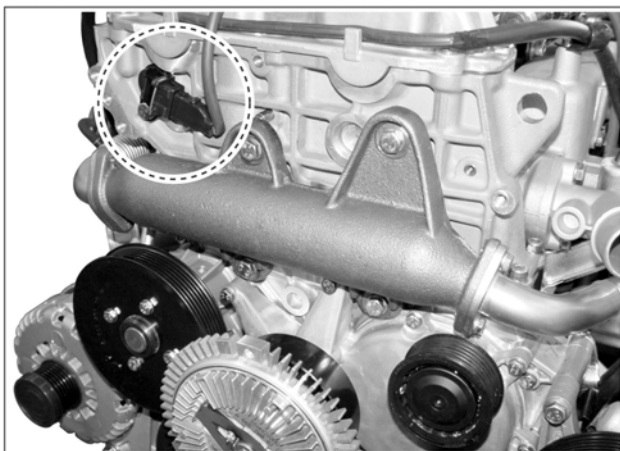
<Location of Camshaft Position Sensor>
