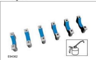
**3. NOTE:** Make sure that these components are installed to the noted removal position.
