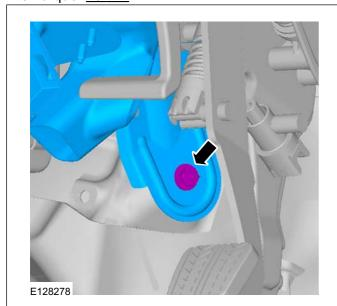
26. On both sides. Torque: 25 Nm
