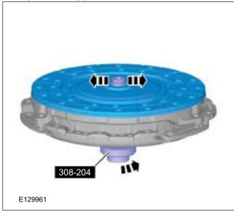
**2. NOTE:** Check the pilot bearing for damage. If damaged, install a new pilot bearing.
