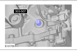
19. Remove the bolt M6 x 18 mm.
