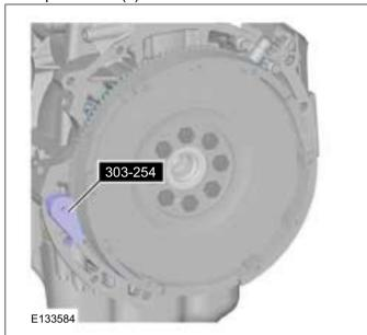
4. CAUTION: Loosen the clutch pressure plate retaining bolts by two turns at a time in the sequence shown.
