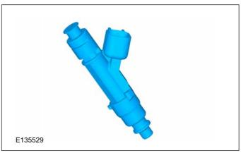
The electromagnetically controlled injectors dose and atomize the fuel. The quantity of injected fuel is regulated by the duration of actuation of the fuel injectors. The fuel injectors are either closed (not actuated) or opened (actuated). Each cylinder has its own injector. The injection is accurately dosed and takes place at a time determined by the PCM. Injection takes place immediately in front of the intake valves of the cylinder.
