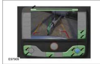
If the blue button is pressed during operation of the reversing camera, the camera view disappears from the screen. When reverse gear is engaged again, the system returns to the camera view. Exception: For incoming telephone calls, the screen shows the corresponding menu and then automatically returns to the camera view.
