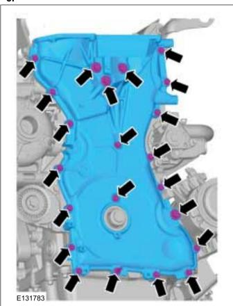
Apply sealant to the engine front cover (bead diameter: 3 mm).
