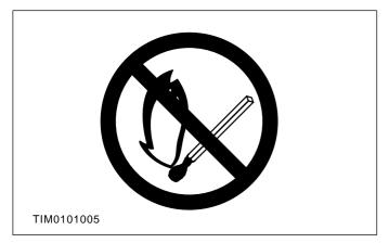
Displaying the caution circle with a deleted lighted match symbol, caution against the use of naked lights or flames within the immediate vicinity due to the presence of highly flammable or explosive liquids or vapors. See Fire in this subsection.
