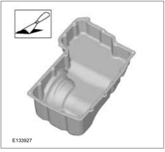
2. CAUTION: Install the oil pan within five minutes of applying the sealer.
