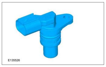
A sensor is installed for the intake camshaft. The CMP sensor is used by the PCM for cylinder number one recognition so that the injection sequence can be determined.
