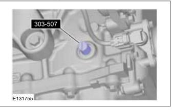
**40.** Mark the balancer unit and shafts on the top for reference that the balancer unit is at TDC.
