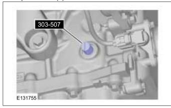
**13.** Reposition the camshaft alignment plate to the slot on the rear of the intake camshaft only.
