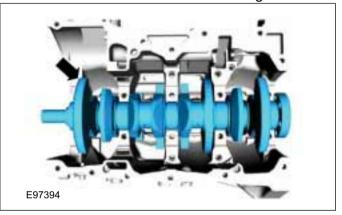
**40. NOTE:** If the main bearings are being reused, mark them in order for correct orientation and reassembly.
