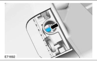
2. CAUTION: The tip of the sensor must rest on a flywheel tooth.
