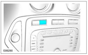
The parking aid switch is located in the instrument panel, above the audio unit or navigation system display module. The parking aid switch is equipped with an integral LED.
