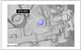
**7. NOTE:** Only tighten the bolt finger tight at this stage.
