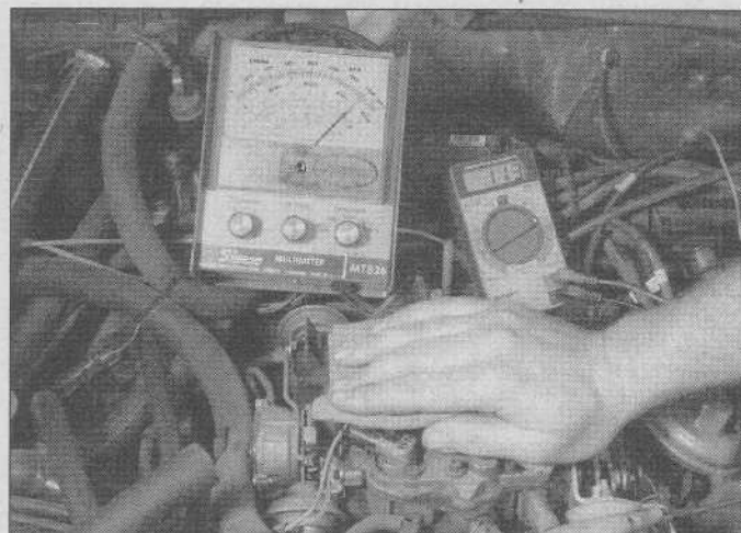
5.15 Place a rag over the carburetor air horn and watch the dwell go LEAN to compensate for a rich running condition
