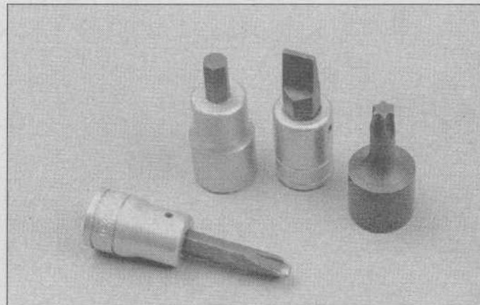
2.9 Standard and Phillips bits, Allen-head and Torx drivers will expand the versatility of your ratchet and extensions even further
