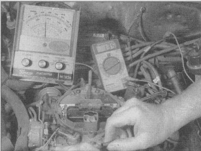
5.16 Disconnect a vacuum line and observe the dwell "on time" indicate rich (low reading) to compensate for the lean running condition
