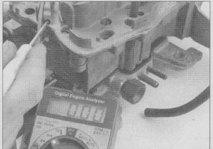
7D.91 . . . then use a small screwdriver to turn the adjusting screw until the voltage readings are correct
