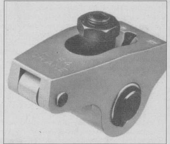
8.29 Roller rocker arms reduce friction, add horsepower and ensure more stable valve lash
