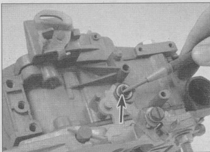
7D.15 Once the housing has been removed, carefully lift out and discard the choke shaft seal (arrow). Replace it with a new seal during reassembly.
