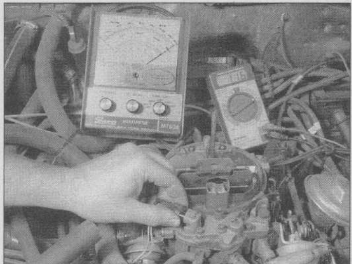
5.18 With the dwellmeter and tachometer properly installed, disconnect the M/C solenoid connector and observe the gauge. Rpm should drop below 300 from normal.
