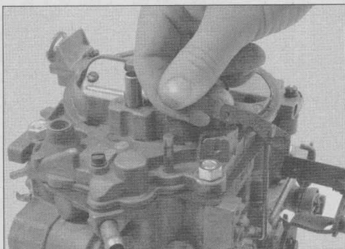
7D.16b . . . just far enough to lift the lever from the air horn and disconnect it from the rod.
