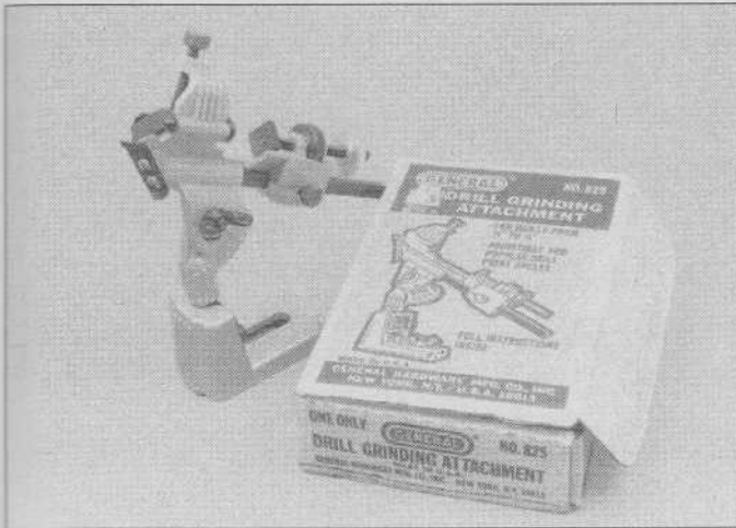
2.43 Inexpensive drill bit sharpening jigs designed to be used with a bench grinder are widely available - even if you only use it to re-sharpen drill bits, it'll pay for itself quickly
