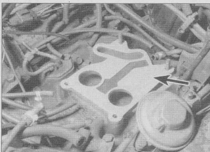
6.12 Always use a new carburetor base gasket (arrow). Old ones become crushed and hardened due to age and heat, and can't provide the kind of seal needed to prevent vacuum leaks (a very common source of driveability problems).
