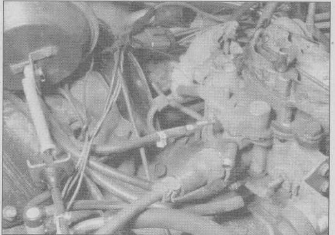
6.5 Be sure to label each vacuum line and its corresponding port with a paint mark or pieces of numbered tape
