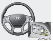
3. Move the lever (1) down (to SET-), and release it at the desired speed. The SET indicator light in the instrument cluster will illuminate. Release the accelerator pedal. The desired speed will automatically be maintained.
