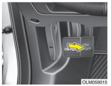
**Releasing the parking brake** Foot type
