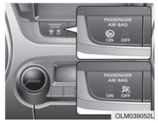
To deactivate or reactivate the passenger's front air bag:
