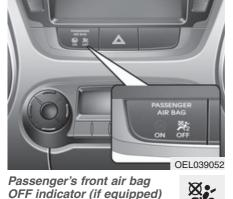
The passenger's front air bag ON indicator illuminates for approximately 4 seconds after the ignition switch is turned to the ON position.
