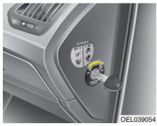
Passenger's front air bag ON/OFF switch (if equipped)
