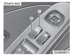
*With central door lock switch* Operate by depressing the central door lock switch.
