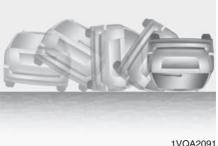
· Air bags may not inflate in rollover accidents because air bag deployment would not provide protection to the occupants.
