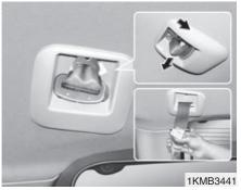
*3 Point rear center belt (if equipped)* To fasten the rear center belt
