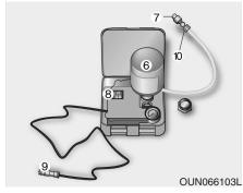
4. Screw the bottle clockwise into the bottle socket (6) until it is tight.
