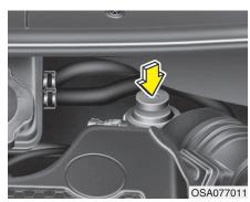
2. Pump up and down until the fuel flows out of the plug opening.
