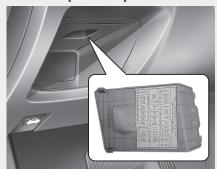
Engine compartment sub fuse panel (Gasoline only)
