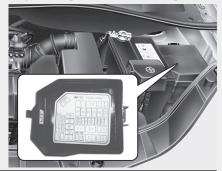
Engine compartment sub fuse panel (Diesel only)
