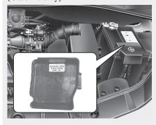
Engine compartment main fuse panel
