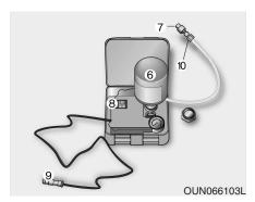
10. Switch the On/Off switch (8) to the "I"-position.
