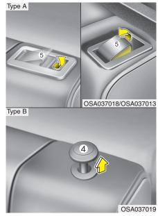
6. Pull up the lock release lever (4), (5).
