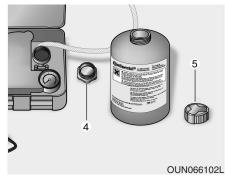
3. Unscrew the bottle holder cap (4) and the lid of the sealant bottle (5).
