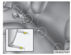
On each side of the rear seat, between the cushion and backrest, are located a pair of ISOFIX anchorage points together with a top tether mounting on the tranverse trim behind the rear seats. During the installation, the seat has to be engaged at the anchorage-points in a way you can hear it clicking (check by pulling!) and has to be fixed with the Top Tether-belt on the belonging point on the floor behind the rear seats.
