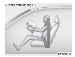
The front air bag modules are located both in the center of the steering wheel and in the front passenger's panel above the glove box. When the SRSCM detects a sufficiently severe impact to the front of the vehicle, it will automatically deploy the front air bags.
