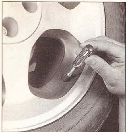
5.4a If a tire loses air on a steady basis, check the valve stem core first to make sure it's snug (special inexpensive wrenches are commonly available at auto parts stores)
