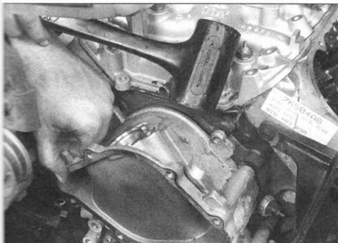
10.10a Gently tap the timing chain cover loose with a soft-face hammer (V6 engine shown)
