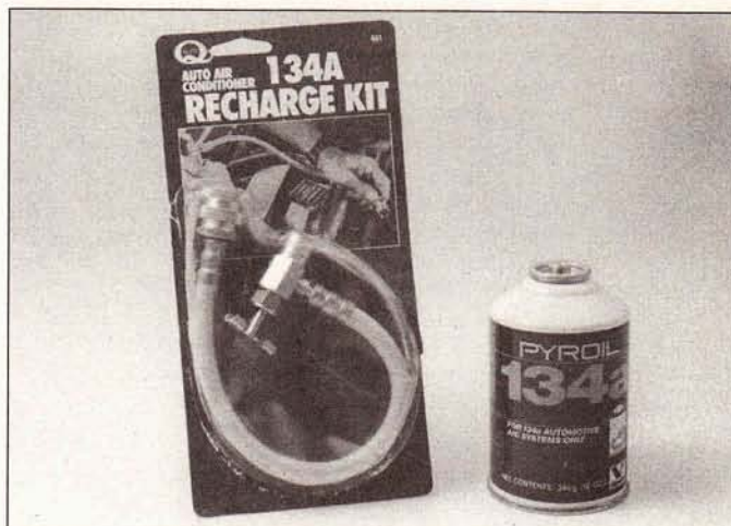
14.9 A basic charging kit for R-134a systems is available at most auto parts stores - it must say R-134a (not R-12) and so must the 12-ounce can of refrigerant
