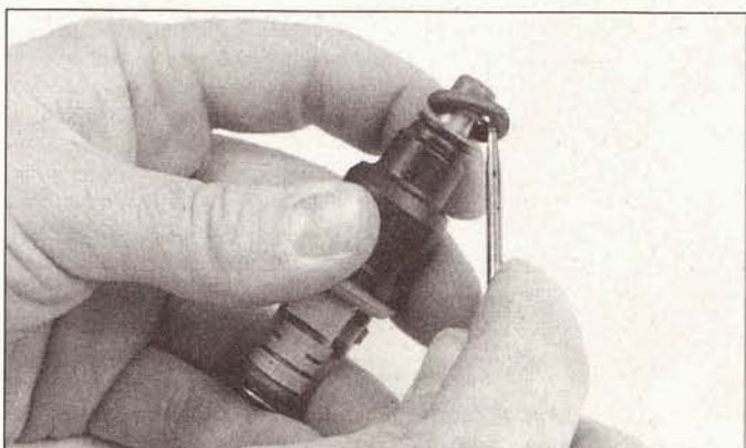
13.57b . . . then remove the lower O-ring from the injector
