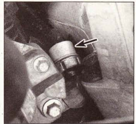
2.4c oil pressure sender location, 3.8L V6 - left side of the block, under the power steering pump
