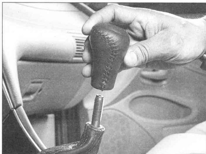
2.1 To remove the shift lever knob from the shift lever, simply unscrew it
