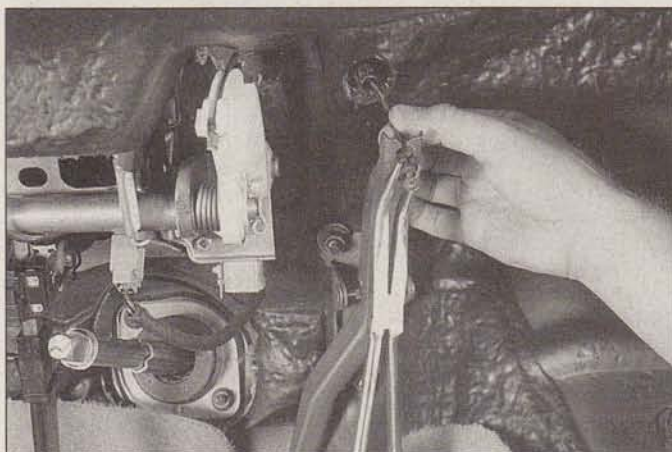
10.5 Working under the dash in the driver's side compartment, pull the cable end from the accelerator pedal recess (4.6L DOHC shown)
