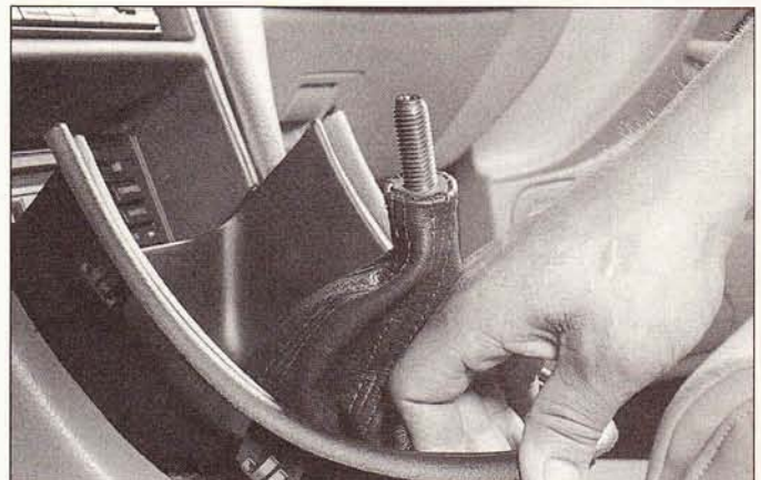
23.2 Pry out the gear selector trim bezel
