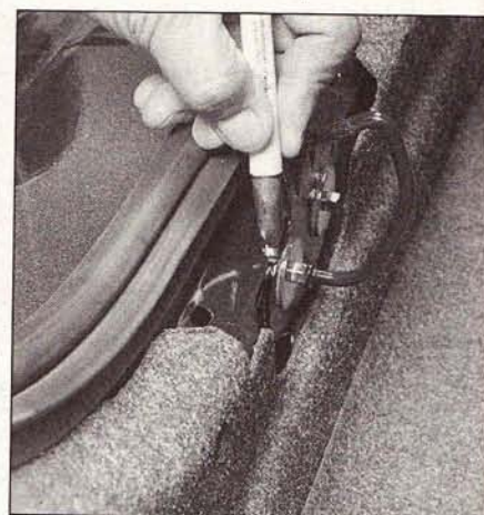
14.10a Scribe a mark around the striker assembly as a reference point to aid in the adjustment procedure
