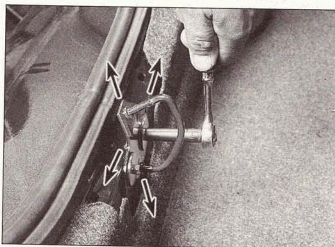
14.10b Loosen the bolts and move the striker assembly as necessary (arrows) to adjust the trunk lid flush with the quarter panels in the closed position
