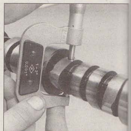
9.10c ... and subtract the camshaft lobe diameter at its smallest dimension to obtain the lobe lift specification
