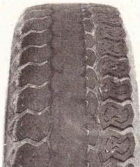
INCORRECT TOE-IN OR EXTREME CAMBER
