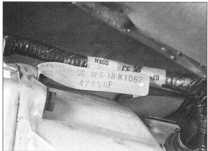
The manual transmission identification tag is retained by a left side engine-to-bellhousing bolt
