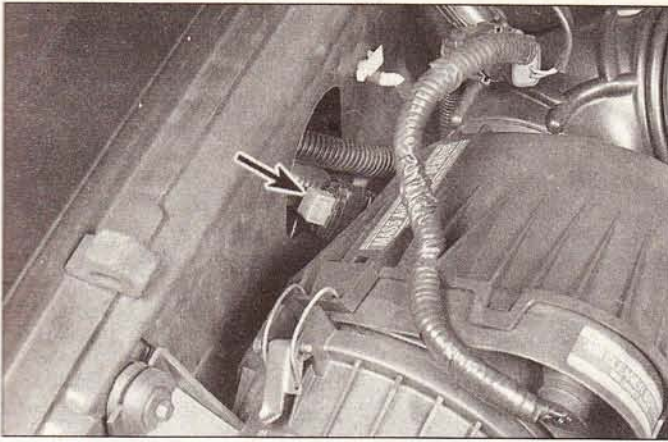
9.3 Before adjusting the ignition timing, unplug the SPOUT (arrow) (single wire connector) attached to the ignition module wire harness (if you do not, the EEC-IV system will still be controlling the base ignition timing)
