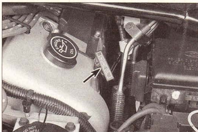
4.2 The oil dipstick is located on the driver side of the engine
