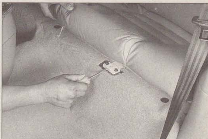
29.5 Press down on the release button to remove the rear seat cushion
