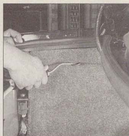
11.12b Pry out the clips securing the trunk compartment driver and passenger side finishing panels
