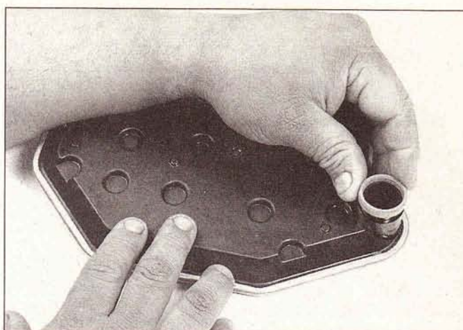
27.11 Install a new seal on the transmission filter
