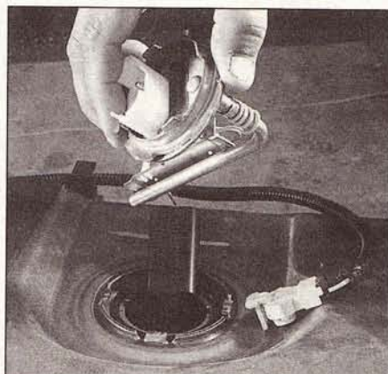
8.8 Lift the sending unit from the fuel tank without damaging the float unit
