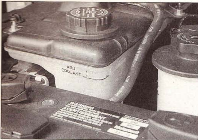
4.9 The coolant expansion tank is located on the front of the engine compartment - keep the level near the arrow at the seam
