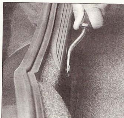
18.6 Detach the clips securing the trunk compartment rear finishing panel
