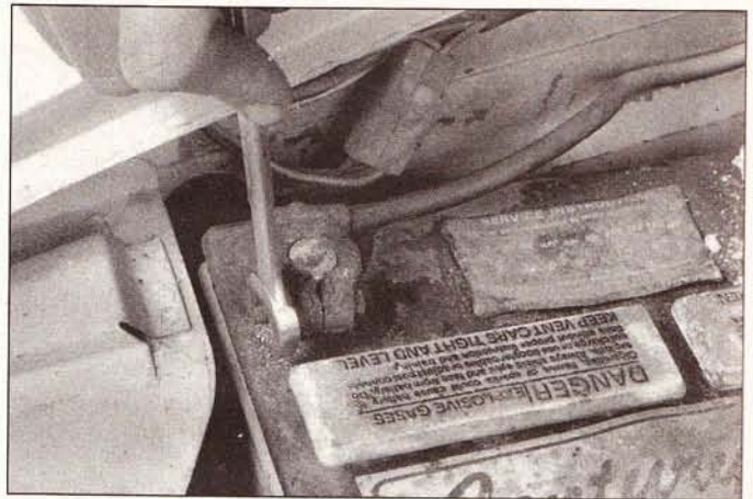
10.6b Removing the cable from a battery post with a wrench - sometimes special battery pliers are required for this procedure if corrosion has caused deterioration of the nut hex (always remove the ground cable first and hook it up last!)
