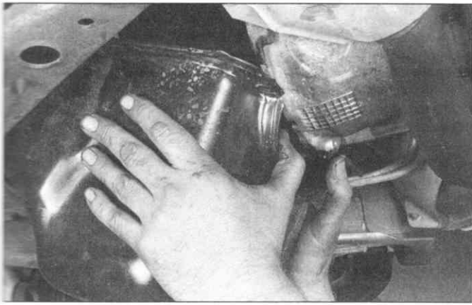
14.18 Slip the oil pan out, turning it slightly to clear the flywheel/driveplate
