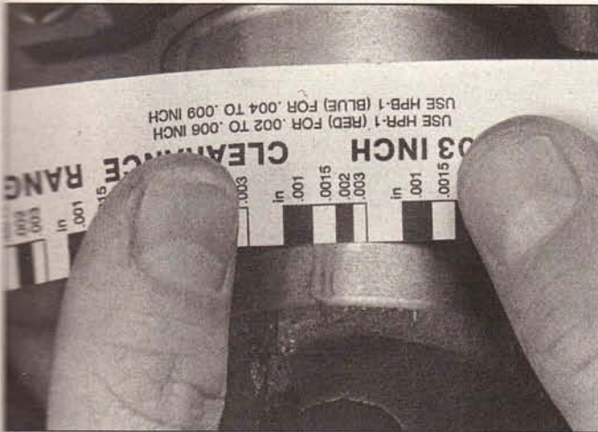
24.18 Measuring the width of the crushed Plastigage to determine the rod bearing oil clearance (be sure to use the correct scale - standard and metric ones are included)
