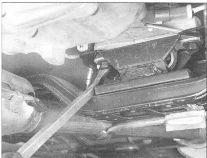
4.2 To check the transmission mount, pry between the crossmember and the mount - there should be very little movement
