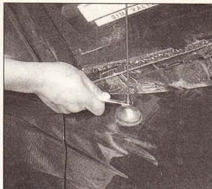
13.2 Use a small wrench to remove the antenna mast
