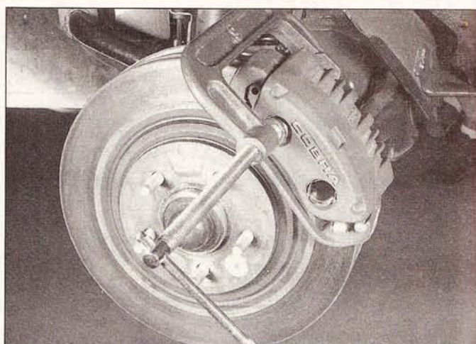
3.7b Insert a socket in one of the holes in the caliper and install a C-clamp, as shown, with one clamping pad on the caliper body and one on the socket, then compress the pistons until they bottom out
