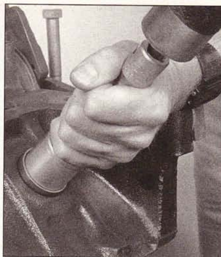
15.10 A large socket on an extension can be used to drive the new core plugs into the bores
