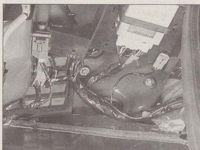
11.13b Detach the retaining nuts on each side of the trunk securing the bumper cover to rear quarter panels
