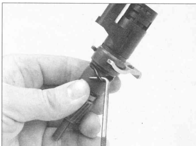
3.9 To replace the O-ring on the speed sensor, simply pull it off with a hooked tool, but be careful not to scratch the seal groove; be sure to lubricate the new O-ring with clean oil so it doesn't become twisted when the sensor is installed
