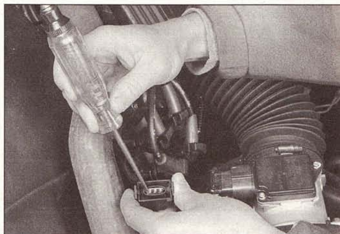
10.25 Connect a LED test light on the coil negative (-) terminals on the ignition coil connectors and watch for a blinking light when the engine is cranked (4.6L SOHC shown)
