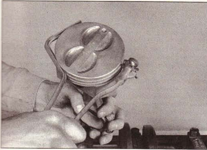
18.4a The piston ring grooves can be cleaned with a special tool, as shown here . . .
