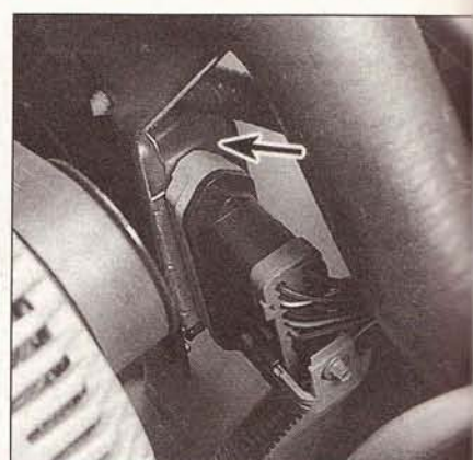
4.8a Location of the CCRM (arrow) on 1994 and 1995 models (to the right of the fan shroud)
