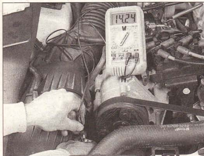
4.47 Disconnect the air conditioning clutch harness connector and check for battery voltage with the system activated (ignition key ON - engine not running)
