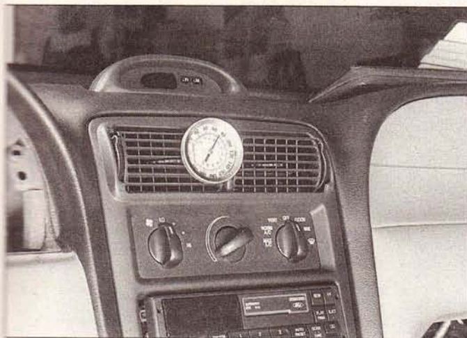
14.7 Place an accurate thermometer in the center dash vent, turn the air conditioning on and check the output temperature
