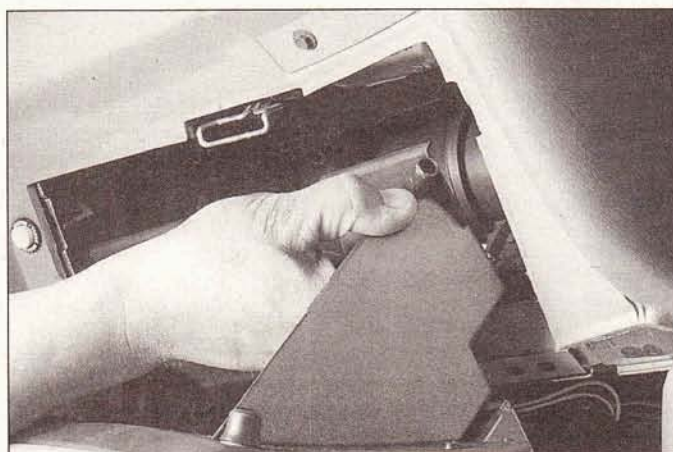
25.11 Push inward to release the glove box door stops - pull straight out to remove it from the vehicle
