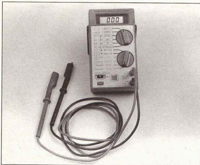
2.1 Digital multimeters can be used for testing all types of circuits; because of their high impedance, they are much more accurate than analog meters for measuring millivoltage-voltage in low-voltage computer circuits
