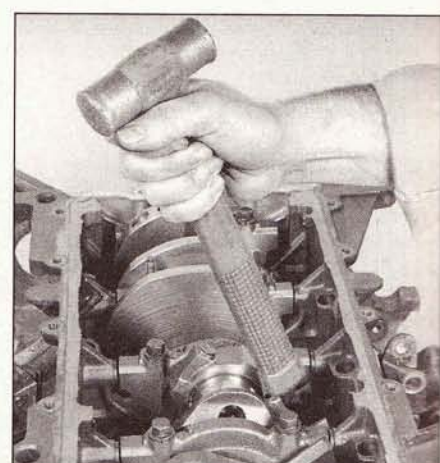
13.8 Use a hammer handle to drive the piston and connecting assembly down and out of the cylinder block, being very careful not to nick the crankshaft on the way out
