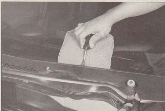
28.3 Detach the retaining clips securing the top cowl cover . . .
