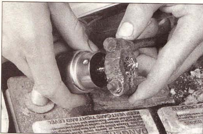
10.7a When cleaning the cable clamps, all corrosion must be removed (the inside of the clamp is tapered to match the taper on the post, so don't remove too much material)
