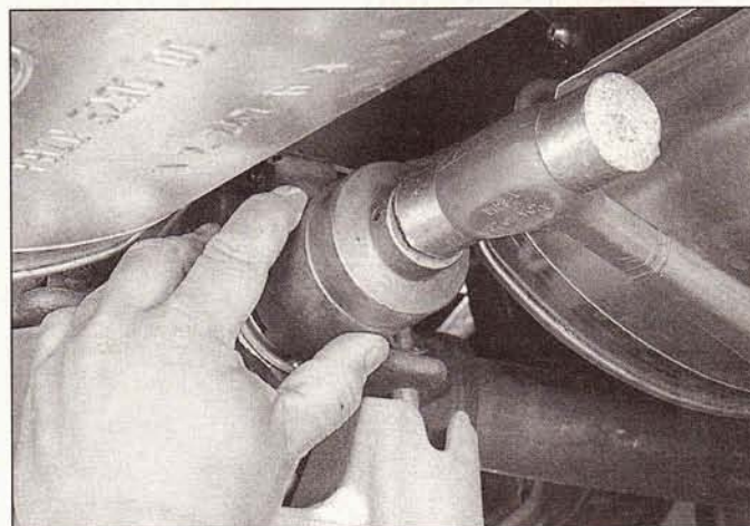
11.8 Using a seal driver or a large socket, tap the new pinion seal into place with the seal square to the bore
