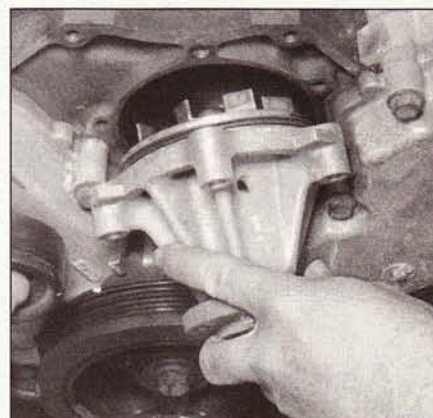
9.9c . . . and remove the water pump from out of the engine block - if it sticks, knock it loose with a soft-face hammer (or a hammer and a block of wood)
