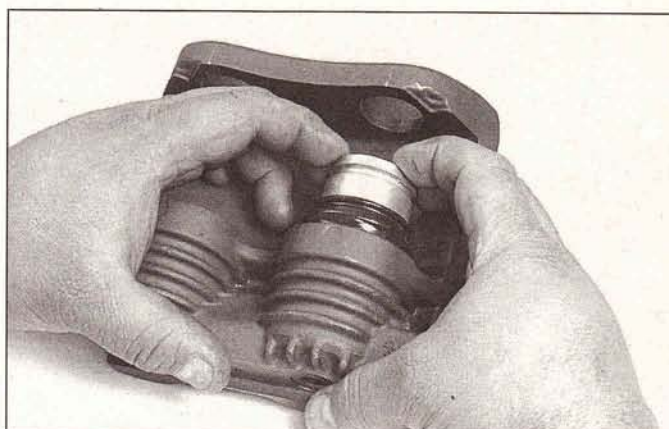
4.31 Seat the outer edge of the dust boot into its groove in the bore, position the piston square to the bore and compress it by hand as far as you can
