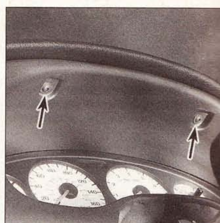
24.3 Detach the bezel retaining screws (arrows) then pull the bezel outward to disengage the lower clips
