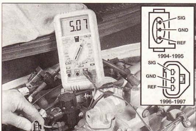
4.25 Check the reference voltage to the TPS with a voltmeter. Backprobe terminal REF with the positive (+) probe and GND (-) with the negative probe of the voltmeter and make sure the reference voltage is approximately 5.0 volts
