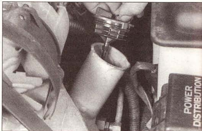
6.5a A dipstick is used to check the power steering fluid level on 3.8L and 5.0L engines
