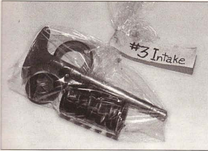
9.1 A small plastic bag, with an appropriate label, can be used to store the valve train components so they can be kept together and reinstalled in the original position
