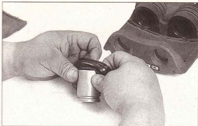
4.30 Lubricate the pistons with clean brake fluid and install the new dust boots onto the bottom of each piston
