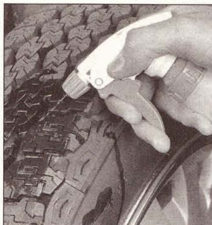
5.4b If the valve stem core is tight, raise the corner of the vehicle with the low tire and spray a soapy water solution onto the tread as the tire is turned slowly - leaks will cause small bubbles to appear
