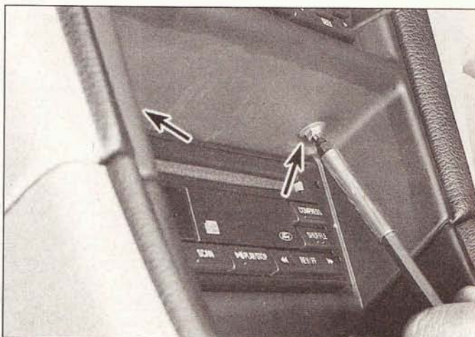
25.7a Remove the screws (arrows) securing the lower half of the center trim panel
