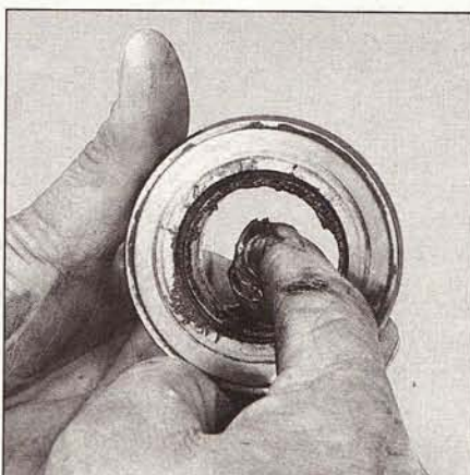
5.6e Lubricate the inner hub and the thrust side (where the release fingers contact it) of the release bearing with high-temperature grease
