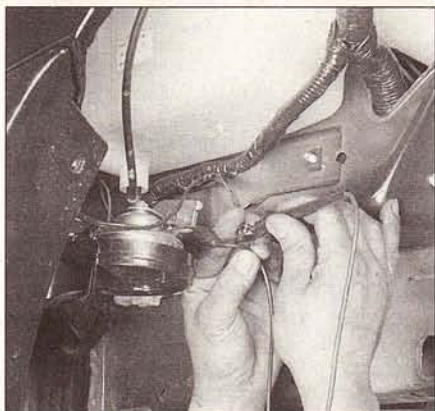
22.3 Connect a voltmeter to the horn wire and ground - test for voltage while the switch is depressed
