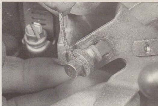
10.2a Remove the accelerator cable end from the throttle lever by twisting until the flattened edge aligns with the keyed slot (3.8L engine shown)
