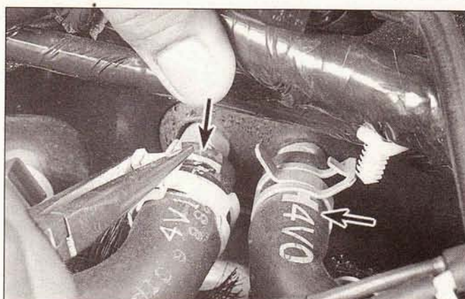
13.3 Slide the clamps back and disconnect the heater hoses from the heater core inlet and outlet pipes (arrows) at the right side of the firewall
