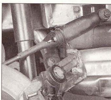
3.8d Hang the caliper from the axle damper with a piece of coat-hanger wire
