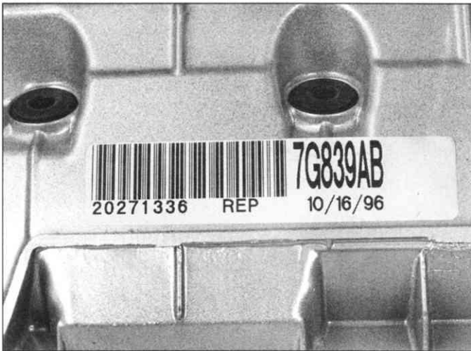
The engine identification label is affixed to the valve cover
