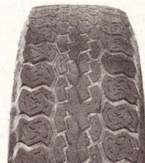
FEATHERING DUE TO MISALIGNMENT
