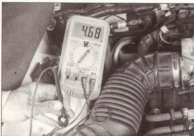
4.59 Check for reference voltage to the IAT sensor with the ignition key ON (engine not running). It should be approximately 5.0 volts
