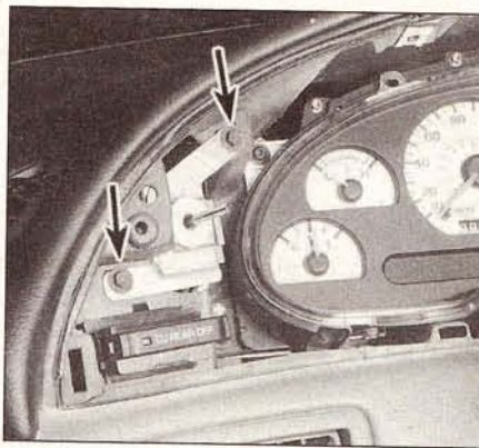
11.5 Detach the switch retaining screws (arrows) - unplug the electrical connector and withdraw the switch from the instrument panel
