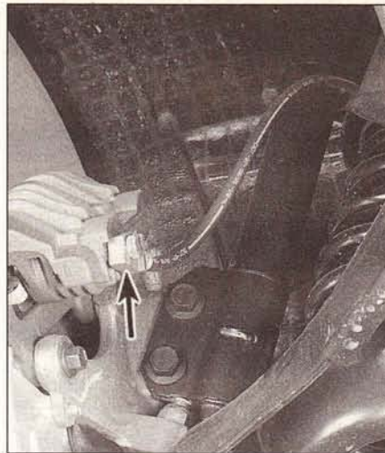
18.11 Check along the brake hoses and at each fitting (arrow) for deterioration and cracks
