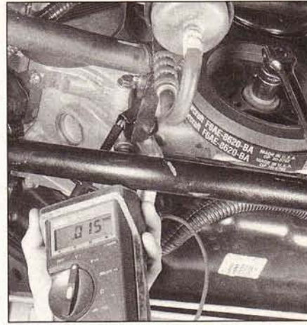
4.68 With the voltmeter set on the AC scale, check for a pulsing voltage signal between 0 and 0.05 volts as the engine is slowly rotated
