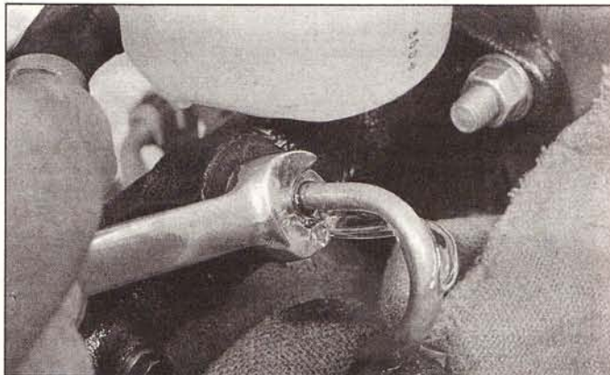
6.26 Have an assistant depress the brake pedal and hold it down, then loosen the fitting nut, allowing the air and fluid to escape; repeat this procedure on both fittings until the fluid is clear of air bubbles
