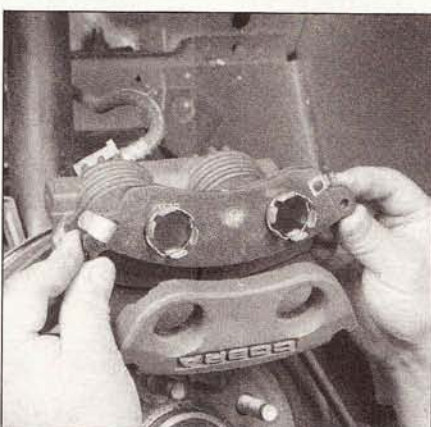
3.7g ... and remove it from the caliper
